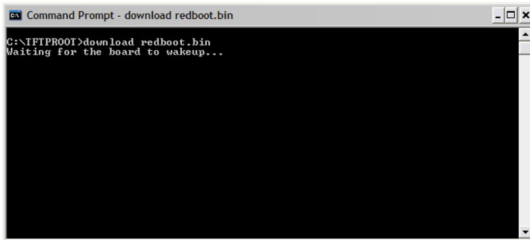
2. At this point, the download program is waiting for the user to press AND hold down pushbutton S1 *SERIAL BOOT*. While holding down S1, press and release pushbutton S3 */POR*. Keep holding down S1 until red LED D2 (next to the flashing green LED) is no longer illuminated. Afterwards, release S1. You should then see the following in the Command Prompt window.
