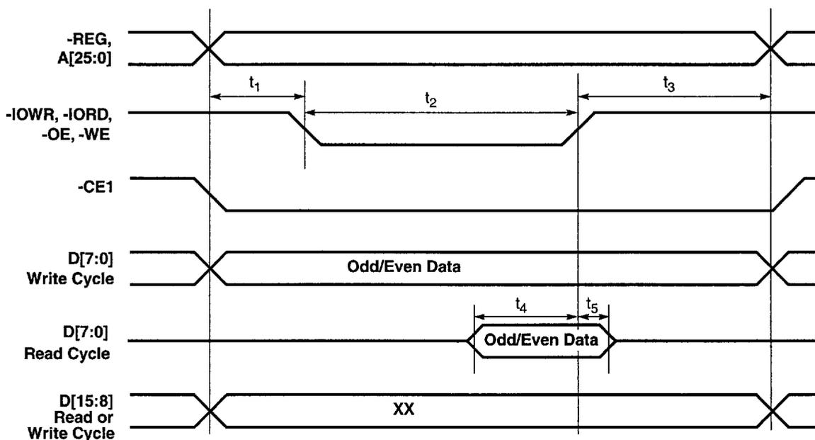
**Figure 13-8. PCMCIA Read/Write Timing when System is 8 Bit (SBHE Tied High)**
