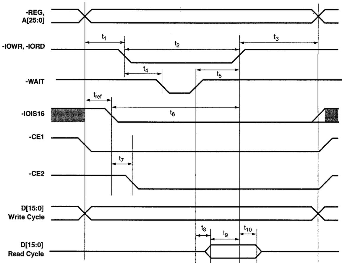
Figure 13-7. Word I/O Read/Write Timing
