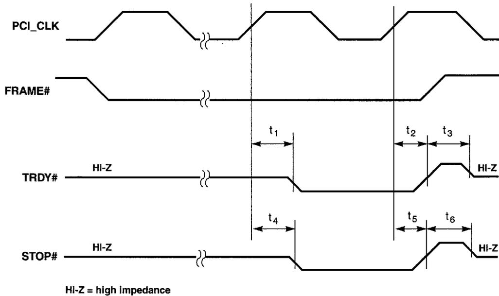
Figure 13-2. TRDY# and STOP# Delay (PCI™ Bus)
