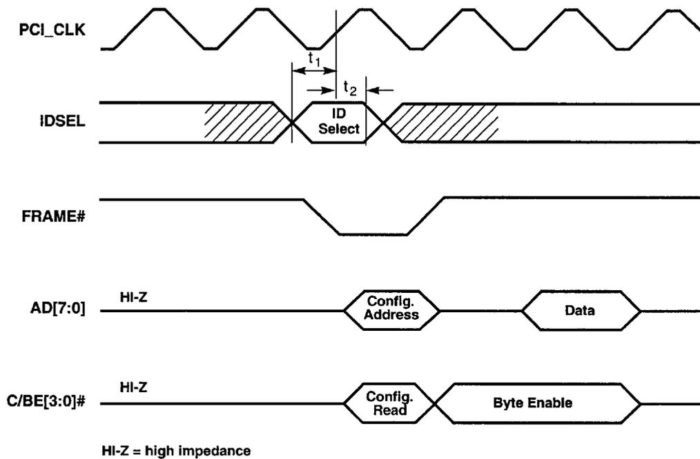
**Figure 13-3. IDSEL Timing in a Configuration Cycle (PCI™ Bus)**
