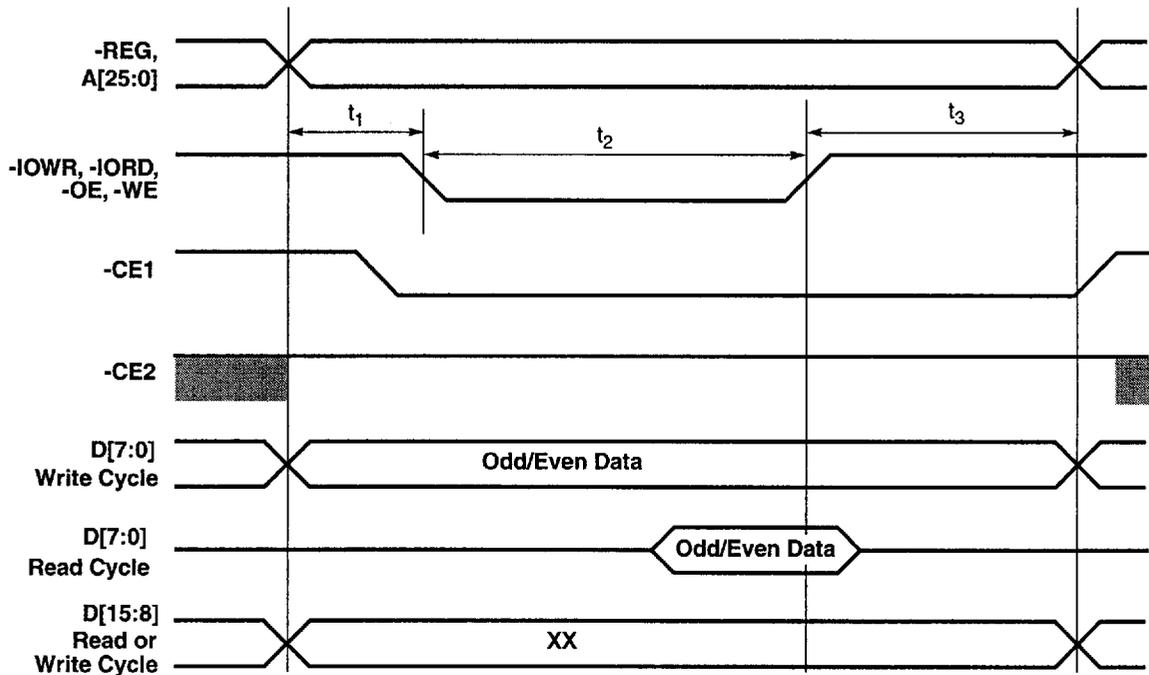
**Figure 13-9. Normal Byte Read/Write Timing** (that is, all other byte accesses, including odd I/O cycles where -IOIS16 is low)
