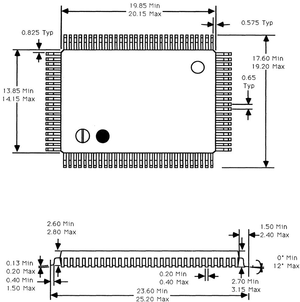
**NOTE:** Dimensions for the QFP package are in millimeters.
