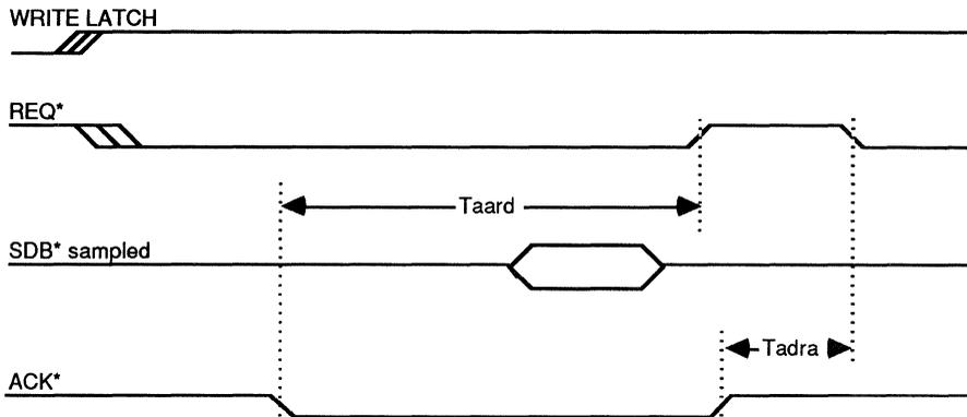
**NOTE:** The MOE\* signal (Pin 15) and the WE\* signal (Pin 16) will be continuously asserted low every unused BUFCLK\* cycle while waiting for the falling (leading) edge of the SCSI ACKNOWLEDGE signal (ACK\* — Pin 70).
