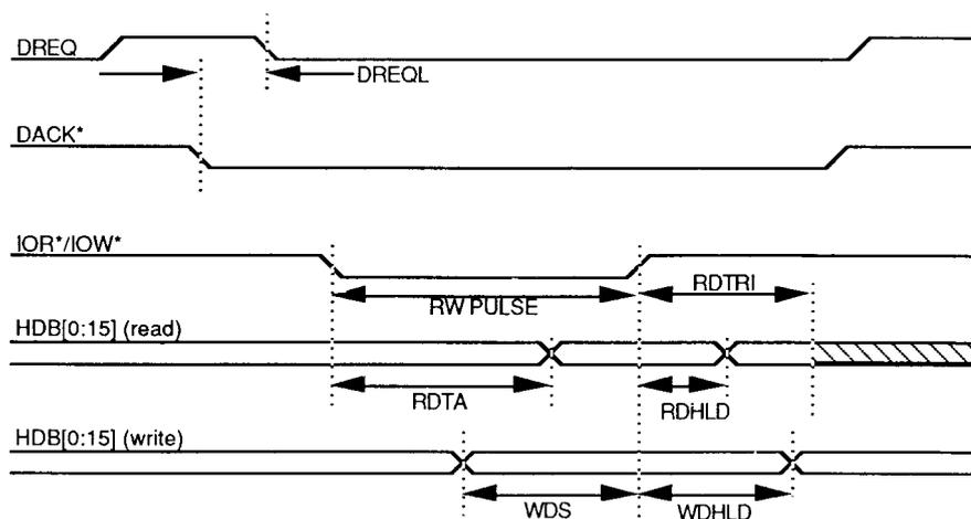
**Host Programmed I/O 8/16-Bit Timing Parameters**
