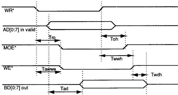
**Buffer Memory Read/Write Timing Parameters**
