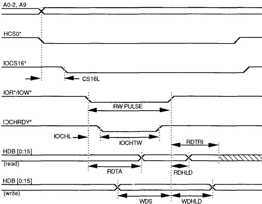
**Microcontroller Interface Timing Parameters**
