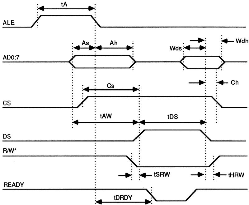
**11.3.3 Disk Read/Write Timing Parameters**
