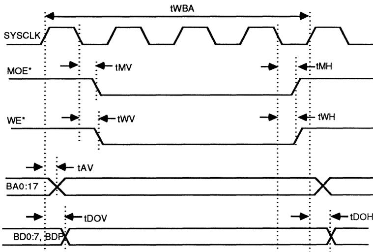
**NOTE:**  $tWBA$  is a functional parameter that gives the duration of one RAM data buffer access cycle in SYSCLK periods. The value is programmed in Bits 1-0 of Register 54H. These examples show  $tWBA = 4t$ .
