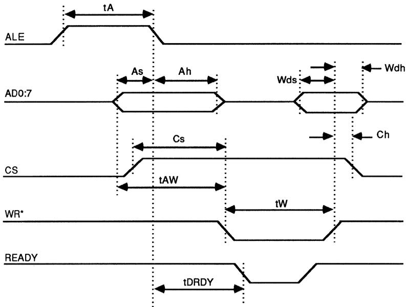
**11.3.2.4 Register Write Operation in Motorola Mode**
