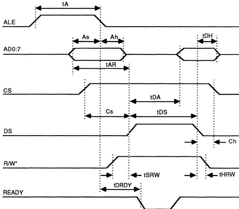
**11.3.2.3 Register Write Operation in Intel Mode**
