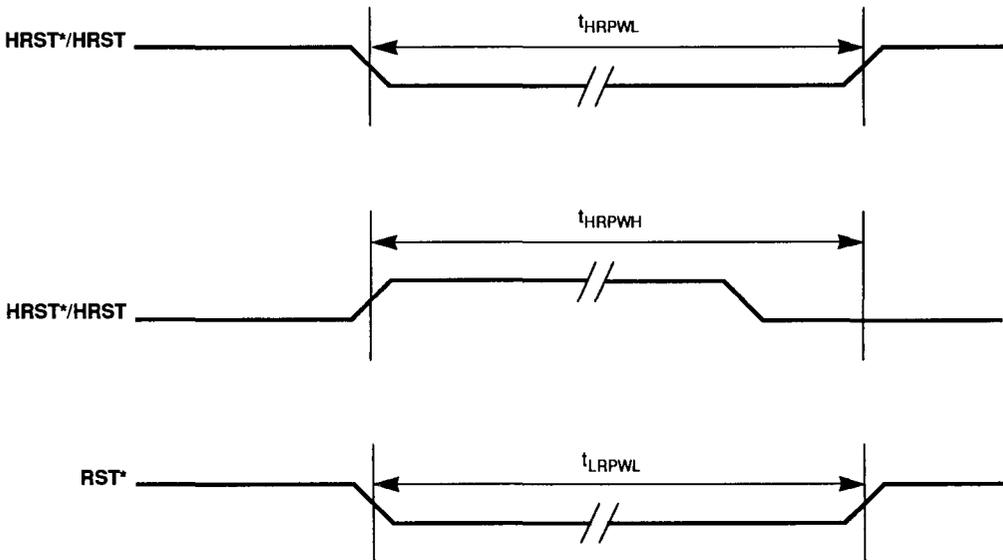
**Figures 9-1a. and 9-1b. RESET Assertion Timings**
