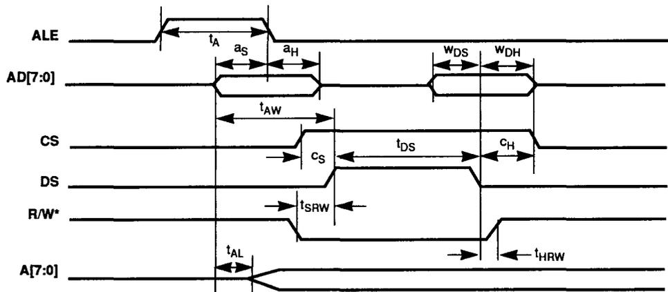
Figure 9-3b. Multiplexed Motorola Register Write Timing
