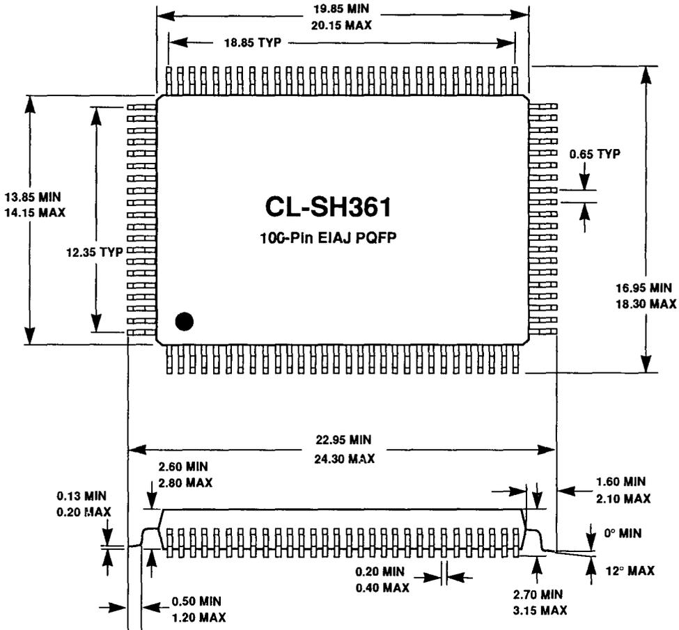
**NOTE:** Package dimensions are in millimeters.
