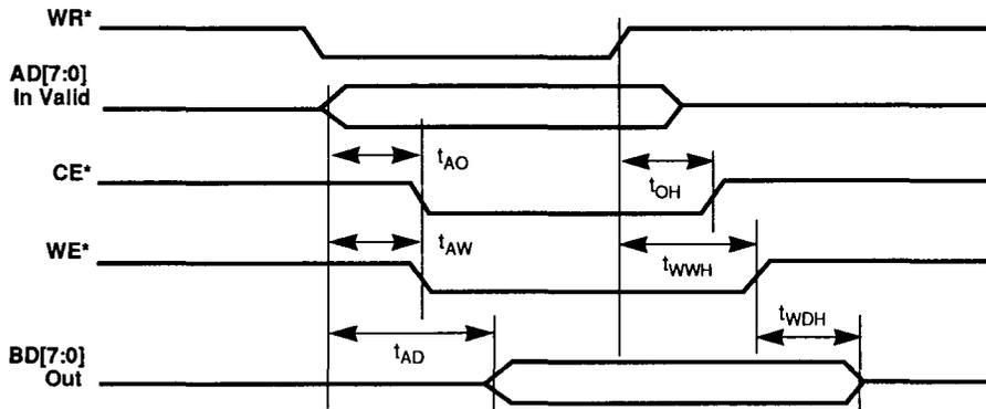
Figures 9-5a. and 9-5b. Register 70H Access Timing Parameters
