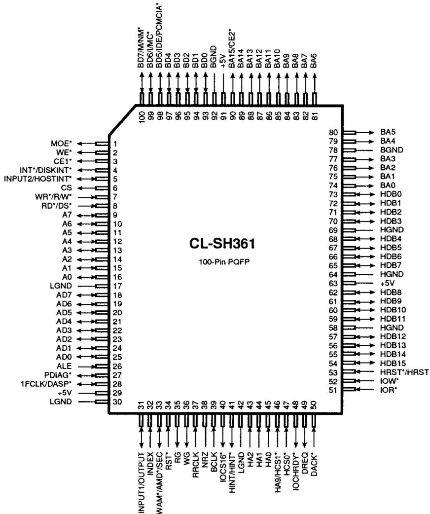
**1.2 Pin Diagram for the 100-Pin Very Low Profile Quad Flat Pack (VQFP)**
