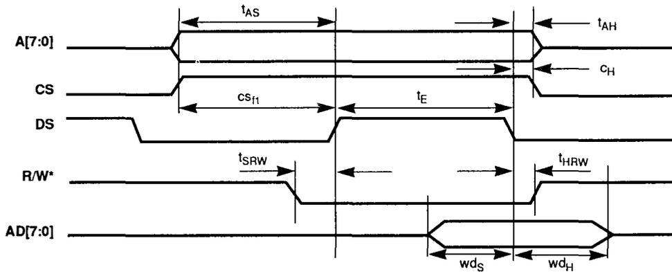
Figure 9-4b. Non-Multiplexed Register Write Timing
