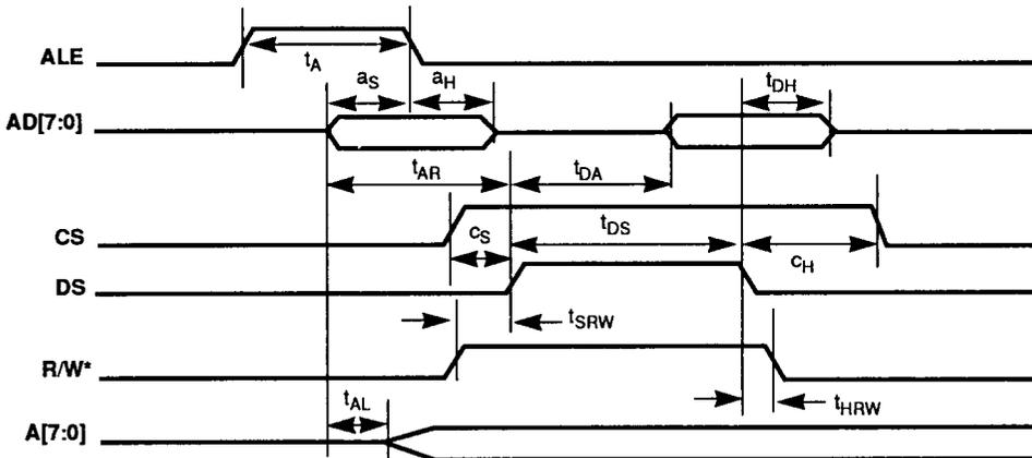
Figure 9-2b. Multiplexed Motorola Register Read Timing
