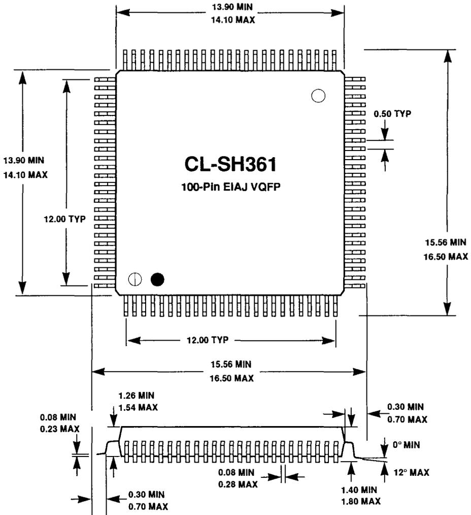
**NOTE:** Package dimensions are in millimeters.
