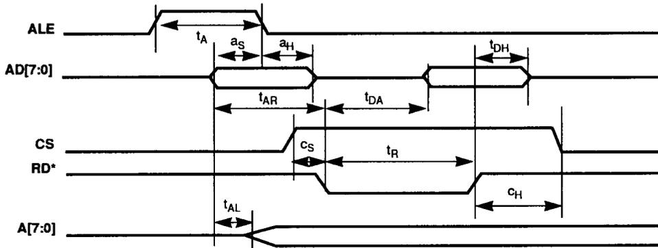
Figure 9-2a. Multiplexed Intel Register Read Timing
