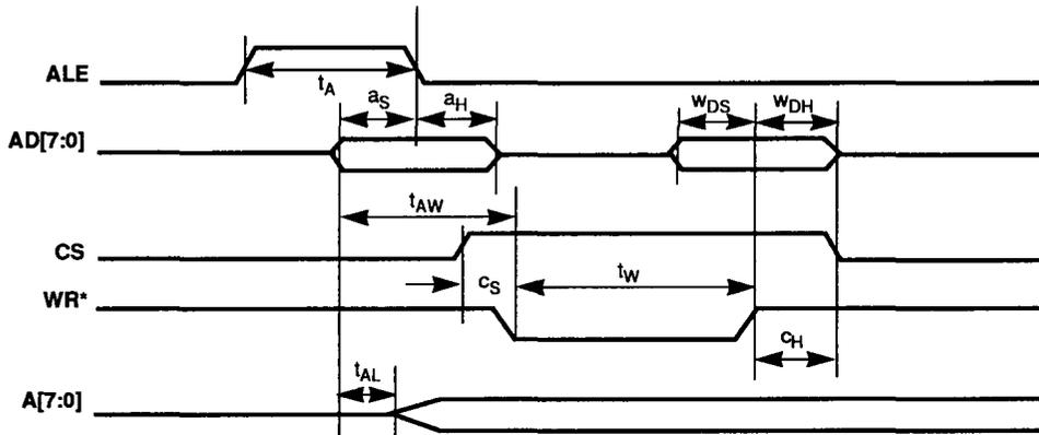
Figure 9-3a. Multiplexed Intel Register Write Timing
