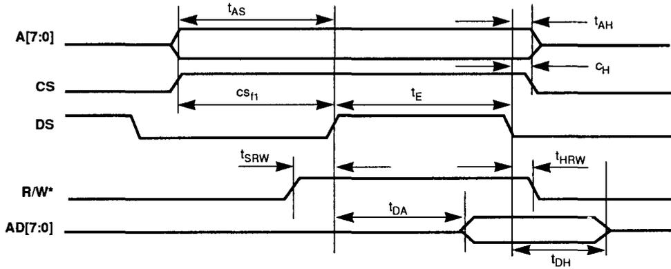
Figure 9-4a. Non-Multiplexed Register Read Timing
