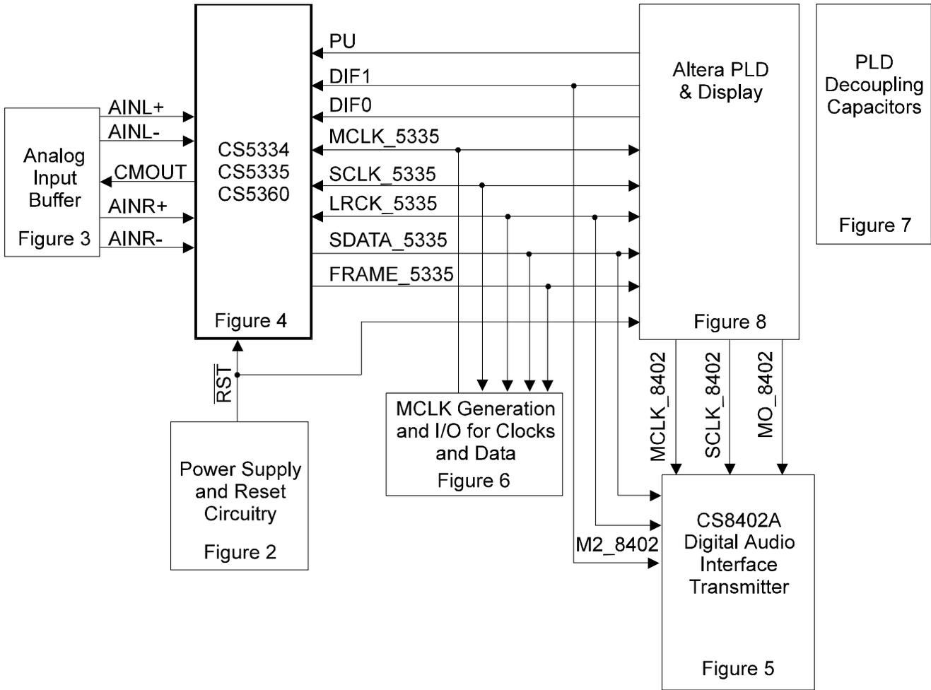
**Figure 1. System Block Diagram and Signal Flow**
