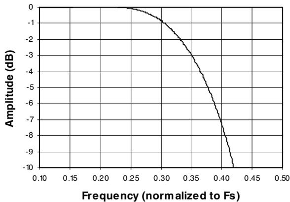
**Figure 11. Quad Speed Mode Transition Band (Detail)**
