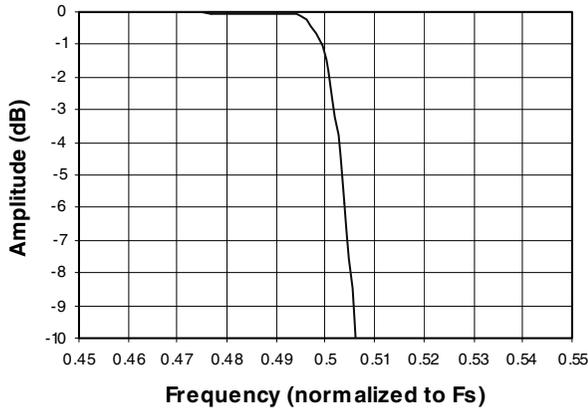
**Figure 3. Single Speed Mode Transition Band (Detail)**
