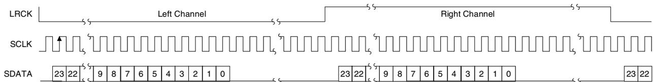
**Figure 20. I<sup>2</sup>S Serial Audio Interface**
