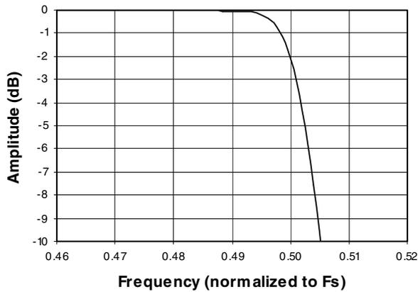
**Figure 7. Double Speed Mode Transition Band (Detail)**
