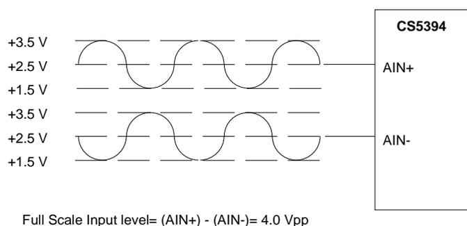
**Figure 4. Full Scale Input Voltage**
