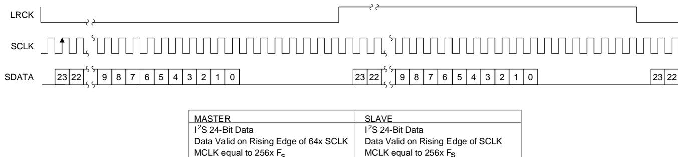
Figure 3 Serial Data Format, DFS High (I<sup>2</sup>S compatible).
