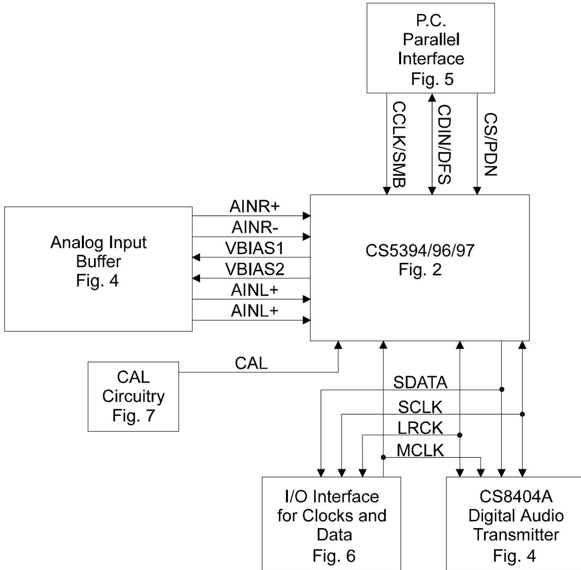
**Figure 1. System Block Diagram and Signal Flow**
