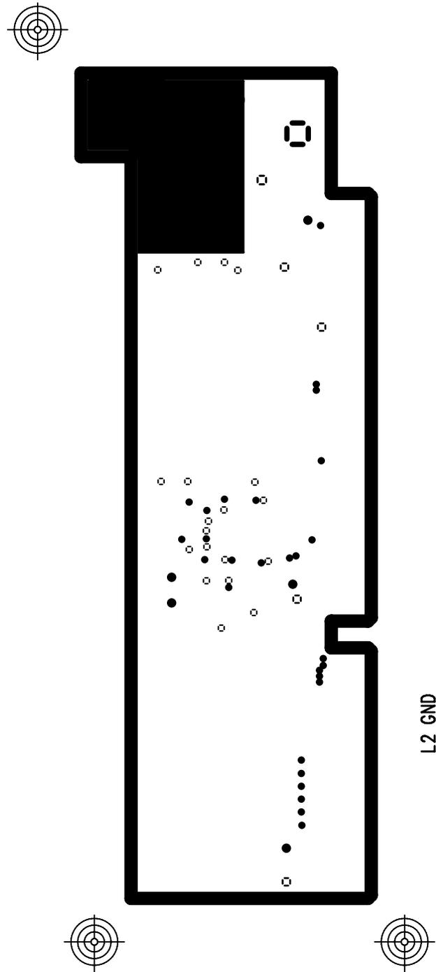
Figure 29. Ground Plane of four-layer board
