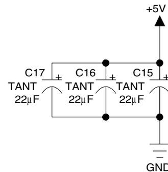
**Figure 11. Decoupling Capacitors Schematic**
