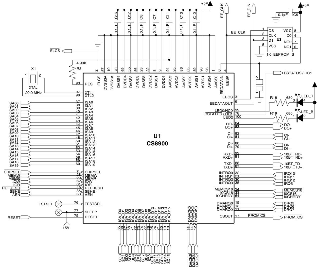
**Figure 13. CS8900A Schematic (Combo Card Application)**
