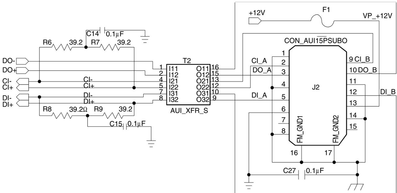
**Figure 16. AUI Schematic**
