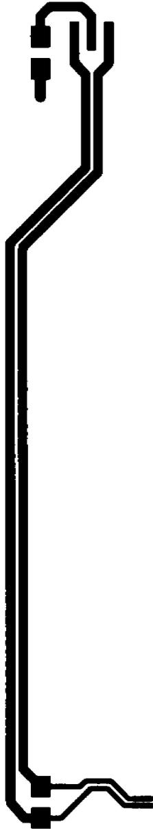
**Figure 34. 10BASE-T Receive Layout Details**
