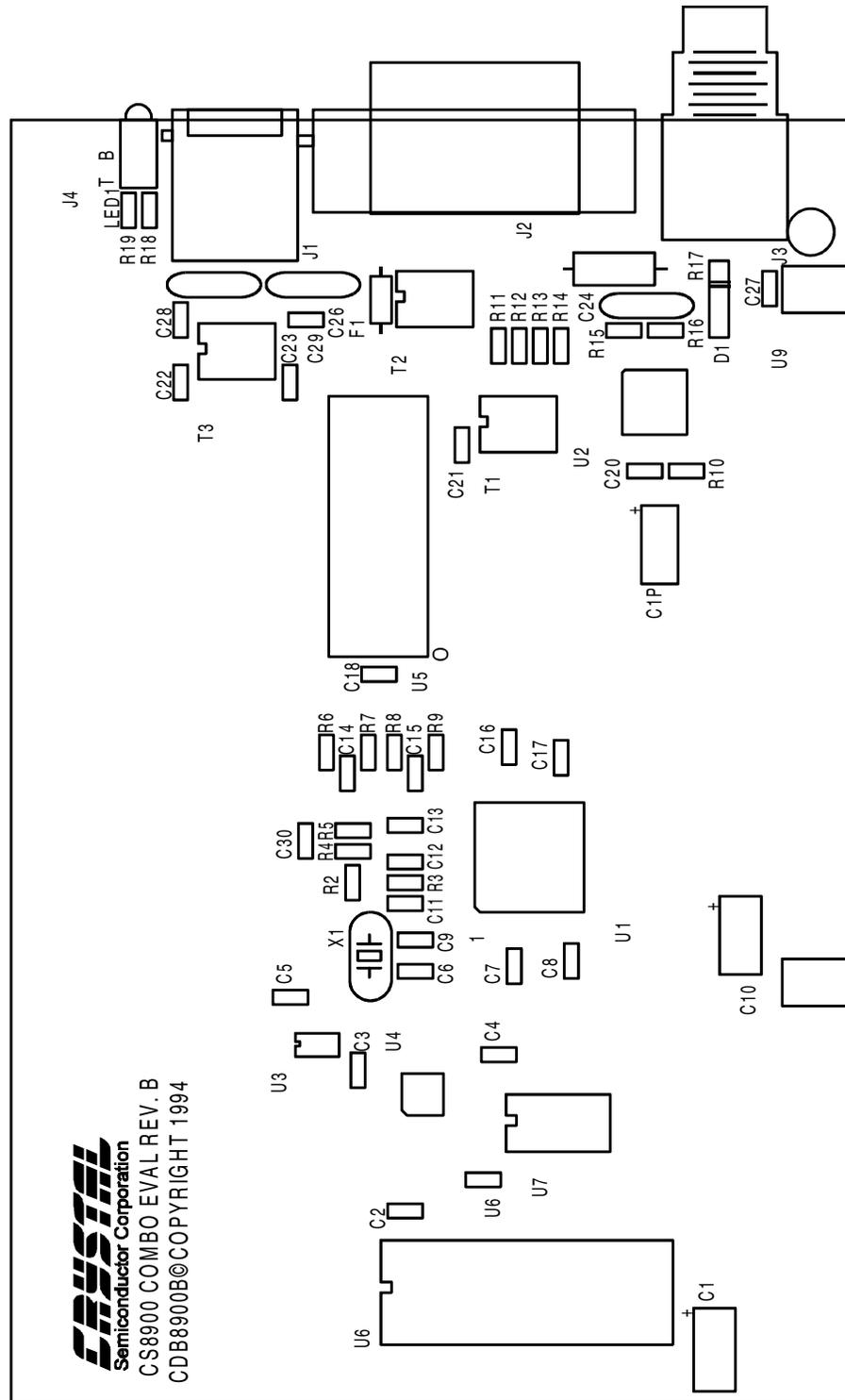
Figure 24. General placement on an ISA adapter card
