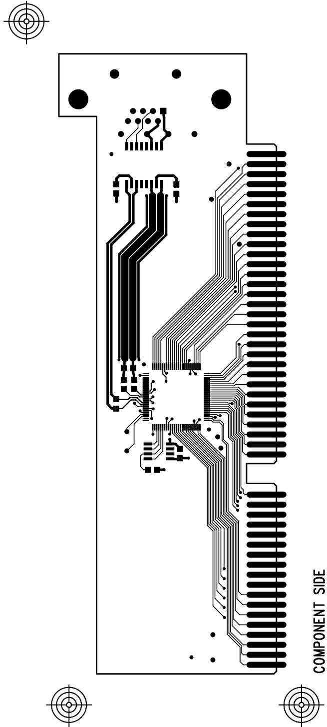
Figure 27. Component (top) side of four-layer board
