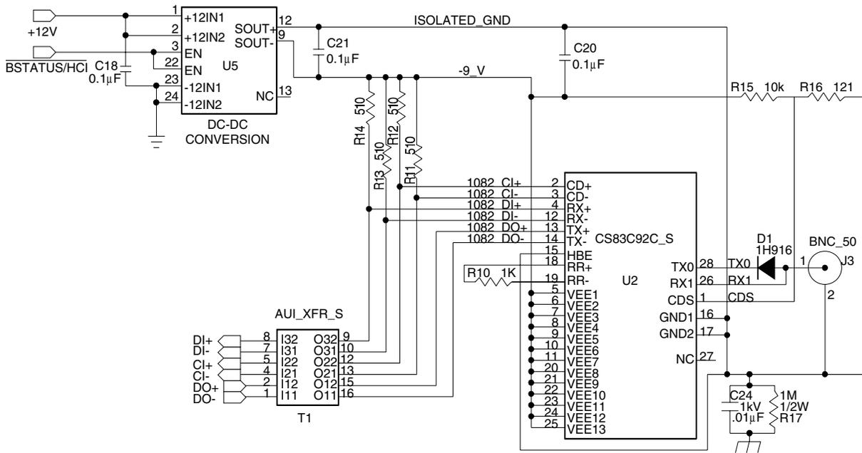
**Figure 17. 10BASE-2 Schematic**
