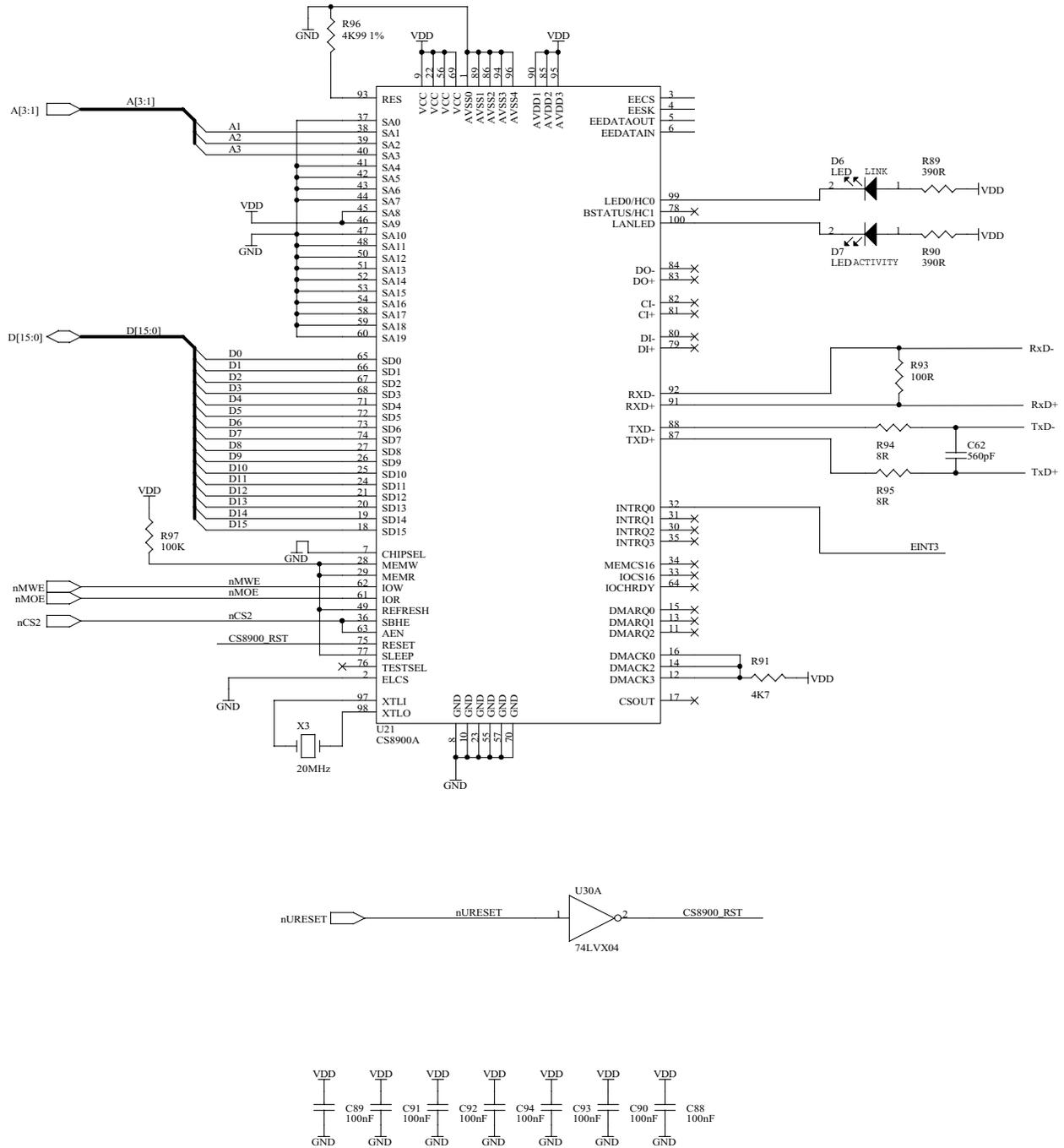
**Figure 4. CS8900A Interface to Cirrus Logic CL-PS7211**
