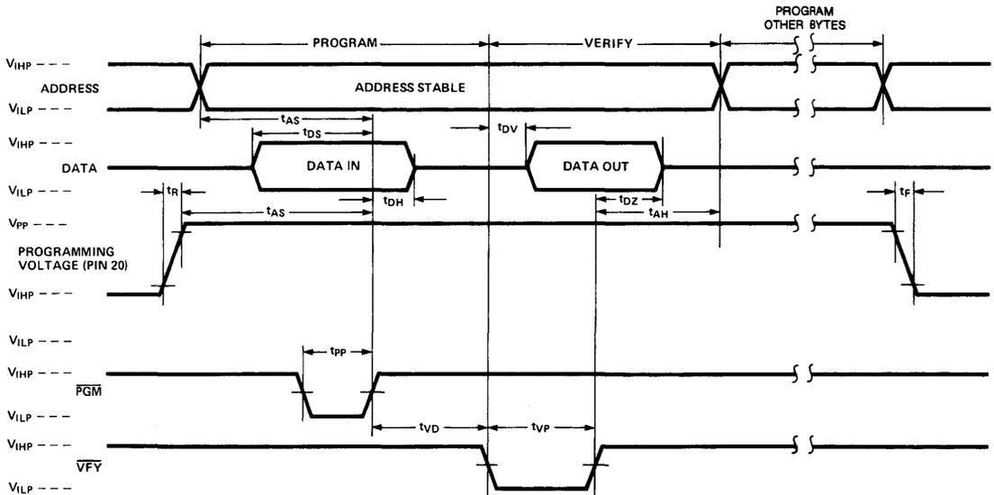
Figure 5. PROM Programming Waveforms
