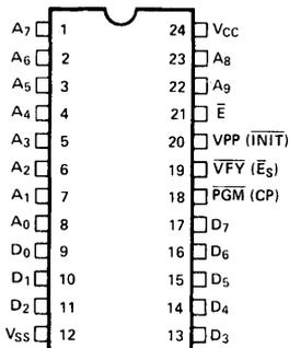
**Figure 3. Programming Pinouts**
