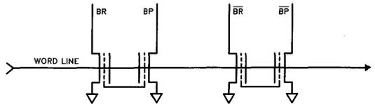
Figure 2. Non-volatile cell optimized for speed and programmability
