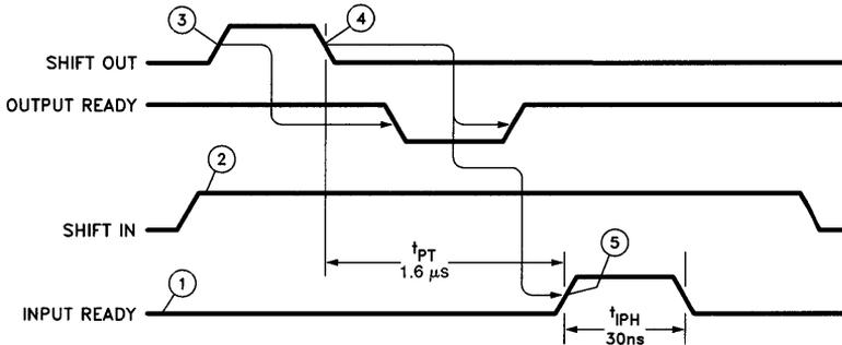
Figure 7. Bubblethrough Timing
