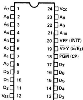
Figure 3. Programming Pinouts
