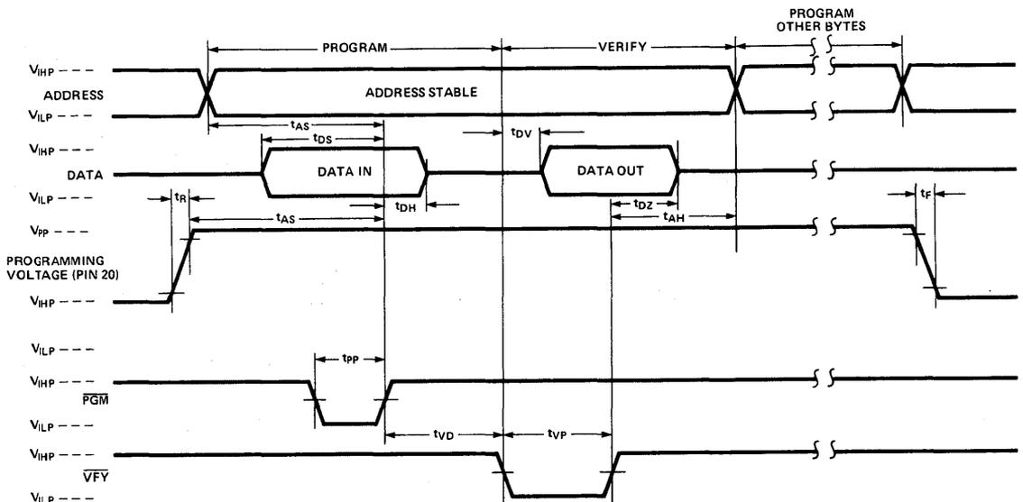
Figure 5. Programming Waveforms
