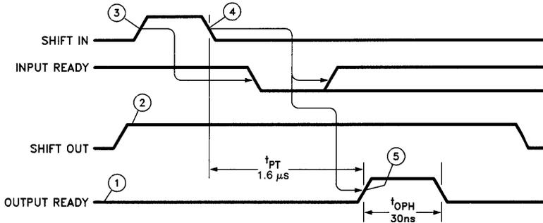
Figure 6. Fallthrough Timing
