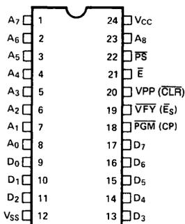
**Figure 3. Programming Pinouts**
