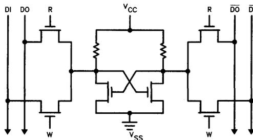
Figure 11B. Cell Schematic
