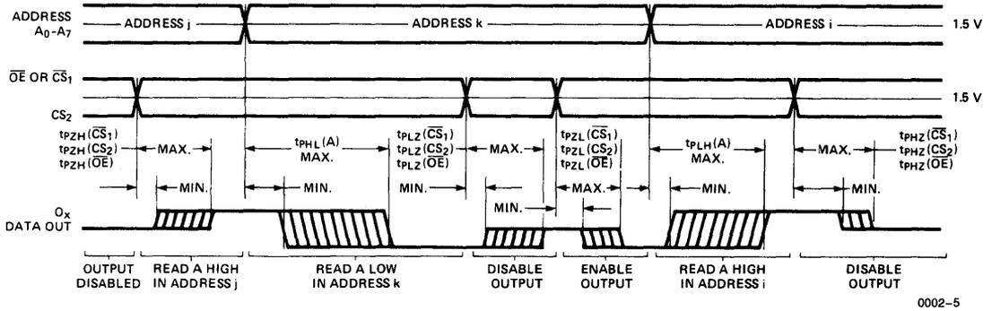
Switching delays from address input, output enable input and the chip select inputs to the data output. The CY93422 disabled output in the "OFF" condition is represented by a single center line.
