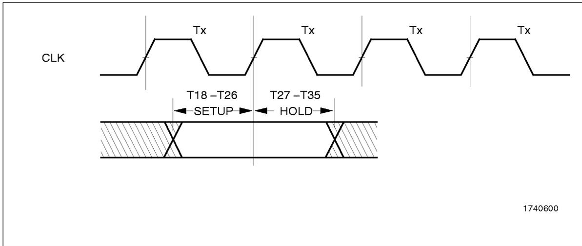
**Figure 2-5. Input Setup and Hold Timing**
