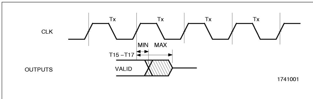
**Figure 2-4. Output Float Delay Timing**
