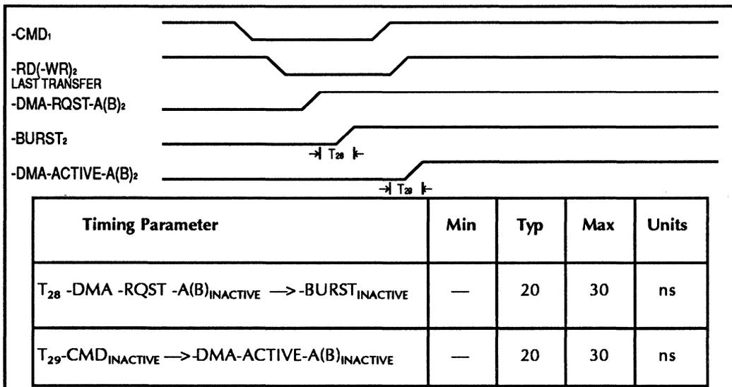
Figure 17. DMA: Slave Terminated Cycle
