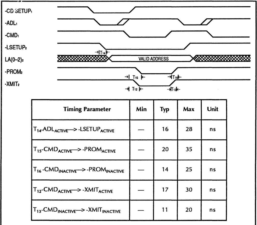
Figure 11. Configuration Cycle: External POS ID Read Cycle
