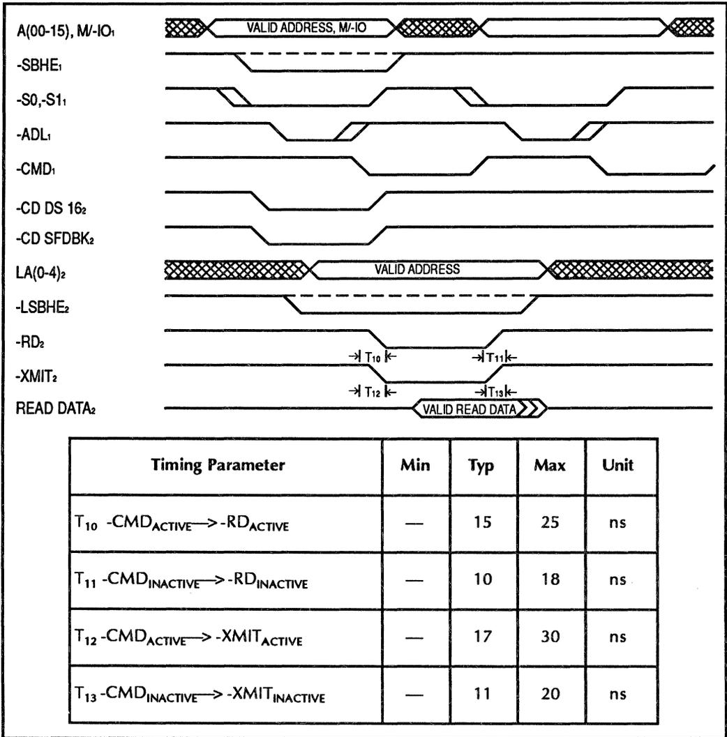
Figure 10. Basic Command Cycle: I/O Read
