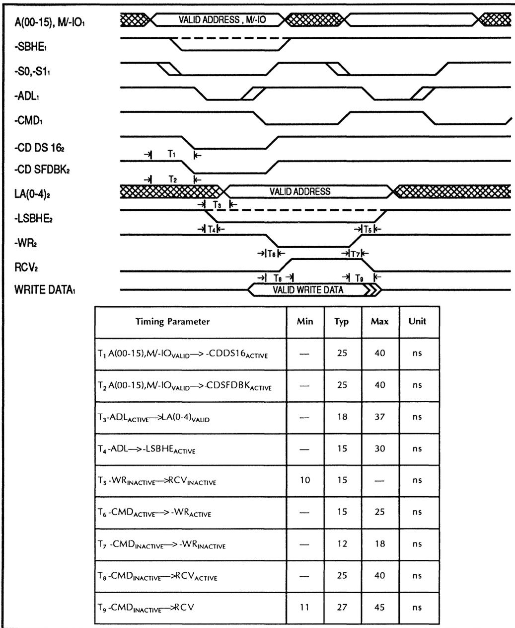
Figure 9. Basic Command Cycle: I/O Write
