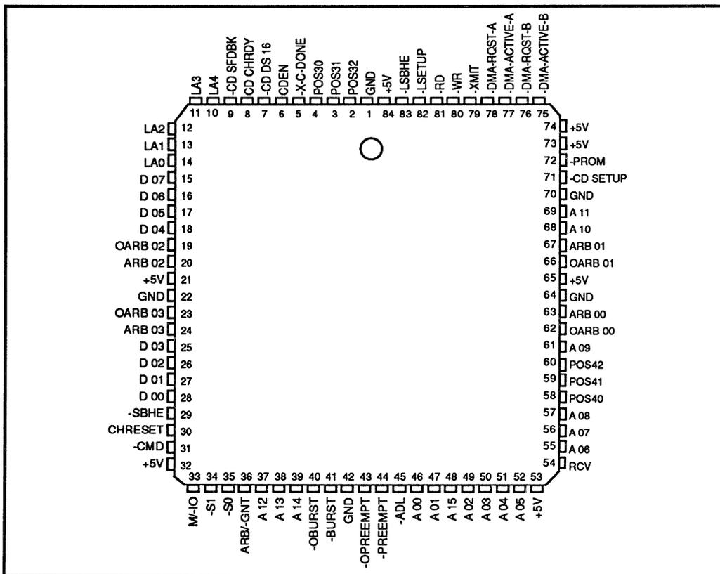
Figure 7. DT7920 Pin Functions
