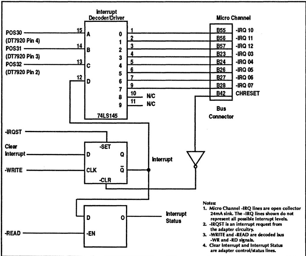
Figure 19. Interrupt Application Circuit
