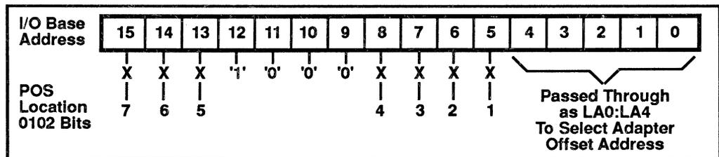
**Figure 6. DT7920 I/O Base Address Bit Assignments**
