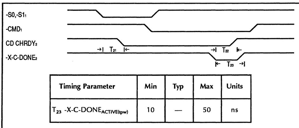
Figure 15. Extended Command Cycles: Asynchronous Extended Cycles
