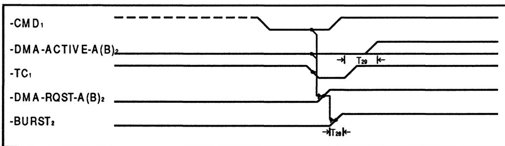
Figure 18. DMA: Controller Terminated Cycle
