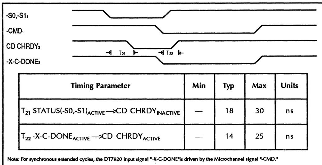
Figure 14. Extended Command Cycles: Synchronous Extended Cycles
