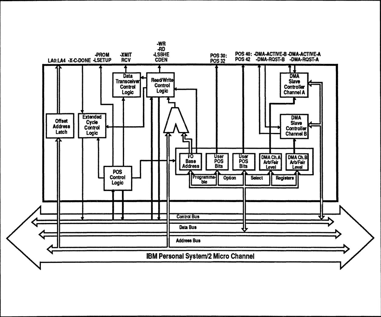
Figure 2. DT7920 Block Diagram
