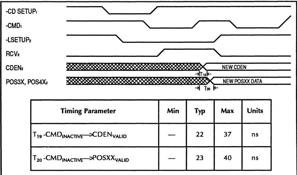
Figure 13. Configuration Cycle: Internal POS Register Access, Write Cycle
