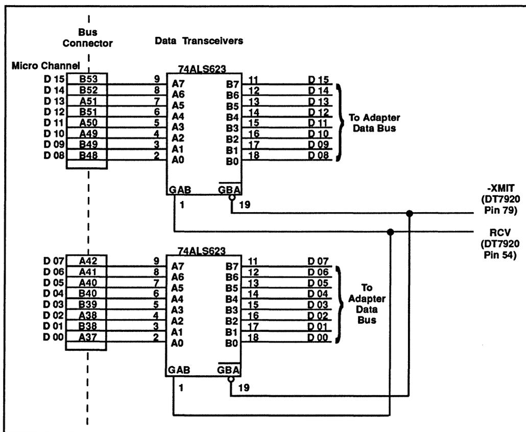
Figure 4. DT7920 signals RCV and -XMIT gate data on and off the Micro Channel bus.
