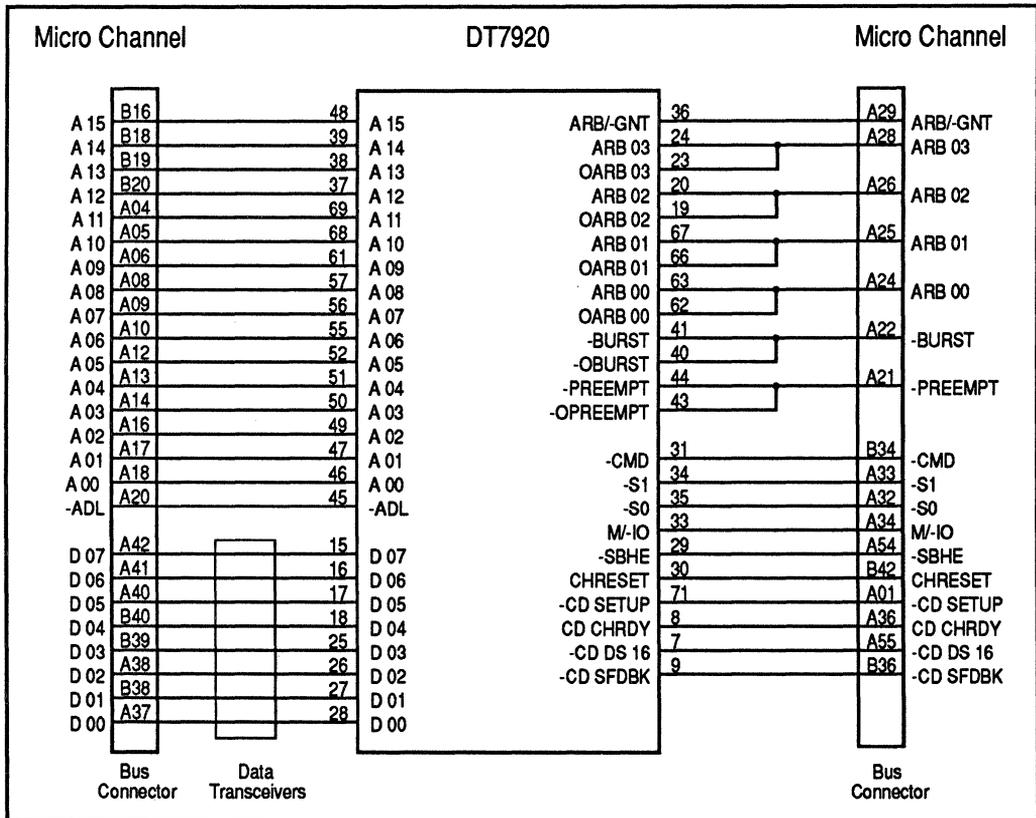
Figure 3. DT920 Bus Connections
