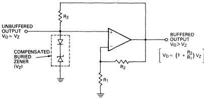
FIGURE 10. Temperature Compensated Reference Circuit
