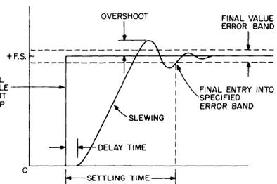
Figure 13. Amplifier Settling Time
