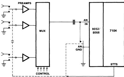
Figure 25: Multiplexed Auto-Zero System With Individual Preamps
