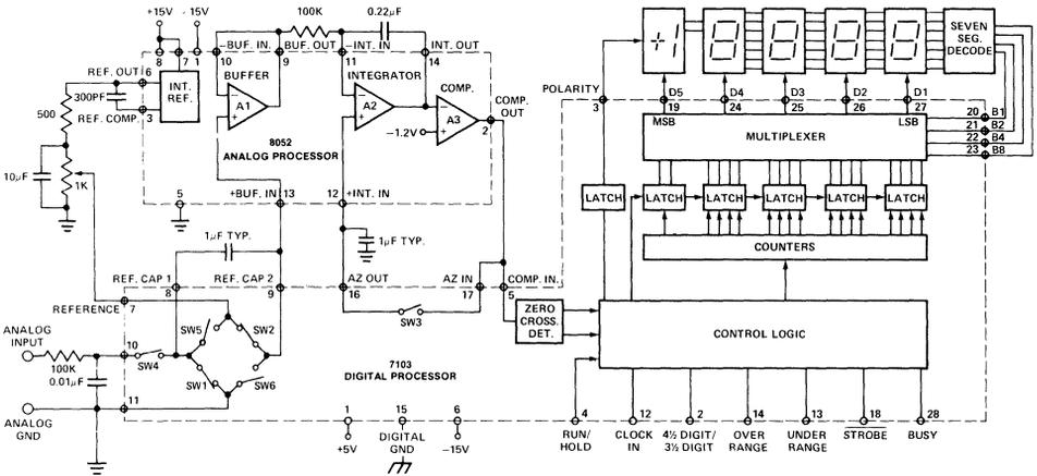
Figure 4: the 7103/8052 A/D Converter pair.
