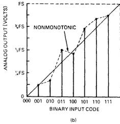
Fig 8 Monotonic (a) and nonmonotonic (b) DAC outputs. Monotonicity means output is continuously increasing function of input
