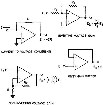
Figure 10. Operational Amplifier Configurations
