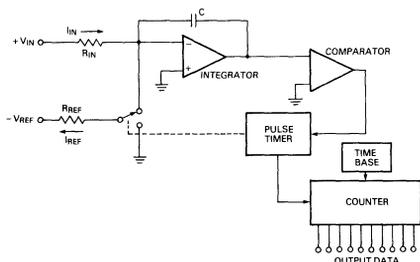
FIGURE 23. Charge Balancing A/D Converter
