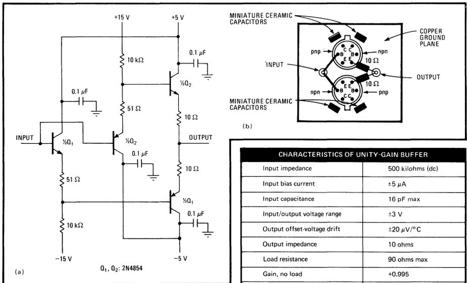
**Wideband buffer.** Emitter-follower configuration yields unity gain from dc to 300 megahertz. Absence of feedback in circuit contributes to buffer stability. Use of matched npn-pnp transistor pairs ensures almost perfect input/output signal tracking (a). Component layout is critical for circuit stability (b).
