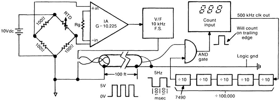
**Fig. 6:** With the addition of a V/F converter, transducer bridge output can be sent over greater distances. A low
