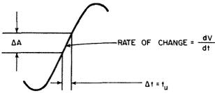
8. **Timing uncertainty in the switch** and driver circuit produces uncertainty in the held voltage, which for a given period of time, increases with the rate of change of the signal voltage.
