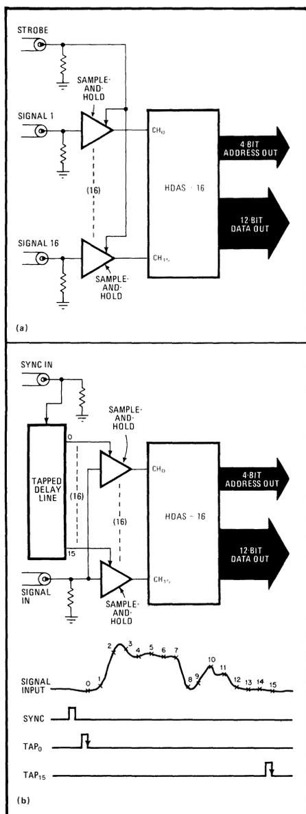
**3. Handling high-frequency inputs.** To acquire signals beyond the mid-audio range requires a sample-and-hold circuit for each channel (a). For a nonrepetitive high-frequency signal, a delay line and a string of sample-and-holds slice the input into 16 pieces (b).
