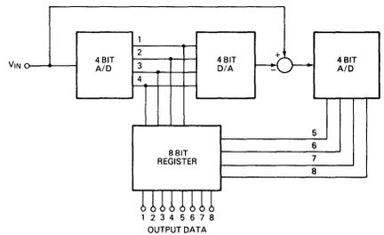
FIGURE 16. Eight-Bit, Two Step Parallel A/D Converter
