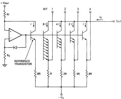
FIGURE 1. Basic Quad Current Switch Circuit
