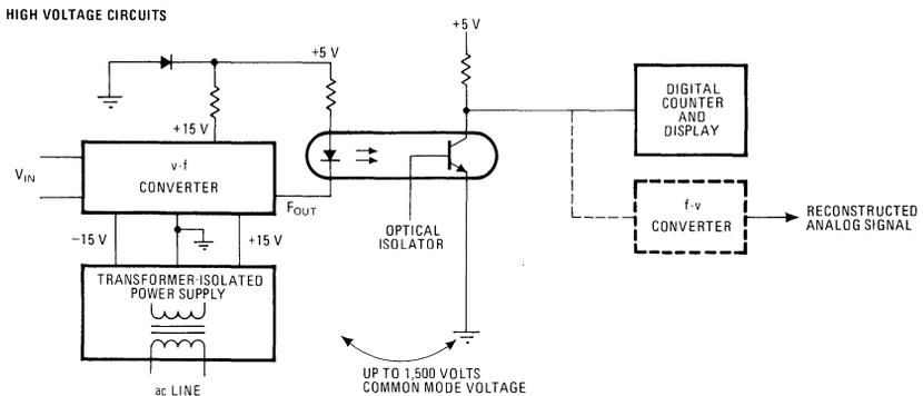
**1. Isolation.** Because the v-f converter has a serial output, the pulses can be transmitted through a single optical isolator. The v-f converter is floated at the high common-mode voltage at which the measurement is made. It is also powered by a floating and isolated supply.
