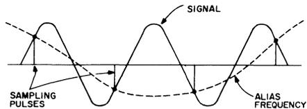
Figure 8. Alias Frequency Caused by Inadequate Sampling Rate
