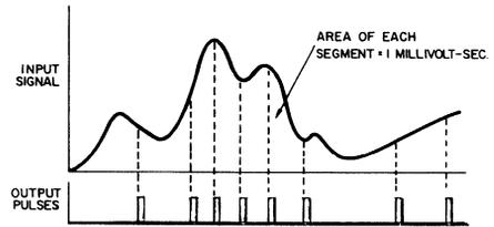
8. The integration process in a v/f converter can be defined in terms of millivolt-seconds for each pulse delivered. To get the total area, simply multiply the total count by 0.001.
