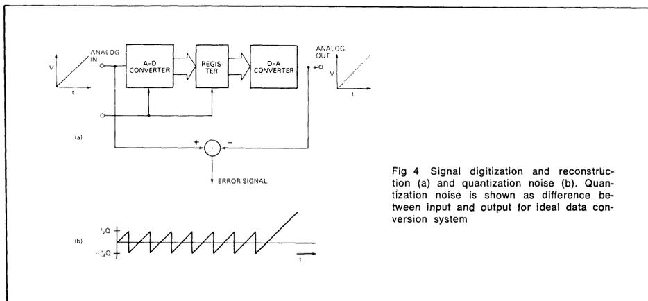
Fig 4 Signal digitization and reconstruction (a) and quantization noise (b). Quantization noise is shown as difference between input and output for ideal data conversion system
