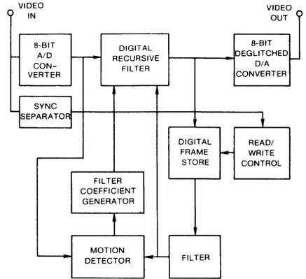
3. **Digital noise reducers** store the converted frame data for element-by-element processing in a recursive filter. To avoid smearing moving pictures, frames whose elements show too much motion aren't filtered.
