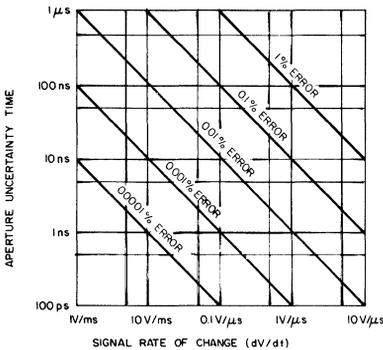
9. **To obtain the error due to aperture uncertainty time** for a given signal rate of change, a full-log plot is helpful. This plot assumes a 10-V full-scale signal.
