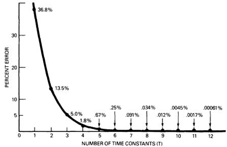
Figure 15. Output Settling Error as a Function of Number of Time Constants
