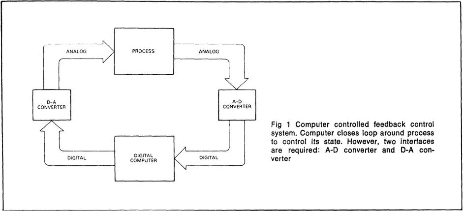
Fig 1 Computer controlled feedback control system. Computer closes loop around process to control its state. However, two interfaces are required: A-D converter and D-A converter
