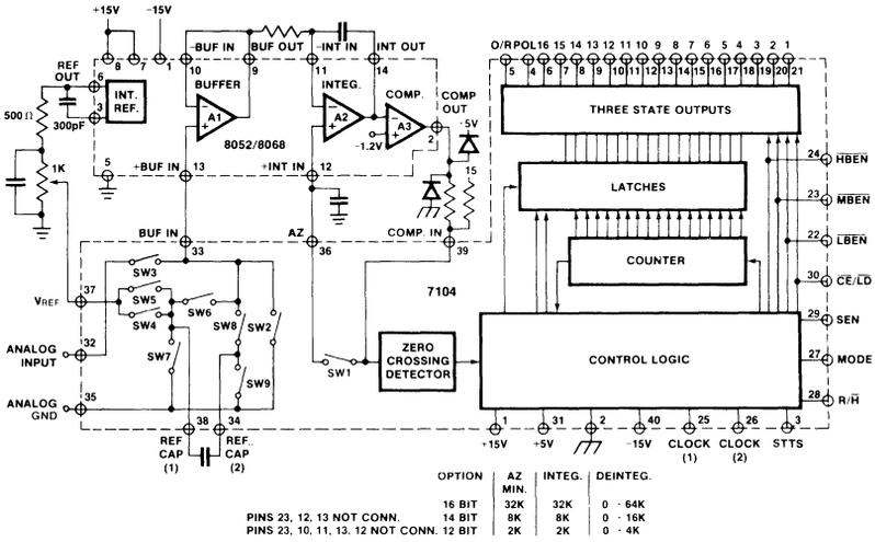
Figure 1: 8052A (8068A)/7104 16/14/12 Bit A/D Converter.
