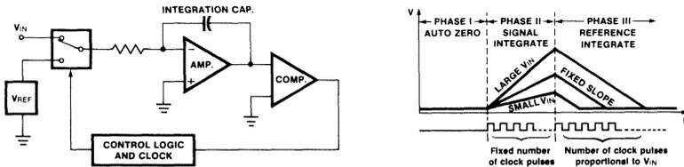
Figure 2: Simplified Dual-Slope Converter and the Three Phases of a Dual-Slope Conversion.
