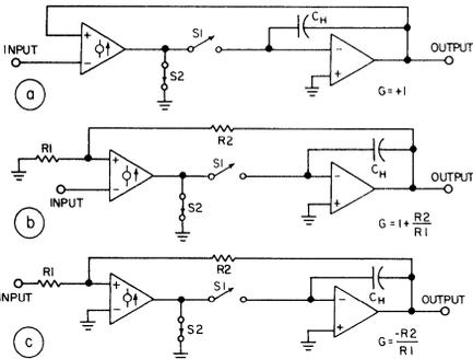
9. Here are three different ways to connect the input and feedback to the partial circuit in Fig. 8. The circuit in (c) has unity gain if the input ( $R_1$ ) and feedback ( $R_2$ ) resistors have equal values.
