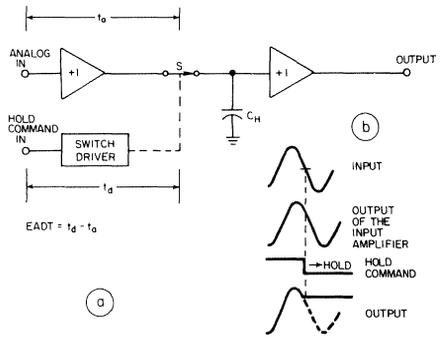
7. **Effective aperture delay time** is the difference between the input amplifier time delay,  $t_0$ , and the delay between the hold command and the time when the switch opens ( $t_d$ ). EADT may be positive, zero, or negative. If  $t_0$  is greater than  $t_d$ , the hold capacitor sees a delayed version of the input (b), which results in holding an input voltage that occurred before the hold command.
