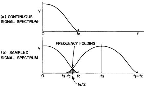
Figure 7. Frequency Spectra Demonstrating the Sampling Theorem
