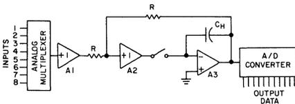
4. In a single-channel system, the settling time of the input buffer amplifier, A<sub>1</sub>, isn't critical because the amplifier can follow changes in the signal (a). With multiplexed inputs (b), however, the input buffer may take additional time to settle to the new value at the multiplexer's output when it switches channels.
