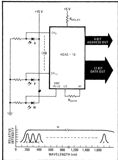
**5. High gain.** In this fast spectrophotometer application for monitoring industrial waste, the hybrid's high-gain capability and adjustable settling time are exploited. Careful tailoring of delay time versus gain provides best system resolution in terms of data rate needs.
