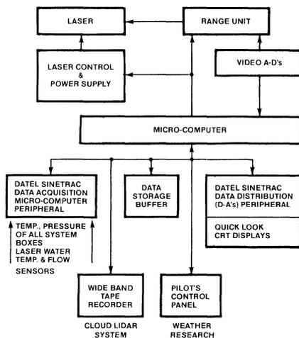
The micro-computer controlled all operating sections of the system. The most important reason a micro-computer was used in this application was physical size as the entire system was to be installed on an aircraft.
