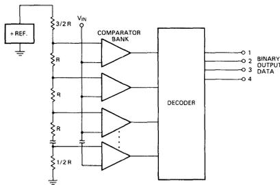
FIGURE 15. Parallel (Flash) Type A/D Converter
