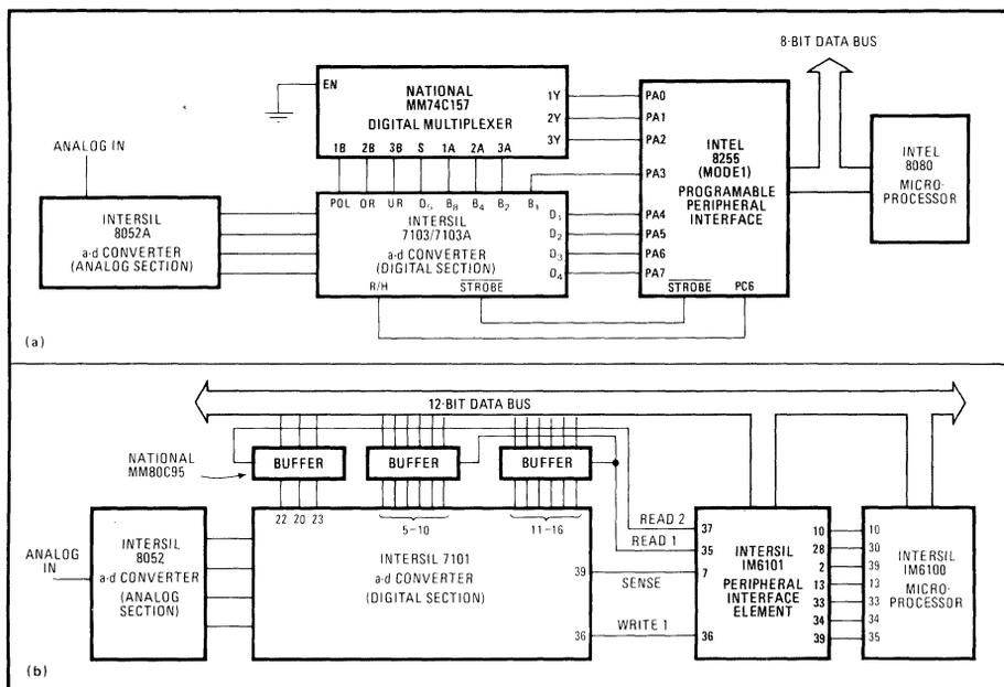
**1. Parallel interface.** All microprocessor families contain a programmable interface device that can mate the converter and the microprocessor when the data format is parallel. Some of these devices (a) handle data directly, while others (b) have read and write lines.
