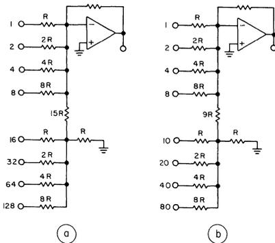
2. Binary (a) and BCD (b) ladder networks in d/a converters use the same weighting in the resistor quads but different divider ratios.
