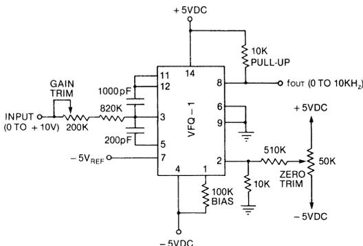
adjustment and external gain adjustment. The connection shown is for a 10-KHz full-scale output frequency with a +10V full-scale input.
