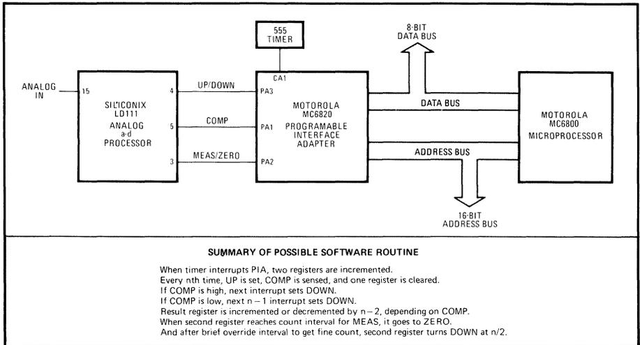
**4. Another approach.** The microprocessor can do the digital processing for charge-balancing a-d. However, because the up/down switching for this type of converter must be continued throughout its operating cycle, microprocessor overhead can be substantial.
