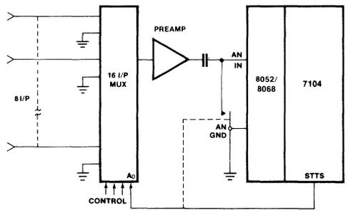
Figure 26: Multiplexed Auto-Zero System With Common Preamp
