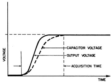
3. **Acquisition time** may be less than or greater than the time it takes the output voltage to settle to its final value. In (a), the capacitor reaches its final value before the
