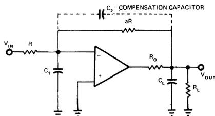
**Fig. 10**—Three sources of extraneous poles appear in this diagram: input capacitance, load capacitance and the op amp itself.  $C_2$  compensates for output ringing and is best chosen via experiments with the actual circuit components and layout.
