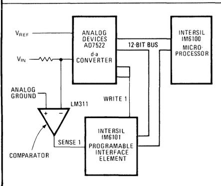
**3. Lending a helping hand.** The microprocessor can even become part of the converter loop. With the setup shown, the software permits changing from a successive-approximation a-d to a tracking a-d, or even using both methods to their best advantage.
