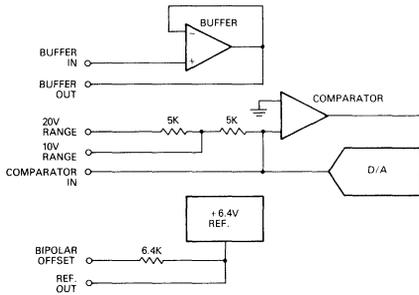
FIGURE 12. Hybrid A/D Converter Input Circuit
