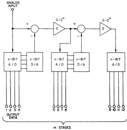
6. **A generalized n-bit, m-stage a/d converter** develops an output with  $n \times m$  bits of resolution. In each stage, except the first, the analog result of the subtraction is amplified by a circuit whose gain is  $2^n$ .
