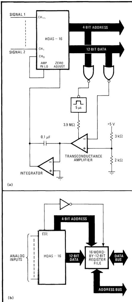
**6. Odds and ends.** Charge-pump loop (a) cancels troublesome offset errors for all time and temperature. A twin circuit could be used to cancel gain errors also. Register file (b) creates memory location for HDAS-16, so data access is independent of the hybrid's status.
