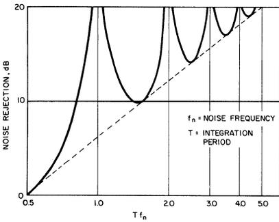
4. Integrating a/d converters can have exceptional noise-rejection capability if you merely adjust their measurement cycle to equal the period (or a multiple) of the noise frequency to be rejected.
