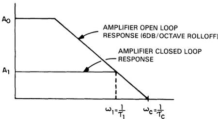
Figure 14. Amplifier Single-Pole Open Loop Gain Characteristic
