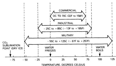
Figure 50. Standard Operating Temperature Ranges for Data Converters
