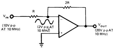
**Fig. 3—**The summing junction is NOT a virtual ground in high speed op-amp applications. Thus the amplifier must be designed with a large input dynamic range (IDR), or distortion, limiting or clipping will result.
