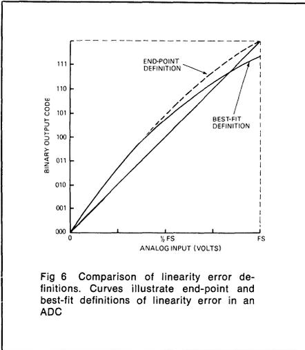
Fig 6 Comparison of linearity error definitions. Curves illustrate end-point and best-fit definitions of linearity error in an ADC
