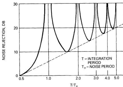
Figure 35. Noise Rejection for Integrating Type A/D Converters
