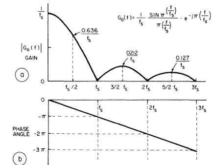
4. The gain response of a zero-order hold (a) in terms of the sampling frequency  $f_s$  takes the form of the absolute value of  $(\sin x)/x$ . The phase response (b) is linear because of the constant time delay.
