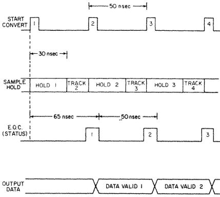
5. **Timing for the 8-bit two-stage a/d converter** allows for two modes in the sample-and-hold circuit—Hold and Track. These occur between successive Start-Converts. The second and succeeding conversions take 50 ns.
