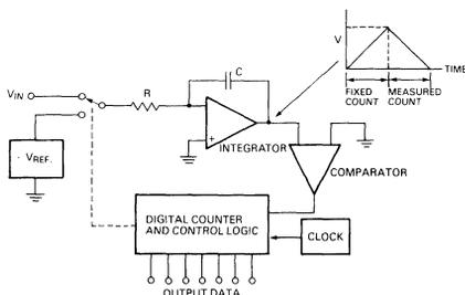
FIGURE 22. Monolithic Dual Slope A/D Converter
