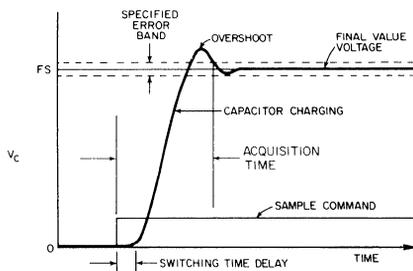
1. **Acquisition time of a sample-hold** starts with the sample command and ends when the voltage on the hold capacitor enters and stays in the error band. Acquisition time is defined for a full-scale voltage change, measured at the hold capacitor.
