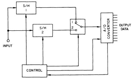
7. In an ultrafast a/d conversion system, acquisition time in a sample-and-hold takes up a sizable part of the cycle. Interleaving two sample-and-holds like this lets one of them acquire while the other one's output is being converted.
