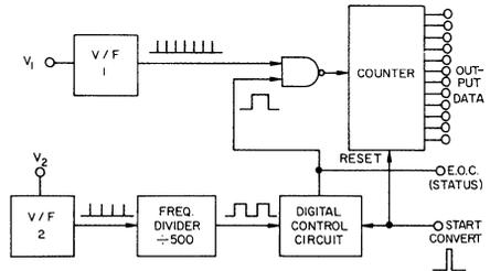
9. If you use two v/f converters, you can make a high-accuracy, ratiometric a/d converter. Because of the wide frequency span covered, the dynamic range of the converter can reach 10,000:1.
