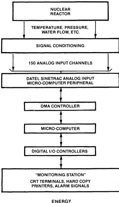
In this application, it was necessary to monitor the status of 150 points. The physical parameters being measured were temperature, pressure, and water flow. The Reactor Vendor chose to use a micro-computer for cost reasons and because the power of a mini was not warranted. The outputs of the transducers were connected to a Signal Conditioning Unit which generated analog voltages in the 0 to +10V range for inputting to the measurement system.
