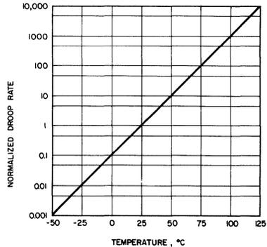
5. **Droop in hold mode** can be positive or negative-going, and may not be linear with time (a). Since most leakage current comes from silicon devices, droop as a function of temperature is predictable (b).
