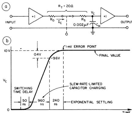
2. **This equivalent circuit for determining acquisition time** (a) shows the importance of the charging time constant,  $R_f C_H$ . Acquisition time is the sum of the various delays incurred in charging the hold capacitor to its final value (b), and is dominated by slew-limited charging.
