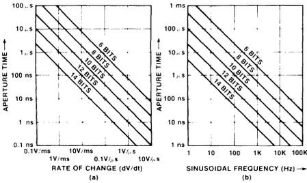
Figure 4: Maximum input signal rate change (a) and sine wave frequency (b) as a function of sampling or aperture time for  $\pm \frac{1}{2}$  LSB accuracy in 'n' bits.
