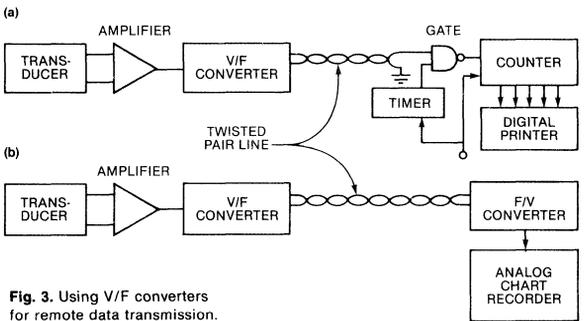
**Fig. 3.** Using V/F converters for remote data transmission.
