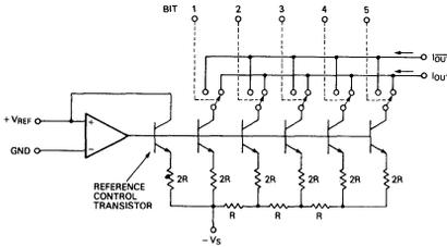
**FIGURE 19. Bipolar D/A Converter with Diffused Resistor Network**
