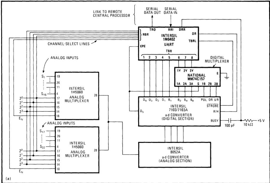
nization, a controlled data rate, parity generation, and clocking, as well as a full complement of handshaking signals for the microprocessor. With two-way communications and a phone-line tie-in through acoustic couplers, any UART-compatible a-d or d-a converter may talk to a friendly microprocessor, no matter how far away it is, over telephone lines.
