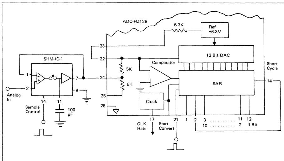
Figure 7 shows the circuit connection for a sampling 10 bit A/D converter. A 12 bit hybrid A/D with 8 μsec conversion time is short cycled to 10 bit operation. This is done by connecting the short cycle terminal, pin 14, to pin 2, the bit 11 output. Pins 3 through 12 then serve as data outputs with complementary offset binary coding. The input to the A/D converter is connected for ±5V bipolar operation.
