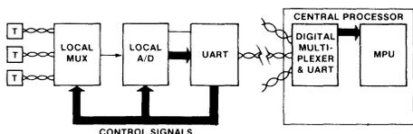
Figure 6(b): Data Acquisition using several local A/Ds
