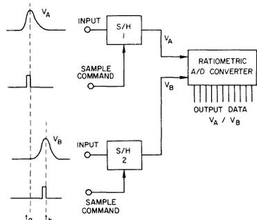
8. Sample-and-holds can serve as temporary analog signal-storage devices. The first sample-and-hold retains signal  $V_A$ 's peak value so the converter can divide it by the peak value of input  $V_B$ , which comes by later.
