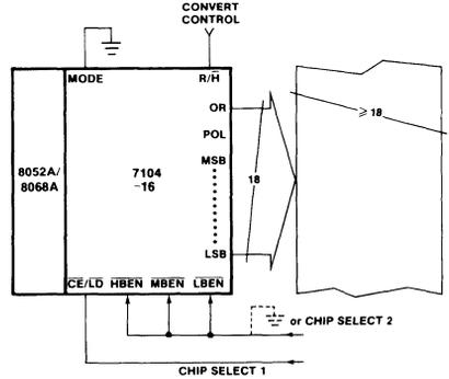
Figure 4: Full 18 Bit Three State Output
