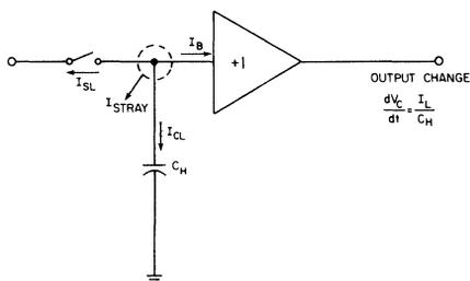
4. **Hold-mode droop is caused by currents** that charge or discharge the hold capacitor. These include switch-leakage, stray-leakage, amplifier-bias currents and leakage within the hold capacitor itself.
