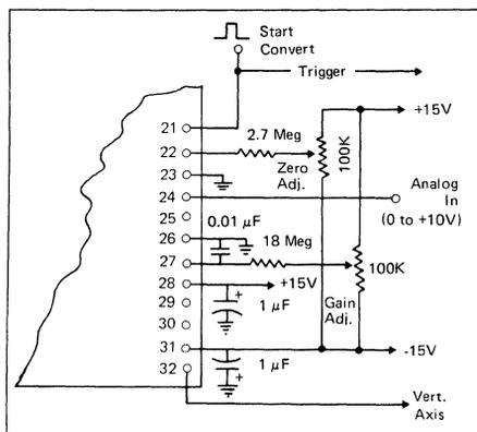
Figure 8 illustrates simple calibration of the hybrid A/D converter. Two external  $100\text{K}\Omega$  potentiometers adjust zero and full scale for the converter.
