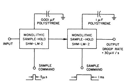
11. Cascaded sample-holds acquire a signal quickly and hold it for a long time with little droop. The first one needs to hold a signal only long enough for the second to acquire it. Typical acquisition would be  $5 \mu\text{s}$  to 0.1%, with a droop rate of  $30 \mu\text{V/s}$ .
