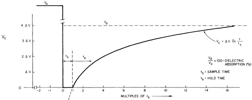
2. A natural log function of time is an accurate approximation to the voltage creep caused by dielectric absorption. Before sampling, the capacitor has been holding a voltage  $V_0$ . A new sample charges the capacitor to a new
