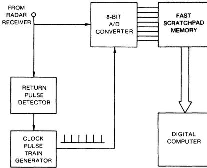
5. **Radar-signature-analysis systems** use powerful computers to process information contained in the return pulse's frequency content, amplitude and wave shape. You need a fast converter but not much memory.
