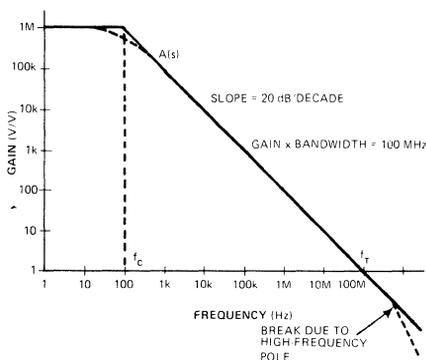
Fig. 1—Well designed high-speed op amps have a smooth 20 dB/decade roll-off. Additional amplifier poles should not occur until well beyond  $f_T$ .
