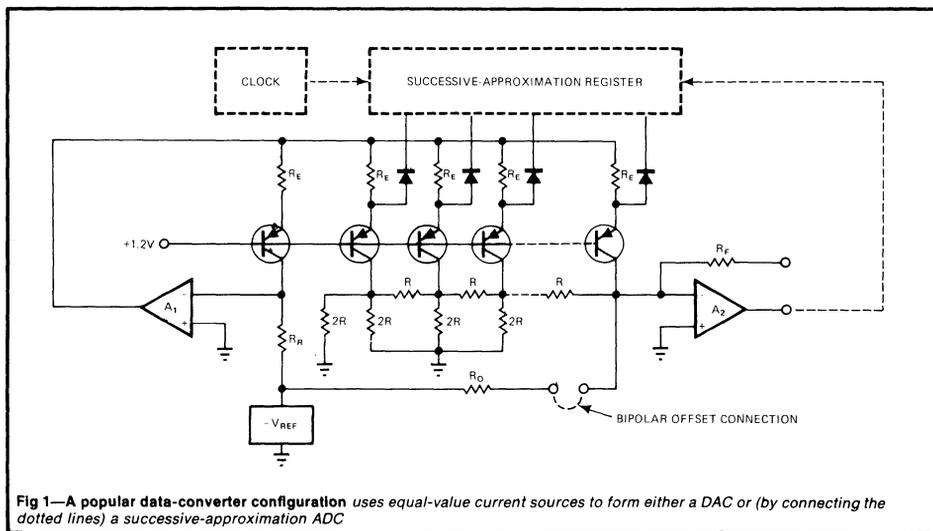
**Fig 1—A popular data-converter configuration uses equal-value current sources to form either a DAC or (by connecting the dotted lines) a successive-approximation ADC**
