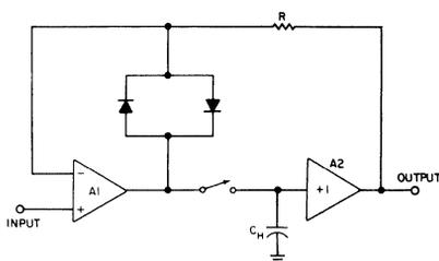
7. Closed-loop sample-holds can also be noninverting. In this configuration,  $A_1$  is both an input buffer and an error-correcting amplifier. When the switch closes, current from  $A_1$  charges the hold capacitor until the output equals the input. The pair of diodes clamps  $A_1$ 's output to keep it stable when the switch is open.
