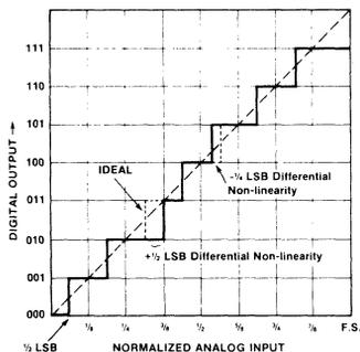
Figure 9: Differential Non-linearity
