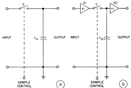
1. In a basic sample-hold circuit (a), the switch closes to sample the input voltage. When the switch opens, the capacitor holds the voltage. A practical circuit (b) has unity-gain buffers to charge the capacitor without loading the source and to drive normal loads without changing the voltage stored by the capacitor.
