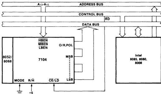
Figure 13: Direct Connection of 8052(8068)/7104 to MCS-80/85 System
