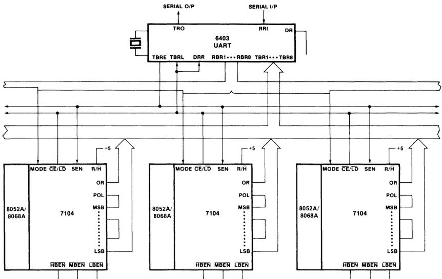
Figure 21: Multiplexing Converters Through the Mode Pin
