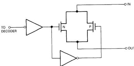
Figure 37. CMOS Analog Switch Circuit
