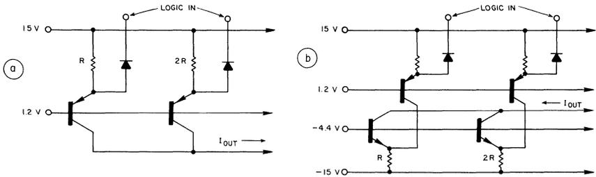
1. Weighted current-source configurations for straight binary (a) and complementary binary (b) coding generation.
