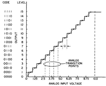
2. The quantizer transfer function for a 4-bit parallel-type converter shows how the analog input is broken into 16 different levels. Each word of digitally coded output signals represents a range,  $Q$ , of input voltage.
