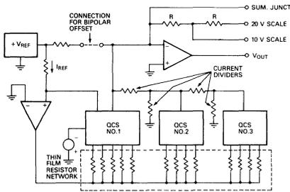
FIGURE 3. 12 Bit Hybrid D/A Converter Circuit
