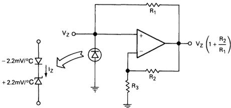
Figure 25. A Precision, Buffered Voltage Reference Circuit
