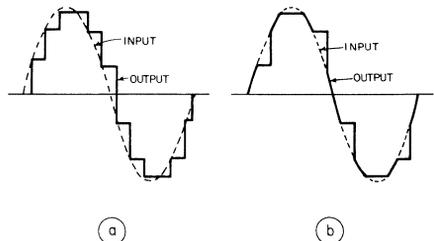
2. A sample-hold can operate in two different ways. It can take a quick sample of the input and return right back to hold mode (a), or it can track the input for part of the time and hold it for the rest (b).
