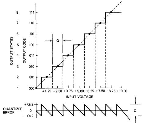
Figure 3. Transfer Function of Ideal 3-Bit Quantizer
