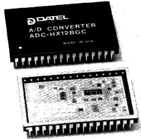
Data converters come in a variety of packages. Shown is a small hybrid 12-bit  $A/D$  converter.
