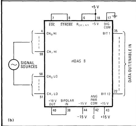
**1. The device.** Hybrid data-acquisition system (a) delivers 12-bit data for 8 differential or 16 single-ended input channels. A few simple connections (b), and the hybrid will automatically address the input channels sequentially for a system throughput rate of 50 kHz.
