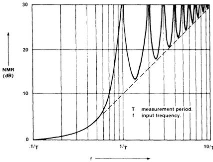
Figure 1: Normal Mode Rejection of dual-slope converter as a function of frequency.
