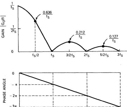
Figure 42. Gain and Phase Components of Zero-Order Hold Transfer Function
