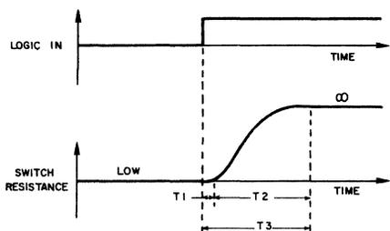
6. A typical analog switch introduces a delay in the sample-to-hold transition.
