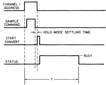
3. A data-acquisition system scans a number of analog inputs and converts them, one at a time, to digital form (a). The sample-hold provides an unchanging input to the
