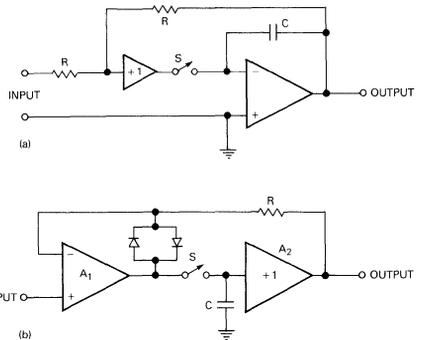
Figure 43. Two Closed Loop Sample-Hold Circuits
