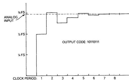
Figure 28. D/A Output for 8-Bit Successive Approximation Conversion
