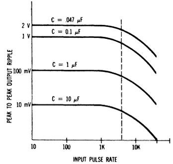
Fig. 2. Output ripple characteristics of the F/F/V-10k.
