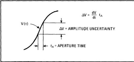
**2. Error.** Possibility of error in a-d conversion depends upon aperture time. The greater  $t_A$  is, the greater the uncertainty in value of an analog voltage that has been converted to digital level.
