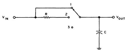
7. An ideal slow opening switch can be modeled by using a simple RC network and a three position switch.
