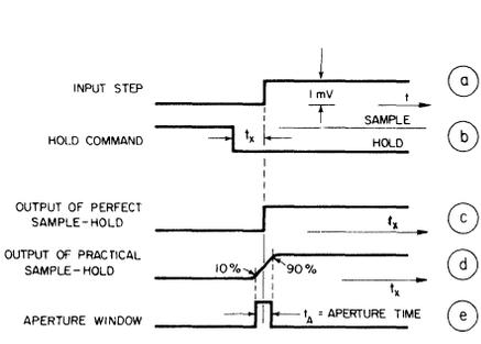
6. **Aperture time can be measured** by repeatedly feeding a tiny step (a) to the sample-hold's input and repeatedly shifting from sample to hold (b) with a varying delay,  $t_x$ . A perfect sample-hold would have an output like (c) as a function of delay time  $t_x$ , but a real sample-hold averages this step over  $t_A$ .
