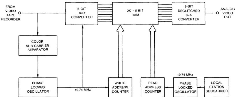
1. Digital time-base correction systems synchronize data converted by this video-speed, 8-bit a/d converter to the
