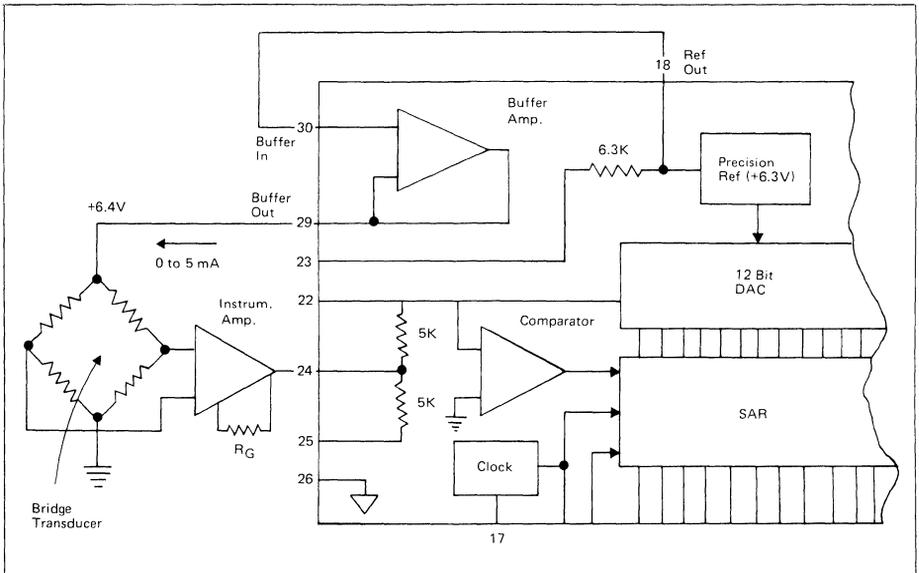
Fig 6 This circuit will provide accurate and stable measurements for computer usage. Because A/D converter's internal buffer amplifier is not used, the amplifier can drive the transducer bridge from the converter's reference.
