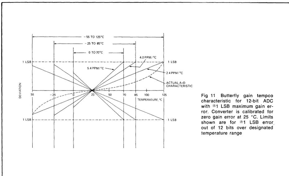
Fig 11 Butterfly gain tempco characteristic for 12-bit ADC with  $\pm 1$  LSB maximum gain error. Converter is calibrated for zero gain error at 25 °C. Limits shown are for  $\pm 1$  LSB error, out of 12 bits over designated temperature range
