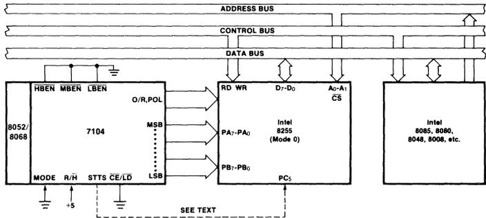
Figure 8: Full Time Parallel Interface 8052(8068)-7104 to MCS-48, 80/85 Families With Interrupt
