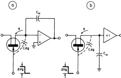
10. **Drain-to-gate capacitance**,  $C_{dg}$ , transfers some charge,  $q$ , when a FET sampling switch opens. The resulting voltage step on the hold capacitor,  $C_H$ , is small if  $C_H$  is large. The switch in the first circuit (a) operates at virtual ground.
