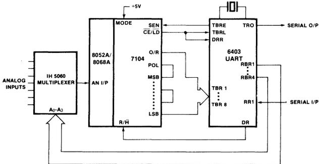
Figure 20: 8052(8068)/7104 Serial Interface Using UART and Analog Multiplexer
