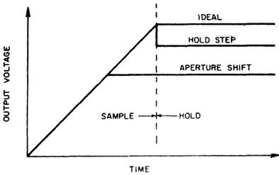
2. Dynamic errors caused by the hold step and the aperture shift are hard to distinguish.
