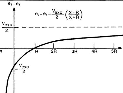
**Fig. 2: This is the plot of a bridge transducer error voltage,  $e_2 - e_1$  vs. the variable leg resistance, X. Plot shows that there is excellent linearity between R and 5R for this transducer, meaning that the transducer is good for monitoring applications in the linear portion.**
