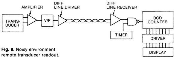
Fig. 8. Noisy environment remote transducer readout.
