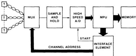
Figure 6(a): Data Acquisition using one central A/D.
