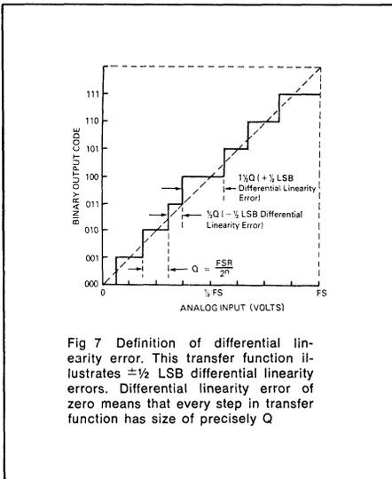
Fig 7 Definition of differential linearity error. This transfer function illustrates  $\pm 1/2$  LSB differential linearity errors. Differential linearity error of zero means that every step in transfer function has size of precisely Q
