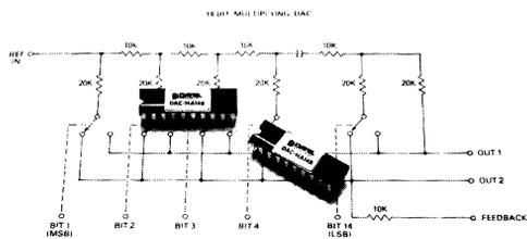
Figure 21. CMOS 14-Bit Multiplying D/A Converters
