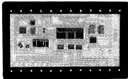
FIGURE 9. Finished Hybrid 12 Bit D/A Converter
