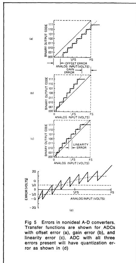
Fig 5 Errors in nonideal A-D converters. Transfer functions are shown for ADCs with offset error (a), gain error (b), and linearity error (c). ADC with all three errors present will have quantization error as shown in (d)
