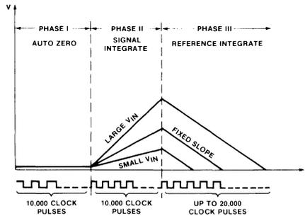
Figure 1:  $4\frac{1}{2}$  Digit A/D Converter Timing Diagram (8052A/7103A)
