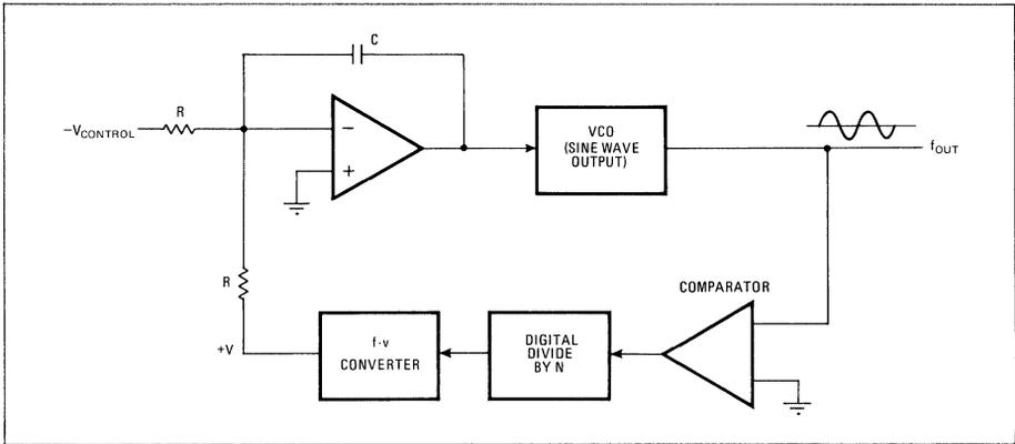
**3. VCO Improvement.** A frequency-to-voltage converter is the key to a low-cost voltage-controlled oscillator. A special feedback control loop forces the VCO output to track the superior linearity and stability of the f-v converter.
