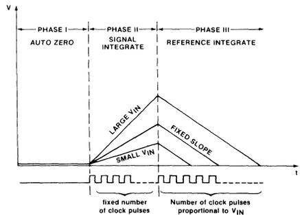
Figure 3: The three phases of a dual-slope conversion.
