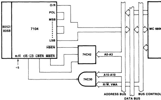
Figure 12: Direct 8052(8068)/7104 to MC6800 Microprocessor Interface
