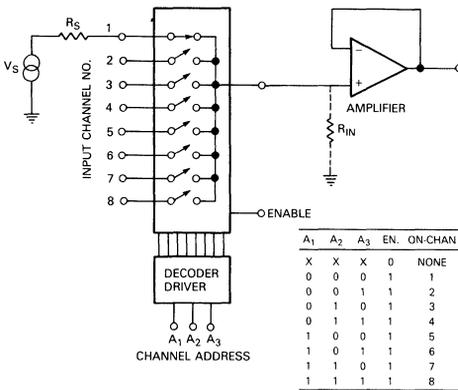
Figure 36. Analog Multiplexer Circuit
