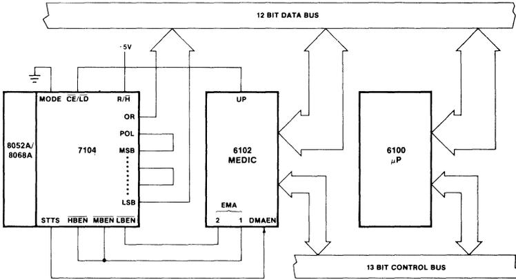
Figure 11: 8052(8068)/7104 Parallel Interface With 6100µP Using DMA
