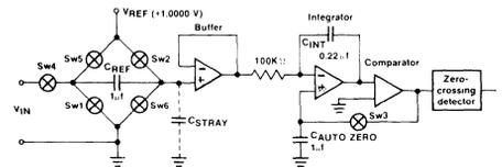
Figure 5: Analog section of a dual slope converter.
