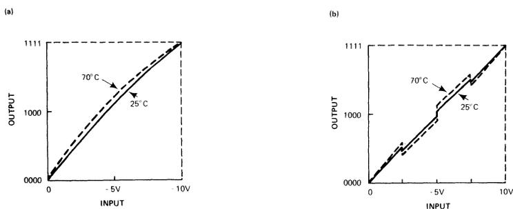
Fig 3—Linearity drift in an integrating A/D converter (a) produces a change in the shape of the transfer function; in a successive-approximation A/D converter (b), it produces larger steps at adjacent code transitions.
