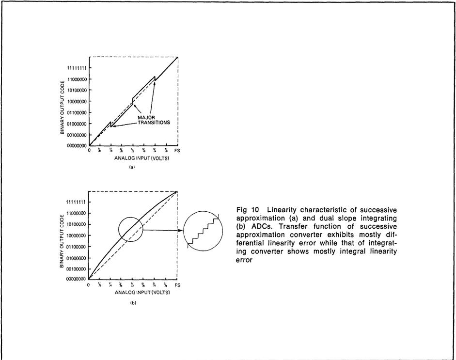
Fig 10 Linearity characteristic of successive approximation (a) and dual slope integrating (b) ADCs. Transfer function of successive approximation converter exhibits mostly differential linearity error while that of integrating converter shows mostly integral linearity error
