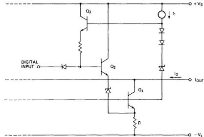
FIGURE 2. Detail Circuit of Quad Current Switching Cell
