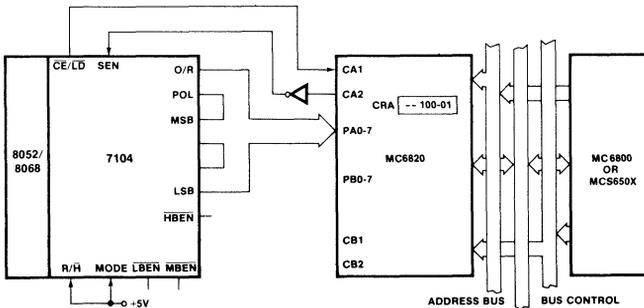
Figure 17: 8052(8068)/7104 to MC6800 or MCS650X Microprocessor With Handshake
