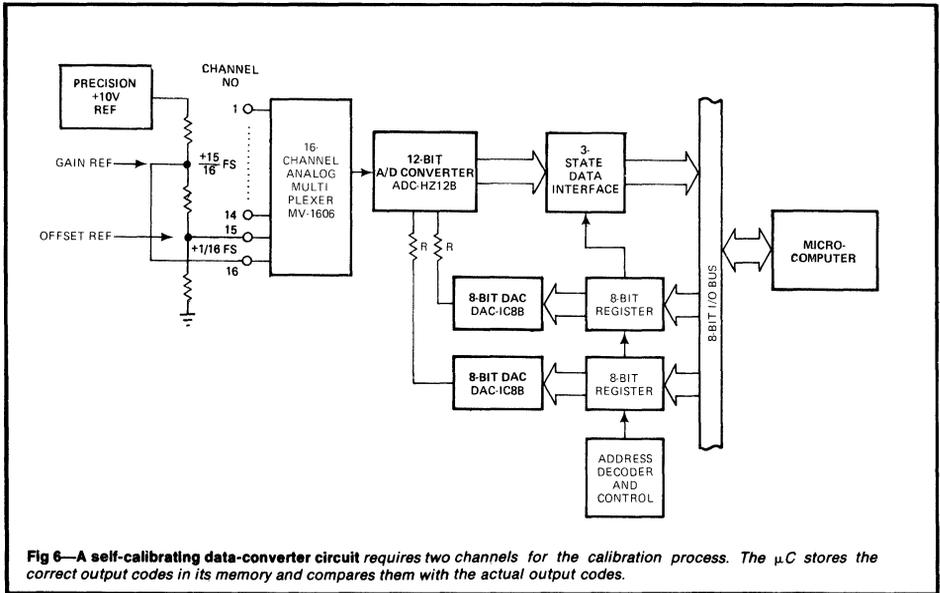
**Fig 6—A self-calibrating data-converter circuit requires two channels for the calibration process. The  $\mu C$  stores the correct output codes in its memory and compares them with the actual output codes.**
