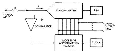
Figure 27. Successive Approximation A/D Converter
