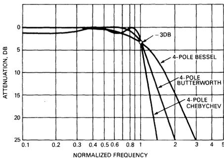
Figure 12. Some Practical Low Pass Filter Characteristics
