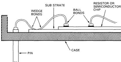
FIGURE 7. Cross-Section of Finished Hybrid Circuit
