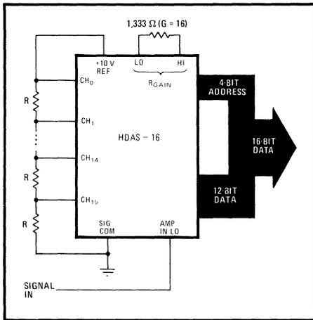
**4. Putting amplifier gain to work.** It is even possible to turn the HDAS-16 into a 16-bit a-d converter by applying the input signal to the internal amplifier's inverting input. Here, the amplifier-input-low line is being viewed as a high-impedance, transient-free signal input.
