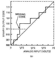
Fig 9 No missing code (a) and missing code (b) in ADC output. Differential linearity error of less than  $\pm 1$  LSB assures that there are no missing codes in transfer function
