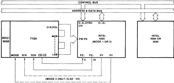
Figure 18: 8052A-7104 to MCS4/40 Microprocessor With Handshake
