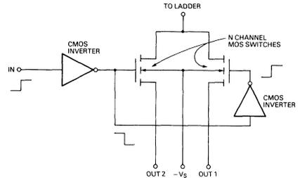
**FIGURE 21. Single Pole, Double Throw CMOS Switch**
