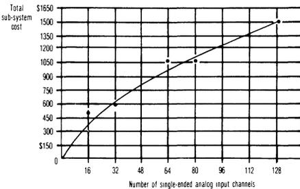
**Fig. 1: The cost per channel for A/D converter subsystems increases linearly after the initial master board is purchased. If major components, such as a printed circuit board or chassis, have to be added, the costs can go up dramatically. Although this figure illustrates Datel Systems components, other manufacturers generally are within 10% of these prices (assuming identical configurations).**
