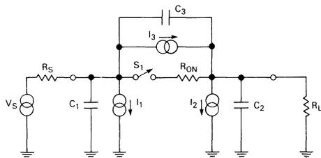
Figure 39. Equivalent Circuit of Analog Multiplexer Switch
