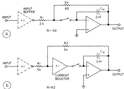
6. This type of inverting, closed-loop circuit is both accurate and simple. The charge time constant,  $R_2 C_H$ , of the basic circuit (a) is much too long for some applications. The current booster in (b) speeds up charging considerably. The input resistance,  $R_1$ , may be too low for some sources; the buffer raises it a great deal.
