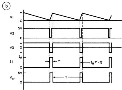
1. The basic charge balancing v/f converter (a) uses an operational integrator with a precision timing circuit con-
