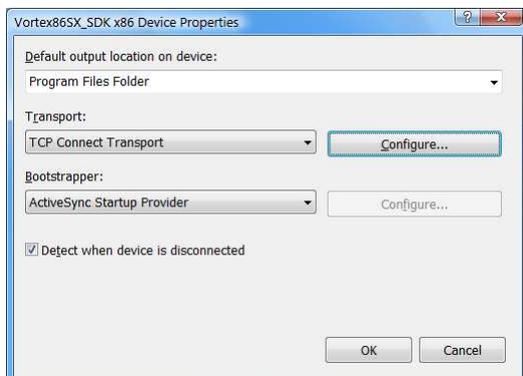
4. You have to get IP address of your Windows CE device. Run **ipconfig** in Windows CE device or run **"s ipconfig /d"** in Tagret Control window and the output of ipconfig will send output to debug window. Select "Use specific IP address" and fill IP address of your device. Press OK three times to finish setup.
