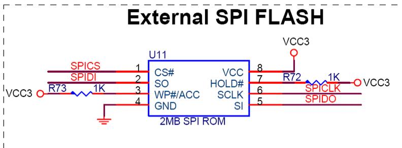
If pin 3 (WP#) in above circuit is pulled high, SPITool can accept “protect” and “unprotect” parameters to set write protection of SPI flash disk. After you setup SPI flash disk and disable changing write protection mode of flash disk, please connect pin 3 to low.
