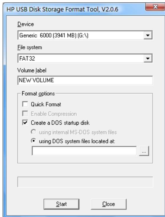
Select your DOS system path and press start button to make USB pen drive DOS bootable.
