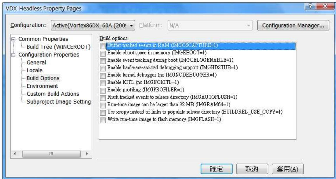
When settings are ready, build new Windows CE image. Boot is from USB or DOM for test in next section.
