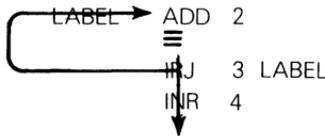
The IRJ instruction specifies Register 3 as the register to be incremented. After incrementing, if the low order eight bits of Register 3 are all 0, then the INR instruction will be executed; otherwise the ADD instruction will be executed.
