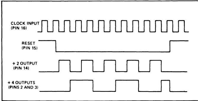
Figure 3. Timing Diagram for Frequency Divider Section.
