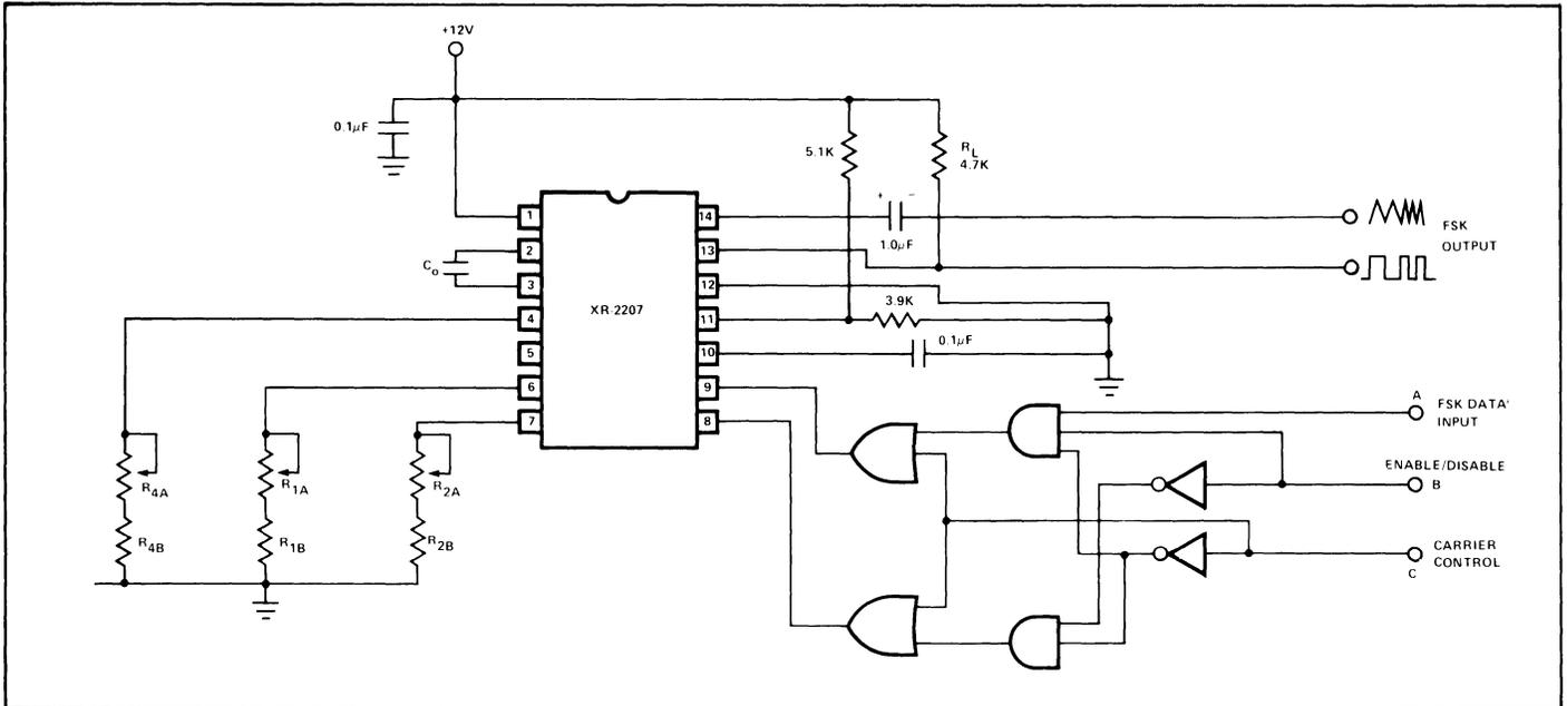
Figure 4. Tri-State FSK Transmitter using the XR-2207.
