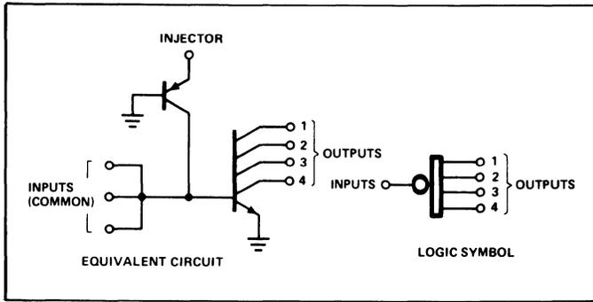
Figure 7. Four-Output I<sup>2</sup>L Gate.
