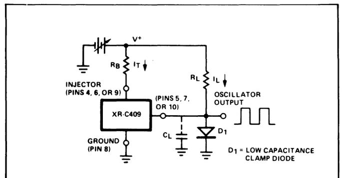
Figure 9. Recommended Test Circuit for Evaluating Power-Delay Characteristics of I<sup>2</sup>L Gates Using Ring Oscillator Sections of XR-C409.
