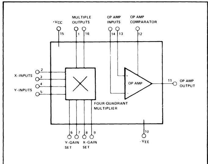
Figure 5. Functional Block Diagram of XR-2228 Multiplier/Detector
