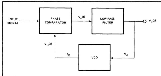
Figure 1. Block Diagram of a Phase-Locked Loop.
