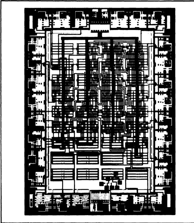
**Figure 14. Photo-Micrograph of a Typical Semi-Custom I<sup>2</sup>L LSI Chip.**
