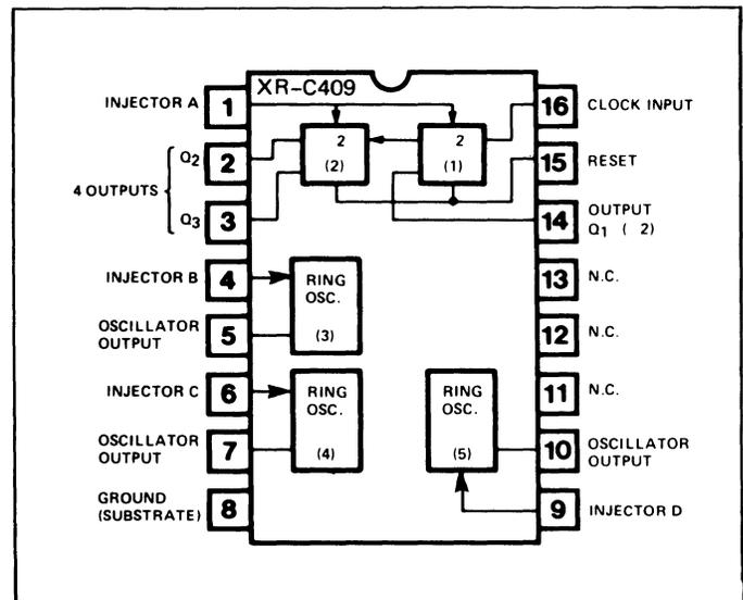
Figure 1. Package Terminals for XR-C409 Test IC.
