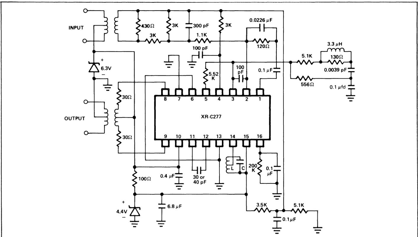
Figure 6. Typical Circuit Connection of XR-C227 in 1.544 MHz T-1 Repeater System. (Note: Set L and C to form a high Q tank resonant at 1.544 MHz. It is recommended that  $Q < 100$ , and  $C \approx \text{pF}$  for most applications).
