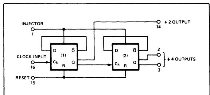
Figure 2. Block Diagram of Frequency Divider Section.
