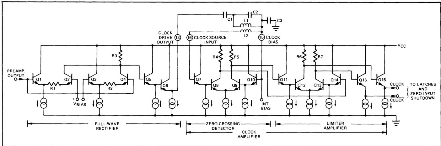
Figure 10. Circuit Diagram of the Clock Recovery Section.
