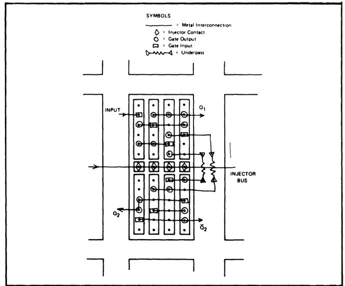
Figure 6. Sample Pencil Layout on a Logic Cell.
