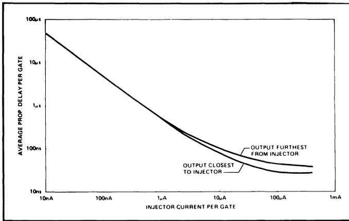
Figure 8. Propagation Delay Characteristics of I<sup>2</sup>L Gates as a Function of Injector Current.
