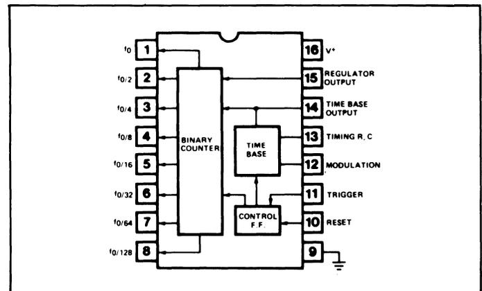
Figure 2. Functional Block Diagram of XR-2240 Counter/Timer.
