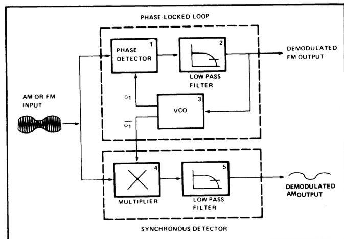
Figure 2. The Basic Phase-Locked Loop AM Detector
