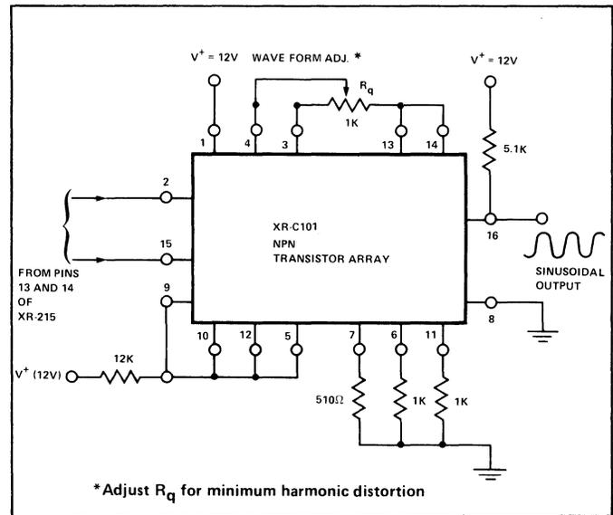
**Figure 5. Use of XR-C101 Transistor Array to Obtain Sinusoidal Output from XR-215 PLL**
