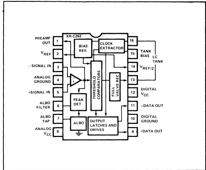
Figure 2. Package Diagram of XR-C262 Monolithic PCM Repeater.
