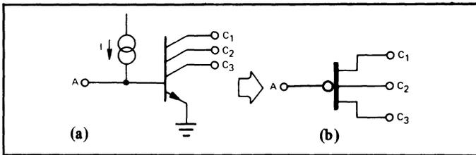
Figure 2. Equivalent Circuit (a), and a recommended symbol (b) for an I<sup>2</sup>L Gate.
