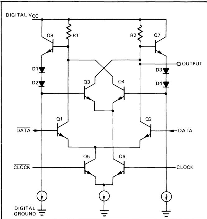
**Figure 8. Circuit Configuration for Tracking Data Latches.**
