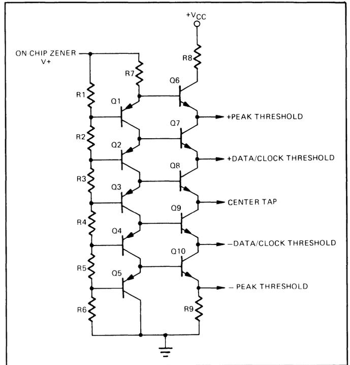
**Figure 9. Internal Voltage-Divider Network for Comparator Threshold Setting.**
