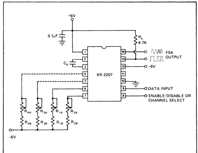
Figure 3. The XR-2207 FSK Modulator Split-Supply Operation
