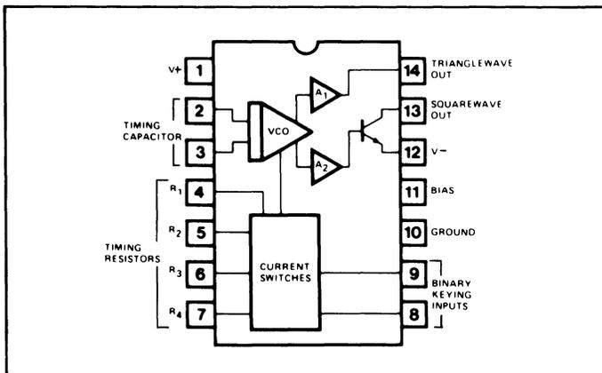
Figure 1. Functional Block Diagram of XR-2207 Oscillator Circuit.
