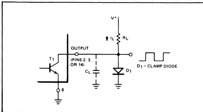
Figure 5. Recommended External Connections to Measure Output Waveforms.
