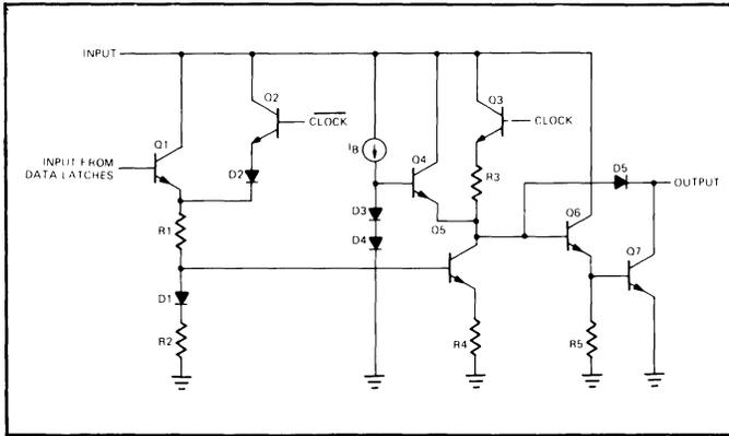
Figure 12. Circuit Configuration for the Output Drivers.
