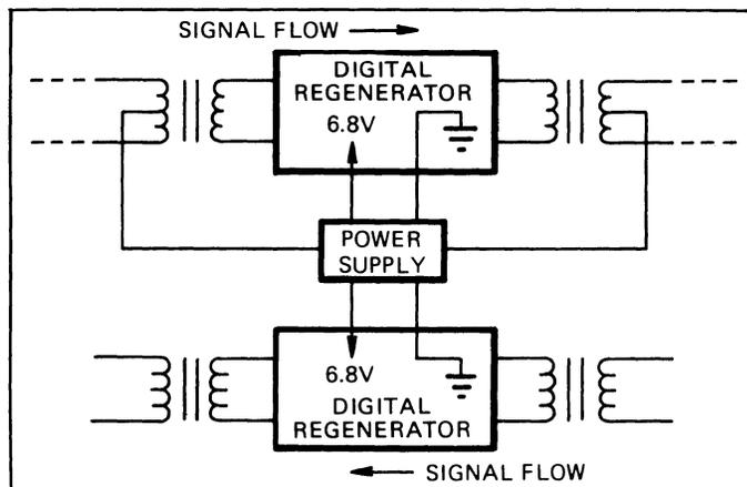
Figure 1. Block Diagram of a Bi-Directional Repeater System.
