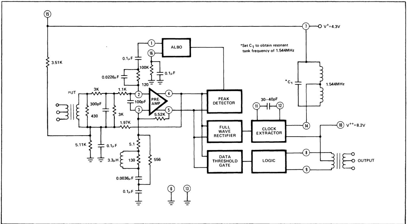
Figure 5. External Components Necessary for Circuit Operation
