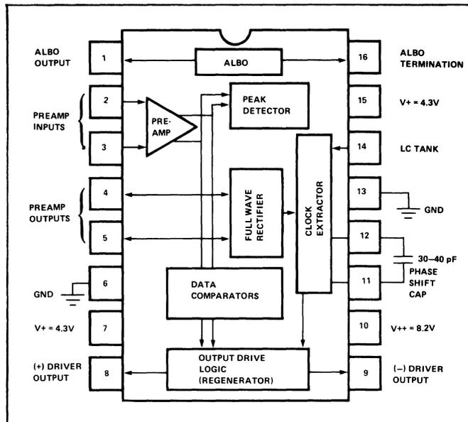
Figure 3. Package Diagram of XR-C240 Monolithic PCM Repeater
