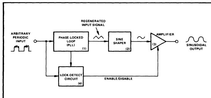
Figure 1. Basic Concept of a Regenerative Sinewave Converter.
