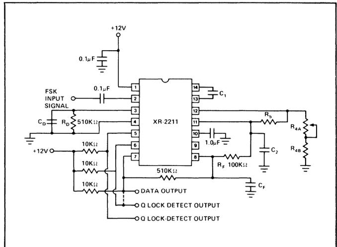
Figure 4. The XR-2211 FSK Demodulator with Carrier Detect
