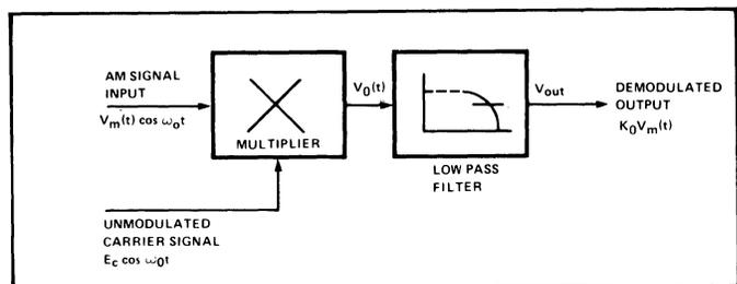
Figure 1. Block Diagram of a Synchronous AM Detector
