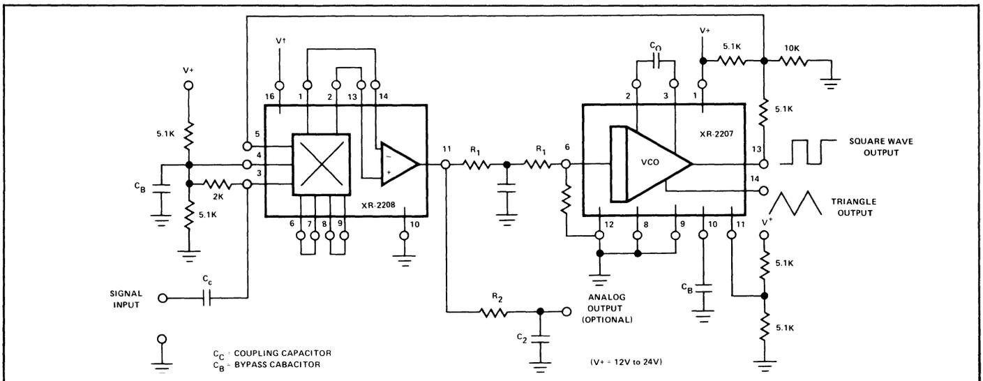
Figure 4. Circuit Interconnections for Single Supply Operation.
