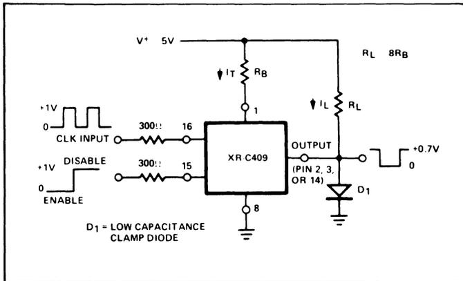
Figure 4. Test Circuit for Frequency Divider Section.
