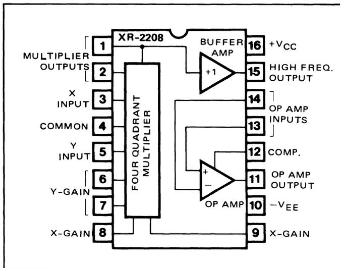
Figure 5. Block Diagram of XR-2208 Operational Multiplier.
