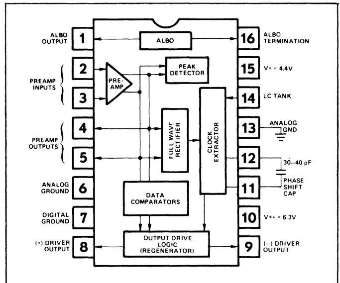
**Figure 3. Package Diagram of XR-C277 Monolithic PCM Repeater**
