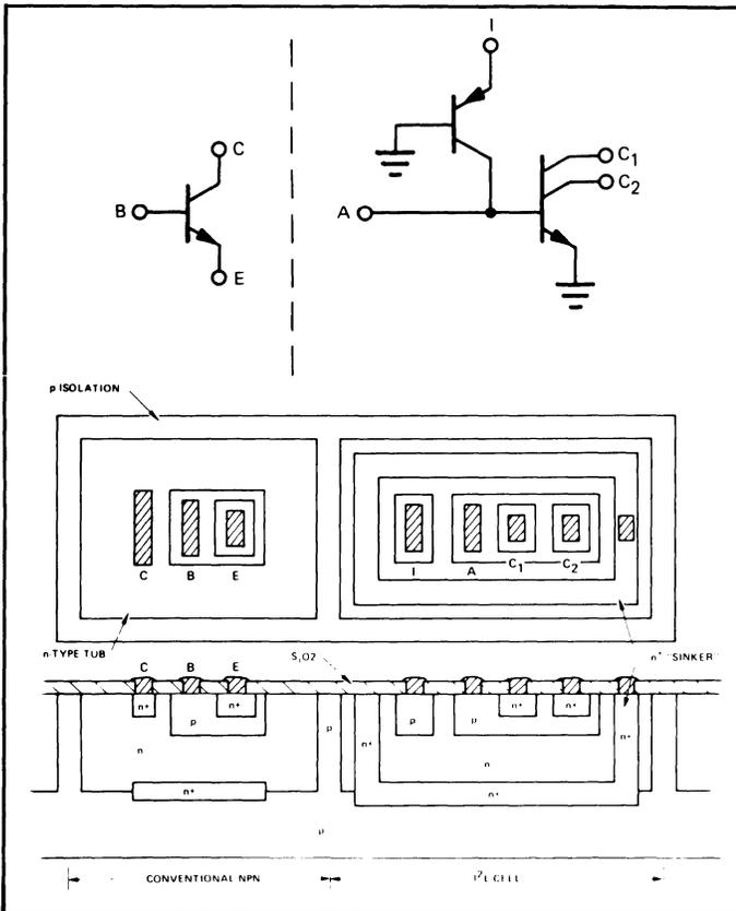
Figure 3. Basic Device Structure for Bipolar Compatible I<sup>2</sup>L.
