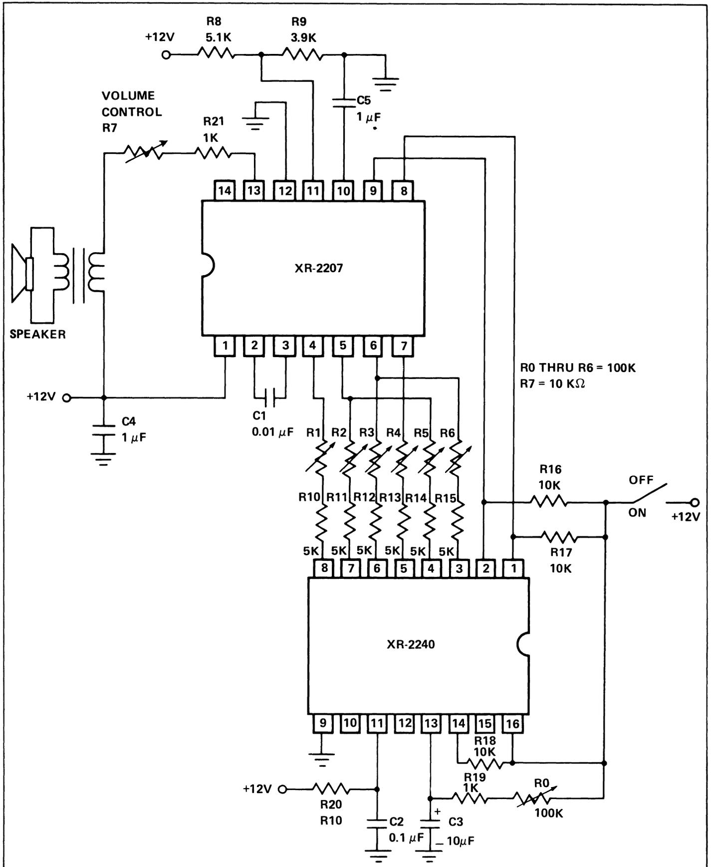
Figure 3. Circuit Connection Diagram for the Music Synthesizer.
