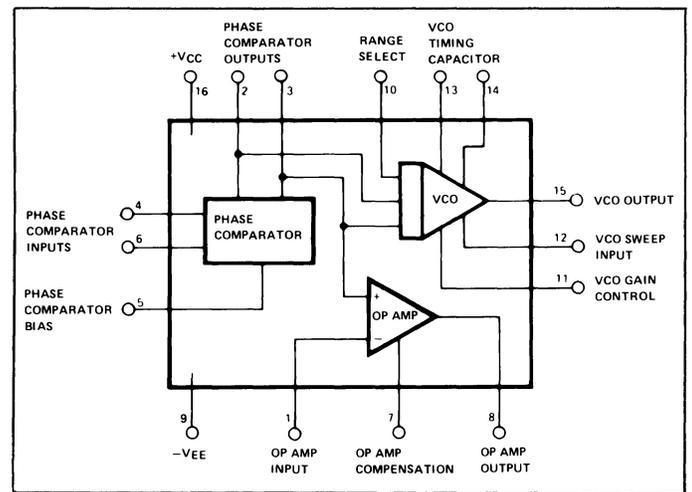
Figure 1. Functional Block Diagram of XR-215 Phase-Locked Loop
