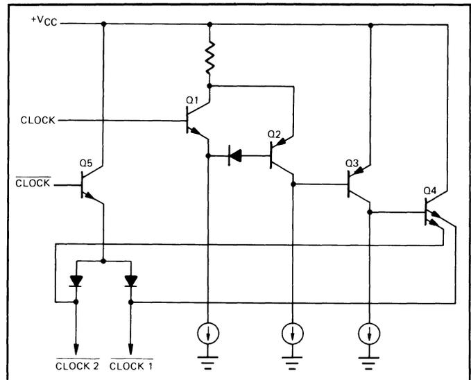
Figure 11. Zero-Input Shutdown Circuit for Output Protection.
