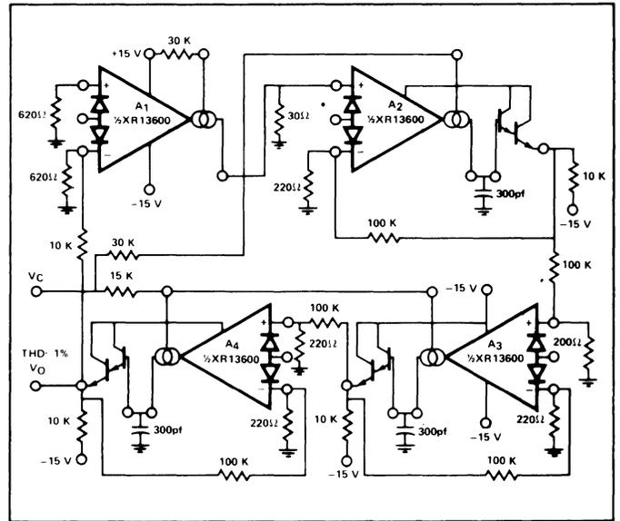
Figure 17. Sinusoidal VCO using two XR-13600 Circuits
