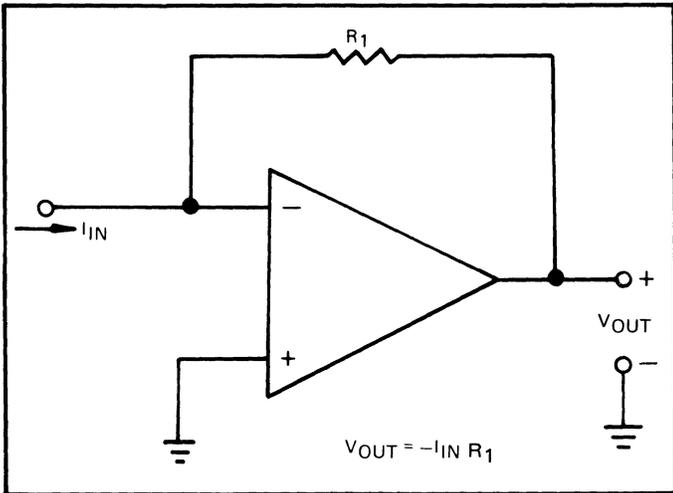
Figure 11. Operational Amplifier as a Current-to-Voltage Converter.
