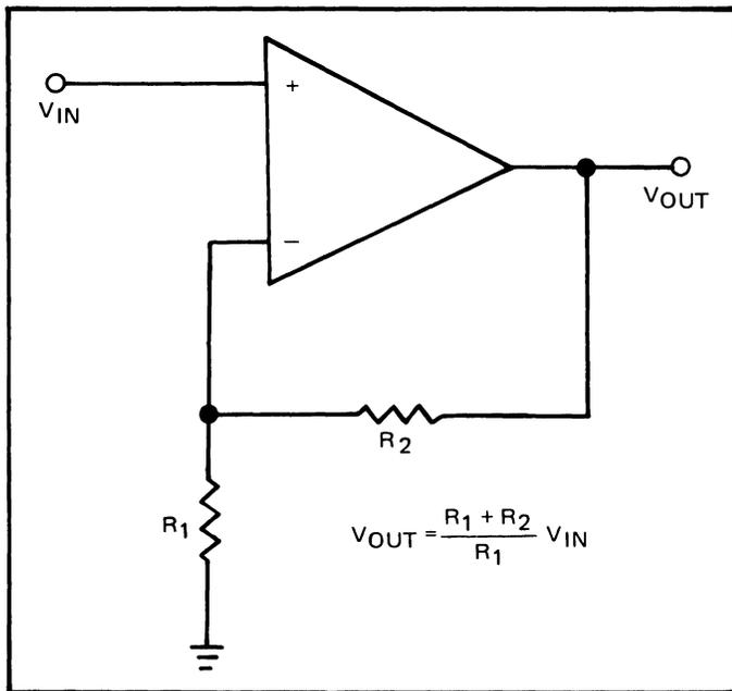
Figure 2. Non-Inverting Amplifier
