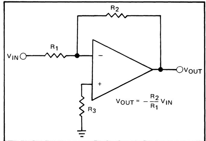
Figure 1. Inverting Amplifier
