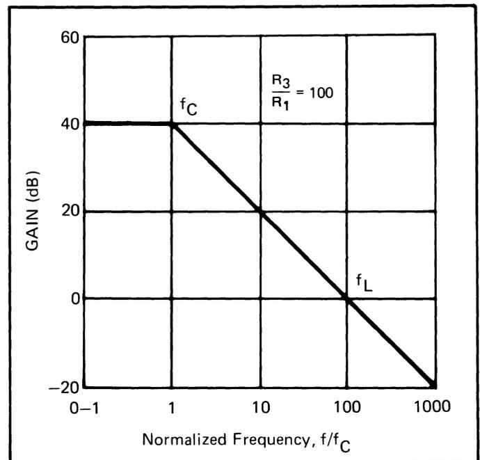
Figure 10. Frequency Response of the Simple Low-Pass Filter.
