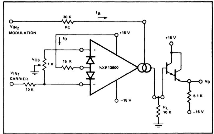
Figure 5. Amplitude Modulator
