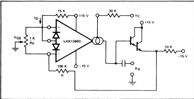
**Figure 9. Voltage Controlled Resistor with Linearizing Diodes**
