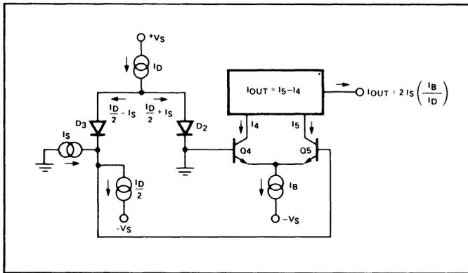
Figure 1. Linearizing Diodes
