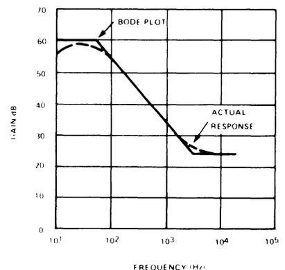
BODE PLOT OF NAB EQUALIZATION AND THE RESPONSE REALIZED IN THE ACTUAL CIRCUIT USING THE XR 5534
