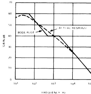
BODE PLOT OF RIAA EQUALIZATION AND THE RESPONSE REALIZED IN AN ACTUAL CIRCUIT USING THE XR 5534
