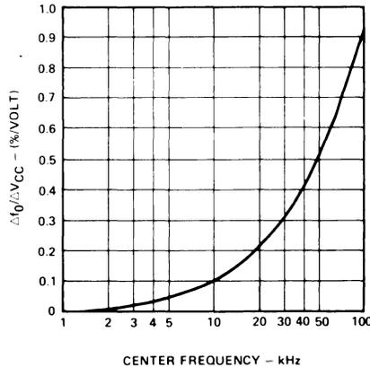
Figure 11. Power Supply Dependence of Center Frequency
