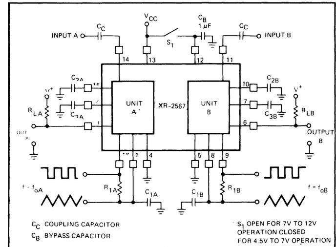
Figure 4. Circuit Connection Diagram
