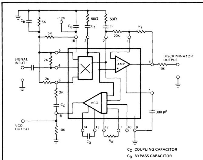
Figure 24 Circuit Connection For Tracking Filter Applications
