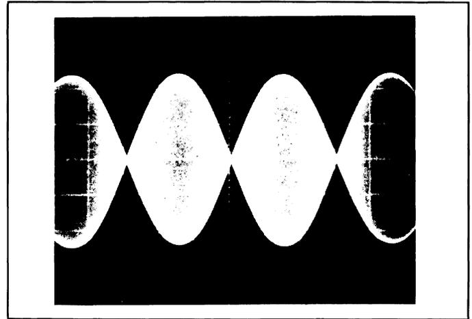
Figure 22-2. Suppressed Carrier AM Output Waveform
