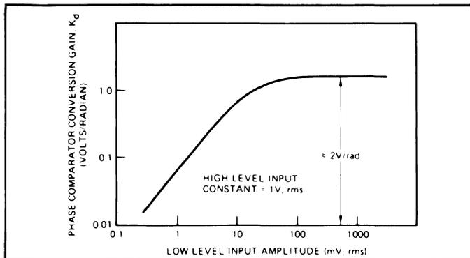
Figure 8. Phase Comparator Conversion Gain, K<sub>d</sub>, versus Input Amplitude
