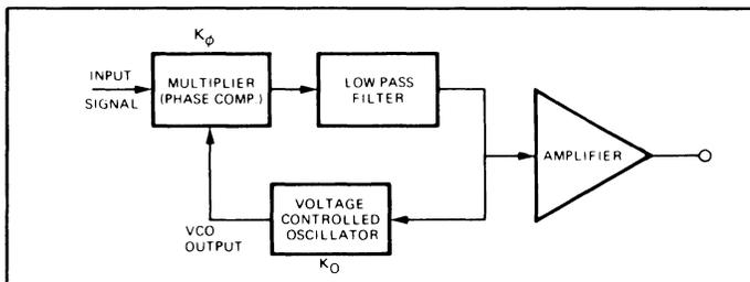
Figure 16. XR-S200 as a Phase-Locked Loop
