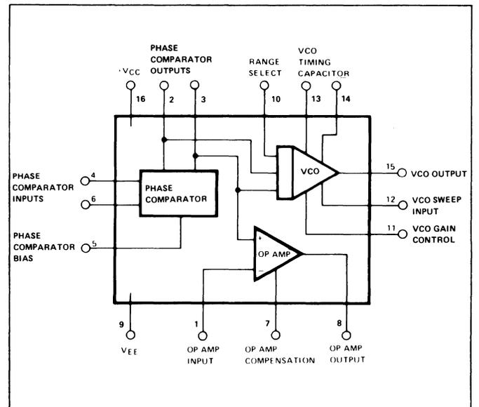
**Figure 5. Functional Diagram of XR-215 High-Frequency Phase-Locked Loop**
