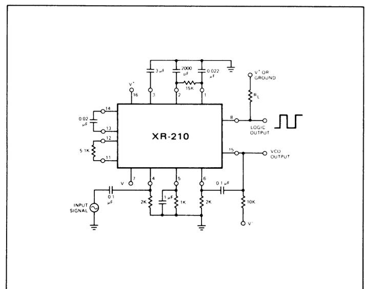
Figure 4. Test Circuit for Split Supply Operation
