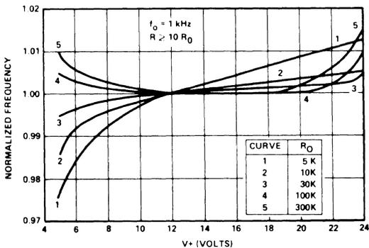
Figure 7. Typical  $f_0$  vs Power Supply Characteristics.
