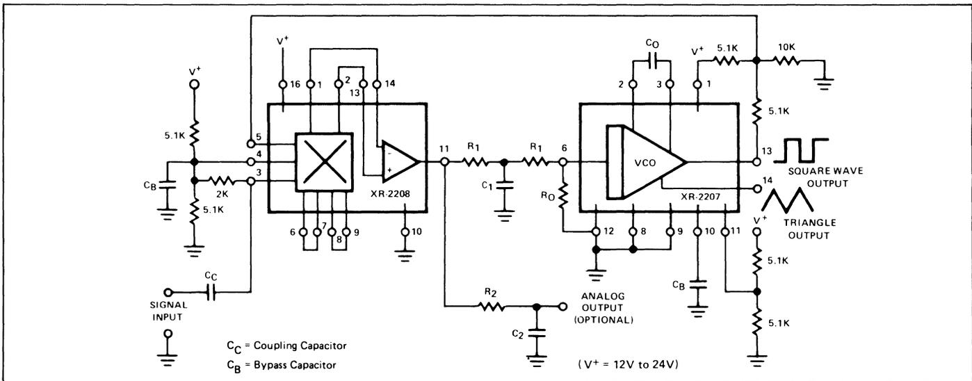
Figure 2. Circuit Interconnections for Single Supply Operation.
