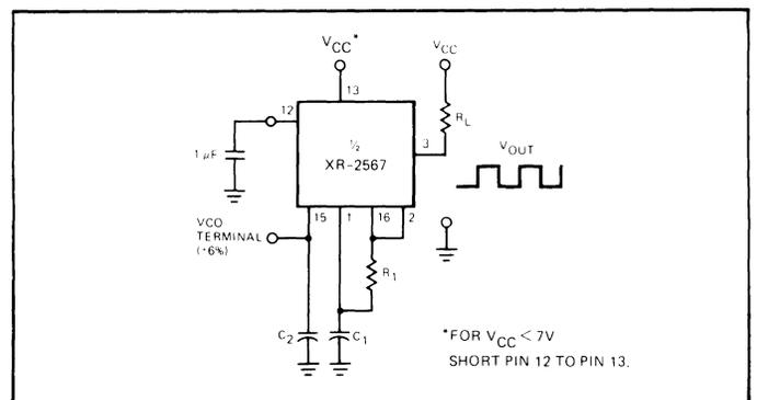
Figure 27. Precision Oscillator with High Current Output Capability
