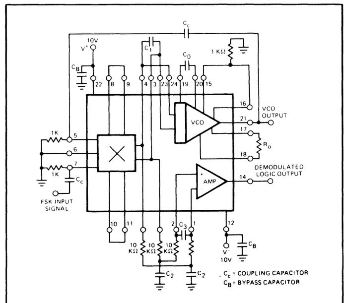
Figure 18. FSK Detection
