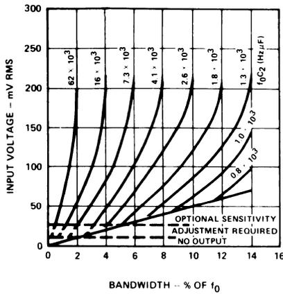
Figure 6. Bandwidth Versus Input Signal Amplitude ( $C_2$  in  $\mu\text{F}$ )
