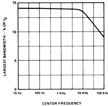
Figure 4. Largest Detection Bandwidth Versus Operating Frequency
