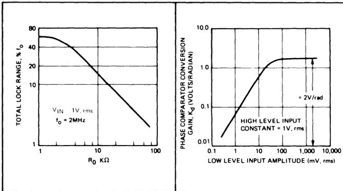
Figure 9. Total Lock Range,  $\pm\Delta f_L$ , vs VCO Gain Control Resistor,  $R_0$  Figure 10. Phase Detector Conversion Gain,  $K_d$ , versus Input Amplitude
