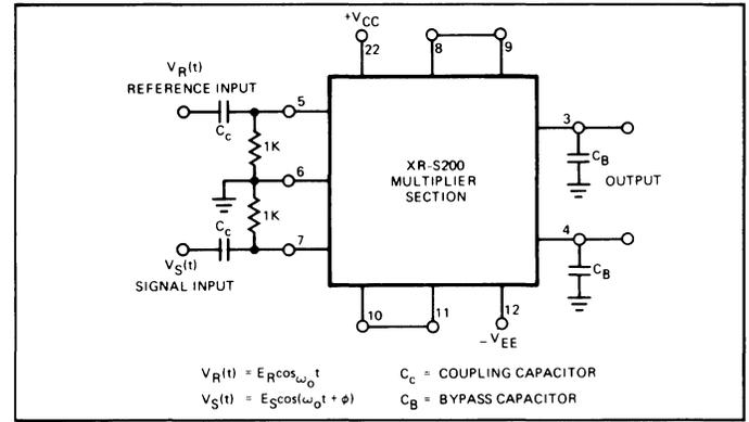
Figure 4. XR-S200 Multiplier Section as a Phase Comparator
