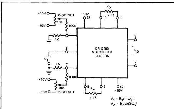
Figure 8. Multiplier Section as Frequency Doubler
