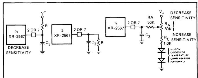
Figure 17. Optional Connections for Sensitivity Control
