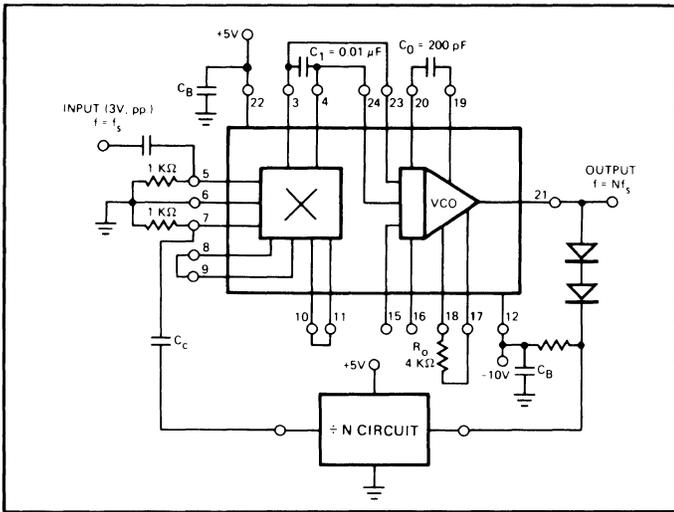
Figure 19. Frequency Synthesizer
