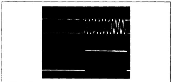
Figure 26. Input and Output Waveforms for FSK Decoding
