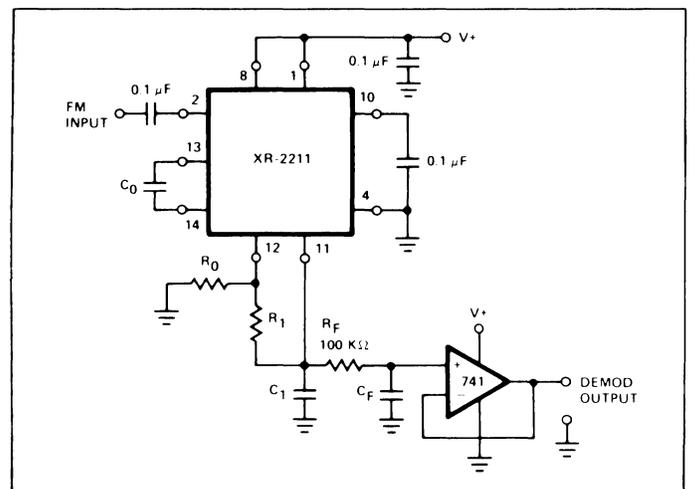
Figure 12. Linear FM Detector Using XR-2211 and an External Op. Amp. (See section on Design Equations, for Component Values)
