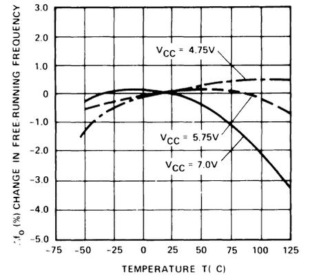
Figure 9. Frequency Drift With Temperature
