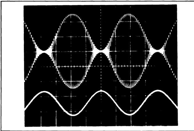
Figure 7-1. AM Modulation, 95% AM,  $f_c = 50$  kHz,  $f_m = 1$  kHz
