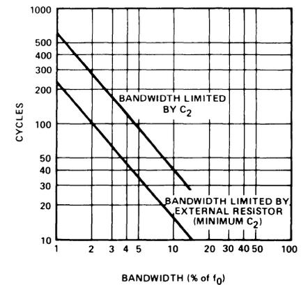
Figure 12. Greatest Number of Cycles Before Output
