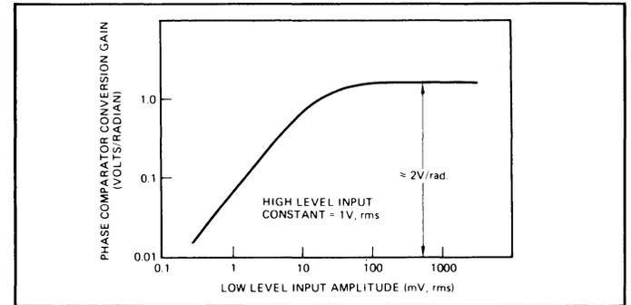
Figure 5. Phase Comparator Conversion Gain Versus Input Amplitude
