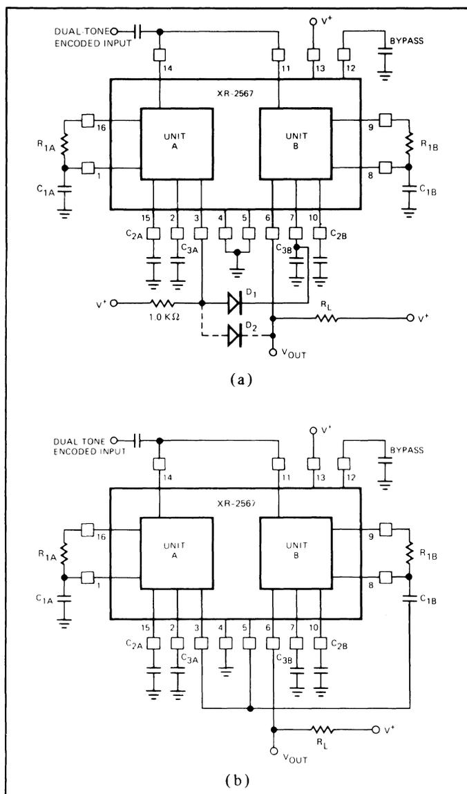
Figure 24. Additional Dual-Tone Decoding Circuits
