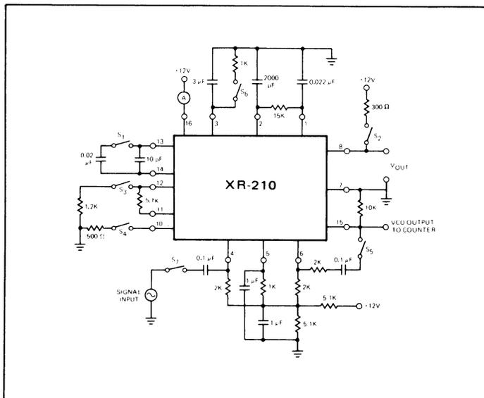
Figure 3. Test Circuit for Single Supply Operation
