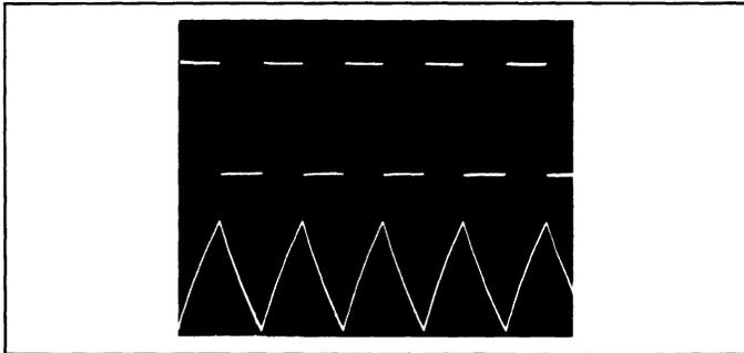
Figure 22. Oscillator Output Waveform Available From CCO Section.
