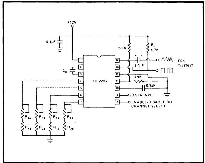
Figure 2. The XR-2207 FSK Modulator Single-Supply Operation
