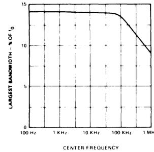
Figure 9. Largest Detection Bandwidth vs. Operating Frequency
