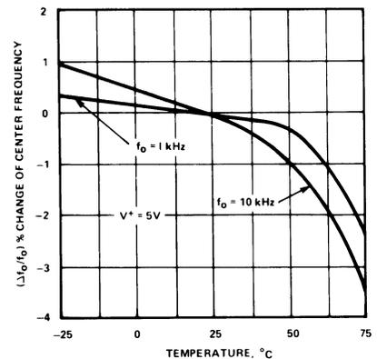
Figure 11. Typical Frequency Drift as a Function of Temperature
