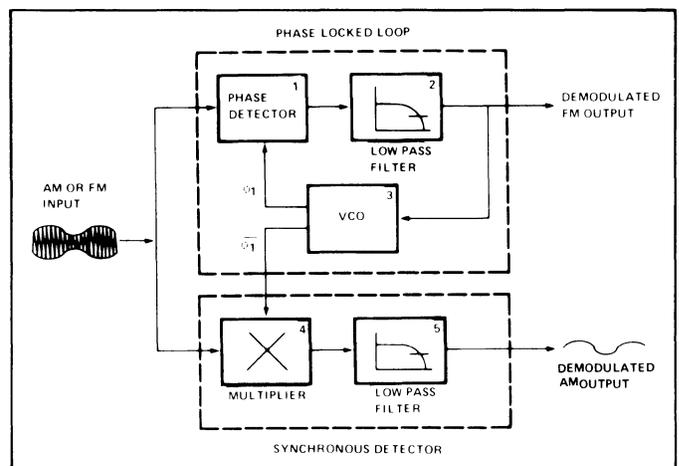
Figure 2. The Basic Phase-Locked Loop AM Detector
