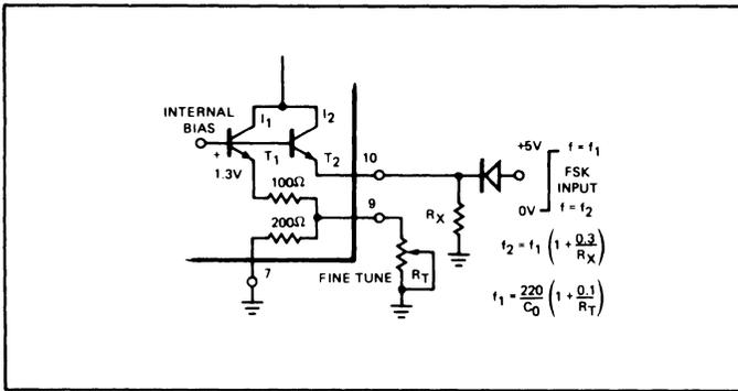
Figure 8. VCO Fine-Tune (Pin 9) and Frequency-Keying (Pin 10) Controls
