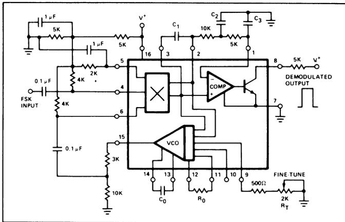
Figure 5. Circuit Connection for FSK Demodulation (Single Supply)
