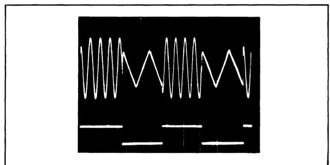
Figure 19 Demodulated Output Waveforms for Time-Multiplexed Operation
