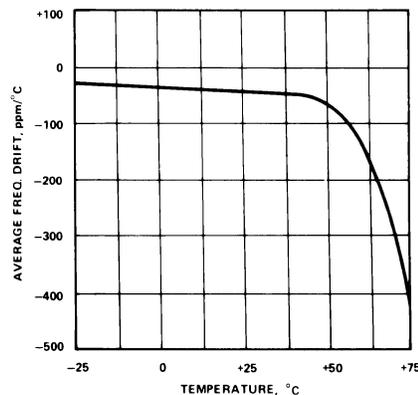
Figure 10. Typical Center Frequency Drift with Temperature ( $V^+ = 5\text{V}$ ,  $R_1 = 80\text{ k}\Omega$ ,  $f_0 = 1\text{ kHz}$ )
