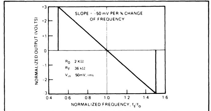
Figure 26. Typical Discriminator Output Characteristics For Tracking Filter Applications
