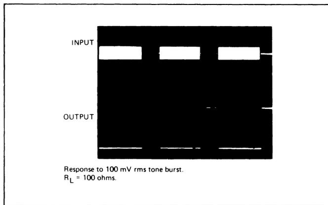
Figure 12. Typical Output Response to 100 mV Input Tone-Burst
