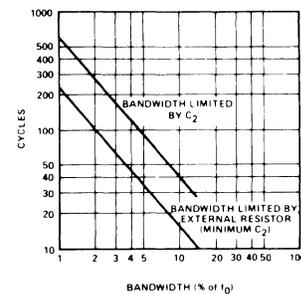
Figure 11. Greatest Number of Cycles Before Output
