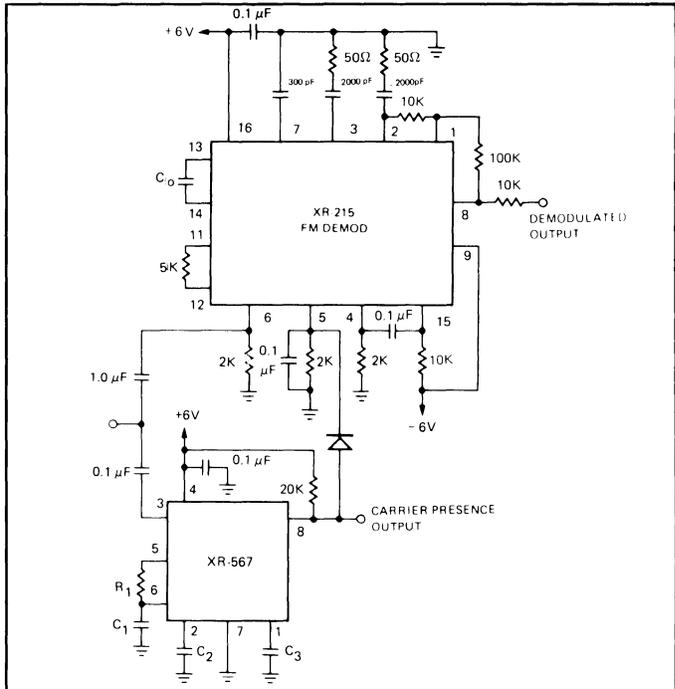
Figure 20. Narrow Band FM Demodulator with Carrier Detect
