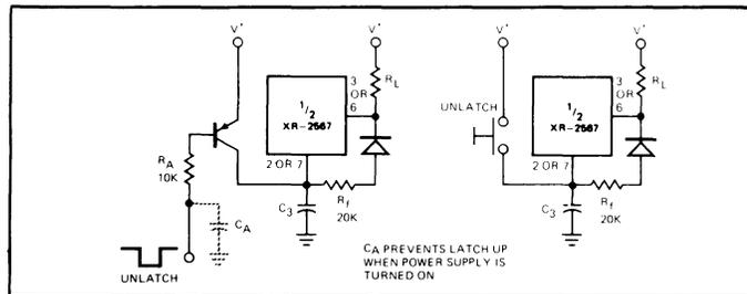
Figure 20. Output Latching
