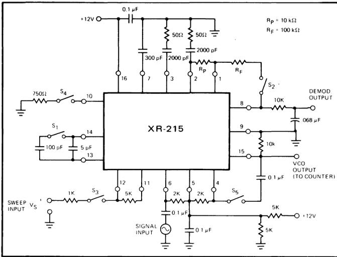
Figure 2. Test Circuit For Single Supply Operation
