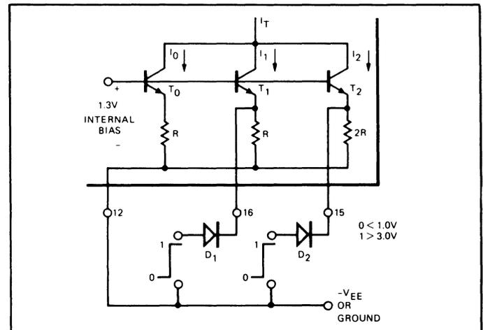
Figure 15. Explanation of VCO Digital Controls
