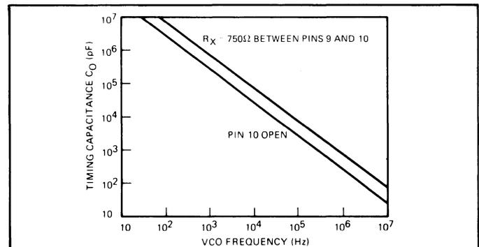
Figure 7. VCO Free Running Frequency vs Timing Capacitor
