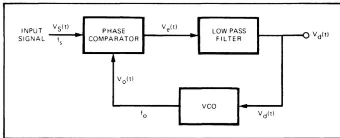
Figure 12 Block Diagram of a Phase-Locked Loop
