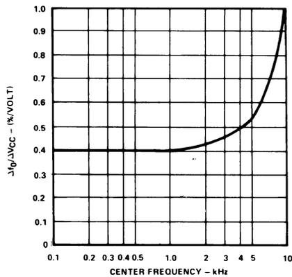
Figure 9. Power Supply Dependence of Center Frequency
