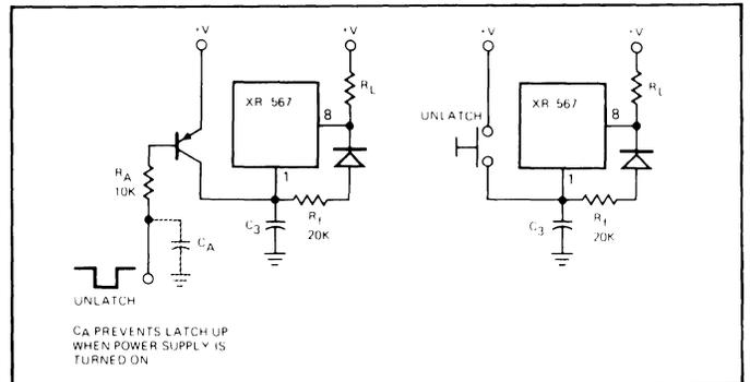
Figure 17. Output Latching
