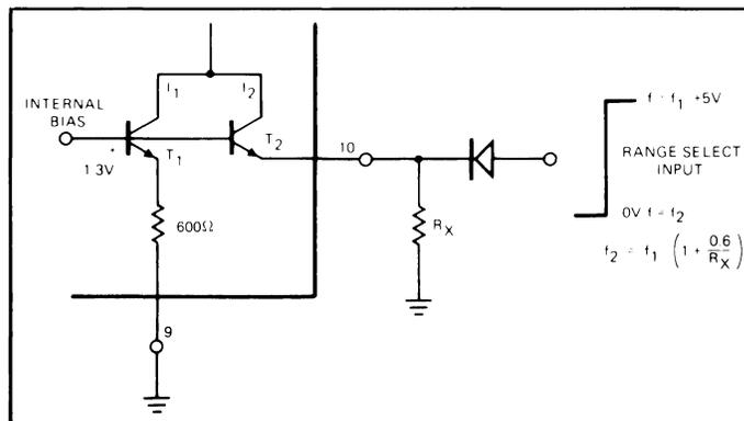
Figure 11 Explanation of VCO Range-Select Controls
