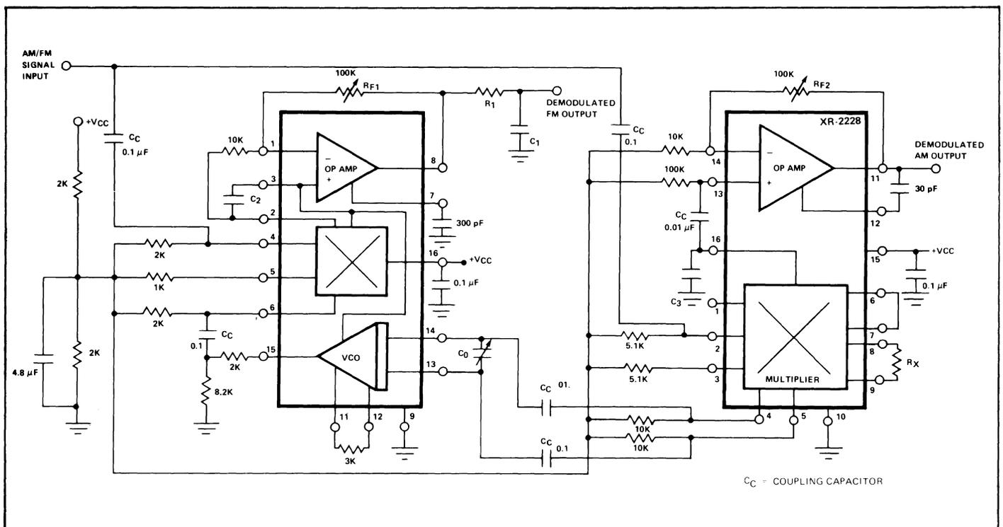
Figure 8. Circuit Connection for a High-Frequency AM and FM Detector Using the XR-215 and the XR-2228
