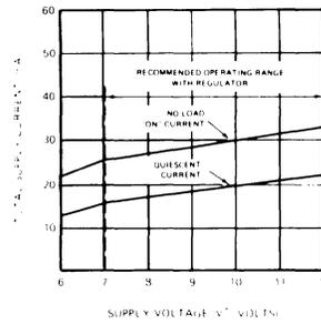
Figure 8. Total Supply Current vs. Supply Voltage for Operation with Internal Regulator (Pins 12 and 13 Not Connected)
