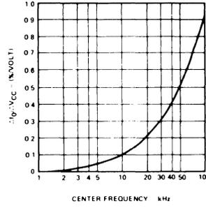
Figure 6. Power Supply Dependence of Center Frequency
