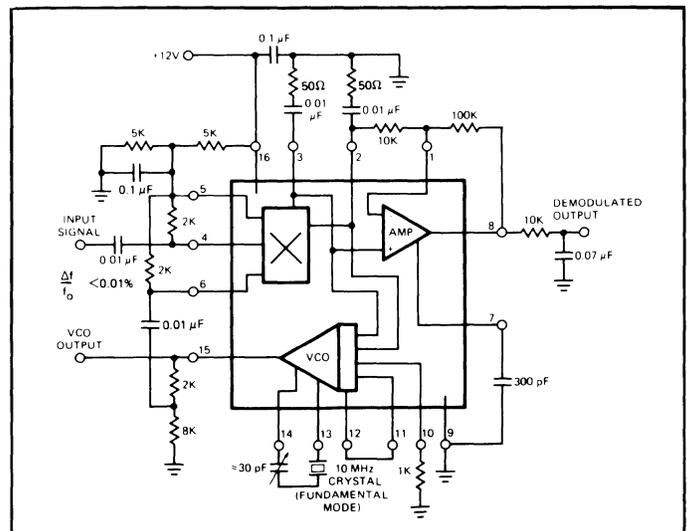
Figure 27 Typical Circuit Connection For Crystal-Controlled FM Detection
