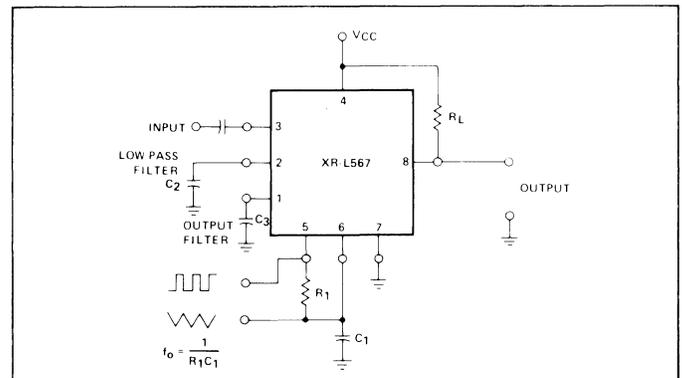
Figure 2. XR-L567 Generalized Connection Diagram
