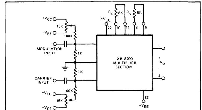
Figure 6. Suppressed Carrier Modulation Using XR-S200 Multiplier Section
