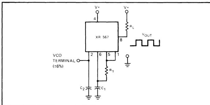
Figure 23. Precision Oscillator to Switch 100 mA Loads
