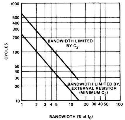
Figure 8. Greatest Number of Cycles Before Output:
