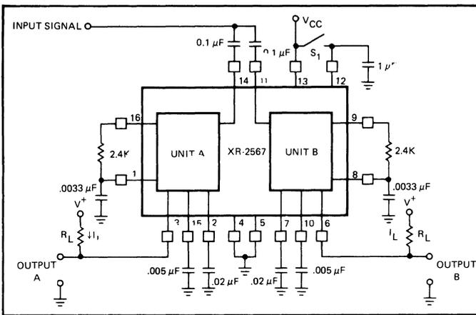
Figure 2. Test Circuit
