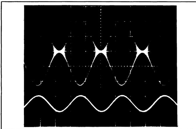
Figure 22-1. Double Sideband AM Output Waveform
