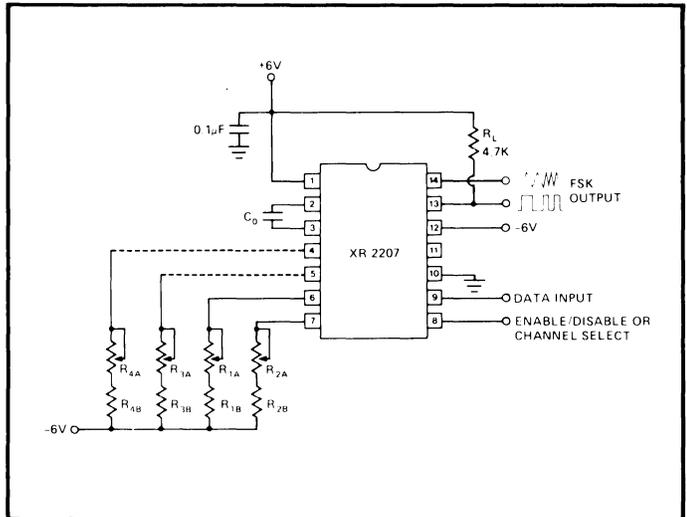
Figure 3. The XR-2207 FSK Modulator Split-Supply Operation
