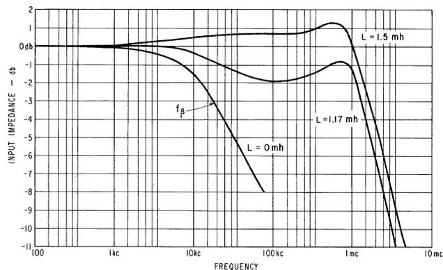
Fig. 4(b) Input Impedance Frequency Response
