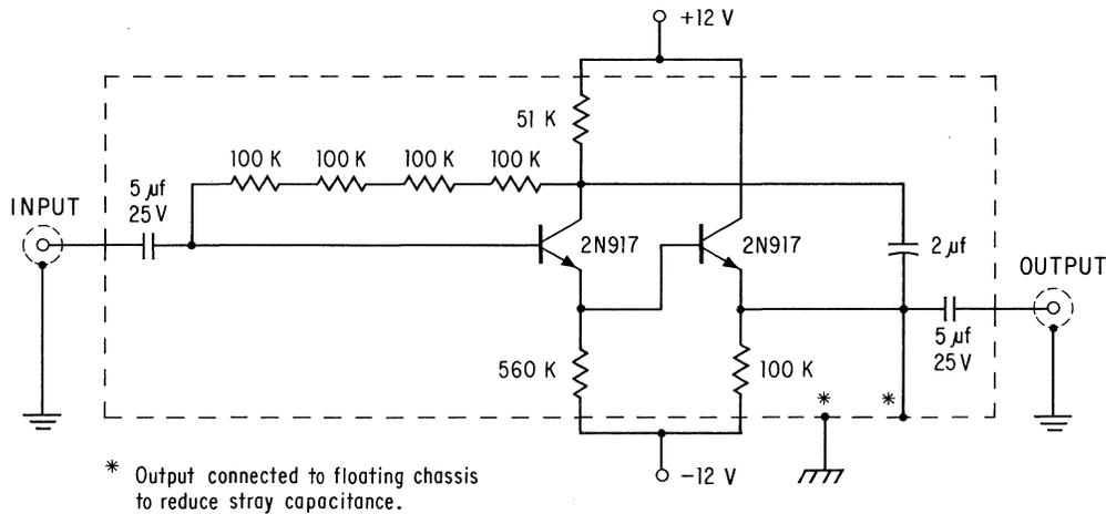
Fig. 5 Wideband High Input Impedance Amplifier.
