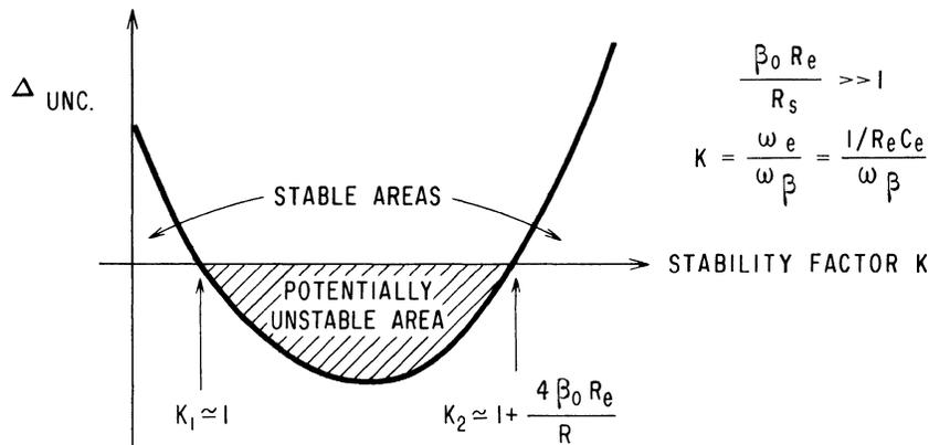
Fig. 2 Graphical Representation of Values of the Stability Factor K Where Nonoscillatory Conditions Are Ensured for the Uncompensated Case
