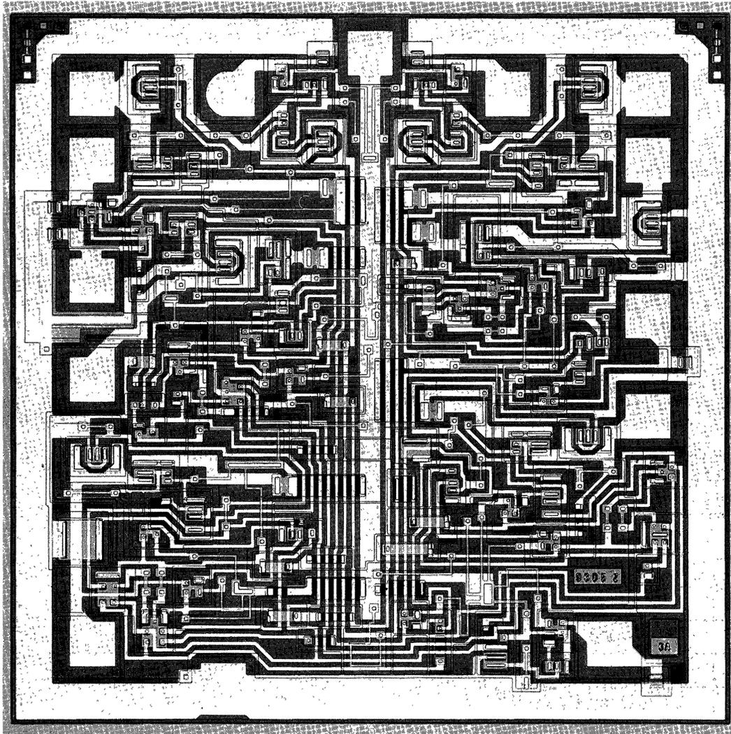
Photomicrograph of the TTL/MSI 9305 Variable Modulo Counter
