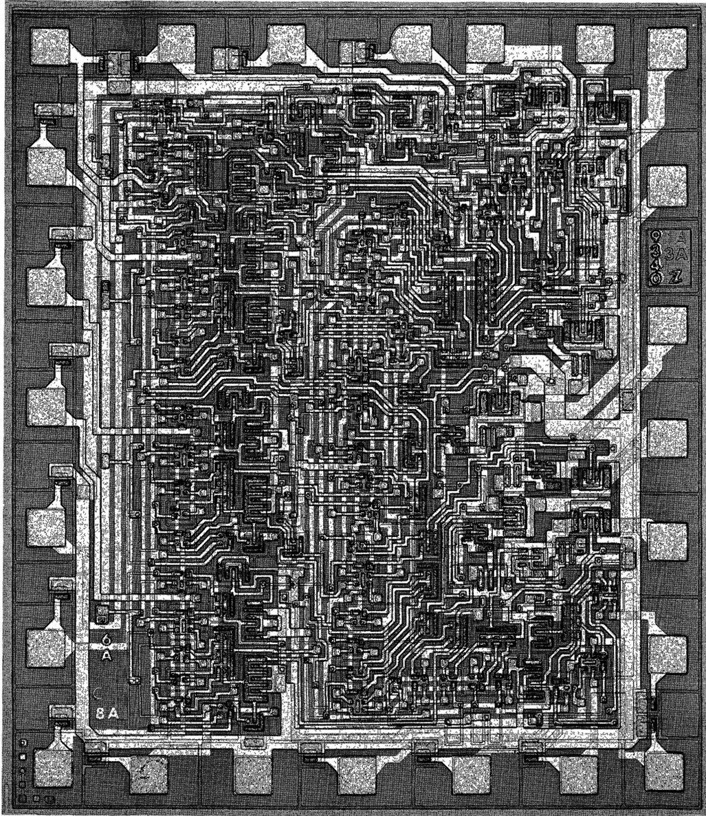
Photomicrograph of the TTL/MSI 9340 Arithmetic Logic Unit Showing Dual Layer Metal Technology
