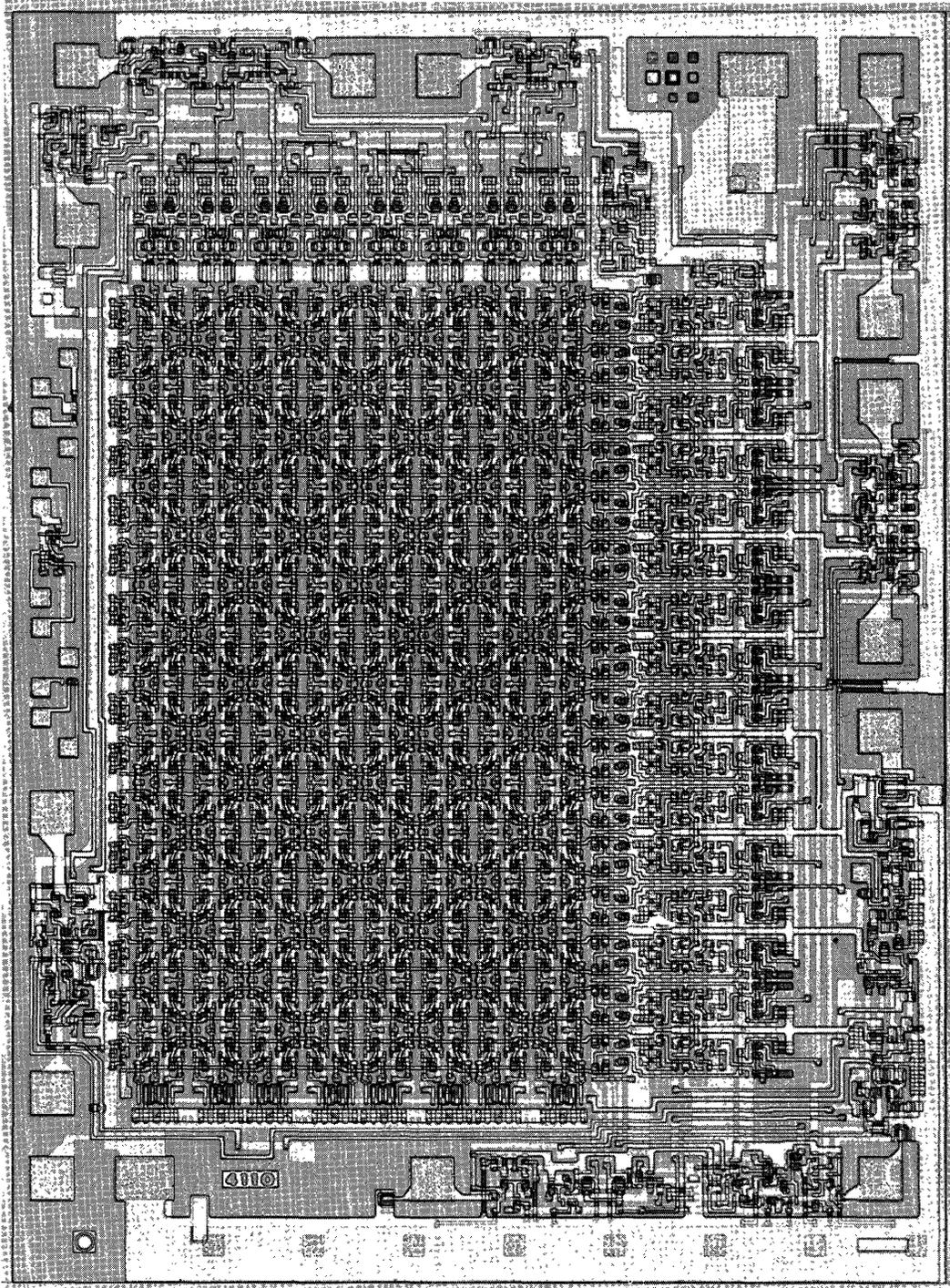
Photomicrograph of the TTL/Memory 93410 256-Bit (256 Word x 1 Bit) fully decoded RAM
