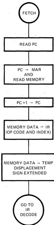
Fig. 5-17 Flow Chart for Fetch Operation
