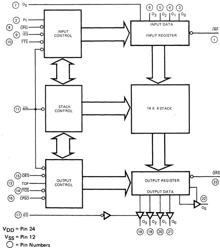
**FUNCTIONAL DESCRIPTION** - As shown in the block diagram the 4703 consists of three sections:
