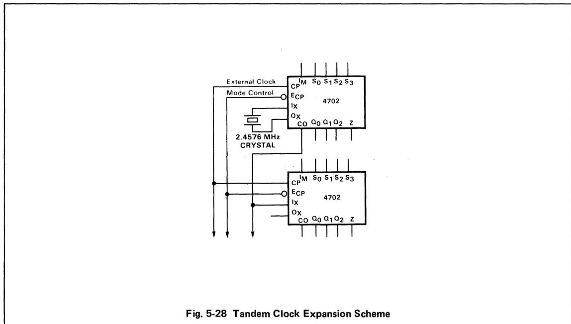
Fig. 5-28 Tandem Clock Expansion Scheme
