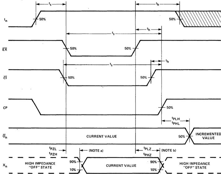
PROPAGATION DELAY  $CP$  TO  $\overline{O_n}$ , OUTPUT  $X_n$  ENABLE AND DISABLE TIMES, AND SET-UP AND HOLD TIMES,  $I_n$  TO  $\overline{EX}$ ,  $\overline{EX}$  TO  $CP$  AND  $\overline{CI}$  TO  $CP$
