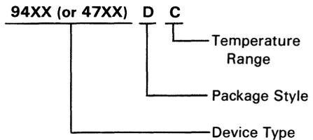
In order to accommodate varying die sizes (MSI, LSI, etc.), numbers of pins (16, 18, 24, etc.), and package outlines, a number of different package forms are required in each of the three package style categories.
