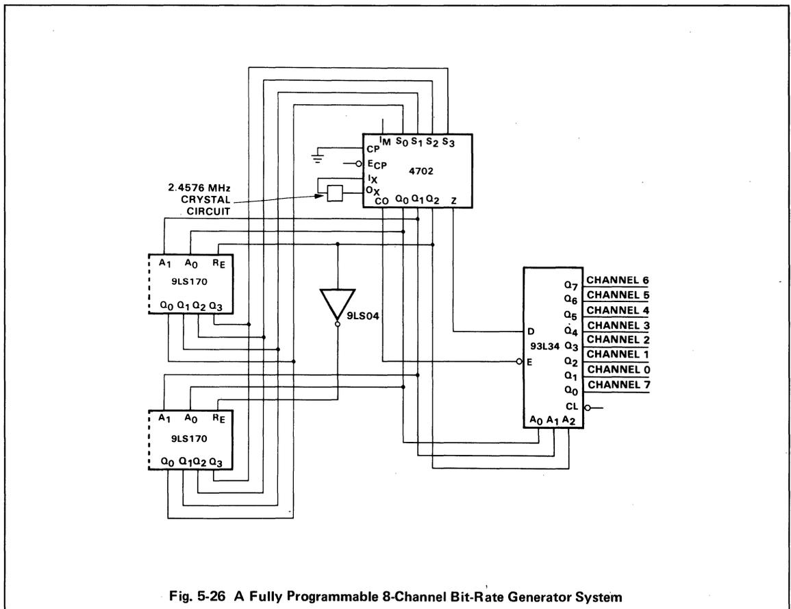
Fig. 5-26 A Fully Programmable 8-Channel Bit-Rate Generator System
