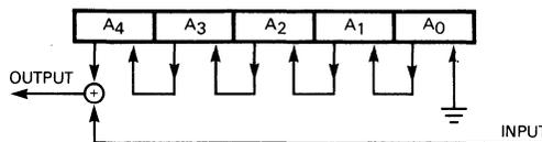
Fig. 5-21 Circuit for Multiplying by  $x^5$
