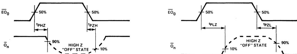
**$\overline{E_0}$  TO OUTPUT ENABLE AND DISABLE TIMES**
