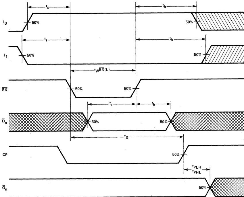
PROPAGATION DELAY, CP TO  $\bar{O}_n$ , MINIMUM EX PULSE WIDTH AND SET-UP AND HOLD TIMES,  $I_n$  TO EX, EX TO CP AND  $I_n$  TO CP
