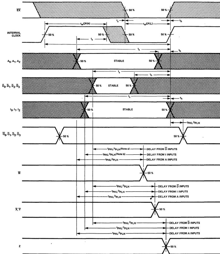
PROPAGATION DELAYS,  $A_n$  to  $Z$ ,  $I_n$  to  $Z$ ,  $\bar{D}_n$  to  $Z$ ,
