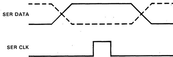
Fig. 5-8 Timing Relationship between SER DATA and SER CLK
