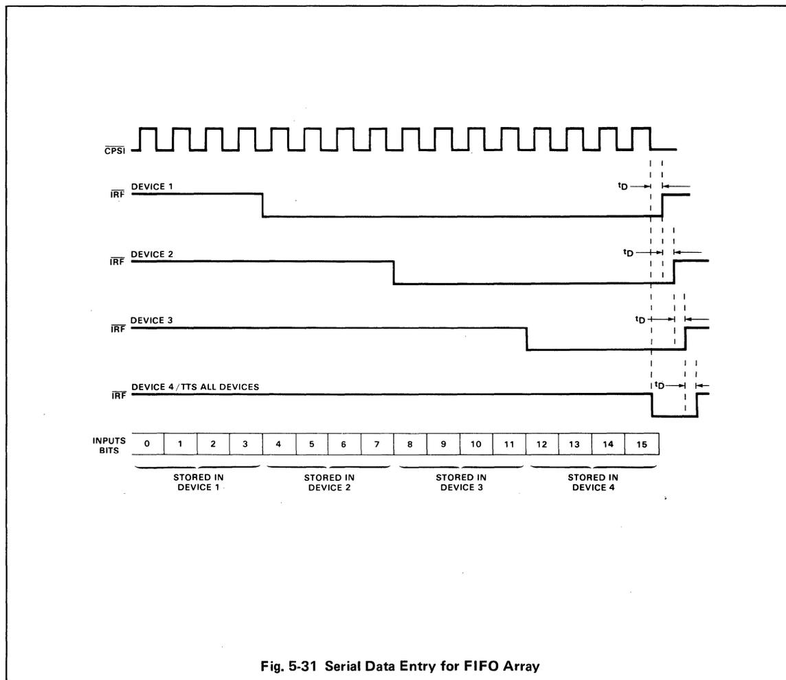
Fig. 5-31 Serial Data Entry for FIFO Array
