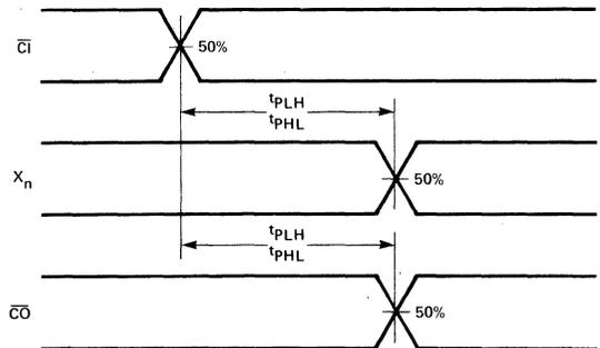
PROPAGATION DELAY,  $\overline{C}_1$  TO  $X_n$  AND  $\overline{C}_1$  TO  $\overline{C}_0$
