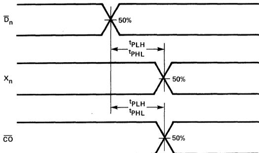
PROPAGATION DELAY,  $\overline{D}_n$  TO  $X_n$  AND  $\overline{D}_n$  TO  $\overline{C}_0$
