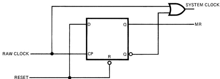
Fig. 5-3 Initialization Circuit
