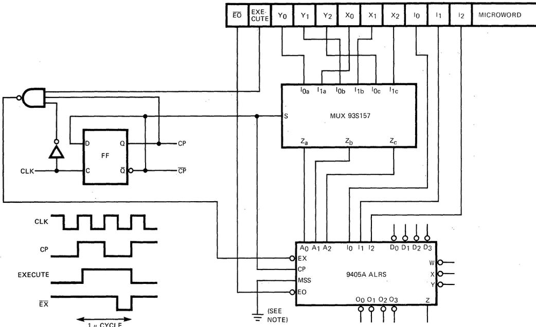
NOTE: MSS is connected to  $V_{CC}$  for most significant slice, otherwise grounded.
