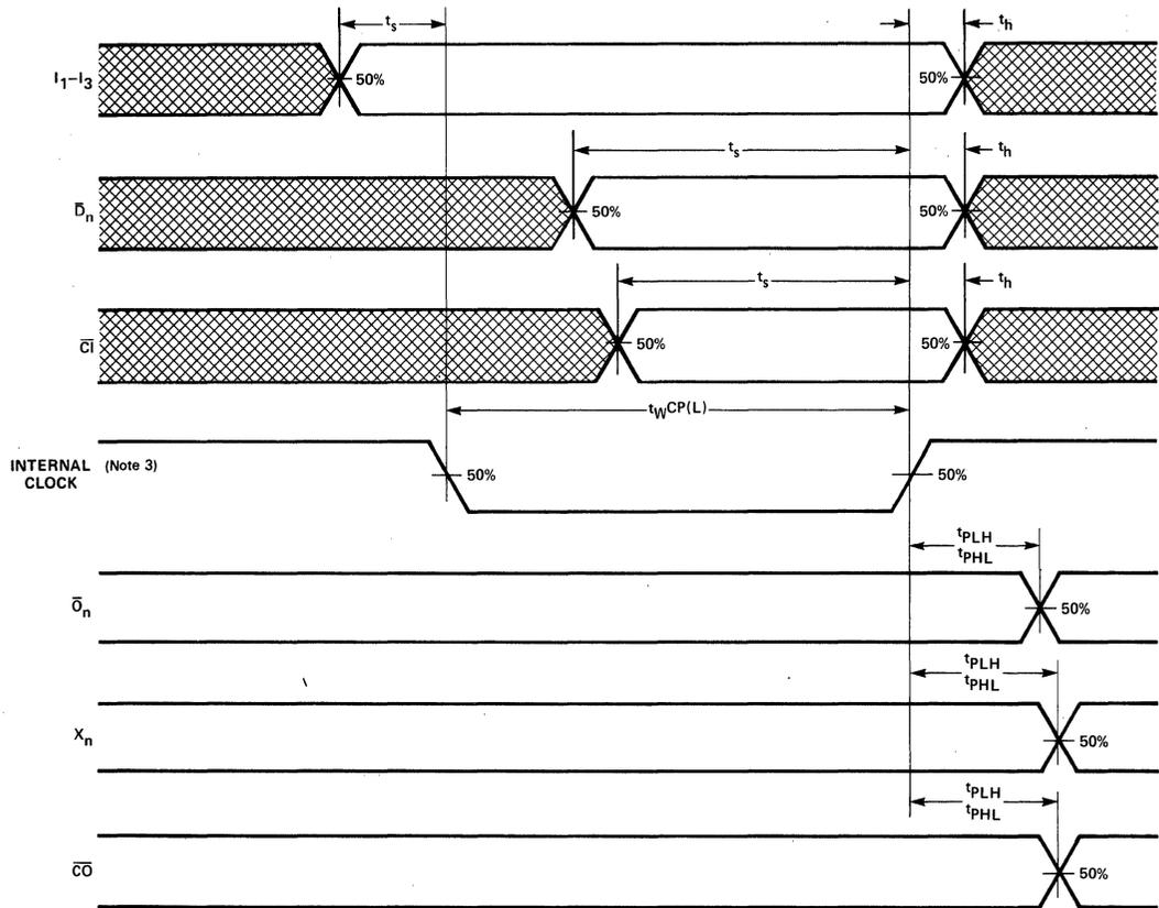
PROPAGATION DELAYS, INTERNAL CLOCK TO  $\bar{O}_n$ ,
