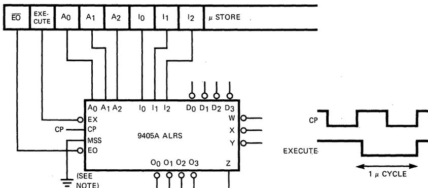
NOTE: MSS IS CONNECTED TO  $V_{CC}$  FOR MOST SIGNIFICANT SLICE, OTHERWISE GROUNDED.
