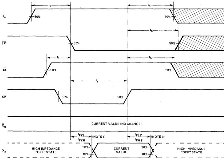
OUTPUT  $X_n$  DISABLE DELAY, OUTPUT  $X_n$  ENABLE DELAY, AND SET-UP AND HOLD TIMES,  $I_n$  TO  $\bar{E}\bar{X}$ ,  $I_n$  TO CP,  $\bar{E}\bar{X}$  TO CP, AND  $\bar{C}\bar{I}$  TO  $\bar{E}\bar{X}$ .
