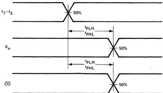
PROPAGATION DELAY,  $I_1-I_3$  TO  $\overline{C}_0$  AND  $I_1-I_3$  TO  $X_n$
