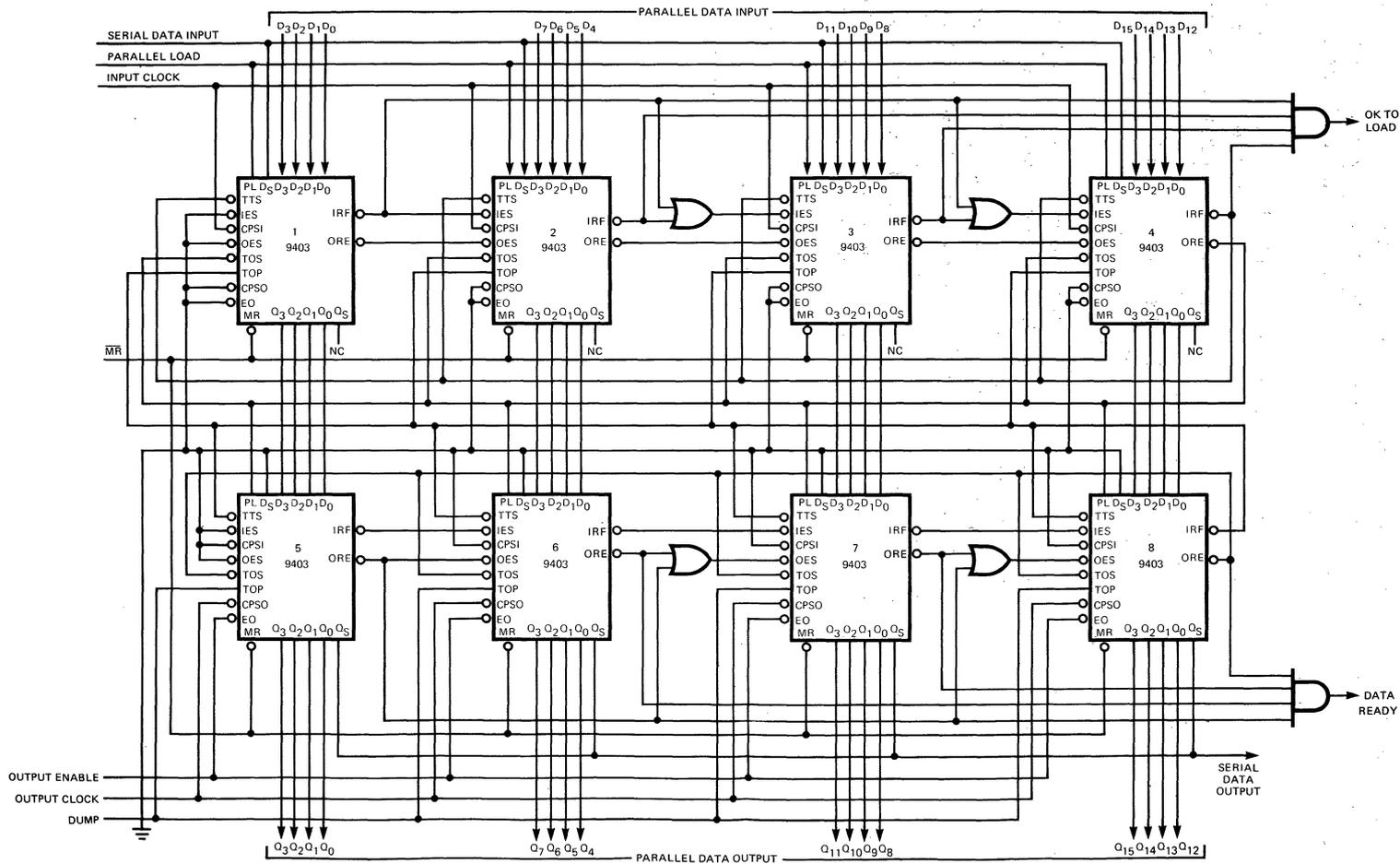
Fig. 5-34 Expansion with Priority Defeated for Faster Operation
