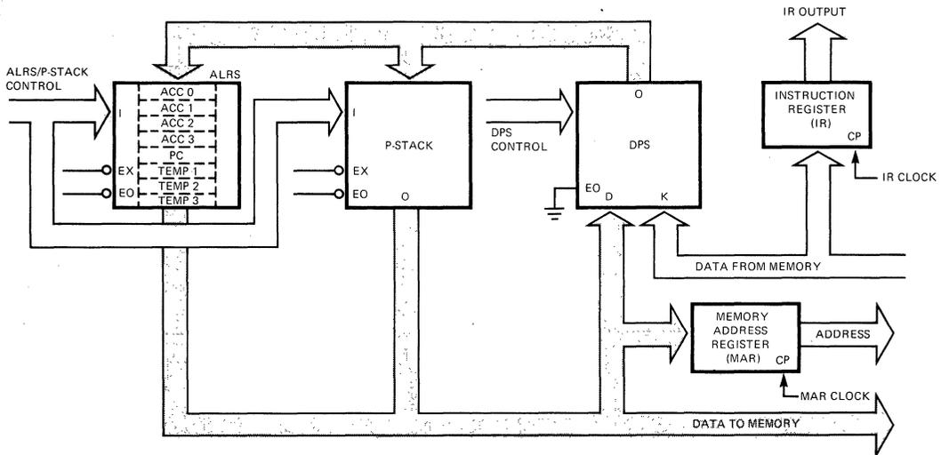
**Fig. 5-15 Data Path for the Processor**
