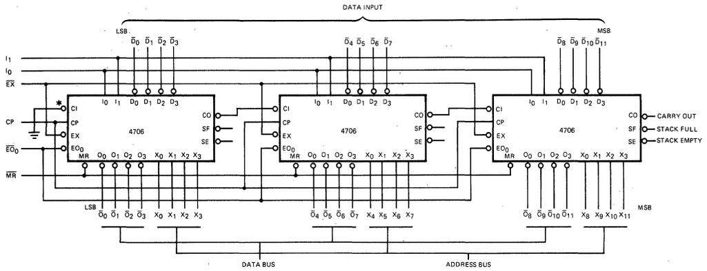
\*Tie to V<sub>DD</sub> to disable automatic increment.
