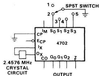
Fig. 5-25 Switch Selectable Bit-Rate Generator Configuration Providing 5 Bit Rates
