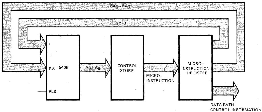
Fig. 5-2 Pipeline System
