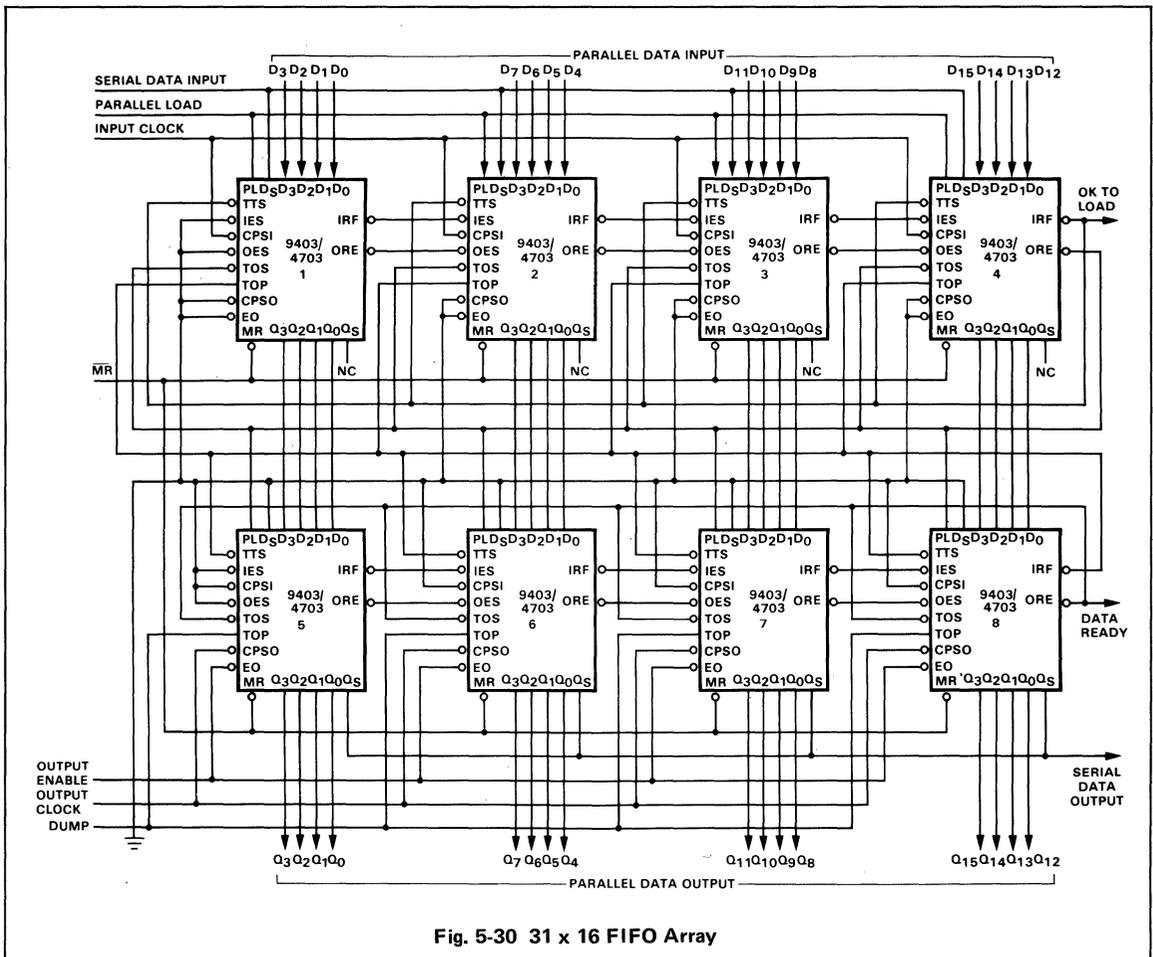
Fig. 5-30 31 x 16 FIFO Array
