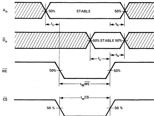
MINIMUM  $\overline{CS}$  PULSE WIDTH, MINIMUM WRITE ENABLE PULSE WIDTH, SET-UP AND HOLD TIMES ADDRESS TO  $\overline{WE}$ , DATA TO  $\overline{WE}$ , AND  $\overline{CS}$  TO  $\overline{WE}$
