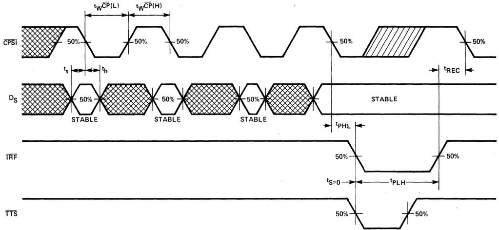
MINIMUM  $\overline{\text{CPSI}}$  PULSE WIDTH, PROPAGATION DELAY,  $\overline{\text{CPSI}}$  TO  $\overline{\text{IRF}}$  AND  $\overline{\text{TTS}}$  TO  $\overline{\text{IRF}}$ , RECOVERY TIME,  $\overline{\text{IRF}}$  TO  $\overline{\text{CPSI}}$ , AND SET-UP AND HOLD TIMES,  $\text{D}_S$  TO  $\overline{\text{CPSI}}$ , AND  $\text{TTS}$  TO  $\overline{\text{IRF}}$ .
