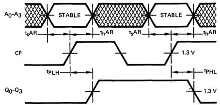
Other Conditions:  $\overline{\text{CS}} = \overline{\text{OE}} = \text{LOW}$
