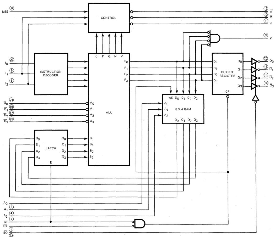
**FUNCTIONAL DESCRIPTION** — As shown in the block diagram, the 9405A consists of a 4-bit ALU, 8-word by 4-bit RAM with latches, an Instruction Decoder, control logic and a 4-bit Output Register.
