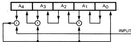
Fig. 5-23 Basic Cyclic Check Circuit for  $P(x) = x^5 + x^4 + x^2 + 1$
