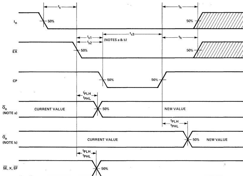
**PROPAGATION DELAY, CP TO  $\bar{O}_n$ ,  $\bar{E}\bar{X}$  TO  $\bar{O}_n$ ,  $\bar{E}\bar{X}$  TO  $\bar{S}\bar{E}$  OR  $\bar{S}\bar{F}$ ,
