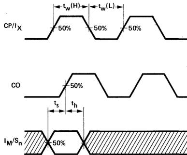
**MINIMUM CP AND  $I_X$  PULSE WIDTHS AND SET-UP AND HOLD TIMES,
