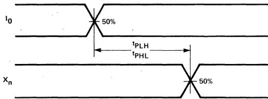
PROPAGATION DELAY,  $I_0$  TO  $X_n$
