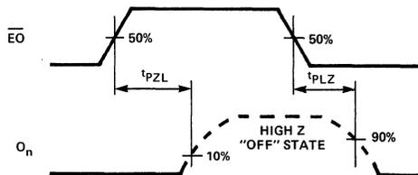
OUTPUT ENABLE TIME (t<sub>pZL</sub>) AND OUTPUT DISABLE TIME (t<sub>pLZ</sub>)
