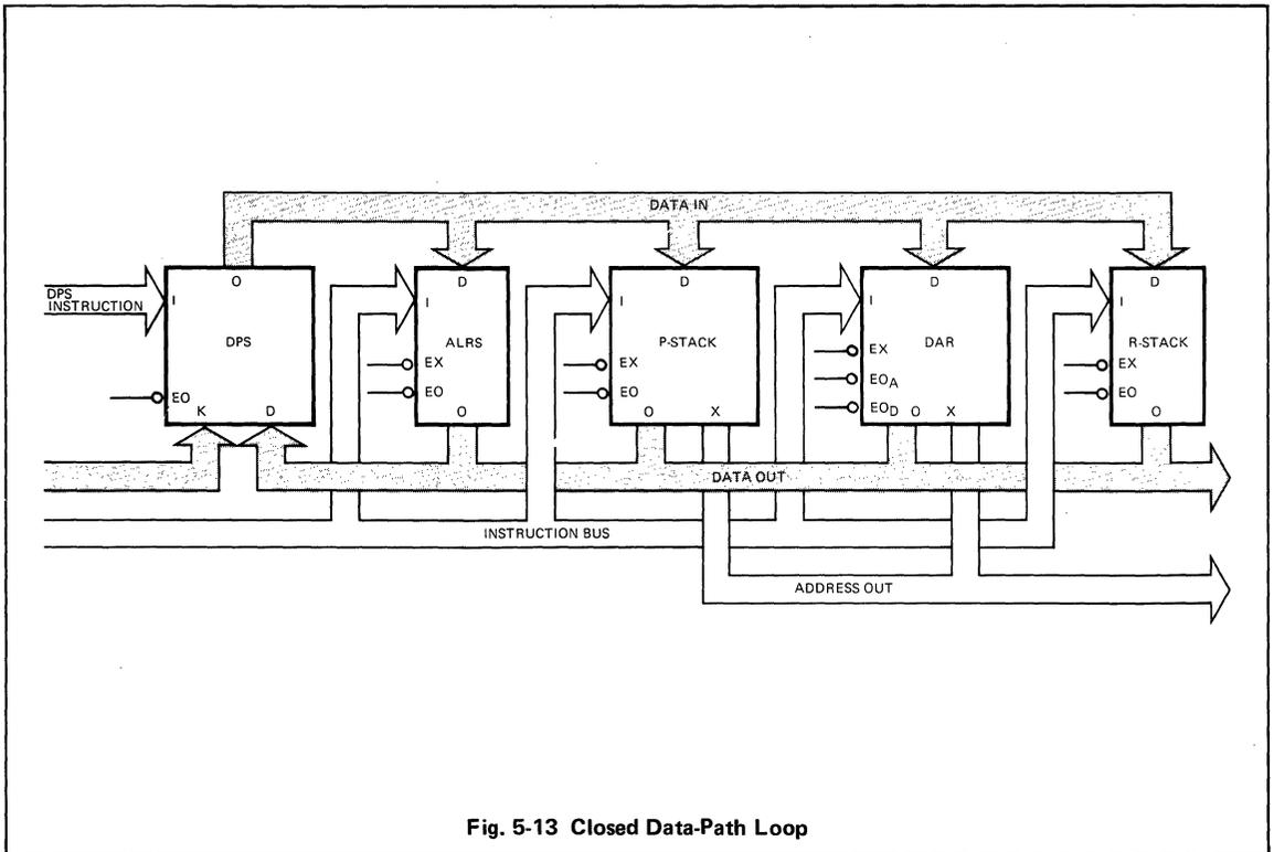
Fig. 5-13 Closed Data-Path Loop
