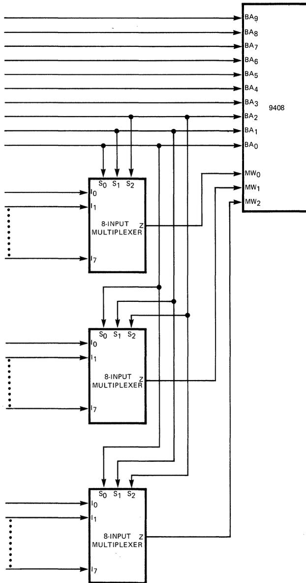
Fig. 5-6 Expanding Multiway Inputs
