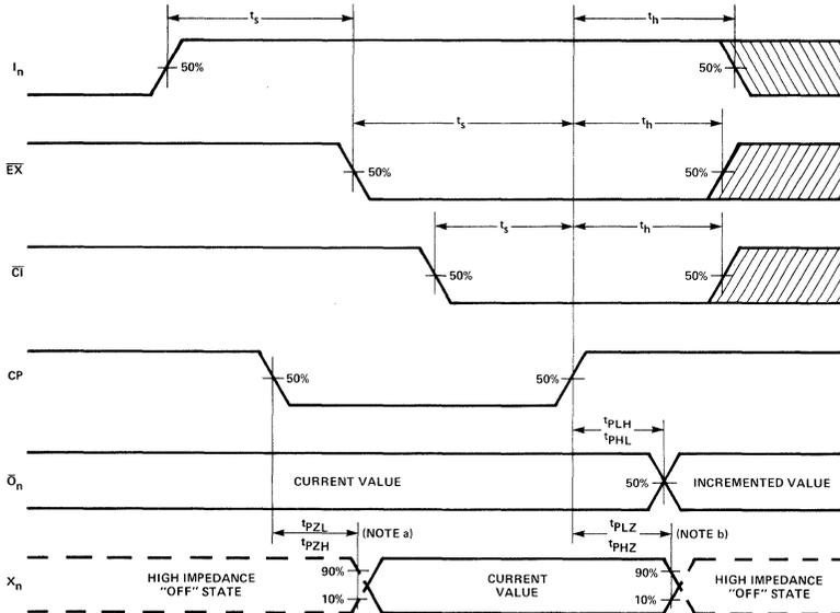
PROPAGATION DELAY,  $CP$  TO  $\overline{O}_n$ , OUTPUT  $X_n$  ENABLE AND DISABLE TIMES AND SET-UP AND HOLD TIMES,  $I_n$  TO  $\overline{EX}$ ,  $\overline{EX}$  TO  $CP$ , AND  $C_i$  TO  $CP$
