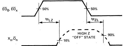
OUTPUT ENABLE TIME ( $t_{pLZ}$ ) AND OUTPUT DISABLE TIME ( $t_{pZL}$ )
