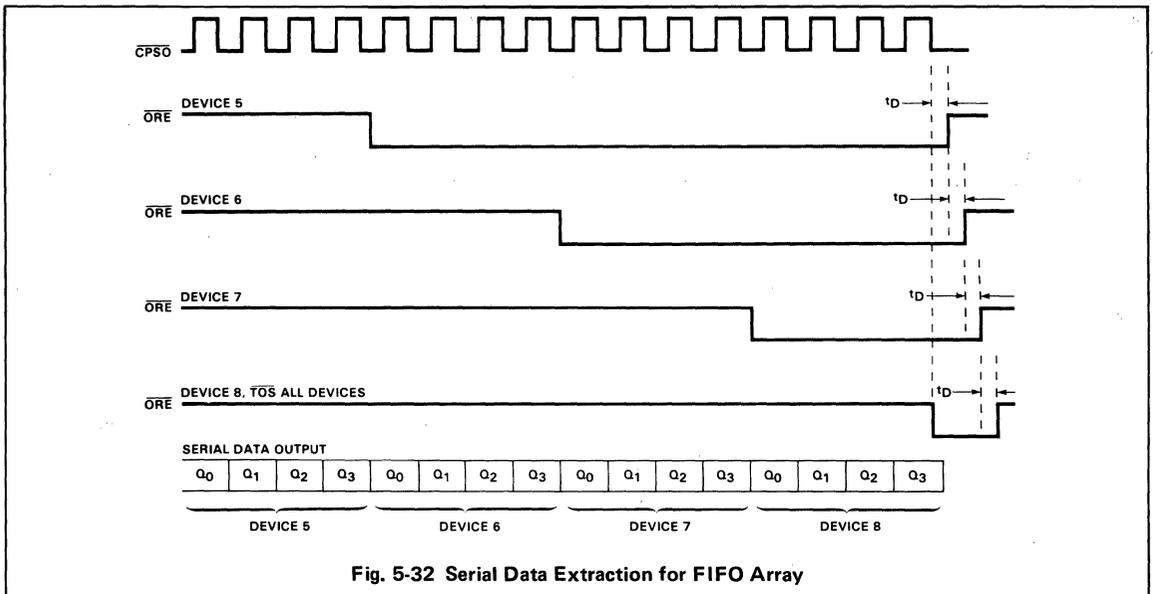
Fig. 5-32 Serial Data Extraction for FIFO Array
