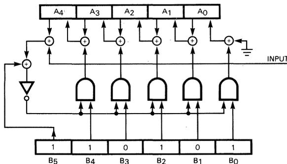
Fig. 5-22 Conceptual Cyclic Check Generator
