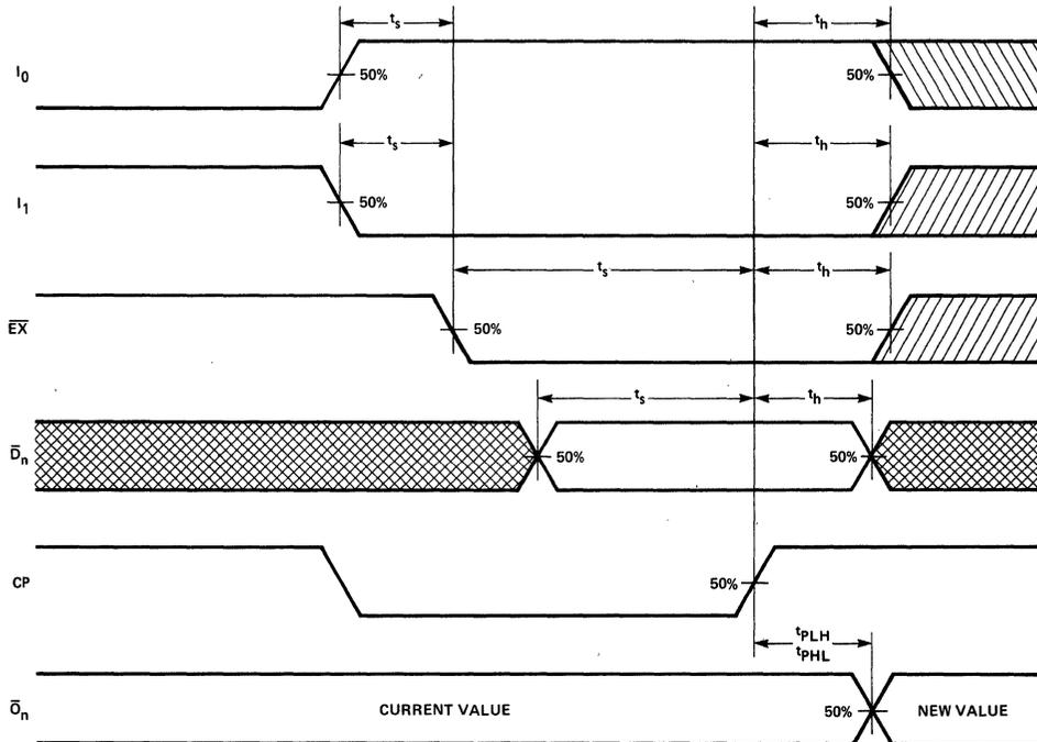
PROPAGATION DELAY CP TO  $\bar{O}_n$  AND SET-UP AND HOLD TIMES,  $I_n$  TO  $\bar{E}\bar{X}$ ,  $\bar{D}_n$  TO CP AND  $I_n$  TO CP
