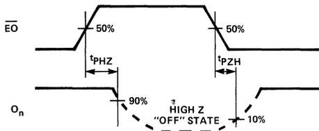
OUTPUT ENABLE TIME (t<sub>pZH</sub>) AND OUTPUT DISABLE TIME (t<sub>pHZ</sub>)
