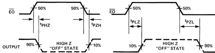
$\overline{E_0}$  TO OUTPUT ENABLE AND DISABLE TIMES
