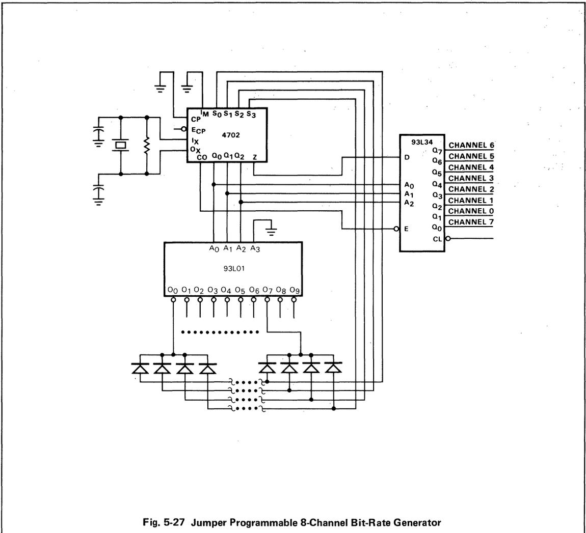
Fig. 5-27 Jumper Programmable 8-Channel Bit-Rate Generator
