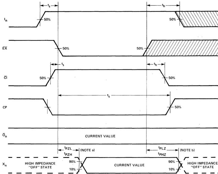
OUTPUT  $X_n$  ENABLE AND DISABLE TIMES AND SET-UP AND HOLD TIMES,  $I_n$  TO  $\overline{EX}$ ,  $C_i$  TO  $\overline{EX}$  AND  $\overline{EX}$  TO  $CP$ .
