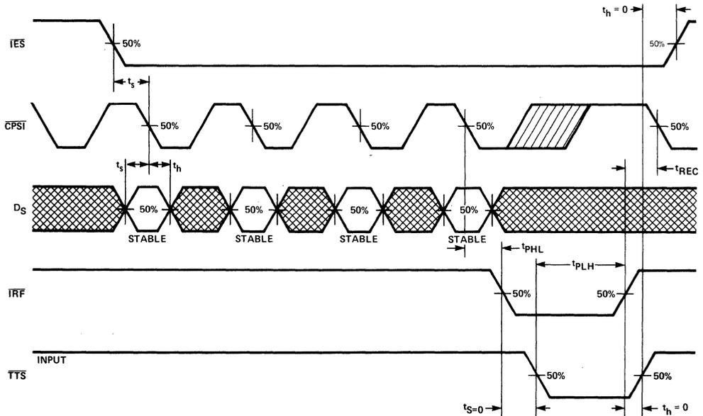
PROPAGATION DELAY,  $\overline{\text{CPSI}}$  TO  $\overline{\text{IRF}}$  AND  $\overline{\text{TTS}}$  TO  $\overline{\text{IRF}}$ , RECOVERY TIME,  $\overline{\text{IRF}}$  TO  $\overline{\text{CPSI}}$  AND SET-UP AND HOLD TIMES,  $\overline{\text{IES}}$  TO  $\overline{\text{CPSI}}$ ,  $\text{D}_S$  TO  $\overline{\text{CPSI}}$  AND  $\text{TTS}$  TO  $\overline{\text{IRF}}$ .
