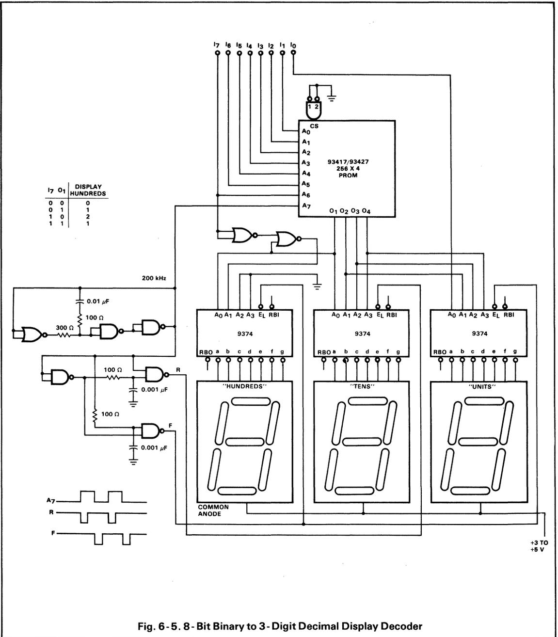
Fig. 6-5. 8-Bit Binary to 3-Digit Decimal Display Decoder
