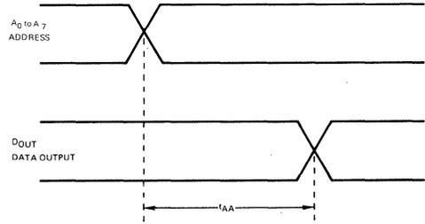
(ALL TIME MEASUREMENTS REFERENCED TO 1.5 V)
