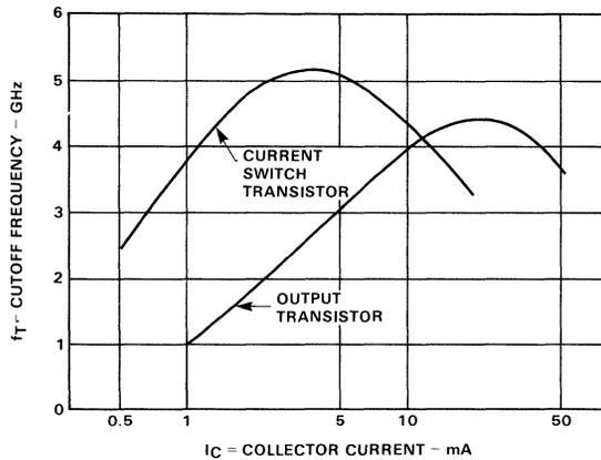
Fig. 4-3. Cutoff Frequency of Isoplanar II Transistors
