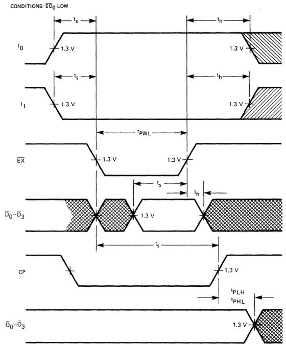
AC CHARACTERISTICS AND SET-UP REQUIREMENTS - CALL (PUSH) OPERATION:
