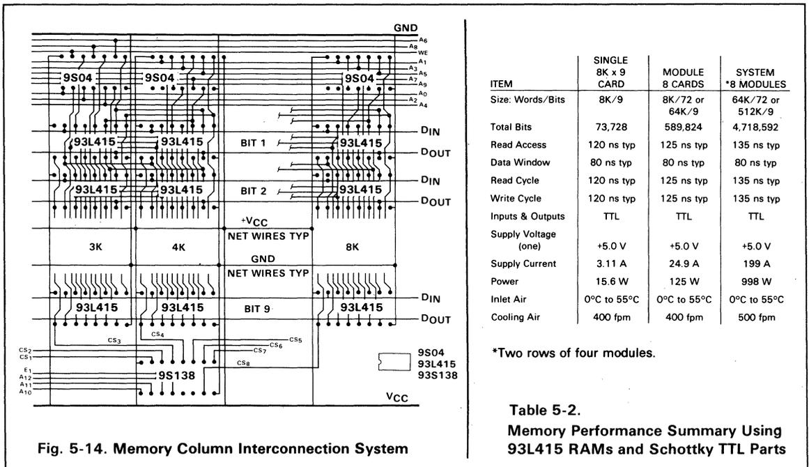
Fig. 5-14. Memory Column Interconnection System
