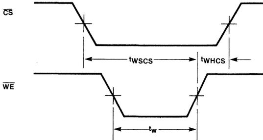
WRITE ENABLE SET-UP AND HOLD TIMES,  $\overline{CS}$  PULSE WIDTH<sup>2</sup>
