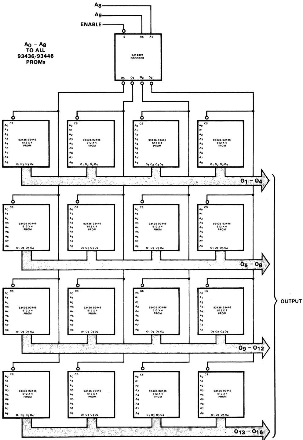
Fig. 6-13. Combined Word and Address Expansion, 2048 x 16-Bit Array Using 512 x 4-Bit PROMs
