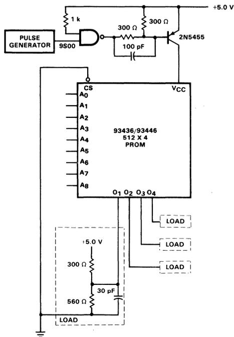
Fig. 6-16. Power Switching Circuit
