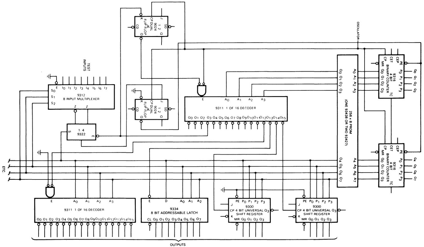
Fig. 6-9. Programmed Logic Controller, Conditional Jump
