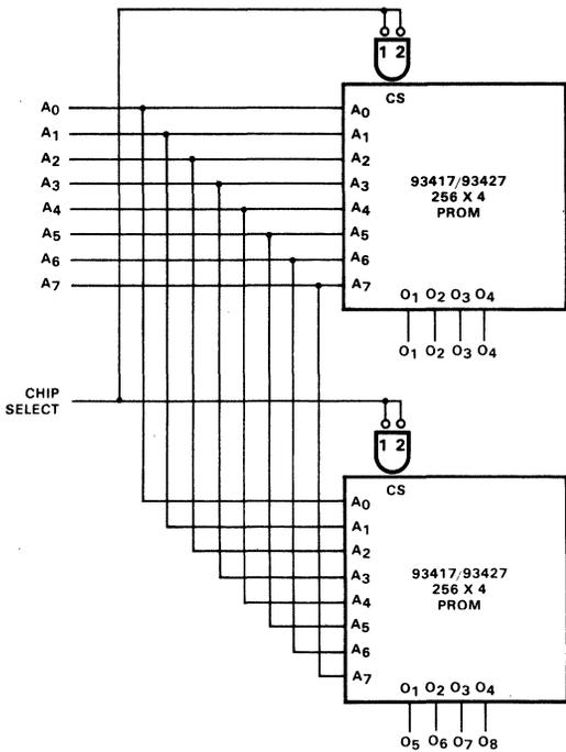
Fig. 6-10. Word-Size Expansion, 256 x 8-Bit Array
