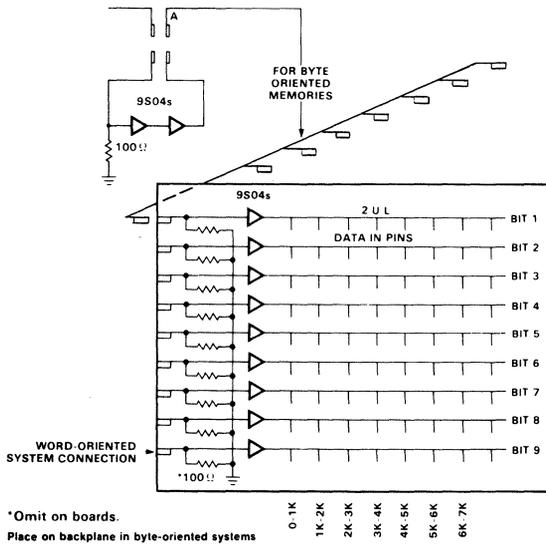
Fig. 5-11. Data Input System
