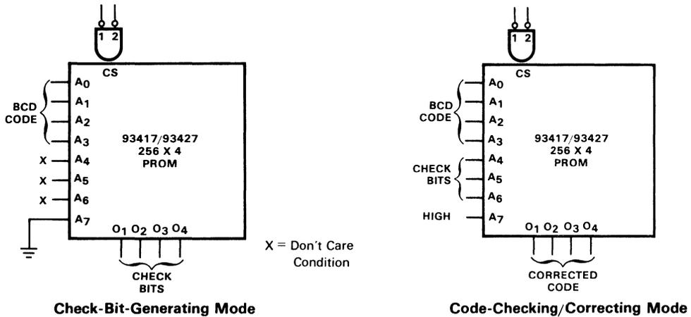
Fig. 6-3. Hamming Code Generator and Checker/Corrector
