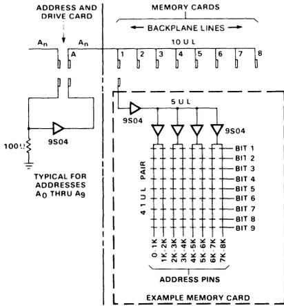
Fig. 5-8. Address Selection for Bits Within a 1024 RAM
