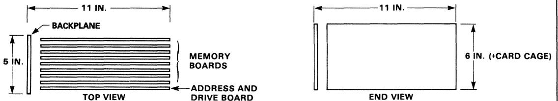
**Fig. 5-7. Physical Layout for a Bipolar Memory Module**
