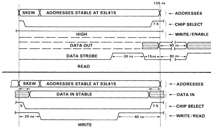
Fig. 5-15. Timing Example for 93L415 Memory
