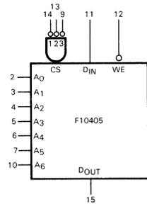
$V_{CC}$  = GND (Pins 1 and 16)
