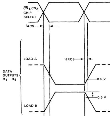
PROPAGATION DELAY FROM OUTPUT ENABLE
