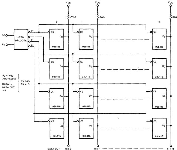
Addressing for a 4096-bit memory plane by 16 bits (4K x 16) requires only half of a 9321 1-of-4 decoder and any necessary buffers.
