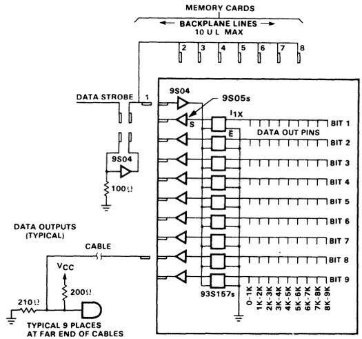
Fig. 5-12. Data Output System
