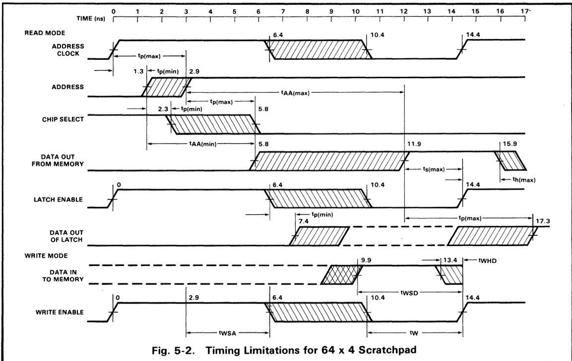
Fig. 5-2. Timing Limitations for 64 x 4 Scratchpad
