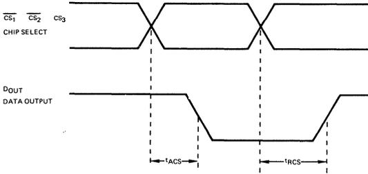
PROPAGATION DELAY FROM ADDRESS
