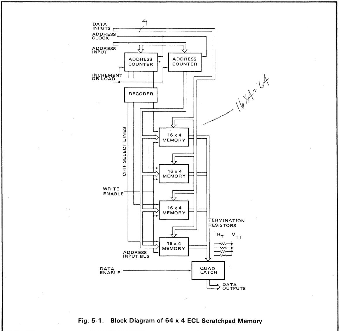
Fig. 5-1. Block Diagram of 64 x 4 ECL Scratchpad Memory
