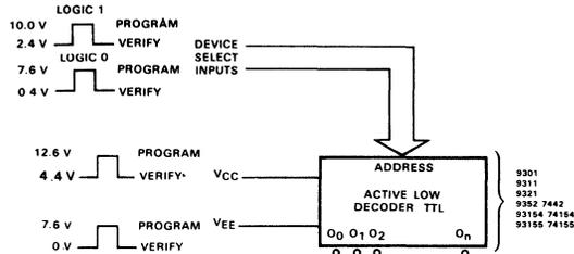
NOTE: All voltage and logic levels must be raised and lowered simultaneously.
