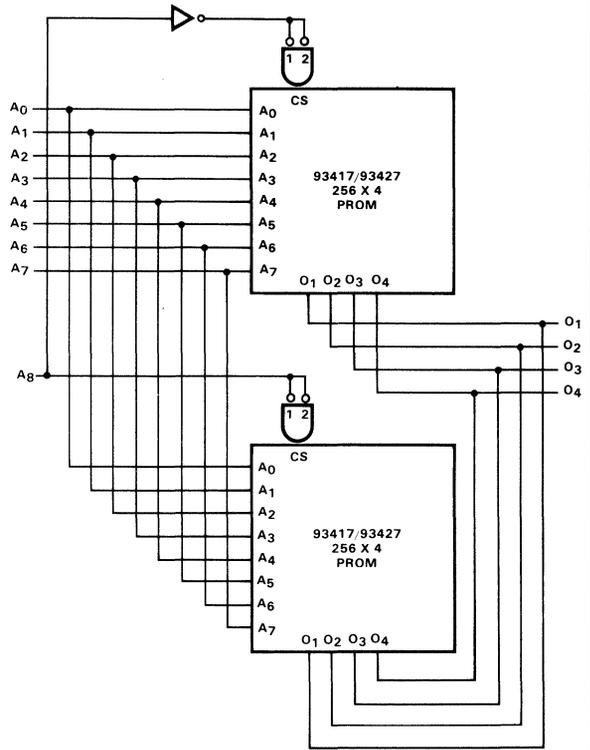
Fig. 6-11. Address Expansion, 512 x 4-Bit Array
