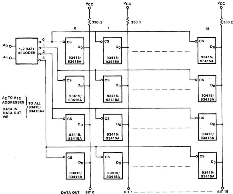
Addressing for a 4096-bit memory plane by 16 bits (4K by 16) requires only half of a 9321 1-of-4 decoder and any necessary buffers.
