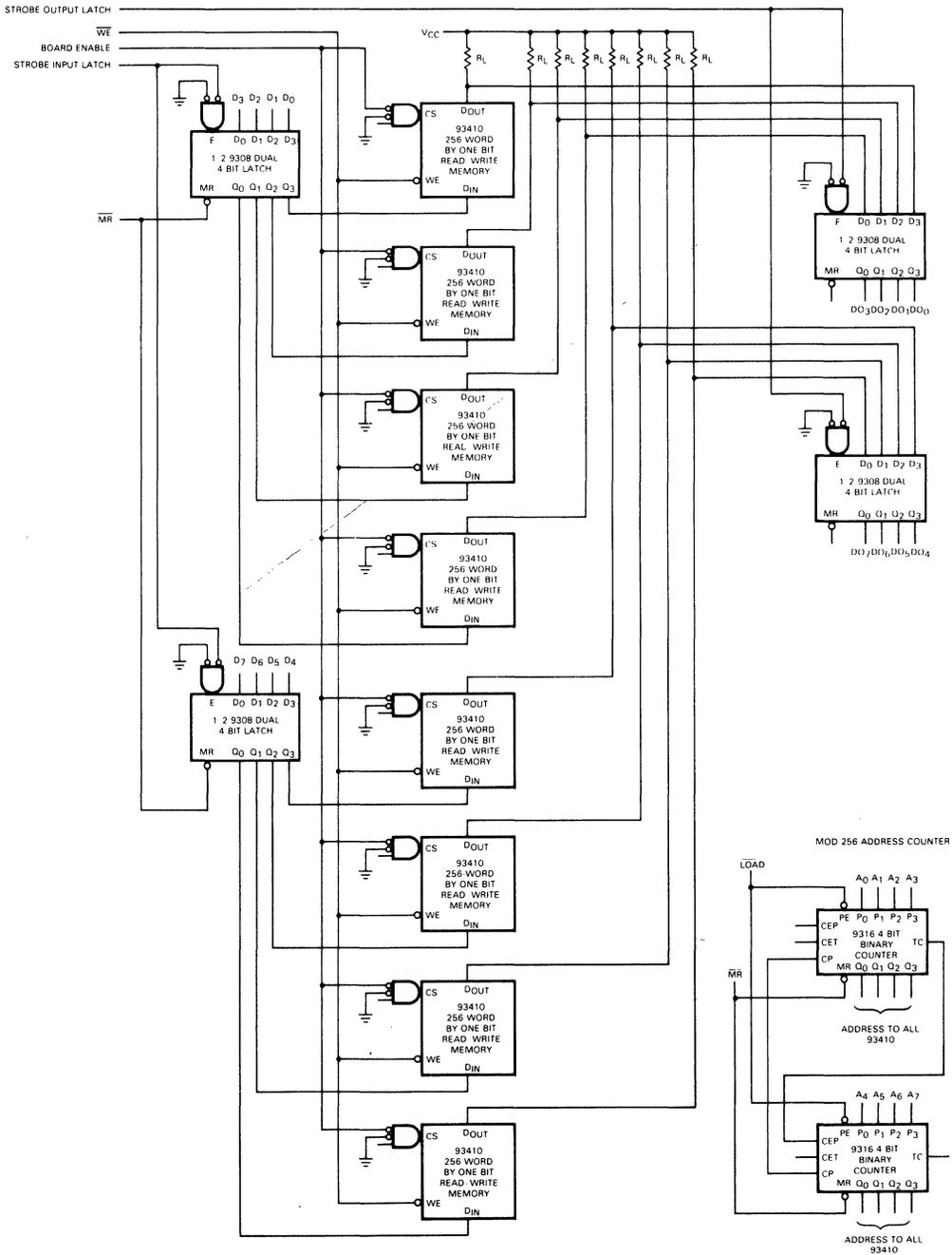
Fig. 5-4. 256 Word by 8-Bit Buffer Memory System
