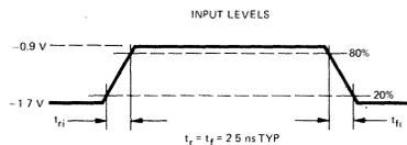
All Timing Measurements Referenced to 50% of Input Levels
