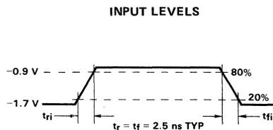
All Timing Measurements Referenced to 50% of Input Levels
