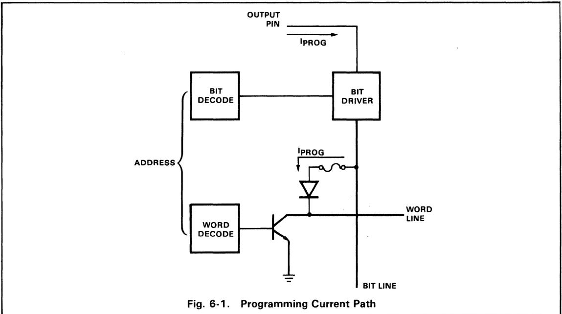
Fig. 6-1. Programming Current Path
