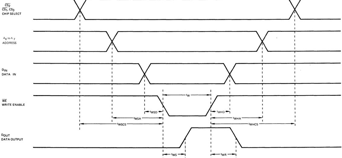
(ALL TIME MEASUREMENTS REFERENCED TO 1.5 V)
