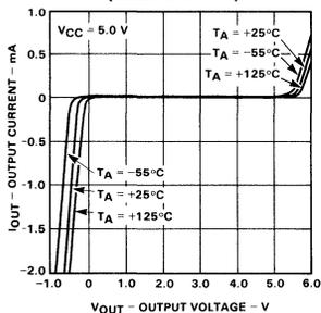
**OUTPUT CURRENT VERSUS OUTPUT VOLTAGE (OUTPUT HIGH Z STATE) (93L471 ONLY)**
