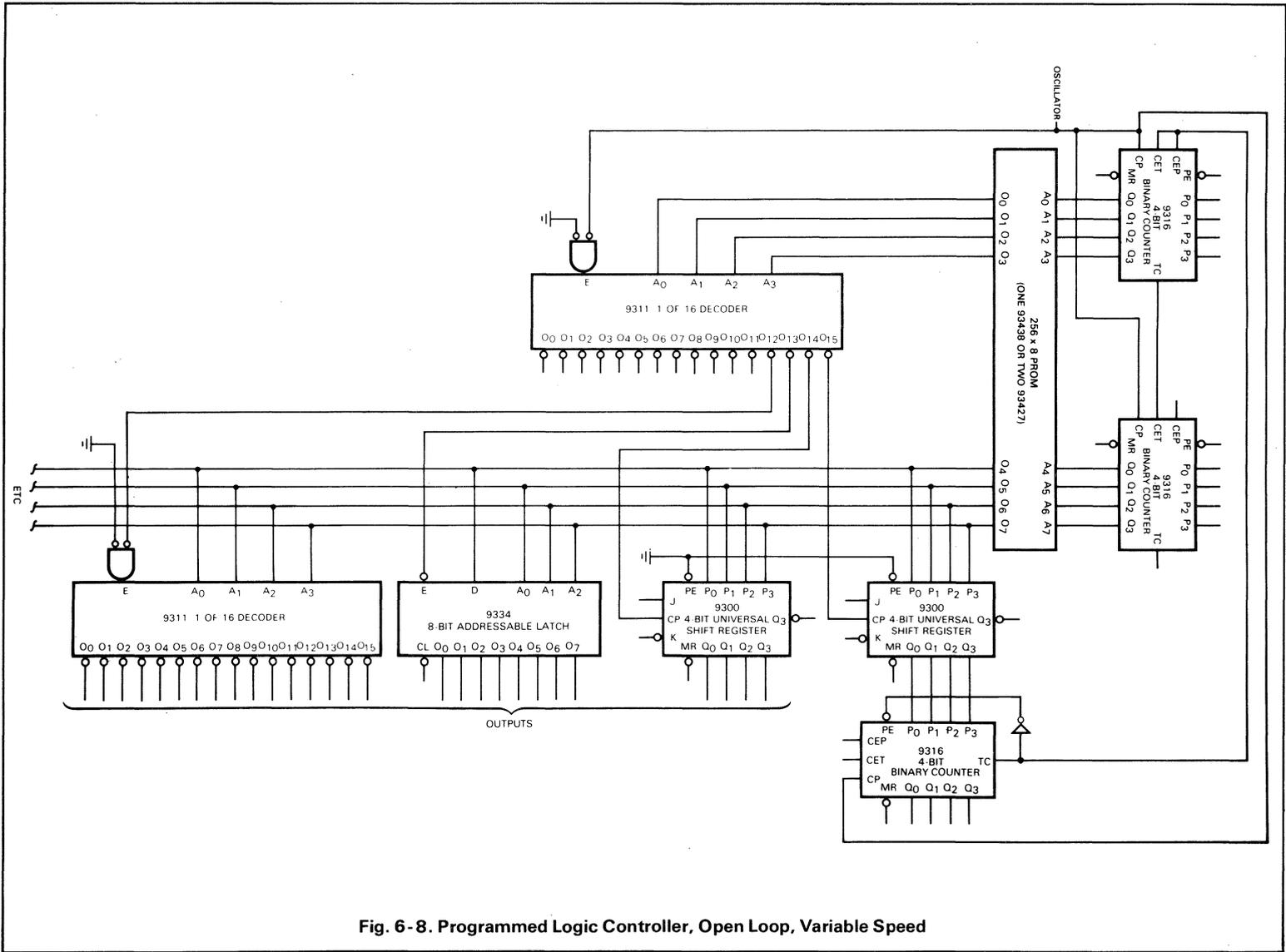
Fig. 6-8. Programmed Logic Controller, Open Loop, Variable Speed
