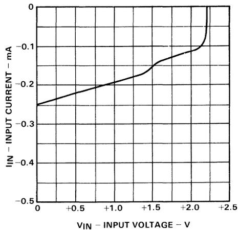
Fig. 4-8. Translator Input Characteristic Showing Threshold Break
