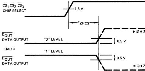
WRITE ENABLE TO HIGH Z DELAY
