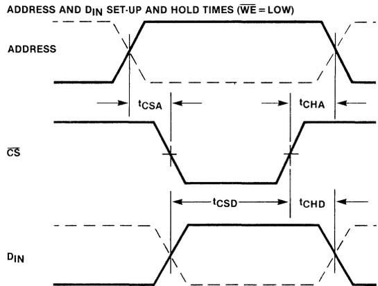
CHIP SELECT SET-UP AND HOLD TIMES
