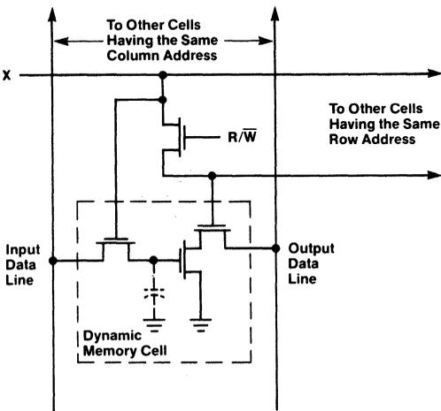
The 4K-bit DRAM generation and the following density levels (16K, 64K, etc.), incorporate the smaller one-transistor-cell design consisting of a capacitor and an access transistor (Figure 12). Because the one-transistor cell is much smaller than its predecessors, the amount of stored signal available for detection is also less. The one-transistor cell requires a more complex *balanced* sense amplifier, but the inherent density advantages make this cell viable.
