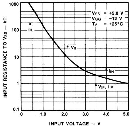
**DC Characteristics**  $V_{SS} = +5\text{ V} \pm 5\%$ ,  $V_{GG} = -12\text{ V} \pm 5\%$ ,  $V_{DD} = 0\text{ V}$ ,  $T_A = 0^\circ\text{C}$  to  $+70^\circ\text{C}$
