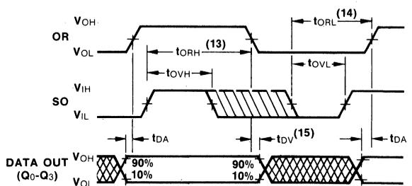
Both SO and OR must be HIGH for  $t_{OVH}$ . Similarly both SO and OR must be LOW for  $t_{OVL}$ . Data will remain stable for  $t_{DV}$  after both SO and OR are LOW.
