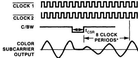
\*Maximum subcarrier amplitude attained within 8 color clock periods following rising edge of C/BW.
