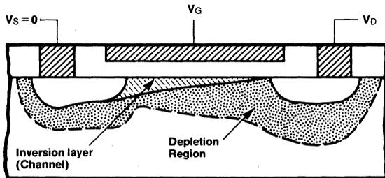
When operated in the linear region, below  $V_{D(SAT)}$ , the MOSFET looks very much like a voltage-controlled resistor. MOSFET gain is typically measured by its transconductance, the rate of change of drain current with respect to gate voltage. The transconductance in the saturation region is given by
