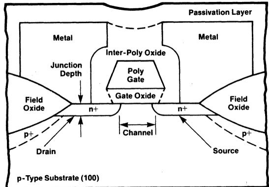
the mobility of carriers (electrons) is roughly two times that of holes, NMOS devices typically exhibit higher speed performance.
