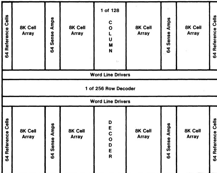
has overcome this problem in the F4164 sense amp by sharing one full-size dummy capacitor between the two halves of each bit line; thus, half the charge is supplied to each to establish the reference voltage. If the memory-cell capacitor has a HIGH charge, connecting it to a half bit line will cause that half to be more positive than the reference. If the cell has a LOW charge, the opposite occurs. This difference is sensed and latched by the sense amp.
