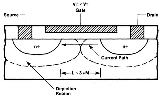
Since vertical dimensions like oxide thickness also shrink during scaling, storage capacitance per unit area for future devices will remain roughly the same as for present-day NMOS. However, since the power supply voltage must be scaled to maintain a constant electric field, the charge written into a dynamic memory cell will be reduced since it is a product of the cell capacitance and writing voltage.
