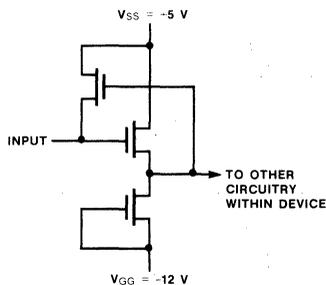
More specifically, the input current increases significantly when  $V_{IN}$  starts to exceed  $V_{II}$  (the pull-up initiation voltage). This current reaches a peak value of  $I_{IP}$  (the input barrier current) when  $V_{IN} = V_{IP}$  (the peak input current voltage point) after which it decreases as  $V_{IN}$  rises to its  $V_{IH}$  value.
