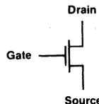
Thus when the channel first begins to form,  $V_T = V_G - V_S$ . As  $V_D$  continues to increase positively, the current increases linearly to a saturated condition (Figure 9), where further increases in  $V_D$  do not produce appreciable changes in drain current  $I_D$ . At this point,
