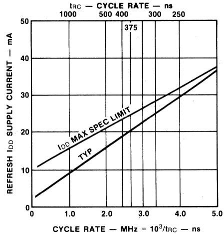
**Normal Operation  $I_{DD}$  vs Cycle Rate**
