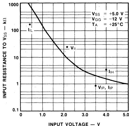
**DC Requirements**  $V_{SS} = 5.0\text{ V} \pm 5\%$ ,  $V_{DD} = 0\text{ V}$ ,  $V_{GG} = -12\text{ V} \pm 5\%$ ,  $T_A = 0^\circ\text{C}$  to  $70^\circ\text{C}$
