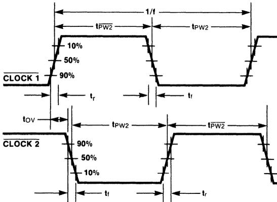
**c) Color Subcarrier Timing and Reset Detail**
