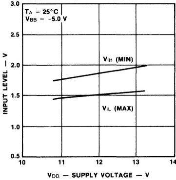
Clock Input Level vs  $V_{DD}$
