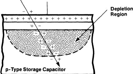
As device dimensions are further reduced, the amount of charge stored in each cell is decreased. Thus, the difference in the number of electrons sensed as a '1' and the number representing a '0' is also smaller. Therefore, since the number of electron-hole pairs produced within the silicon by an incident alpha particle is roughly constant, the probability of an error caused by this extra charge increases as device geometries and stored charge are scaled.
