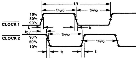
**c) Color Subcarrier Timing and Reset Detail**
