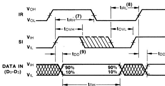
Input data must remain stable during timing window  $t_{DH}$ . Both SI and IR must be HIGH for  $t_{OVH}$ . Similarly, both SI and IR must be LOW for  $t_{OVL}$ .
