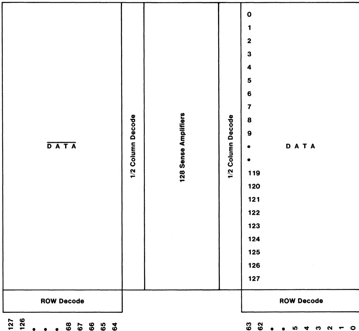
Actual column and row position addresses converted to decimal. Conversion to the external address is explained in the text.
