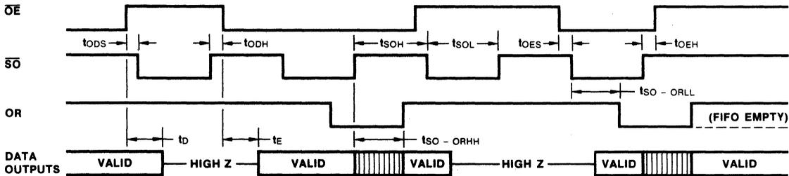
Fig. 3 Bubble-through Timing
