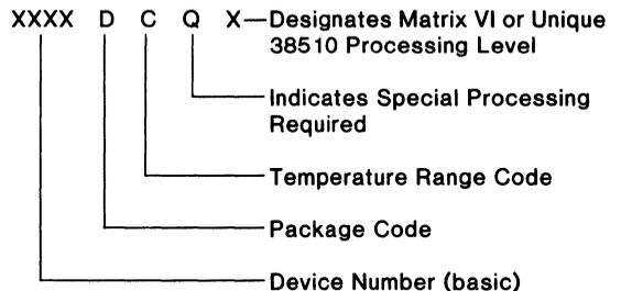
**Package Code**—One letter represents the basic package type. Different package outlines exist within each package type to accommodate varying die sizes and number of pins, as indicated below:
