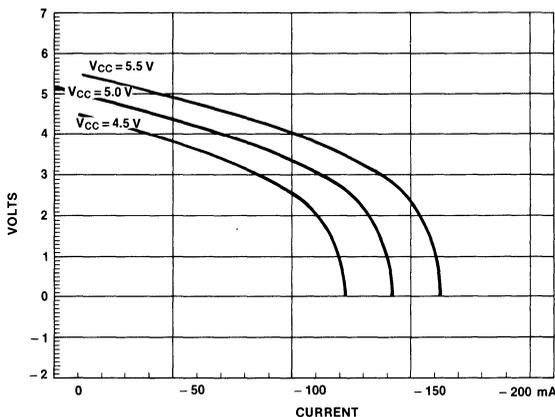
Figure 3-2 Output Characteristics ( $V_{OH}$ ,  $I_{OH}$ )
