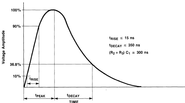
Figure 2-12 ESD Pulse Waveform
