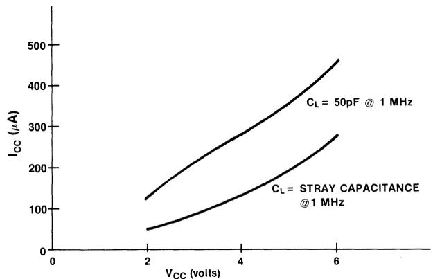
Figure 2-1  $I_{CC}$  vs  $V_{CC}$
