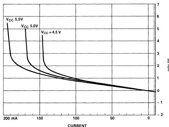
Figure 3-3 Output Characteristics ( $V_{OL}$ ,  $I_{OL}$ )
