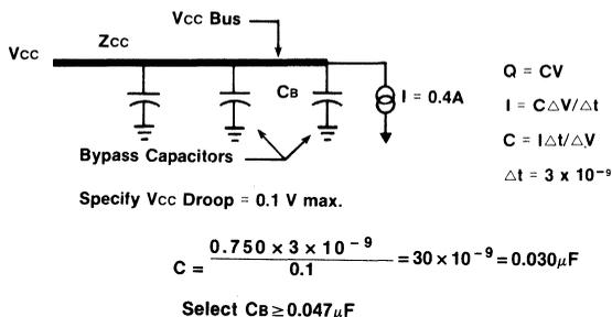
Good practice is to place one decoupling capacitor adjacent to each package driving any transmission line and distribute other capacitors evenly throughout the logic, one capacitor per three packages.
