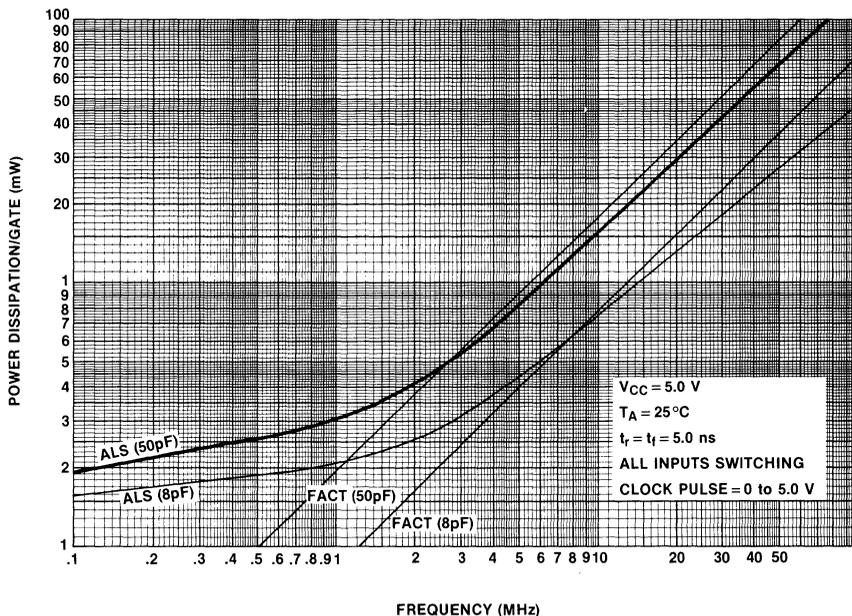
Figure 2-4 Power Dissipation per Gate vs. Frequency
