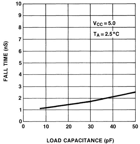
Figure 2-8  $t_f$  vs. Capacitance
