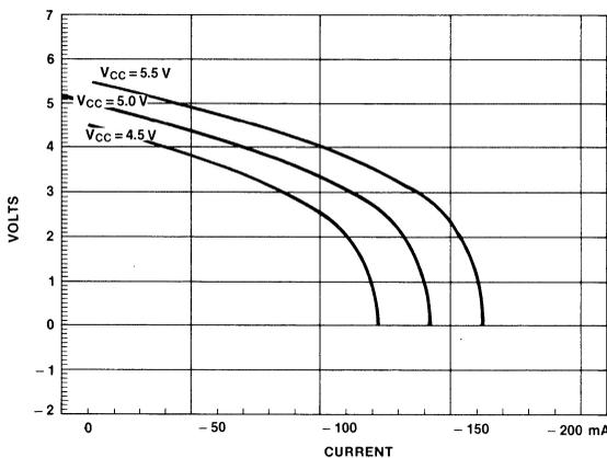
Figure 2-13 Output Characteristics  $V_{OH}/I_{OH}$ , 'AC00DC
