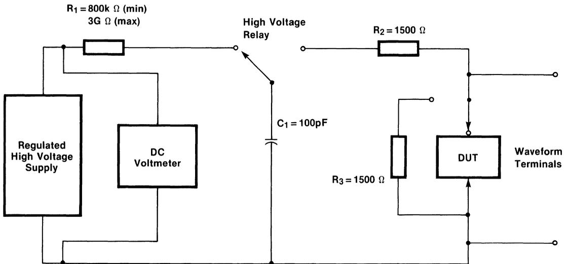
Figure 2-11 ESD Test Circuit
