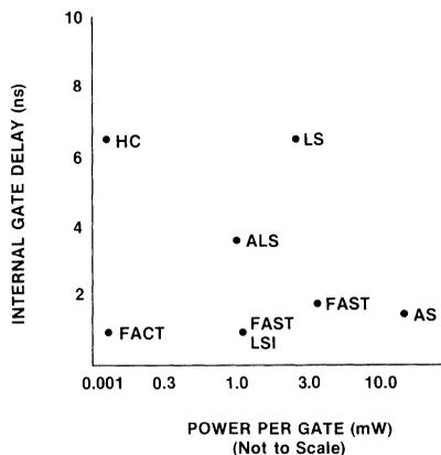
Figure 2-3 Internal Gate Delays
