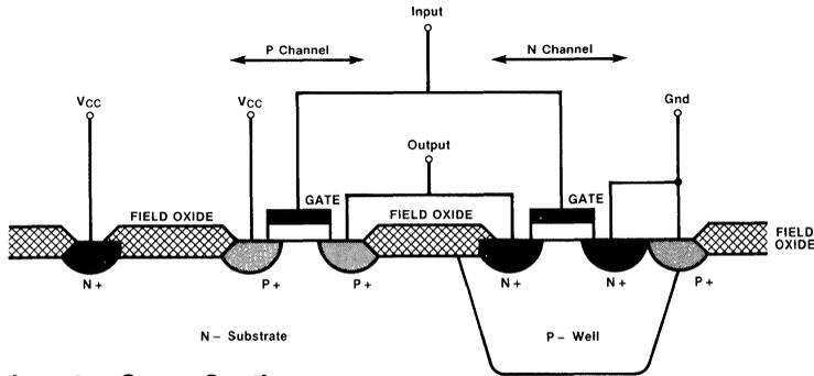
Figure 2-9 CMOS Inverter Cross Section
