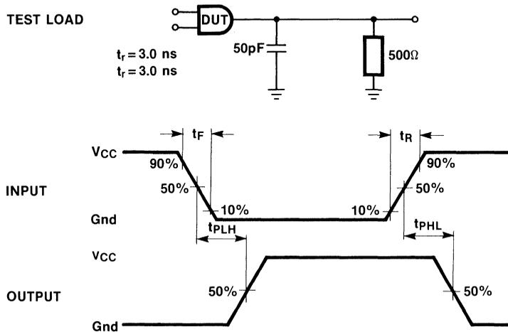
Figure 2-15 AC Measurement Conditions (Standard Outputs)
