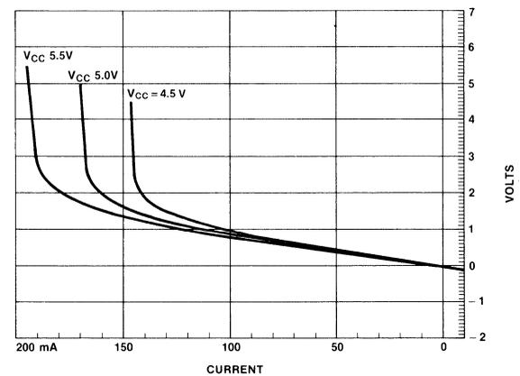
Figure 2-14 Output Characteristics  $V_{OL}/I_{OL}$ , 'AC00DC
