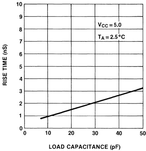
Figure 2-7  $t_r$  vs. Capacitance
