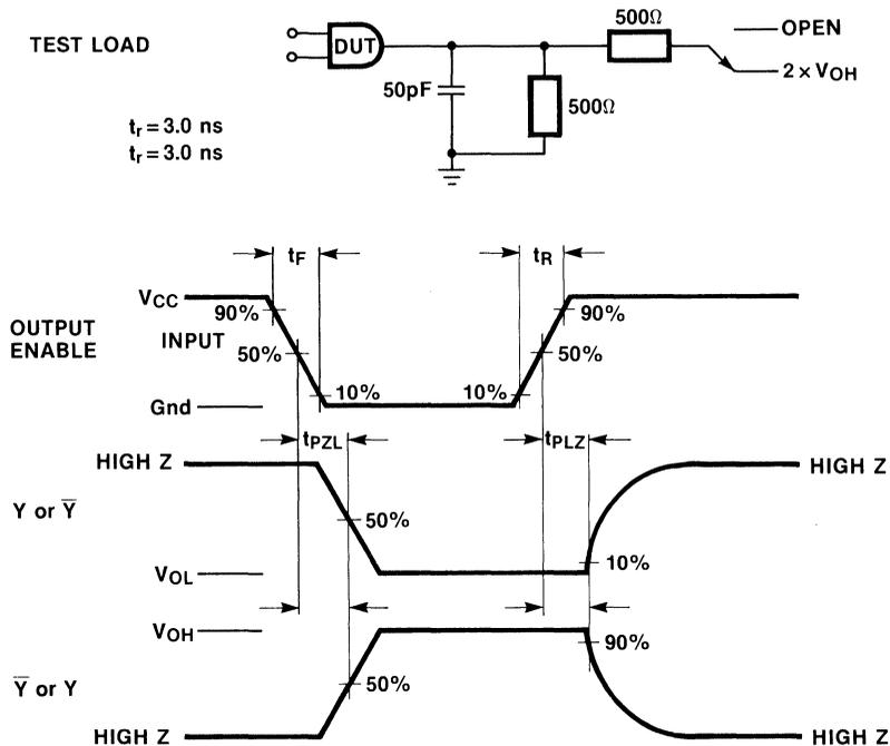
Figure 2-16 AC Measurement Conditions (3-State Outputs)
