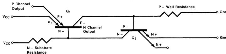
Figure 2-10 Latch Up Circuit Schematic
