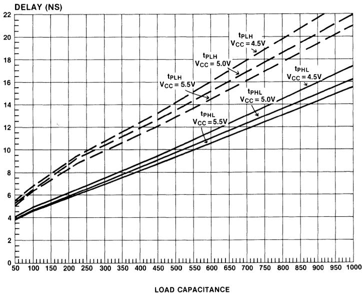
Figure 2-6 Propagation Delay vs. CL ('AC00)
