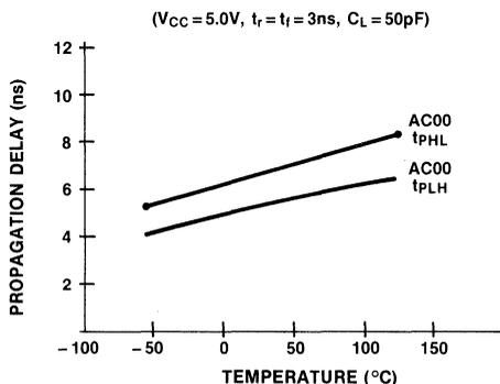
**Figure 2-2 Propagation Delay vs. Temperature**
