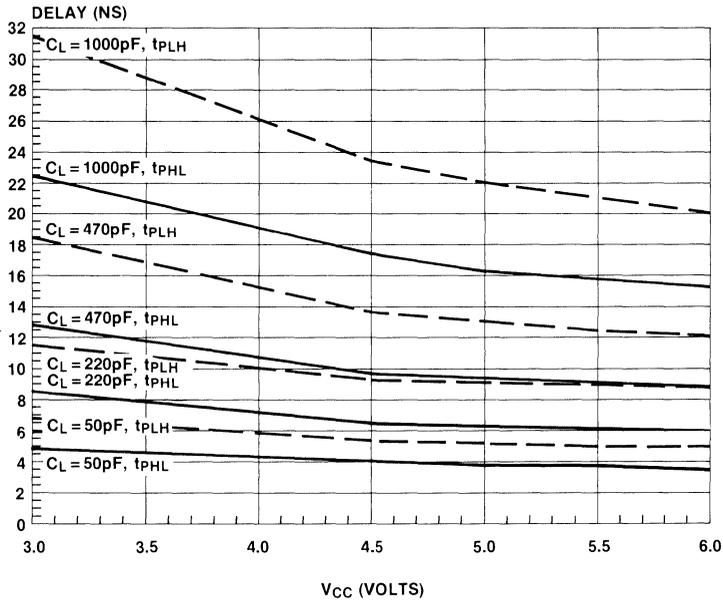
Figure 2-5 Propagation Delay vs. VCC ('AC00)
