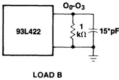
\*Includes jig and probe capacitance
