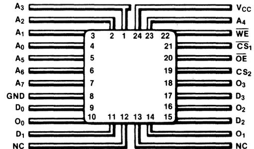
24-Pin Leadless Chip Carrier (Top View)
