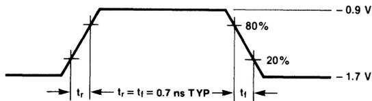
Fig. 3 Read Mode Timing
