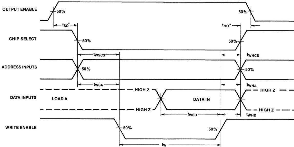
\* These timing parameters are only necessary to guarantee High Z state during the entire write cycle
