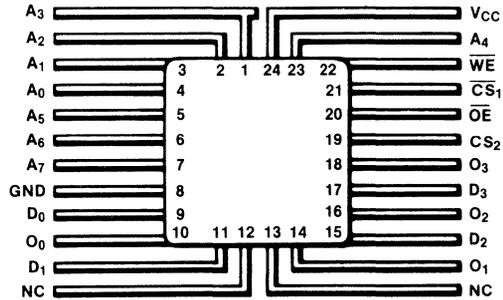
24-Pin Leadless Chip Carrier (Top View)
