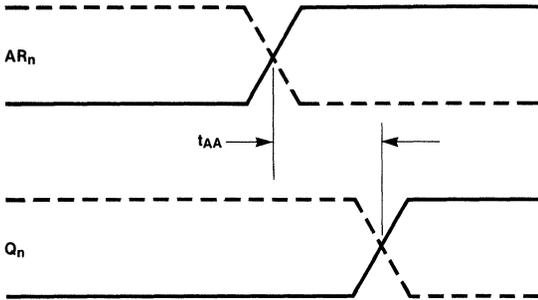
3b Address Setup Time before  $\overline{WE}$ , to Ensure Minimum Delay (unpulsed  $\overline{WE} = \overline{OE}_1 = \overline{OE}_2 = \text{LOW}$ )
