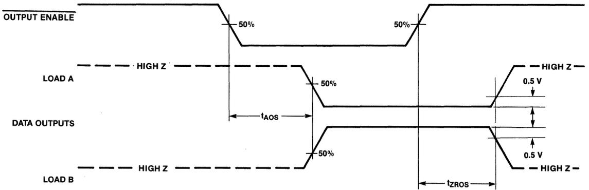
Fig. 4 Write Mode Timing
