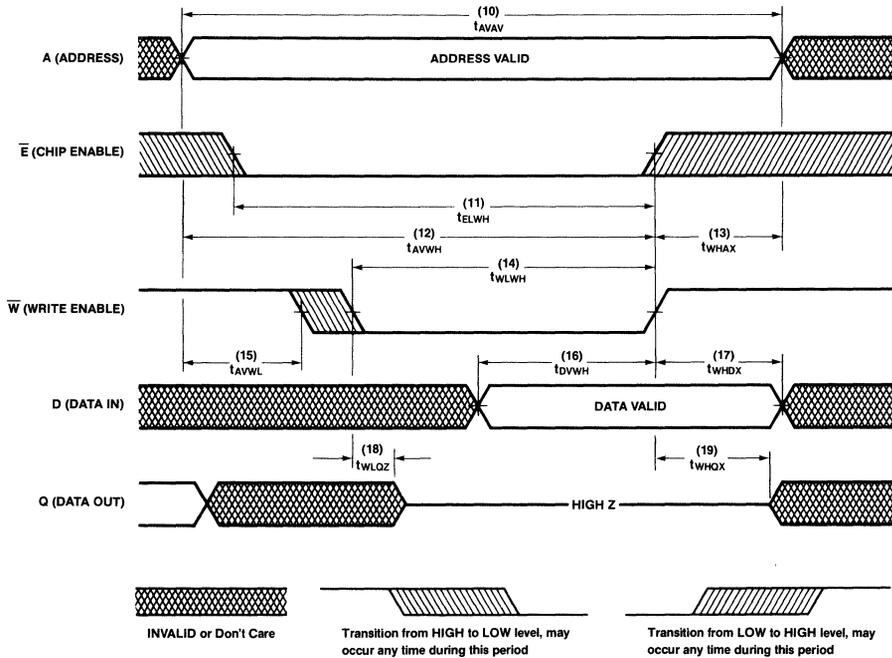
**Write Cycle 2** ( $\overline{E}$  controlled, where  $\overline{W}$  is active prior to  $\overline{E}$  becoming active. See Note 9.)
