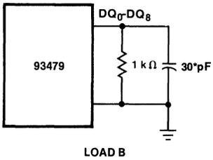
\*Includes jig and probe capacitance
