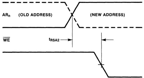
3d Address Hold Time to Ensure Latching Data from Old Address (unpulsed  $\overline{WE} = \text{LOW}$ )
