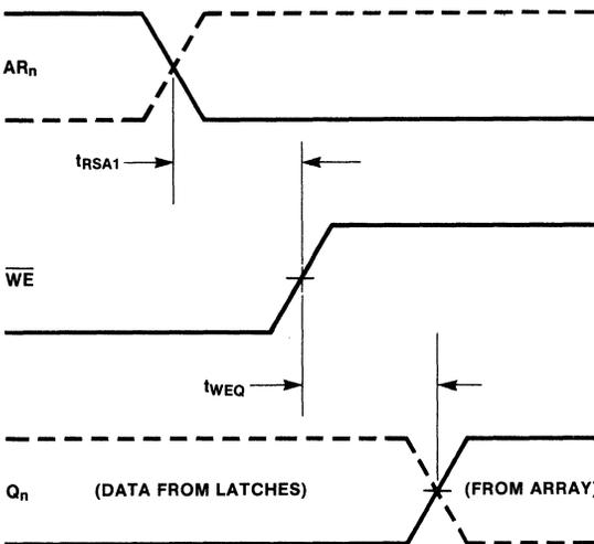
3c Address Setup Time to Ensure Latching Data from New Address (unpulsed  $\overline{WE} = \text{LOW}$ )
