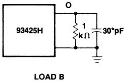
\*Includes jig and probe capacitance
