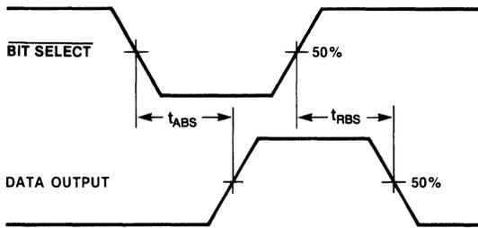
3b Read Mode Propagation Delay from Address
