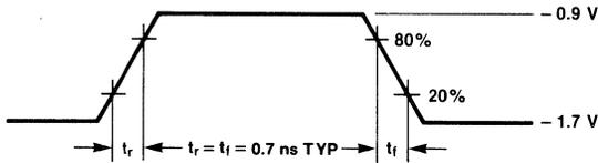
Fig. 3 Read Mode Timing
