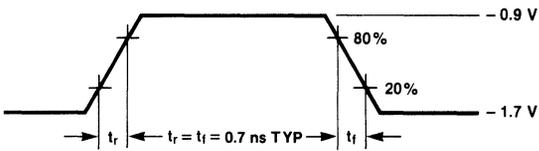
Fig. 3 Read Mode Timing
