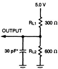
\*Includes jig and probe capacitance
