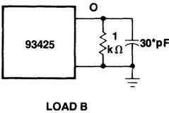
\*Includes jig and probe capacitance
