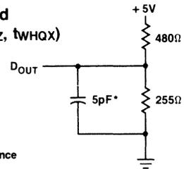
\*Includes jig and probe capacitance
