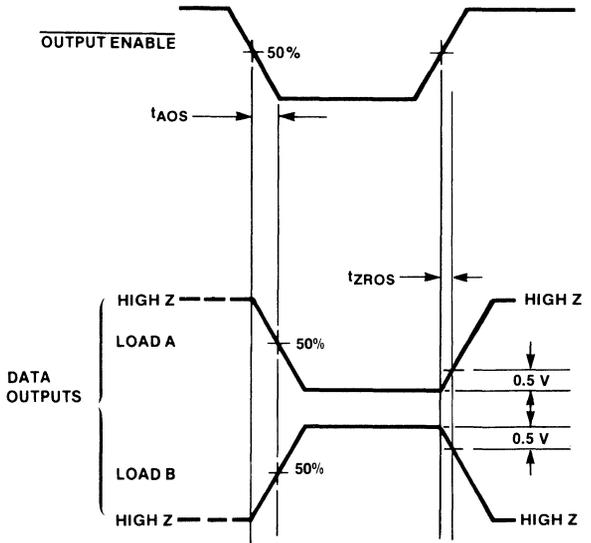
Fig. 4 Write Mode Timing
