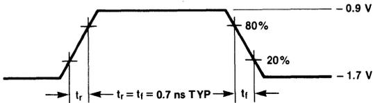
Fig. 3 Read Mode Timing
