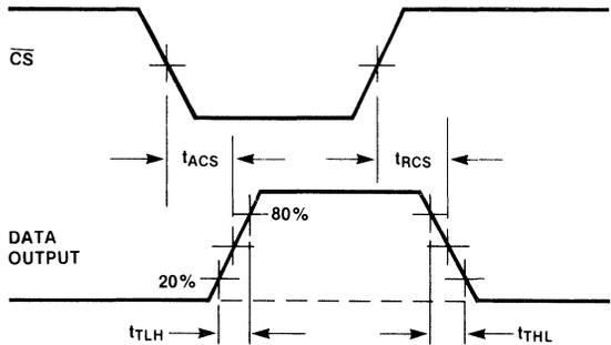
Write Enable Input to Data Output ( $\overline{CS} = \text{LOW}$ )
