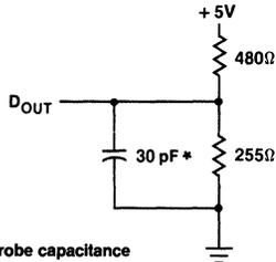
\*Includes jig and probe capacitance
