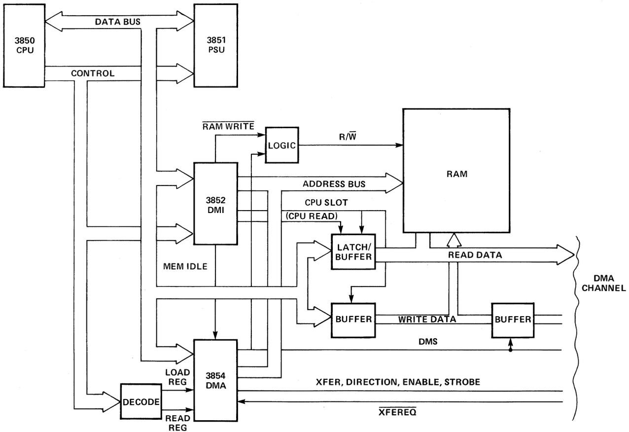
Figure 13-1. A Typical DMA Configuration
