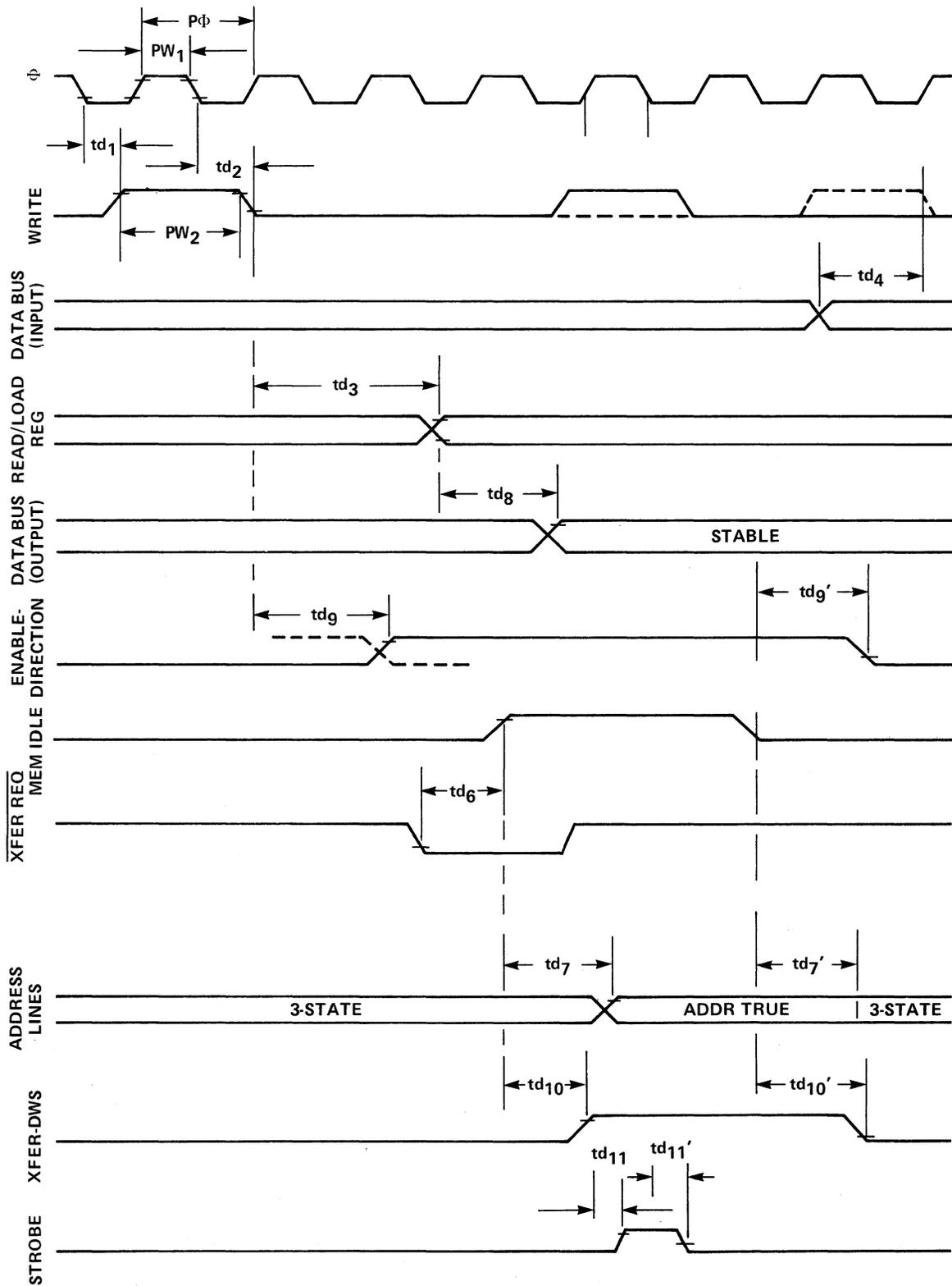
Figure 6-5. 3854 DMA Device Signals and Timing
