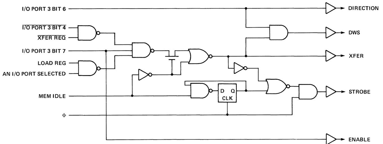
Figure 6-4. DMA Control Signals Output by the 3854 DMA Device
