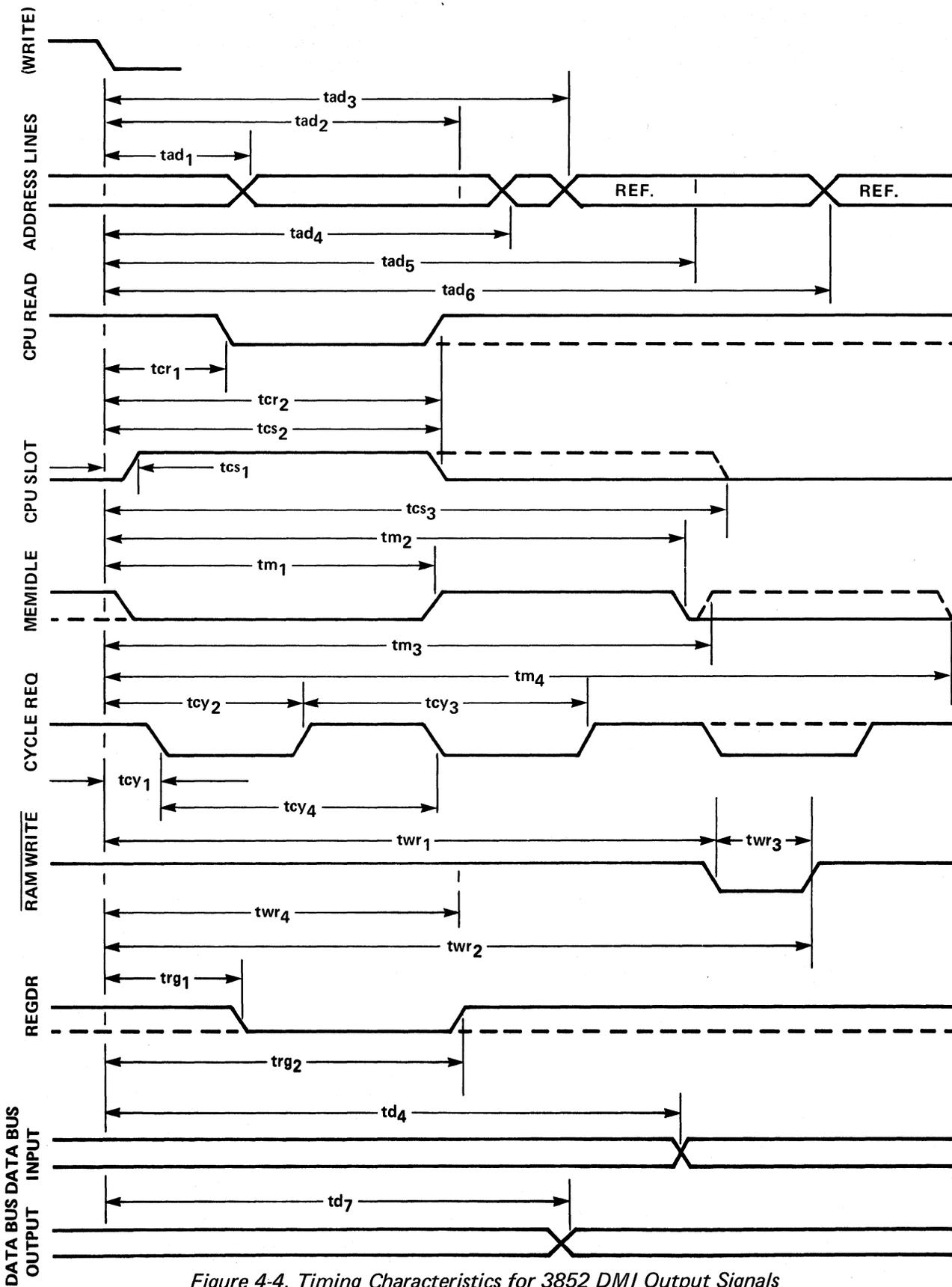
Figure 4-4. Timing Characteristics for 3852 DMI Output Signals
