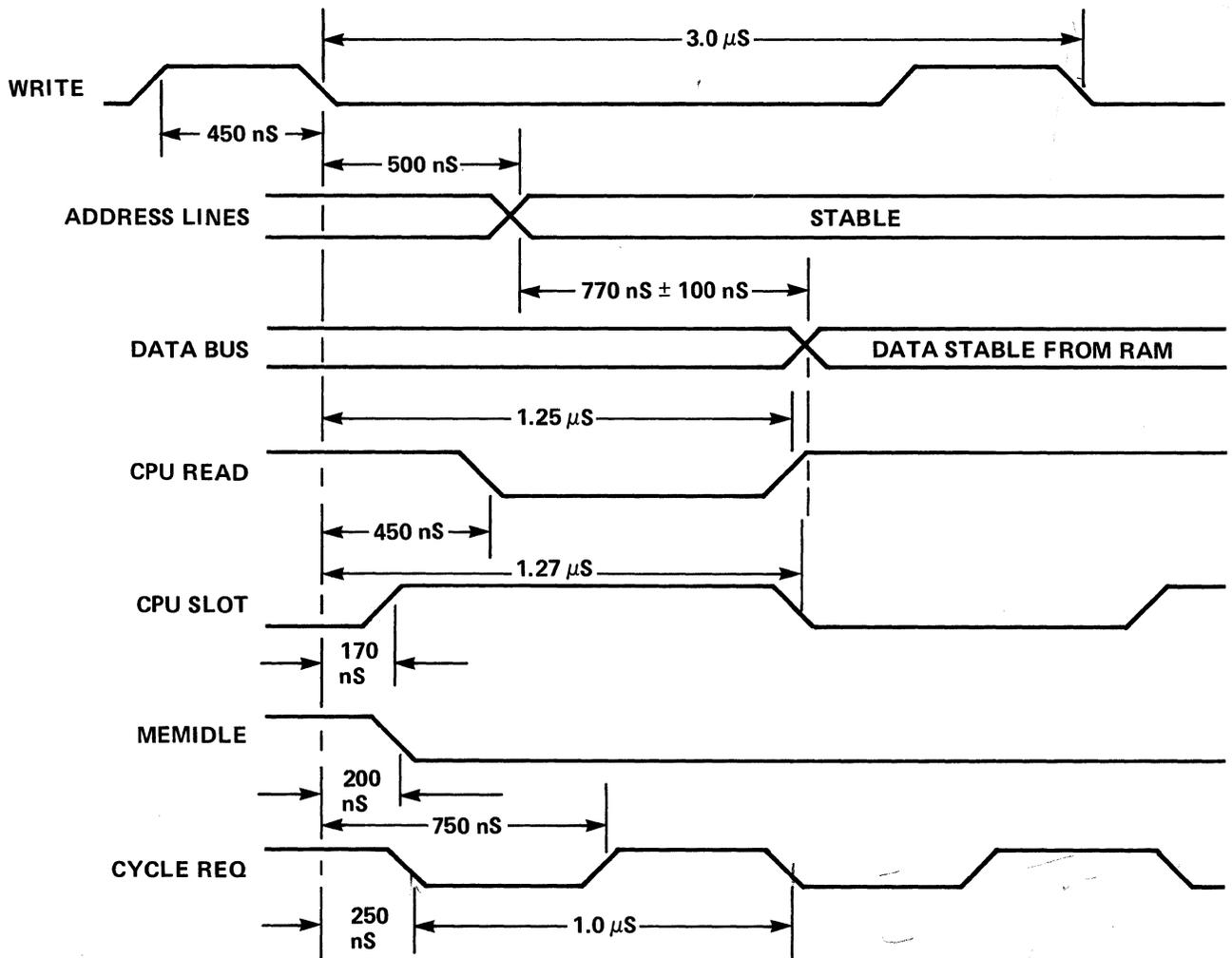
Figure 4-6. 3852 DMI Timing Signals Output during a Long Cycle Memory Read, with Address Out of Program Counter
