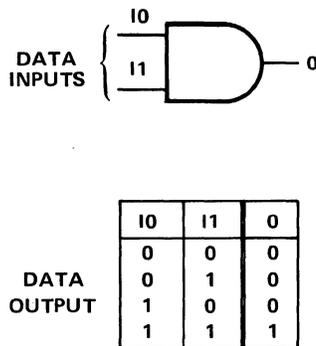
Figure 1-1. A Very Elementary Logic Device
