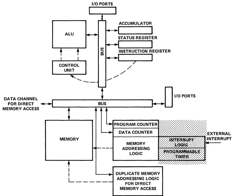
Figure 1-13. 3861 Peripheral Input/Output Device Logic
