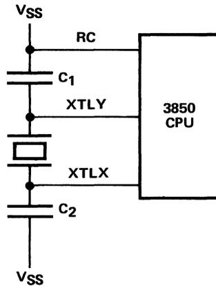
Figure 2-5. Crystal Mode Clock Generation
