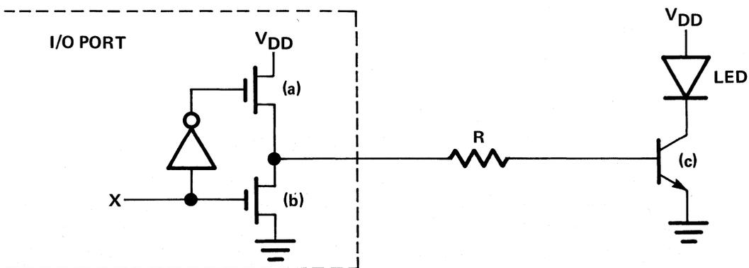
Figure 3-6. Driver Pull-up Configuration
