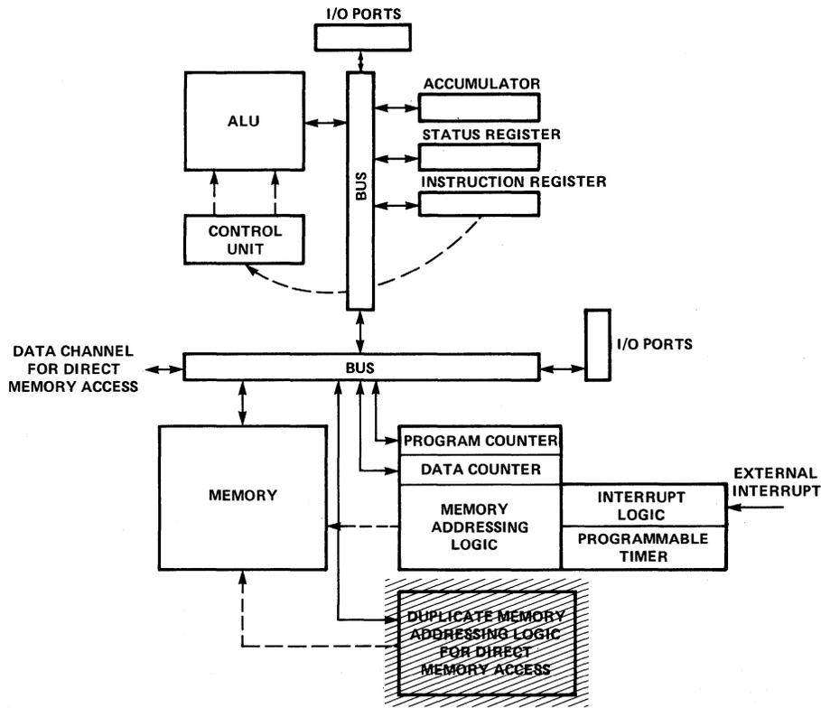
Figure 1-14. 3854 Direct Memory Access Device Logic
