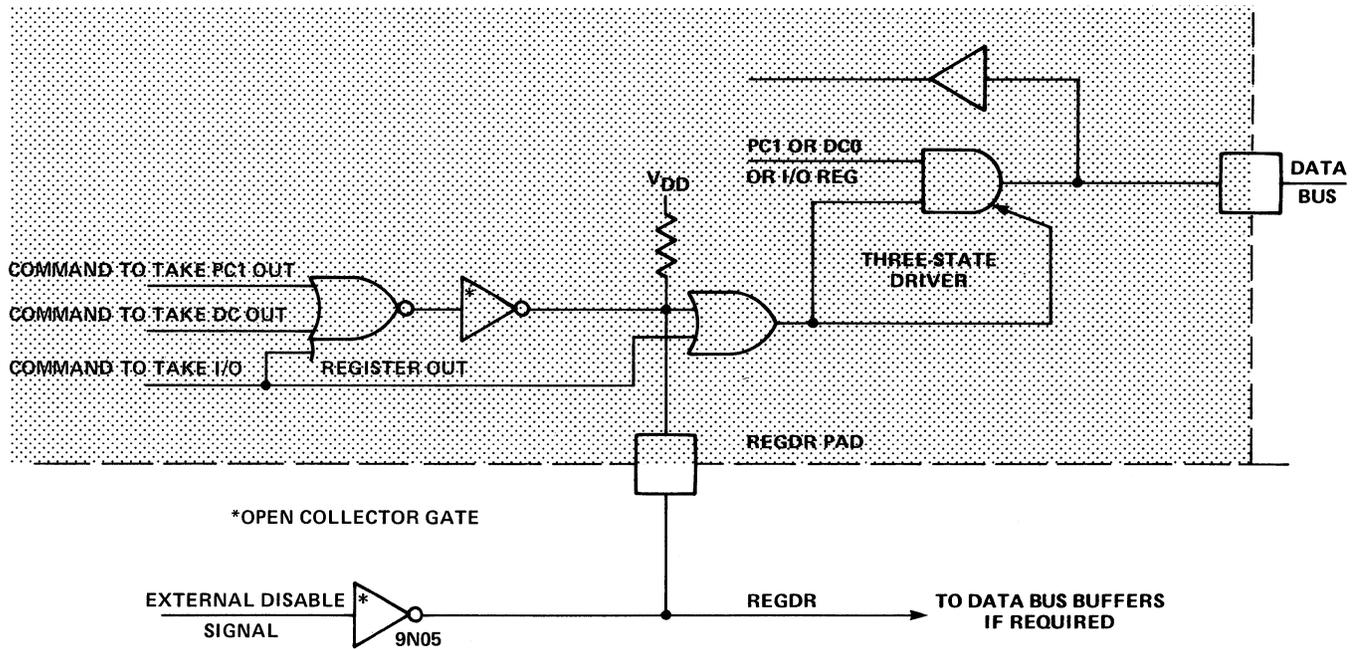
Figure 12-3. REGDR Controls Data Bus Drivers
