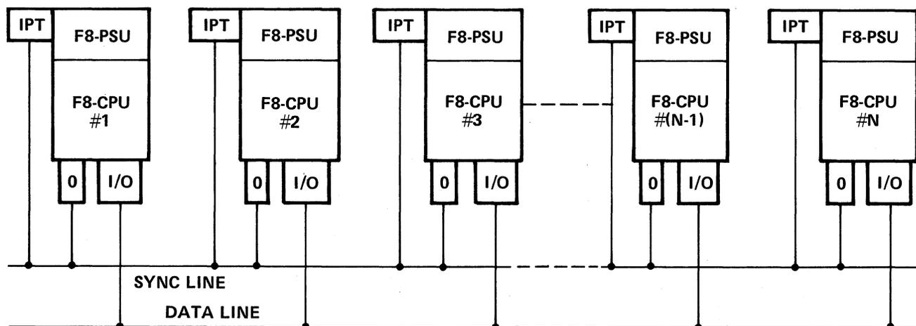
Figure 14-4. F8 Microprocessor Network using a Symetrically Connected Two-Wire System
