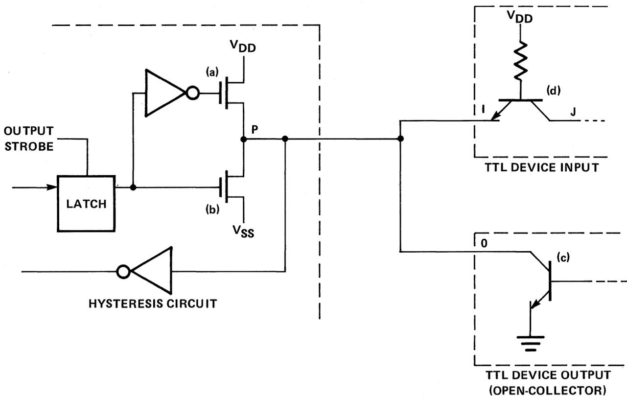
Figure 2-12. An F8 I/O Port Bit
