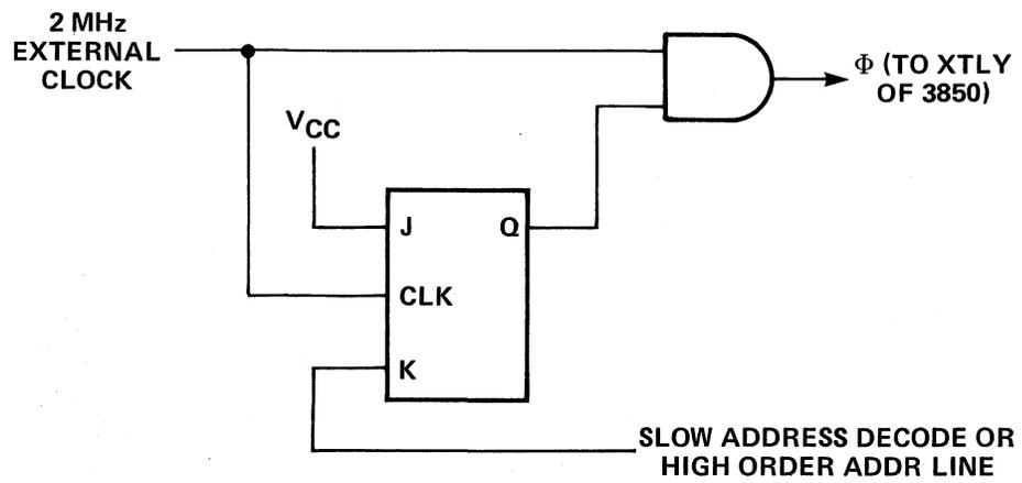
Figure 12-7. Modifying Clock Period under Hardware Control
