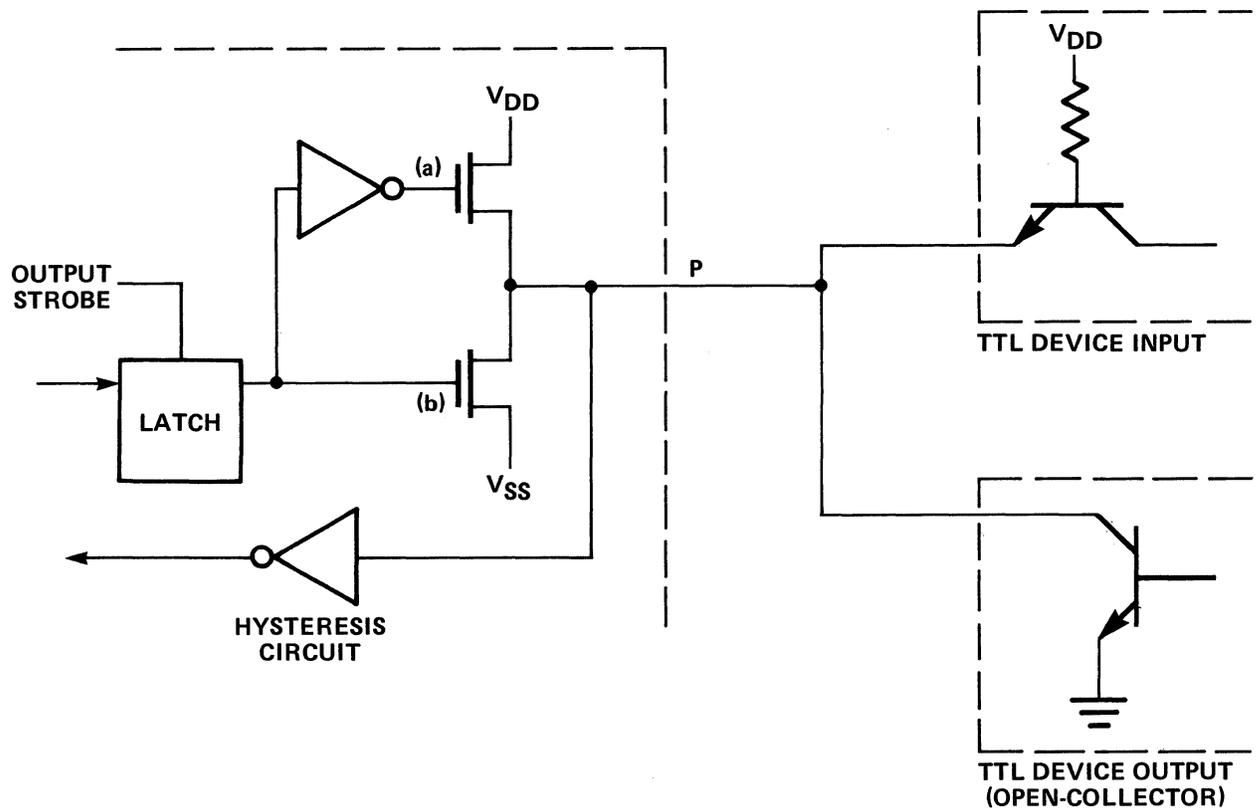
Figure 7-5. An F8 I/O Port Bit
