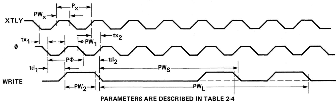
*Figure 2-8. Timing Signal Specifications*
