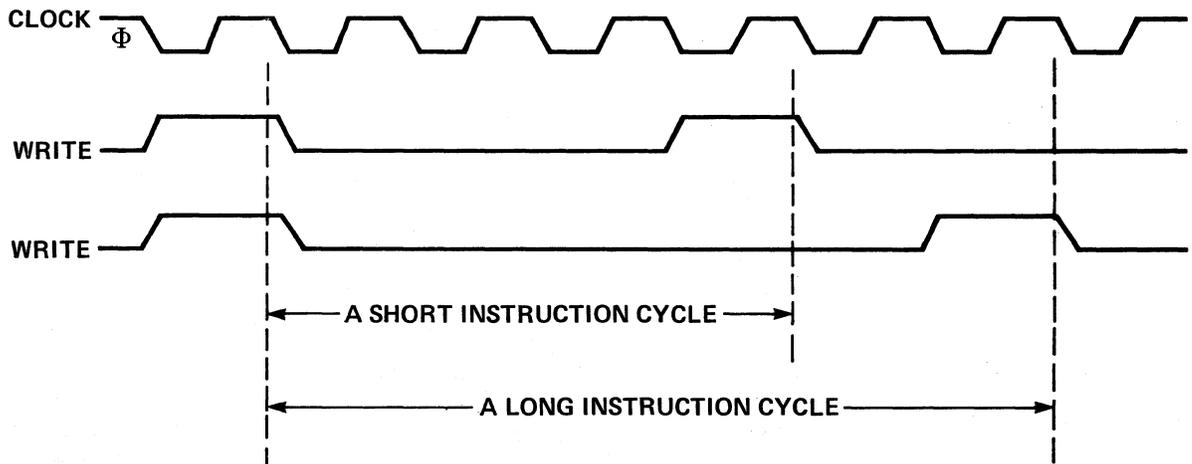
Figure 1-9. F8 Microcomputer Timing
