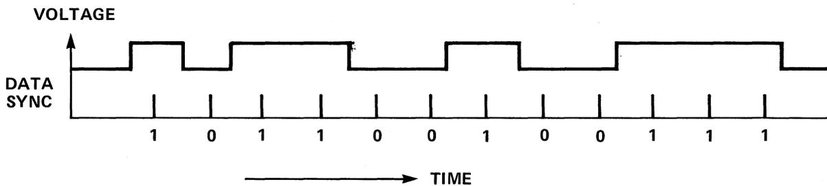
Figure 14-3. Timing Relationship between Data and Sync Signals
