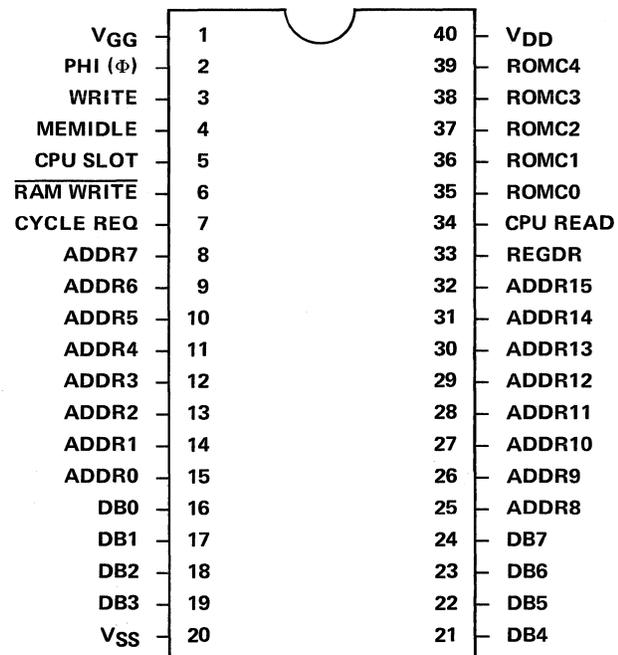
Figure 4-2. 3852 DMI Pin Assignments
