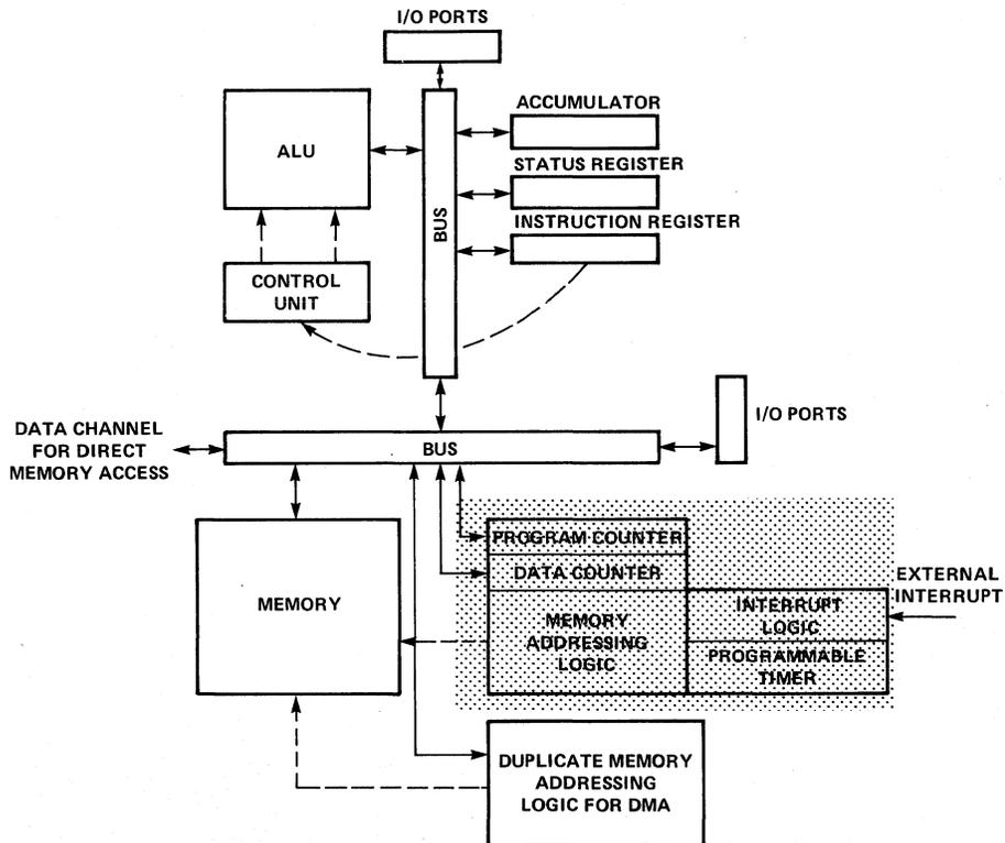
Figure 1-12. 3853 Static Memory Interface Device Logic
