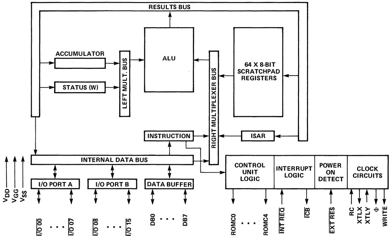
Figure 2-1. Logical Organization and Pins for the 3850 CPU
