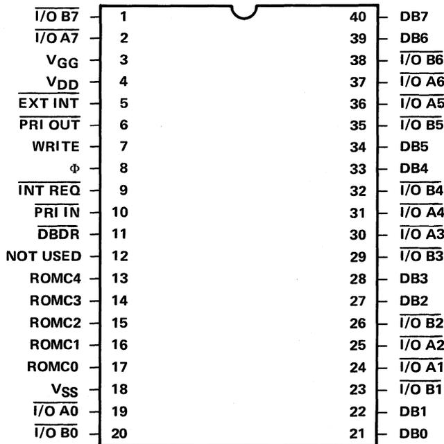
Figure 3-2. 3851 PSU Pin Assignments
