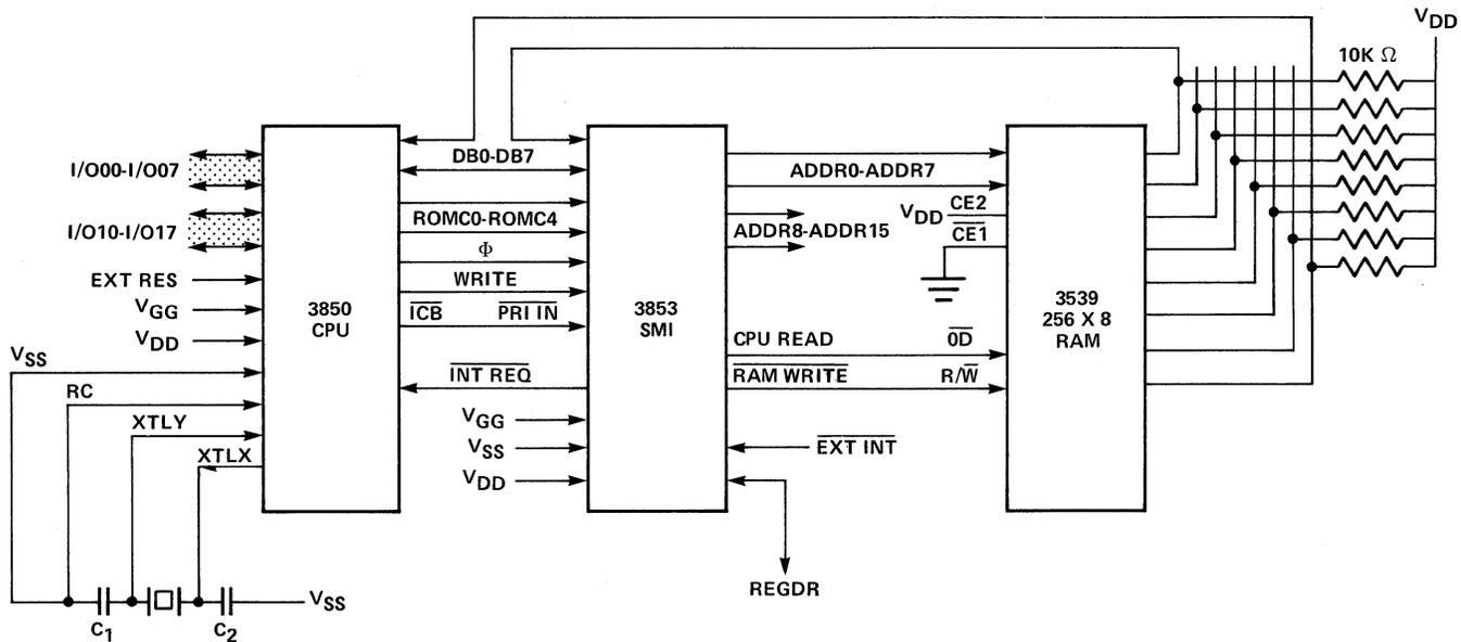
Figure 12-1. Interfacing RAM using a 3853 SMI
