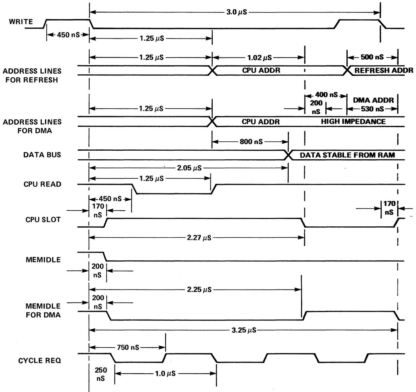
Figure 4-12. Timing for Memory Refresh and DMA during a Long Cycle Memory Read, with Address Out of Data Counter
