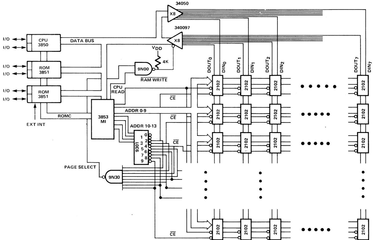
Figure 12-4. 2K ROM and 8K RAM Configuration using 2102 Memory Devices
