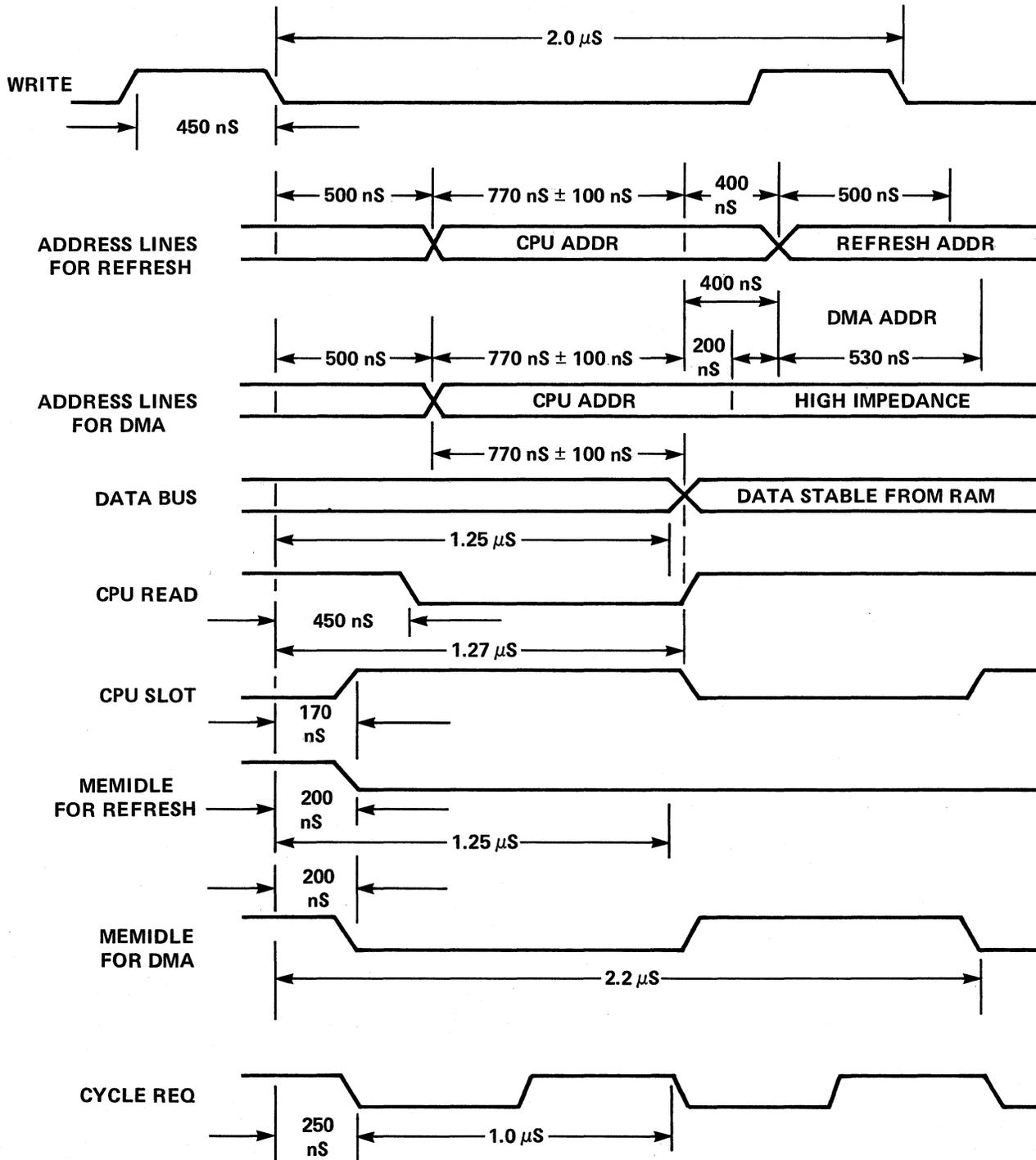
Figure 4-10. Timing for Memory Refresh and DMA during a Short Cycle Memory Read, with Address Out of Program Counter
