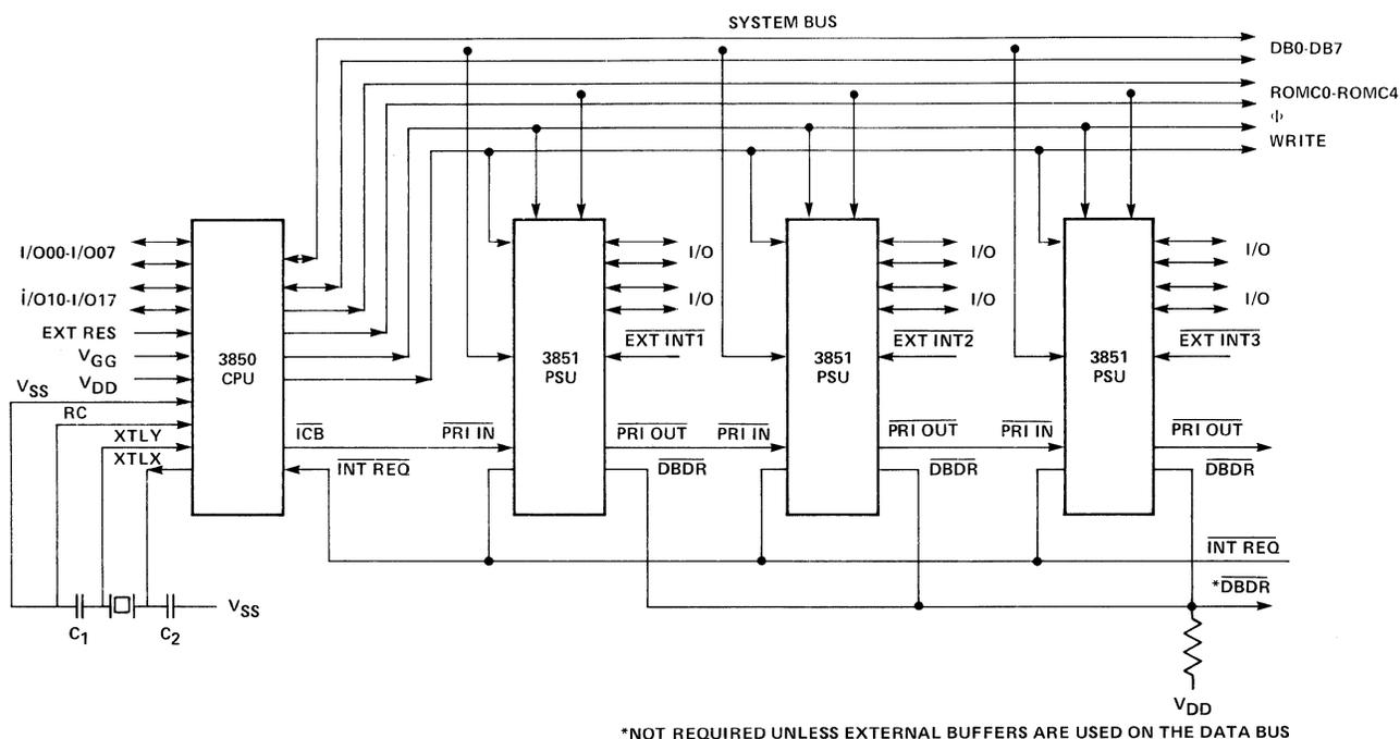
Figure 11-6. A Multi PSU F8 Configuration
