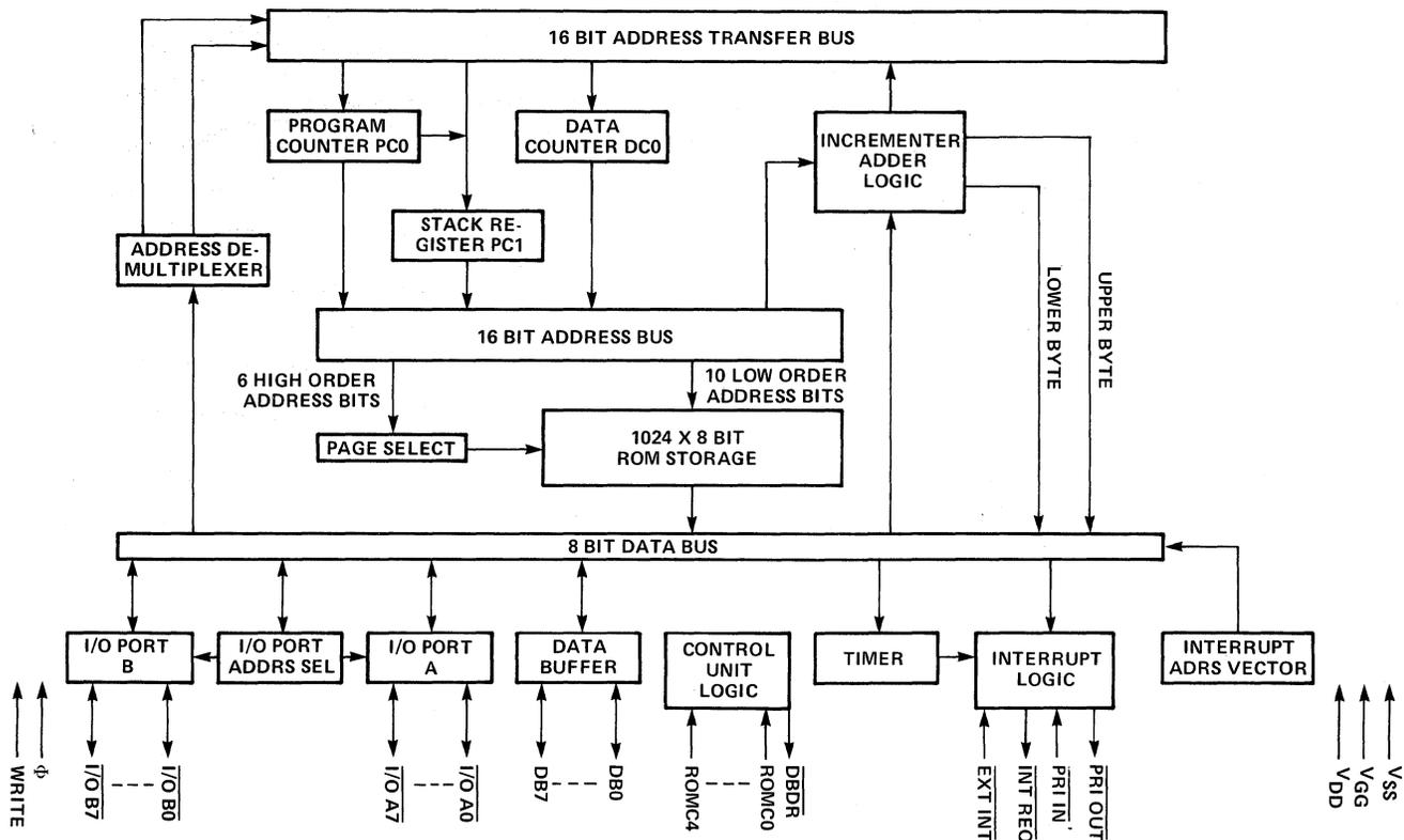
Figure 3-1. Logical Organization and Pins for the 3851 PSU
