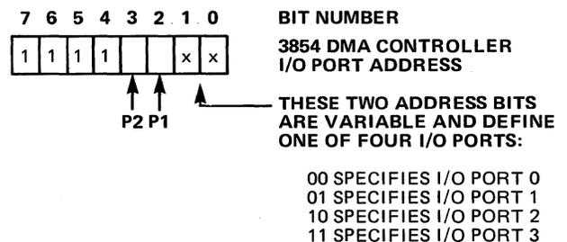
Table 6-1. Addresses of I/O Ports Used by 3854 DMA Devices
