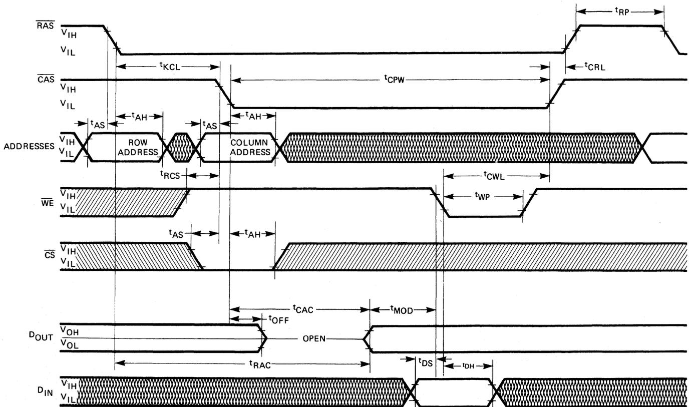
\*Read-modify-write cycle time =  $t_{RCL} + t_{CAC} + t_{MOD} + t_{CWL} + t_{CRL} + t_{RP} + 3t_f + t_r$ .
