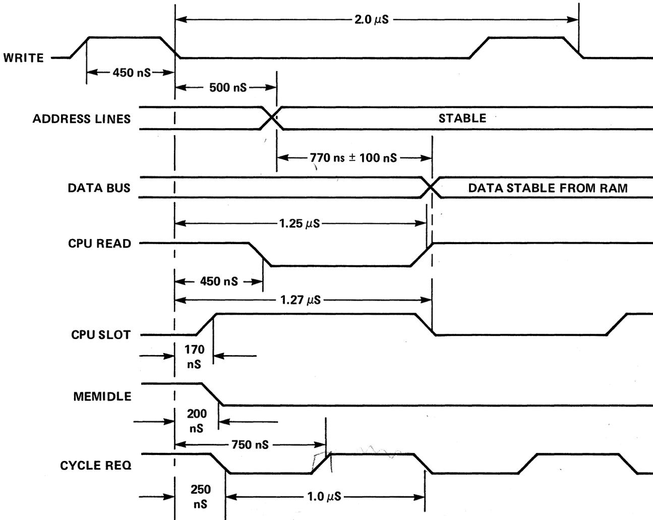
Figure 4-5. 3852 DMI Timing Signals Output during a Short Cycle Memory Read with Address from PC0
