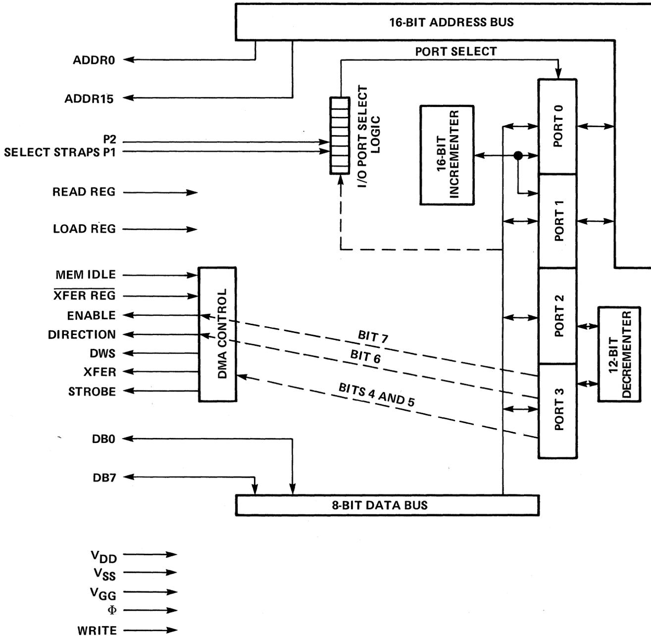
Figure 6-1. Logic Organization and Pins for the 3854 DMA Device
