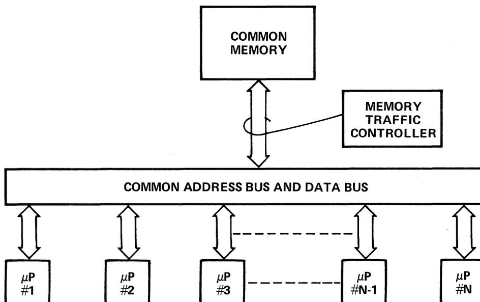
Figure 14-5. Microprocessor Network with Common Memory
