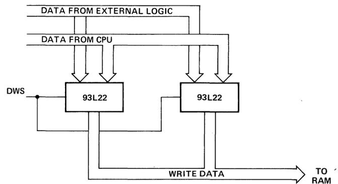
The 83L22 devices are low power quad two-input multiplexers. Each is four bits wide. DWS is used to select between the two data sources.
