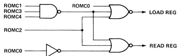
The principle input from external logic to the 3854 DMA device is  $\overline{XFER REQ}$ . Here is one way in which this signal might be generated out of an input request and an output request:
