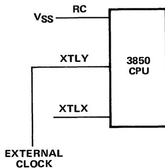
Figure 2-6. External Mode Clock Generation
