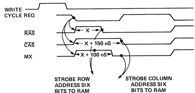
X is the address set-up time for the DMI, and has a worst case, maximum value of 400 nS.
