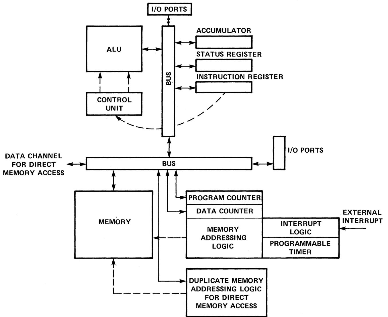
Figure 1-8. Functional Logic of a Complete Microcomputer System
