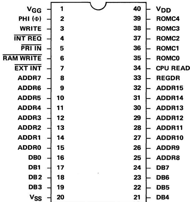
Figure 5-2. 3853 SMI Pin Assignments
