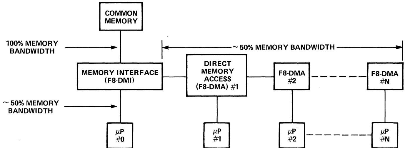
Figure 14-6. Multiprocessor Network using F8-DMI and F8-DMA Chips
