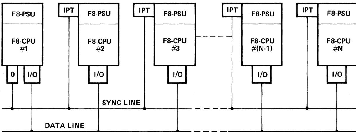
Figure 14-2. F8 Microprocessor Network using a Two-Wire Bus
