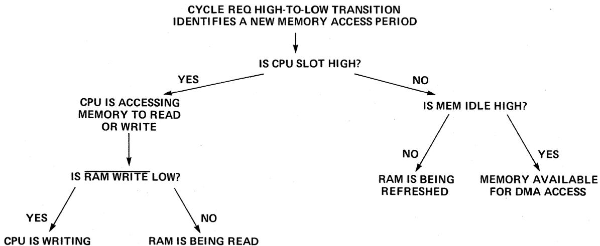
Figure 4-9. Interpretation of Signals Output by the 3852 DMI
