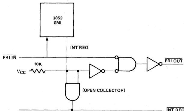
Second, the 3853 SMI interrupt address vector consists of two programmable I/O ports. The interrupt address vector is set under program control, rather than being a mask option, as it is with the 3851 PSU. Even though the 3853 SMI interrupt address vector is programmable, bit 7 is still set to 0 for a timer interrupt, or to 1 for an external interrupt, as described for the 3851 PSU.
