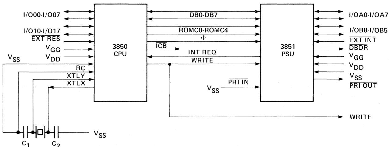
Figure 11-1. A Basic, Two-Device F8 Configuration
