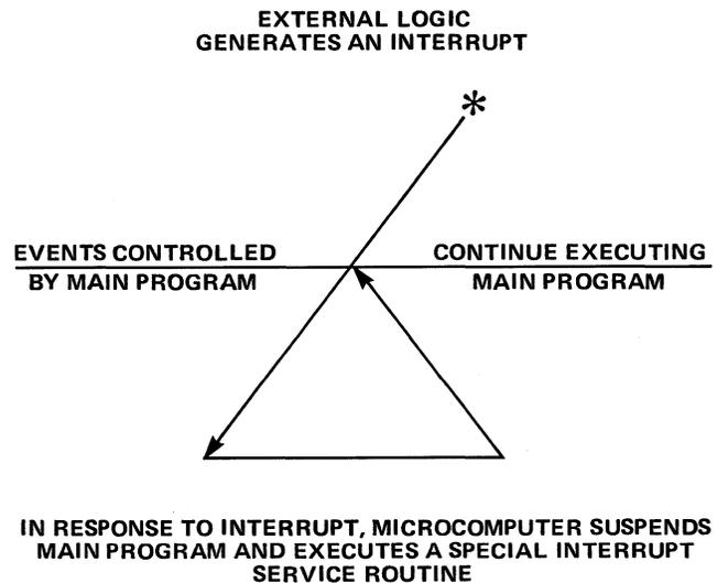
Figure 1-6. The Concept of an Interrupt
