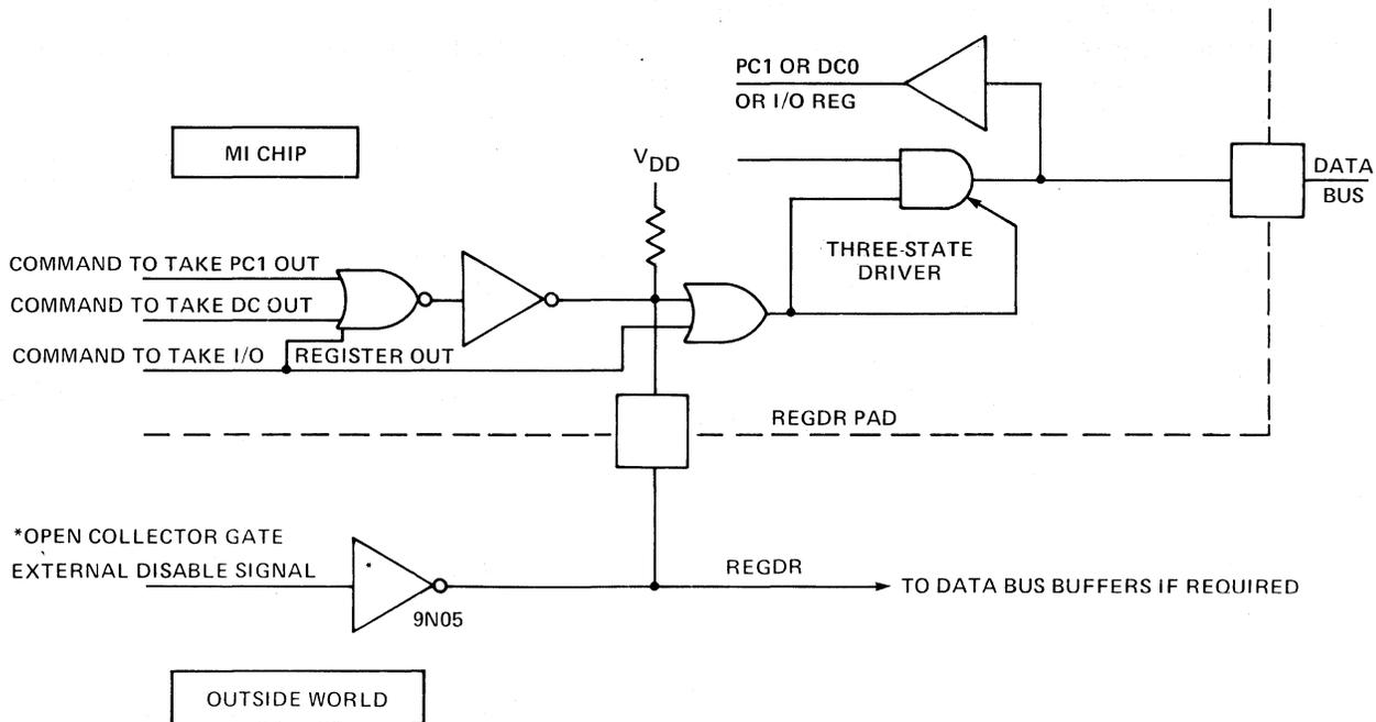
Figure 5-3. REGDR Controls Data Bus Drivers
