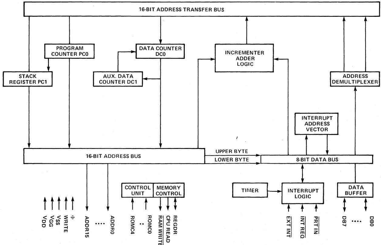
Figure 5-1. Logic Organization and Pins for the 3853 SMI
