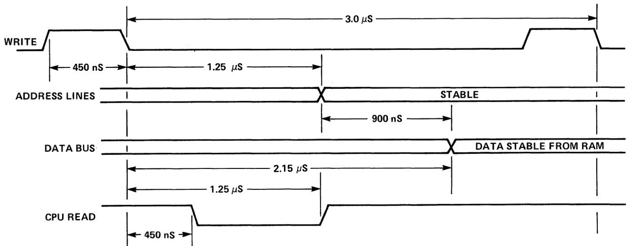
Figure 5-7. 3853 SMI Timing Signals Output during a Long Cycle Memory Read, with Address Out of Data Counter
