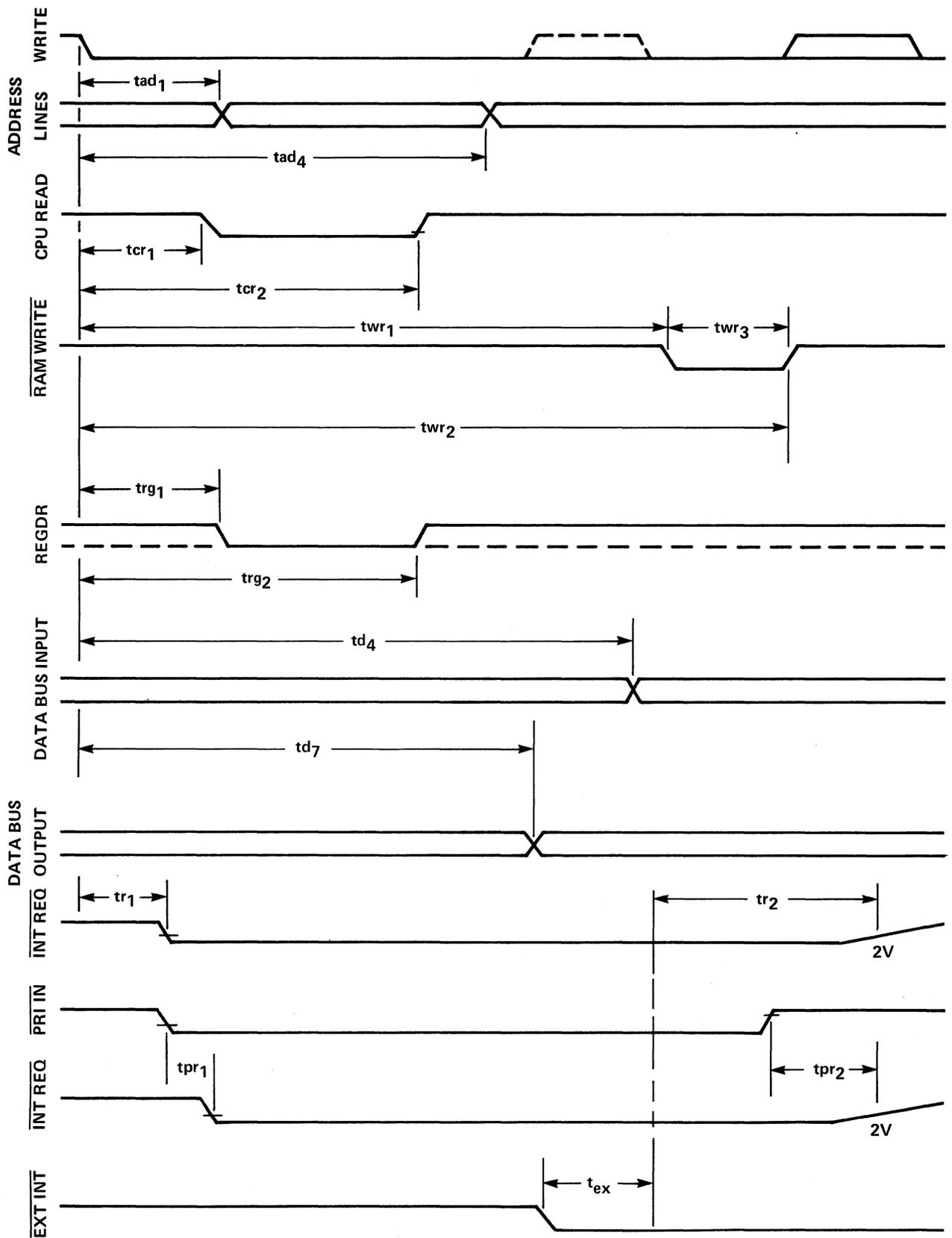
Figure 5-4. 3853 Signal Timing
