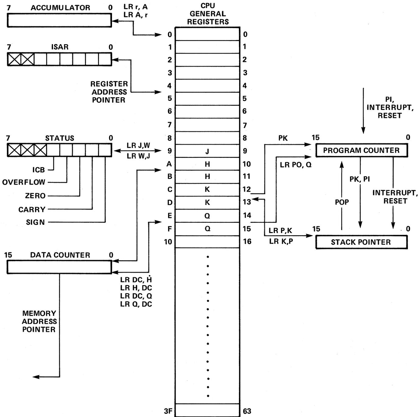
Figure 2-15. Instructions that Move Data between the Scratchpad and Registers
