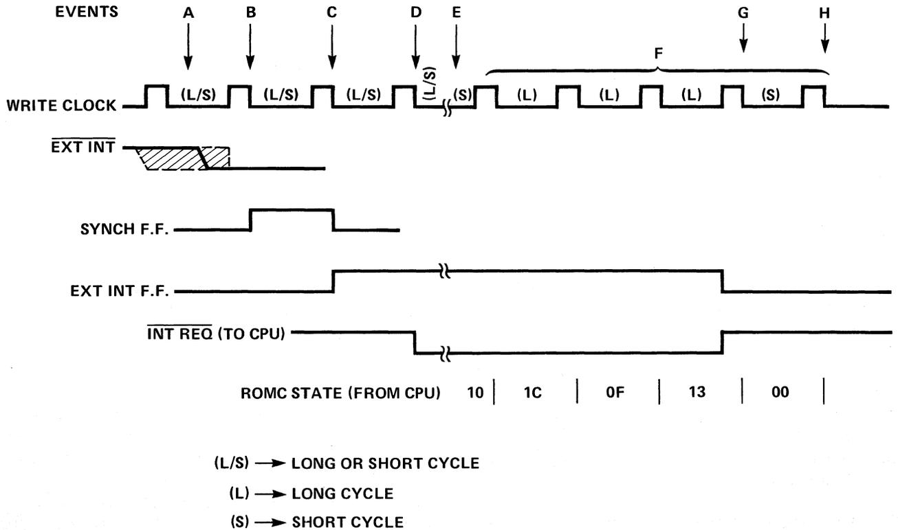
Figure 3-12. External Interrupt Sequence
