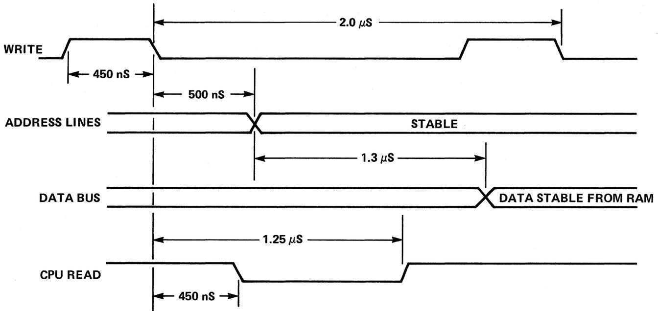
Figure 5-5. 3853 SMI Timing Signals Output during a Short Cycle Memory Read Using PC0
