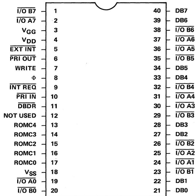
Figure 7-2. 3861 PIO Pin Assignments
