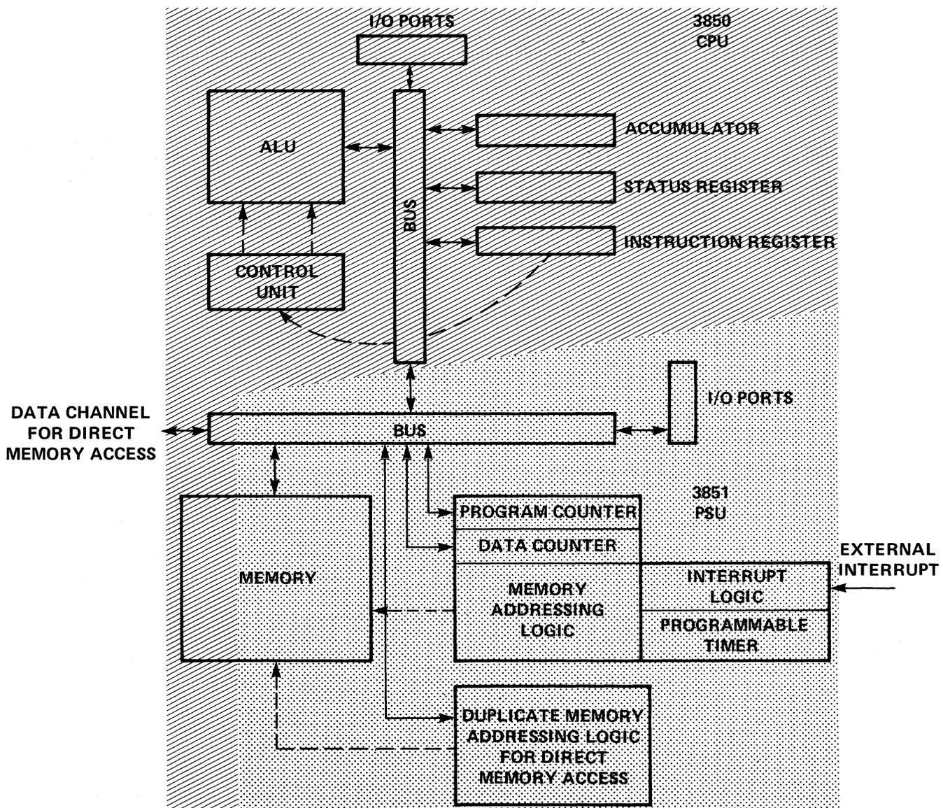
Figure 1-10. A Two-Device Configuration Consisting of a 3850 CPU and a 3851 PSU
