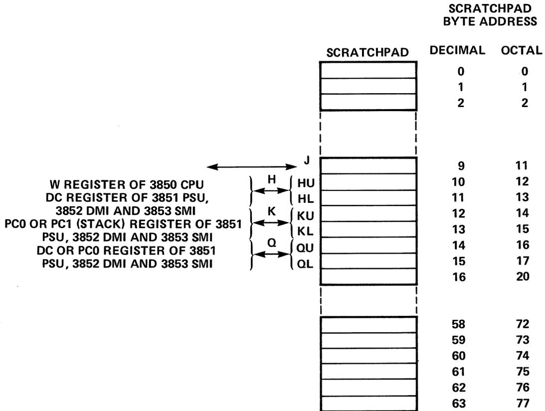
Figure 2-3. The 3850 CPU Scratchpad Registers
