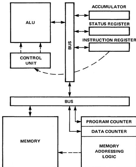
Figure 1-5. A Simple CPU with Memory
