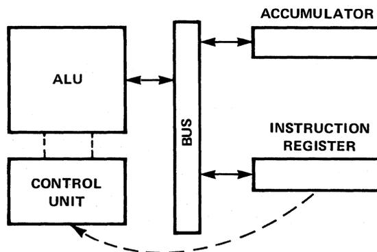
Figure 1-4. An Elementary Central Processing Unit
