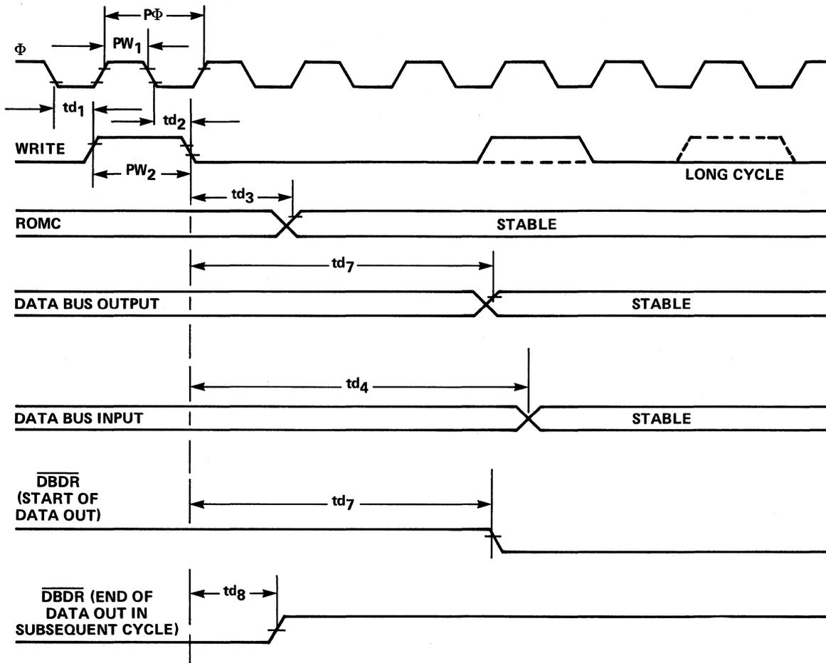
Figure 7-3. 3861 PIO Data Bus Timing
