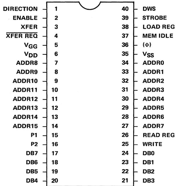
Figure 6-3. 3854 DMA Pin Assignments
