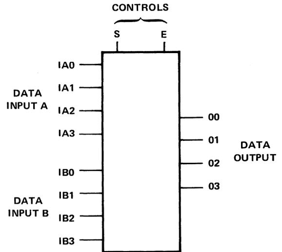
Figure 1-2. A Logic Device Using Control Signals
