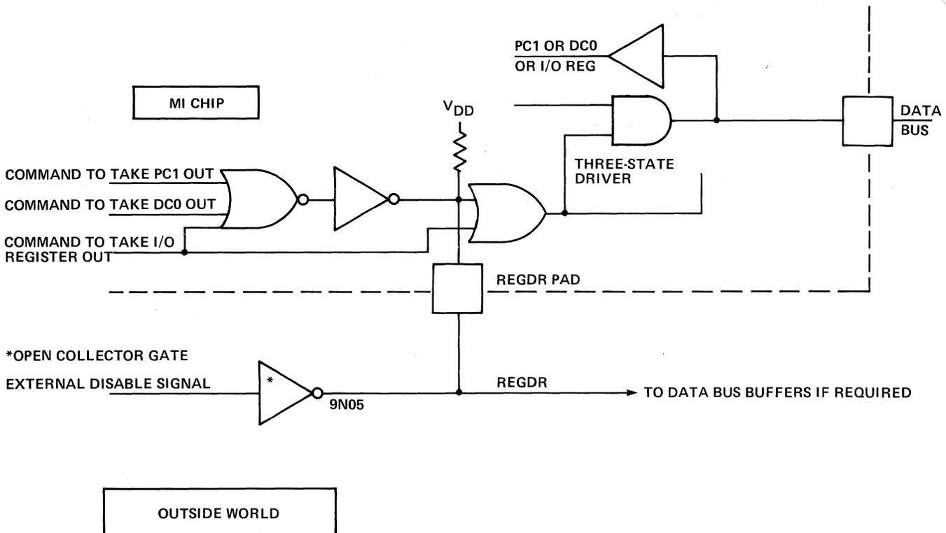
Figure 4-3. REGDR Controls Data Bus Drivers
