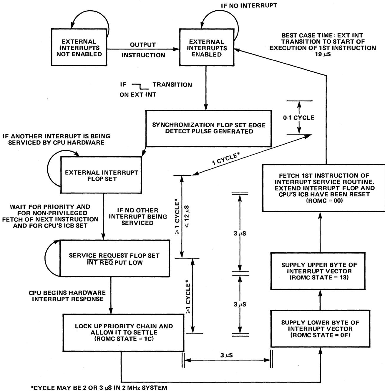
Figure 11-5. A Time State Diagram for the 3851 PSU External Interrupt Request Logic
