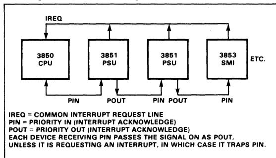
Fig. 8-1. Daisy Chaining and Interrupt Priority Determination
