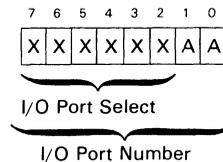
The 3852 DMI and 3853 SMI devices have a fixed (pre-assigned) I/O port select code, but have no on-board chip select code.
