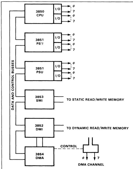
Fig. 2-5. F8 Microprocessor System Configurations
