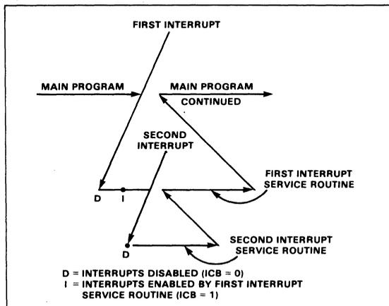
Fig. 8-2. Two Levels of Interrupt
