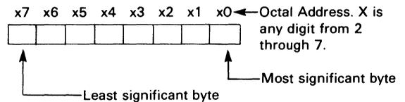
By starting ISAR at x7, all eight bytes of the buffer will be processed identically, since ISAR will be decremented to x6 before the first execution of BR7. Thus the loop will be executed seven times, until ISAR decrements from x0 back to x7. Program steps are as follows:
