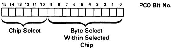
Each 3851 device has a unique select code that is a permanent mask option; 3851 memory access logic is only activated when the six Chip Select bits of PC0 match the 3851 select code. Thus, if more than one 3851 is present in an F8 system, every 3851 device's PC0 register holds the address of the memory byte from which the next instruction code will be fetched for transmittal to the 3850 CPU; but an instruction fetch will actually be executed from one 3851 device only.
