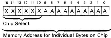
The 3851 PSU I/O port select code is also a six digit binary number, and is independent of the chip select code. The I/O port select code is always the highest six bits for I/O port numbers on that device:
