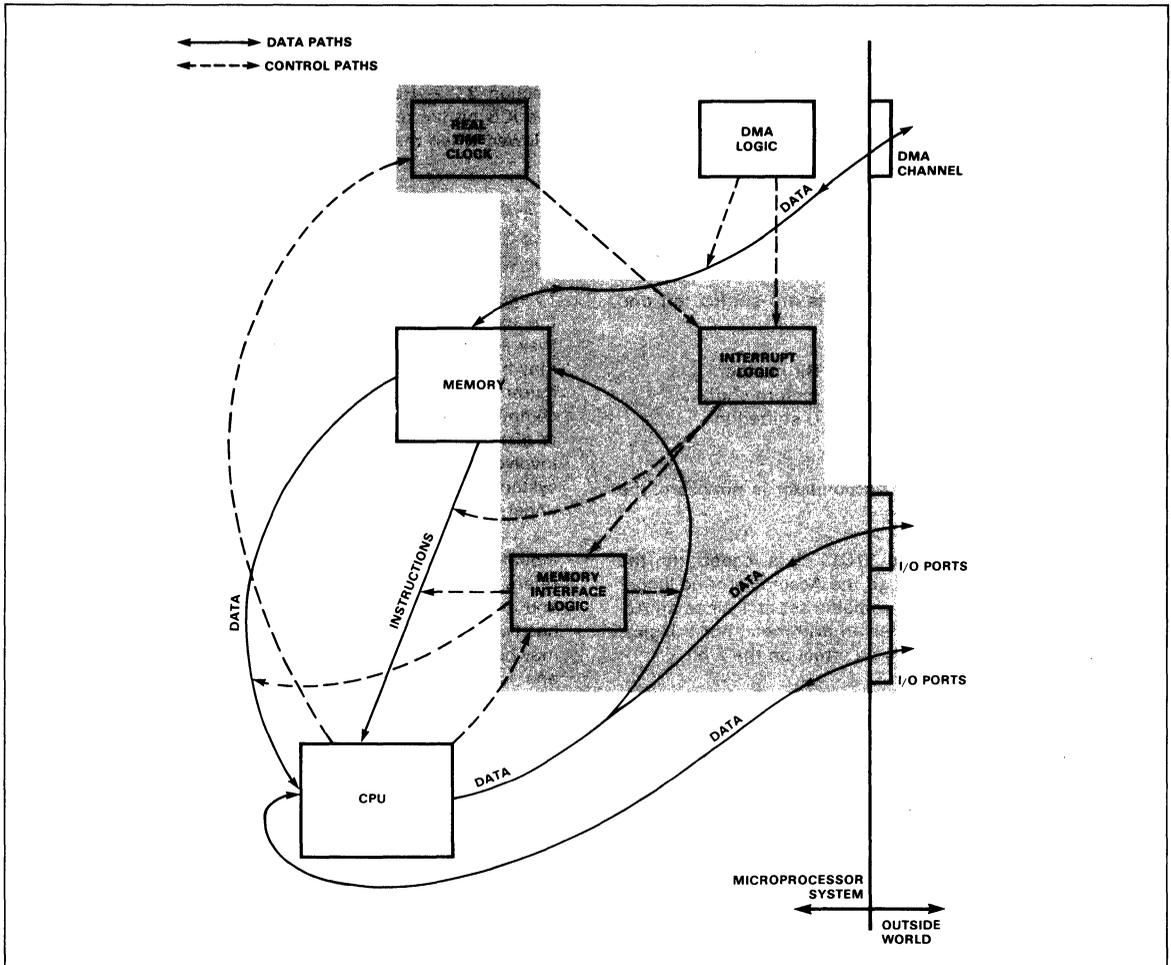
Fig. 2-9. Logical Functions of the 3851 PSU
