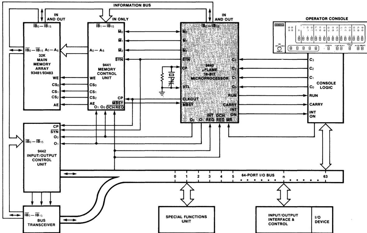
Fig. 7 9440 Microflame System
