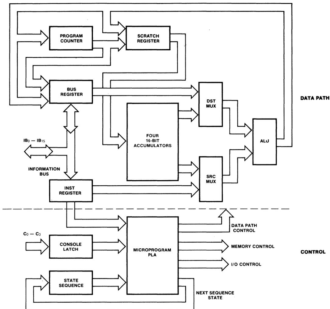
Fig. 1 9440 MICROFLAME CPU Block Diagram
