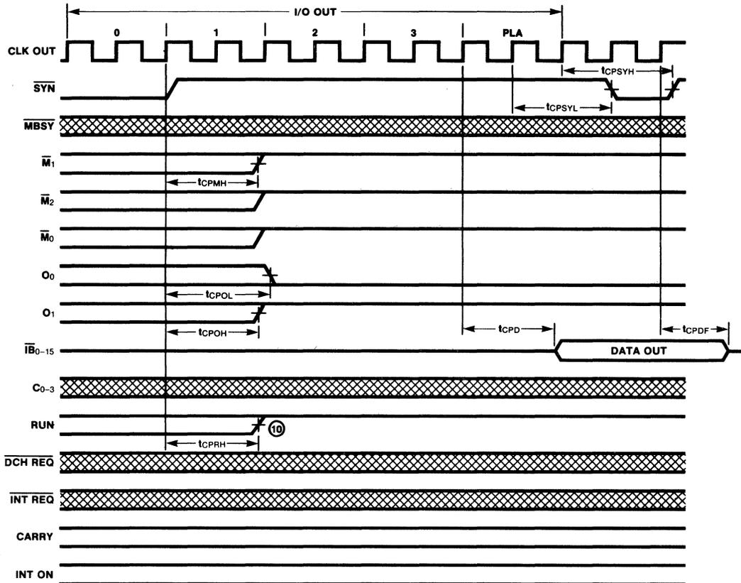
Fig. 12 I/O Out Cycle
