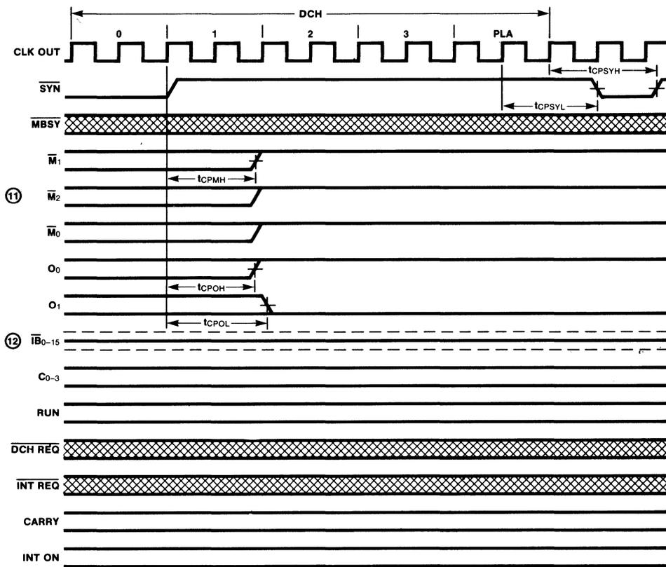
Fig. 15 Data Channel Request Cycle
