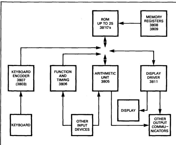
Fig. B-1. PPS-25 Micro-Programmed Processor System
