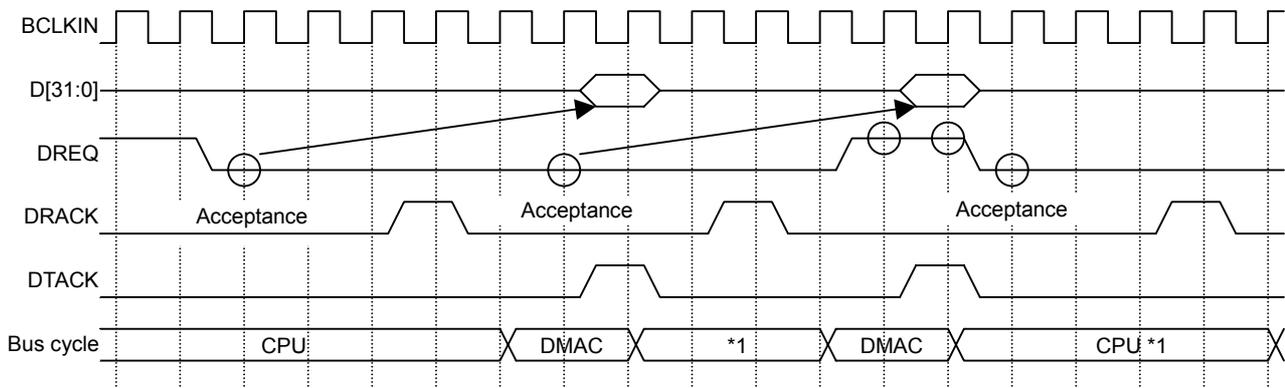
O: DREQ sampling and channel priority determination for SH mode (DREQ = level detection)
