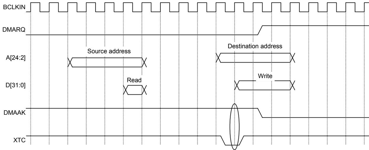
For the MB86290A, the read/write operation is performed according to the SRAM protocol.
