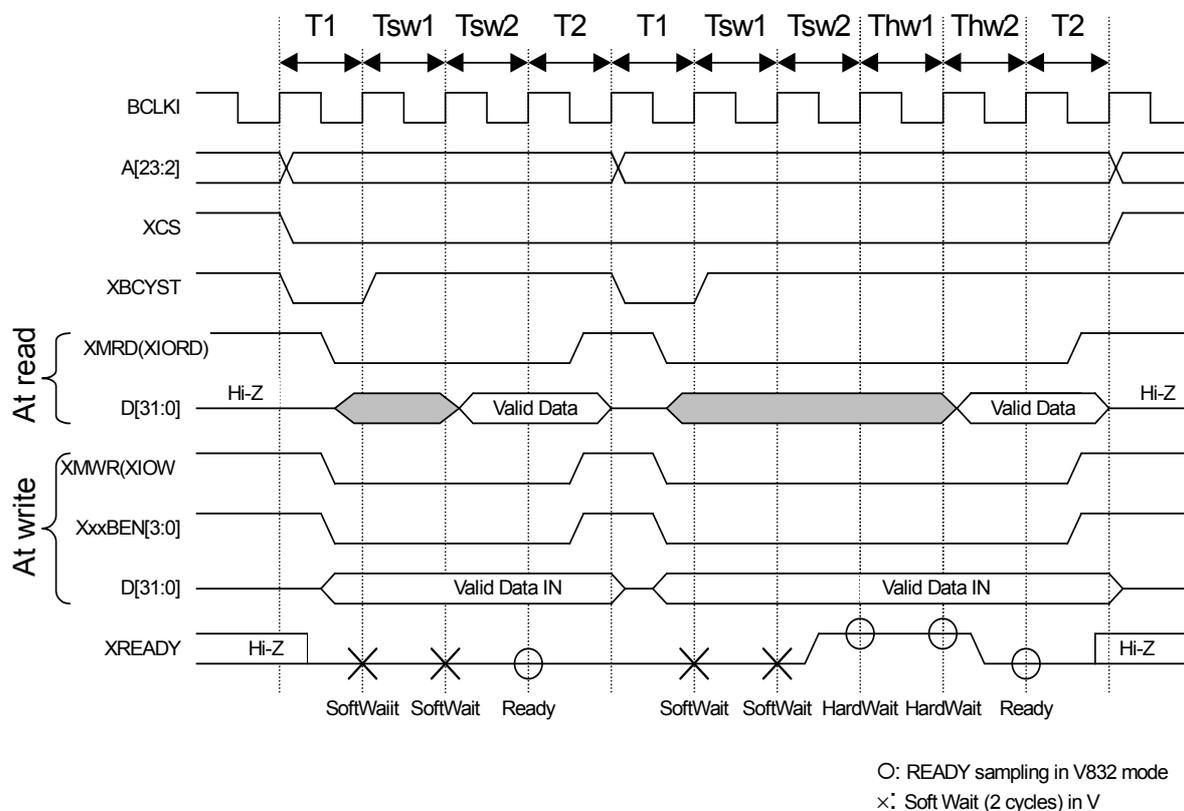
Fig. 11.6 Read/Write Timing Diagram in V832 Mode (Normally Ready Mode)
