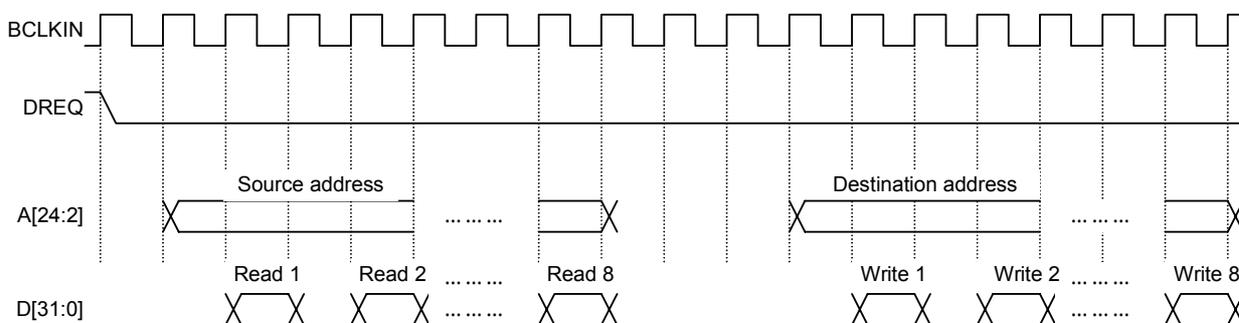
For the MB86290A, the read/write operation is performed according to the SRAM protocol.
