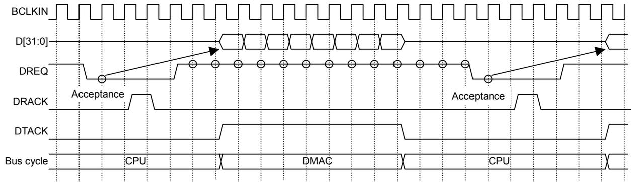
○: DREQ sampling and channel priority determination for SH mode (DREQ = level detection)
