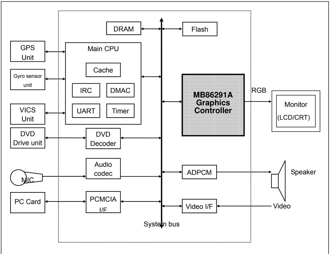
Fig.1.1 System Configuration (TBD)
