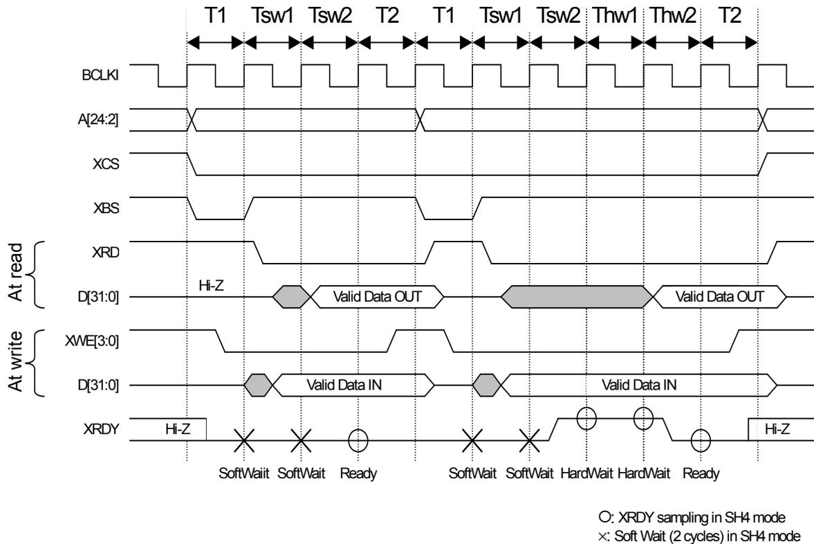
**Fig. 11.4 CPU Read/Write Timing Diagram for SH4 Mode (Normally Ready Mode)**
