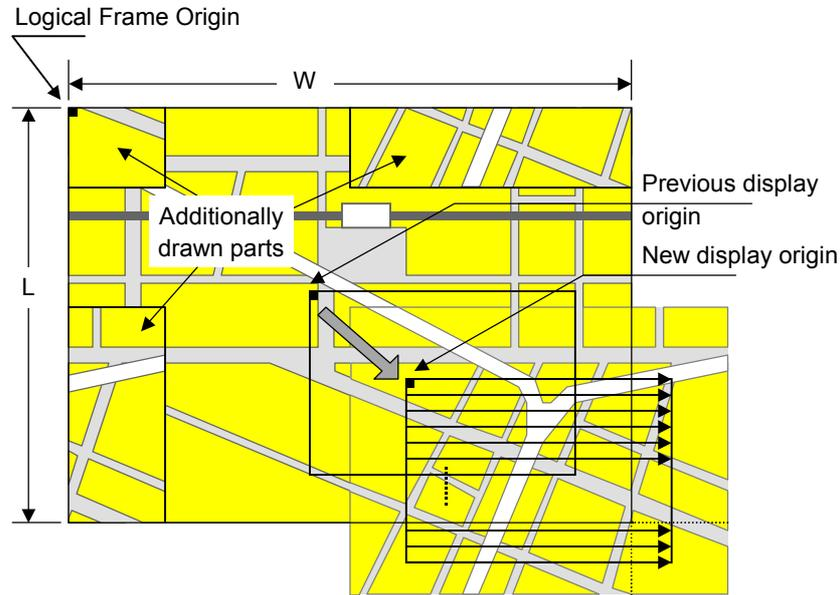
**Fig. 5.3 Wrap Around Management of Display Frame**
