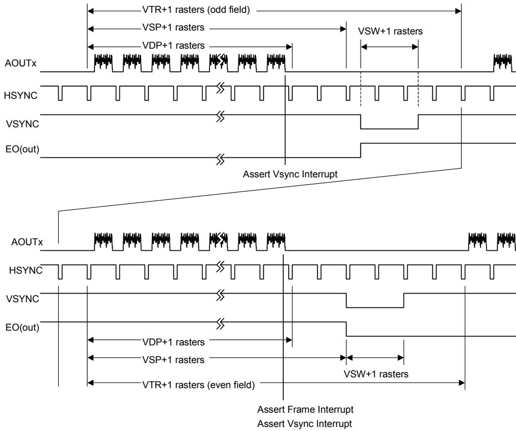
In the above diagram, VTR, HDP, etc., are the settings of their associated registers.
