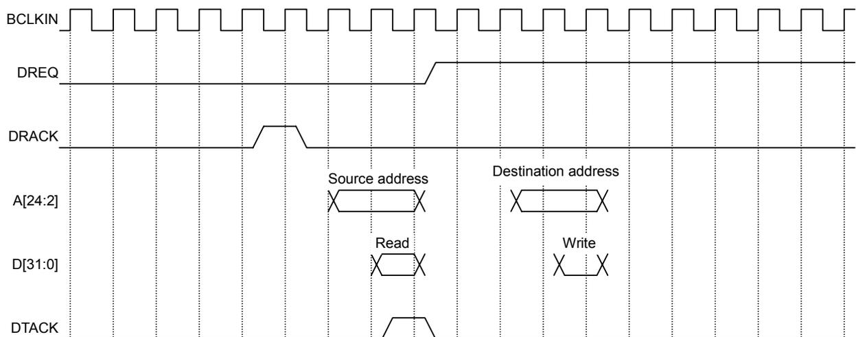
For the MB86290A, the read/write operation is performed according to the SRAM protocol.
