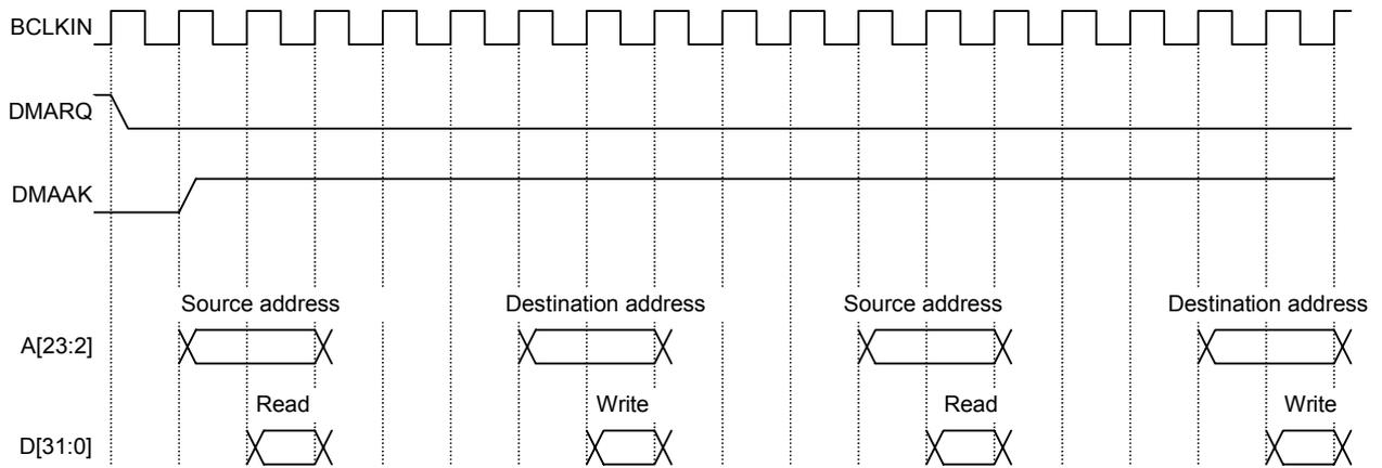
For the MB86290A, the read/write operation is performed according to the SRAM protocol.
