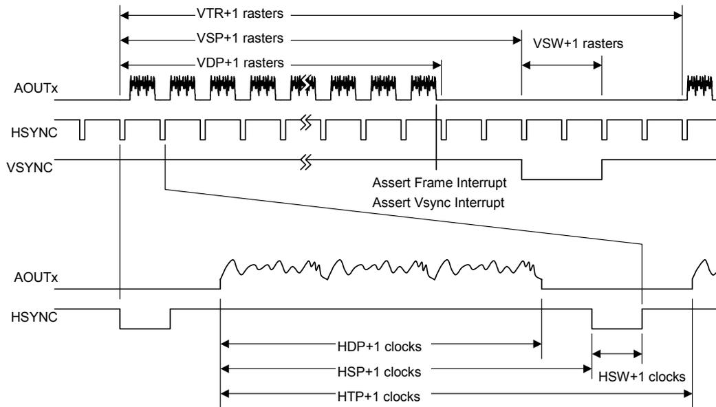
In the above diagram, VTR, HDP, etc., are the settings of their associated registers.
