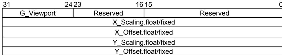
The **G\_Viewport** command sets the “X,Y” scale/offset value used when a normalized device coordinate (NDC) is transformed into a device coordinate (DC).
