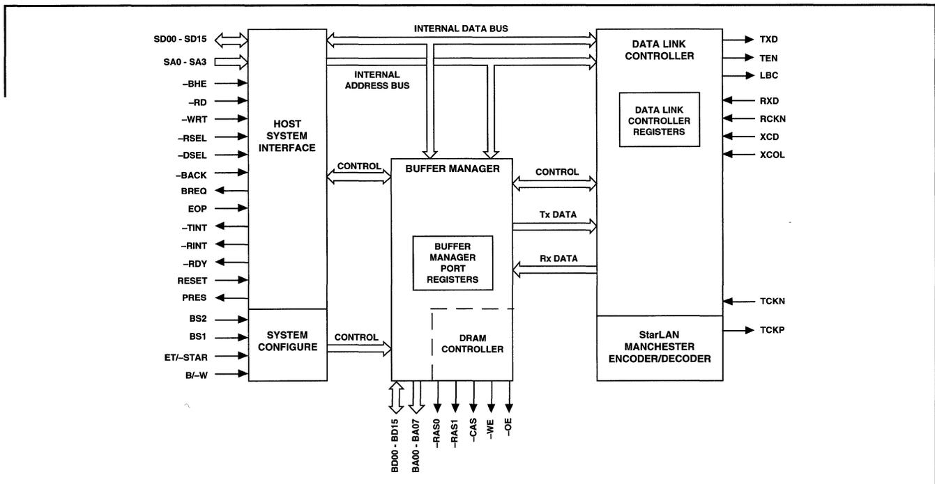
EtherStar Ethernet Controller Block Diagram
