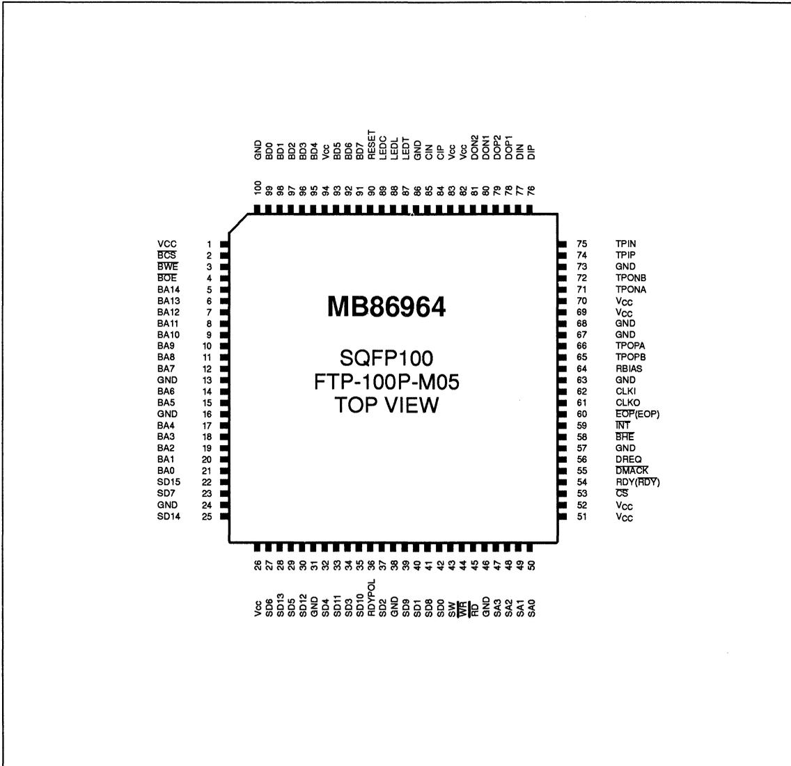
Figure 1. MB86964 Pin Assignments
