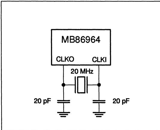
Figure 4. Crystal Oscillator Connection
