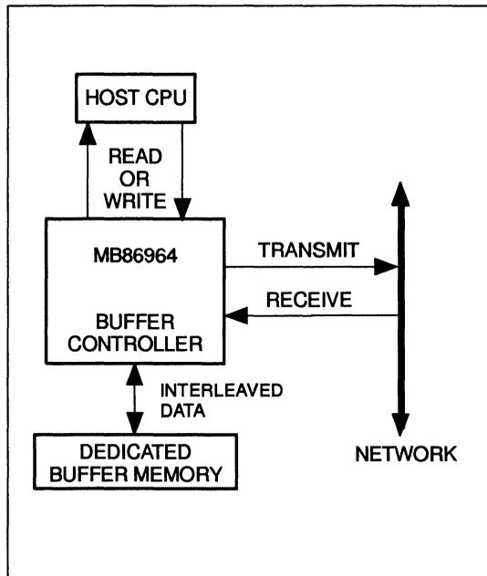
Figure 6. Simultaneous Access to Buffer Memory
