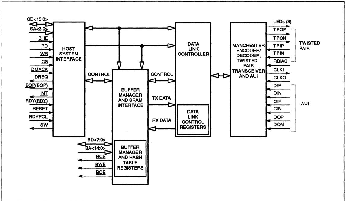
Figure 2. MB86964 Block Diagram
