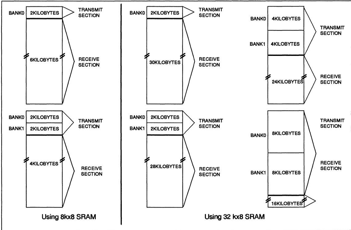
Figure 7. Transmit Buffer Configurations
