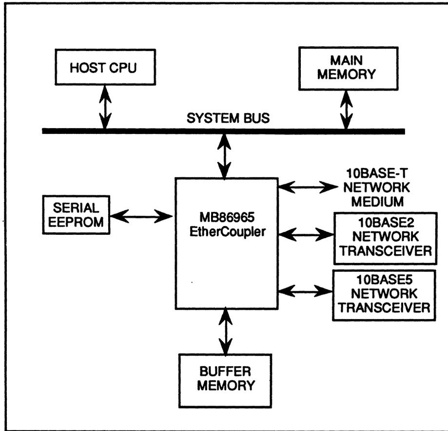
**Figure 3. System Configuration, Simplified Block Diagram**
