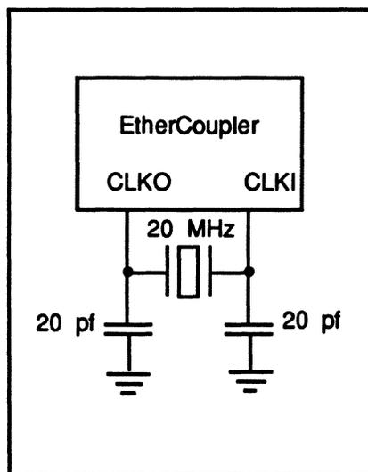
**Figure 4. Crystal Oscillator Connection**
