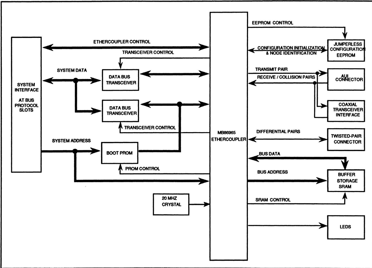
Figure 1. Typical Application, Block Diagram
