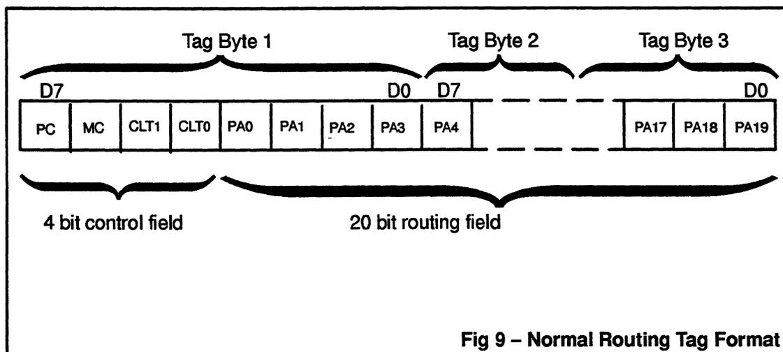
Fig 9 – Normal Routing Tag Format
