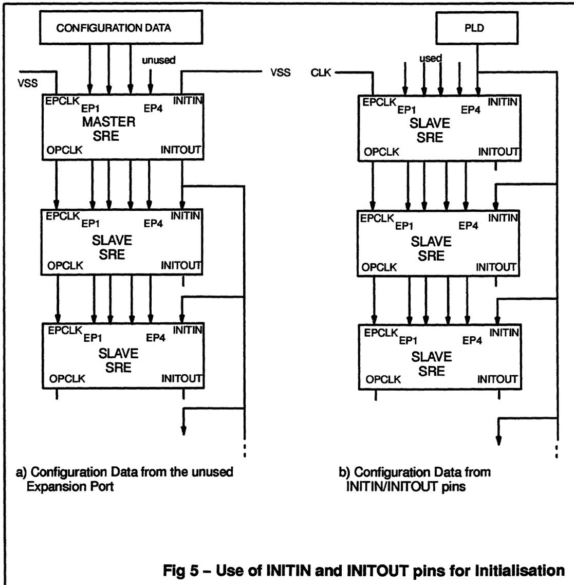
may be internally configured via the data present on Expansion ports 1, 2 & 3.
