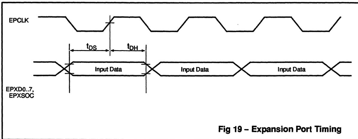
**Fig 19 - Expansion Port Timing**
