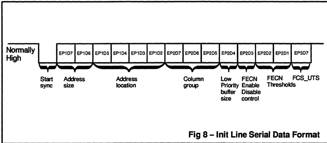
Fig 8 – Init Line Serial Data Format
