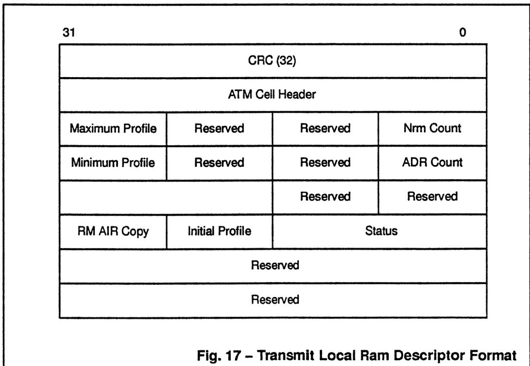
Fig. 17 – Transmit Local Ram Descriptor Format
