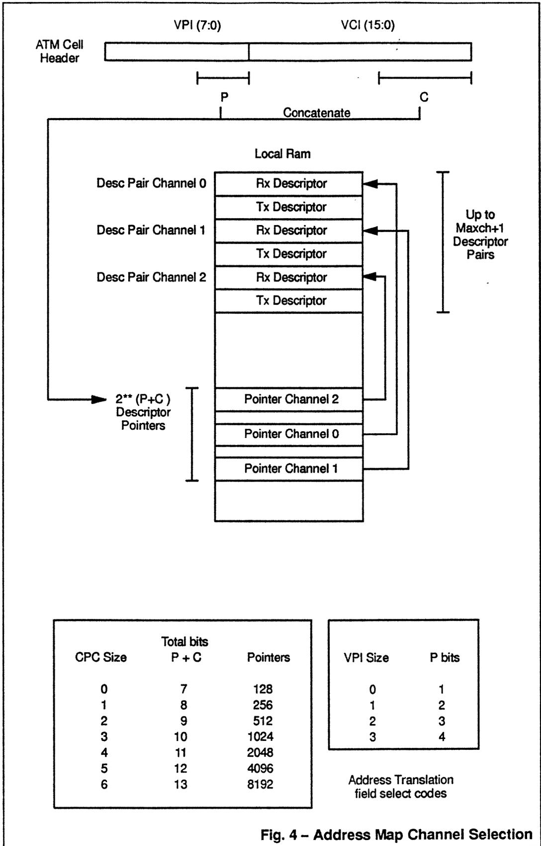
Fig. 4 – Address Map Channel Selection
