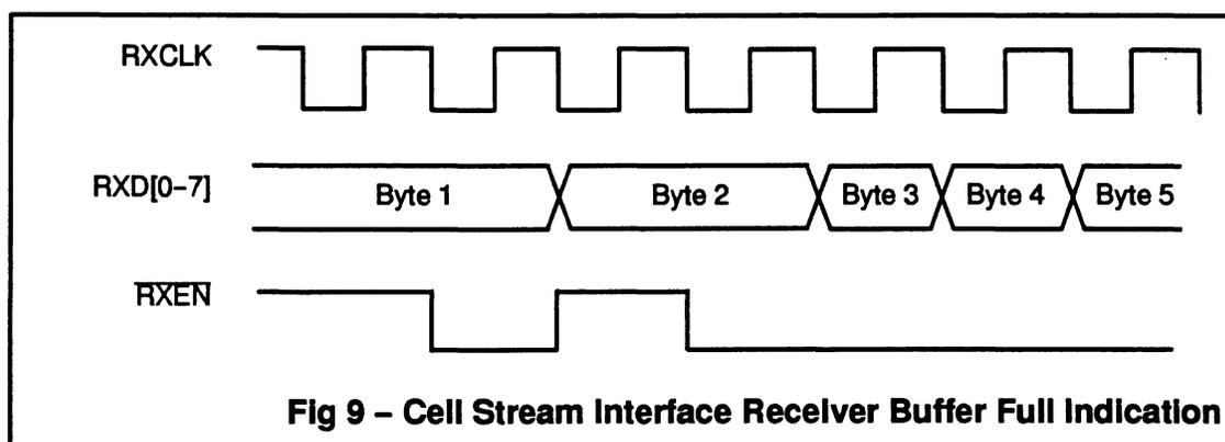
Fig 9 - Cell Stream Interface Receiver Buffer Full Indication
