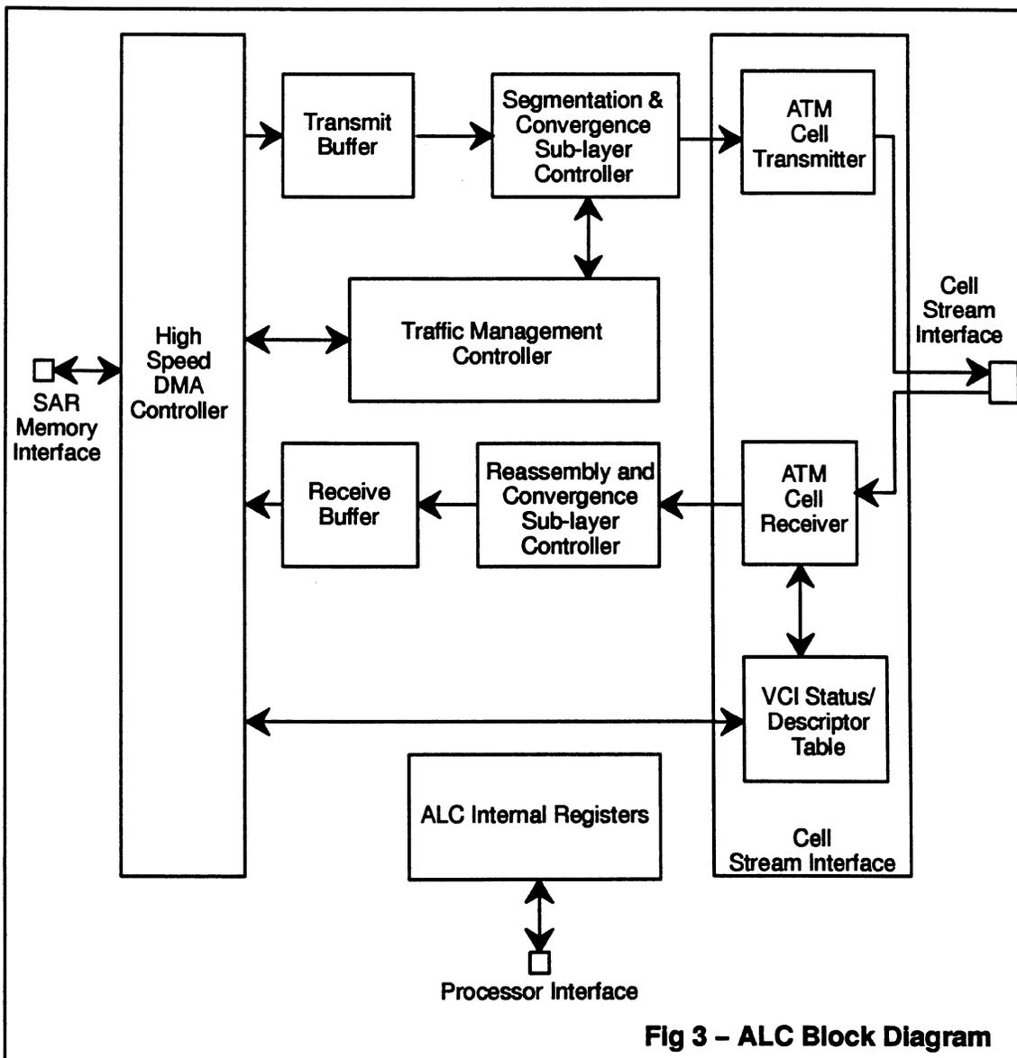
Fig 3 – ALC Block Diagram
