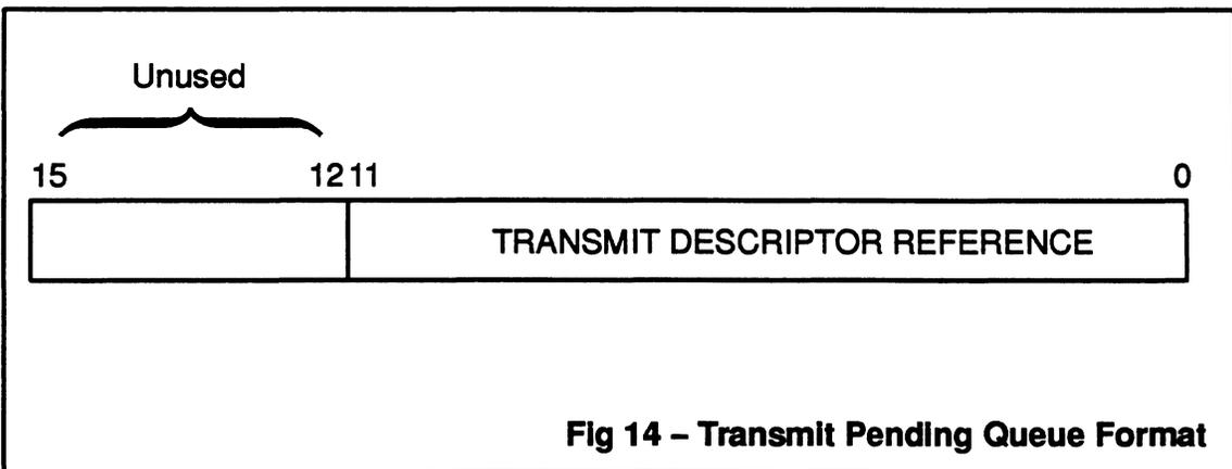
**Fig 14 – Transmit Pending Queue Format**
