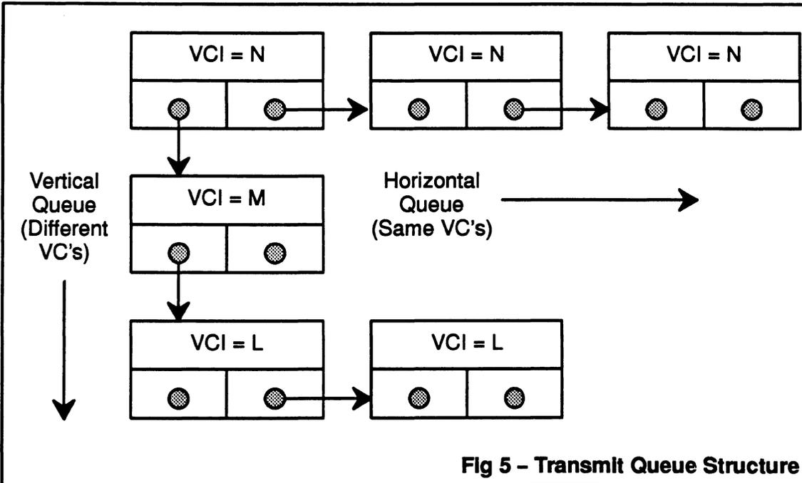
Fig 5 - Transmit Queue Structure
