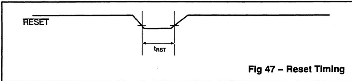
Fig 47 – Reset Timing
