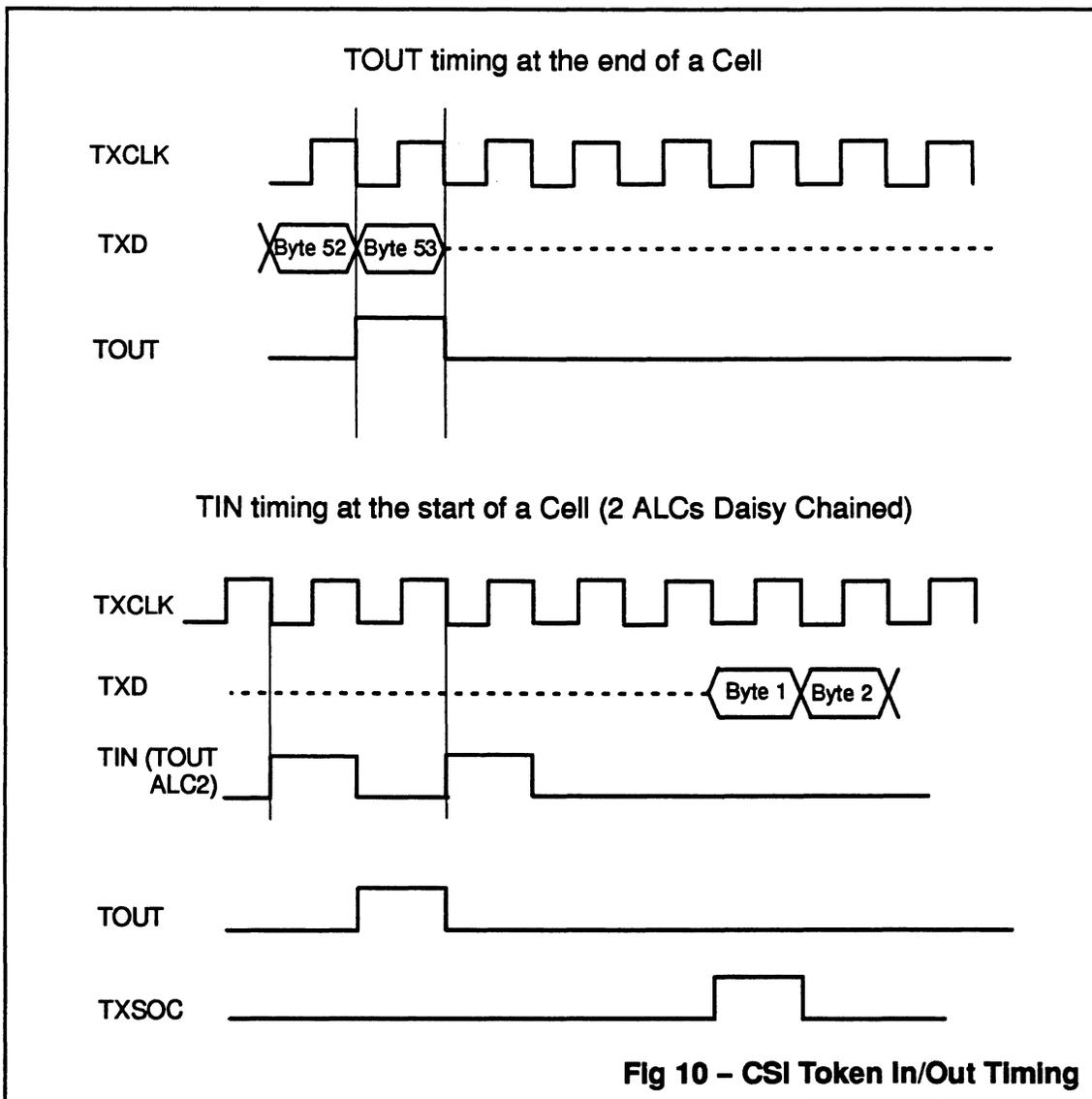
Fig 10 - CSI Token In/Out Timing
