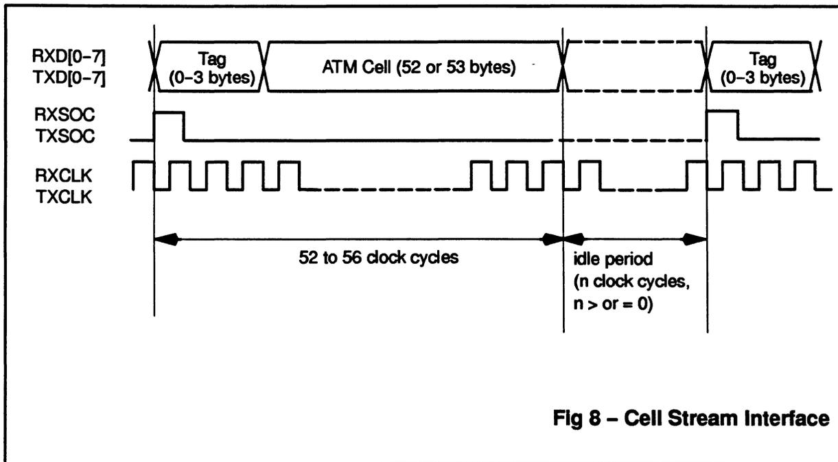
Fig 8 – Cell Stream Interface
