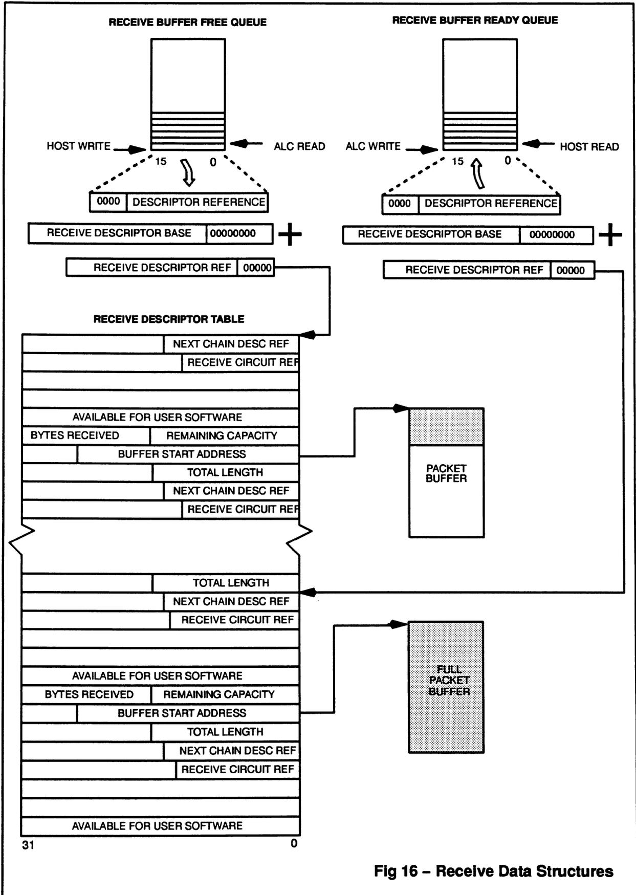
Fig 16 - Receive Data Structures
