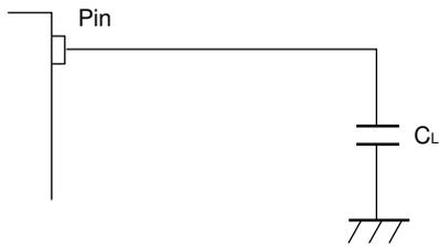
$C_L$  : Load capacitance at testing
