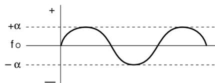
Because the PLL frequency fluctuates around the set frequency with a certain cycle [approximately  $CLK \times (1 \text{ to } 50 \text{ CYC})$ ], the worst value is not maintained for long. (The pulse, if featured with the long period, would produce practically no error.)
