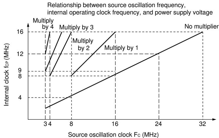
Note: Operation of the evaluation tool is also assured to +2.7 V on the low-voltage side.
