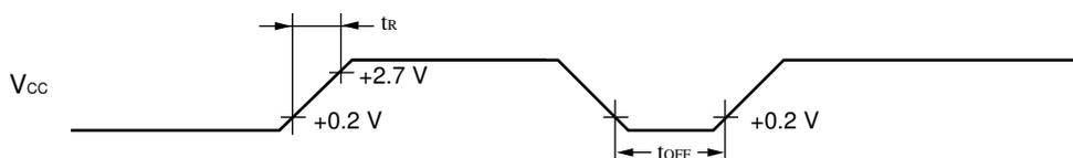
If power supply voltage needs to be changed in the course of operation, a smooth voltage rise is recommended by suppressing the voltage variation as shown below.
