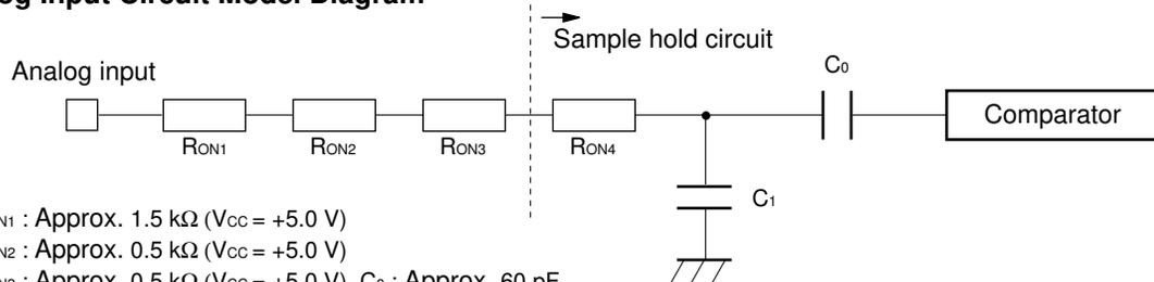
$R_{ON1}$  : Approx. 1.5 k $\Omega$  ( $V_{CC} = +5.0\text{ V}$ )
