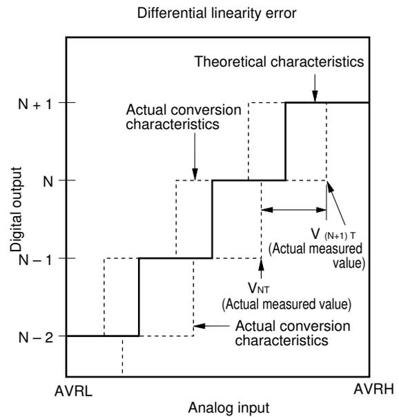
$$\text{Digital output N linearity error} = \frac{V_{NT} - \{1 \text{ LSB} \times (N - 1) + V_{OT}\}}{1 \text{ LSB}} \text{ [LSB]}$$
