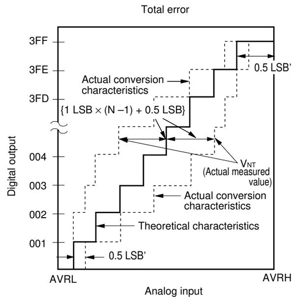
$$1\text{LSB}' = (\text{Theoretical value}) \frac{\text{AVRH} - \text{AVRL}}{1024} [\text{V}]$$
