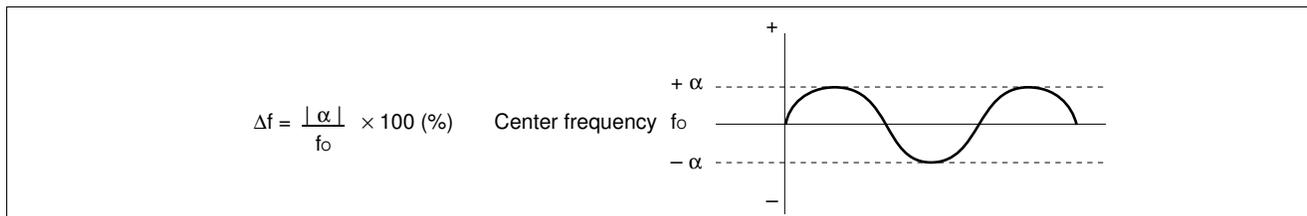
The PLL frequency deviation changes periodically from the preset frequency “(about CLK × (1CYC to 50 CYC))”, thus minimizing the chance of worst values to be repeated (errors are minimal and negligible for pulses with long intervals).
