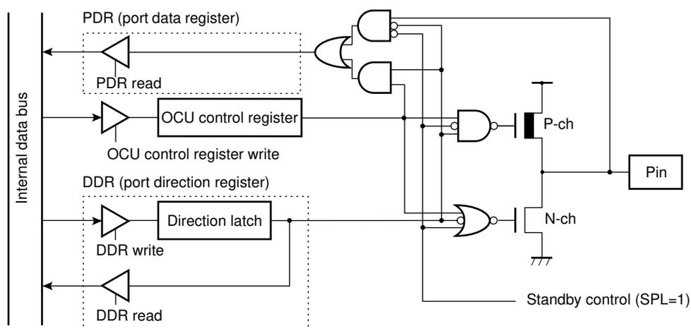
Standby control: Stop, timebase timer mode and SPL=1, or hardware standby mode
