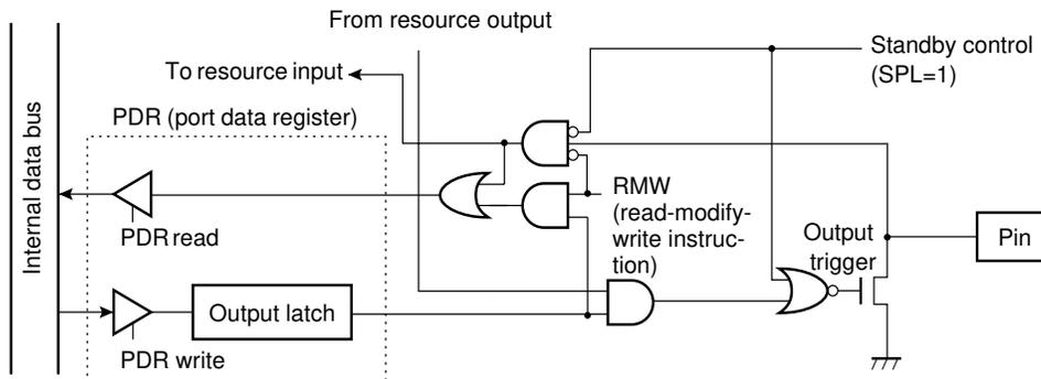
Standby control: Stop, timebase timer mode and SPL=1, or hardware standby mode
