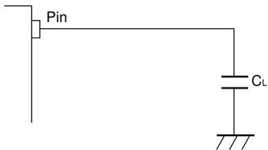
$C_L$  is a load capacitance connected to a pin under test.
