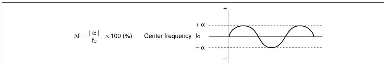
The PLL frequency deviation changes periodically from the preset frequency “(about  $CLK \times (1CYC$  to  $50\text{ CYC})$ ”, thus minimizing the chance of worst values to be repeated (errors are minimal and negligible for pulses with long intervals).
