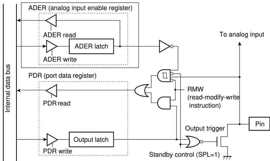
Standby control: Stop, timebase timer mode and SPL=1, or hardware standby mode
