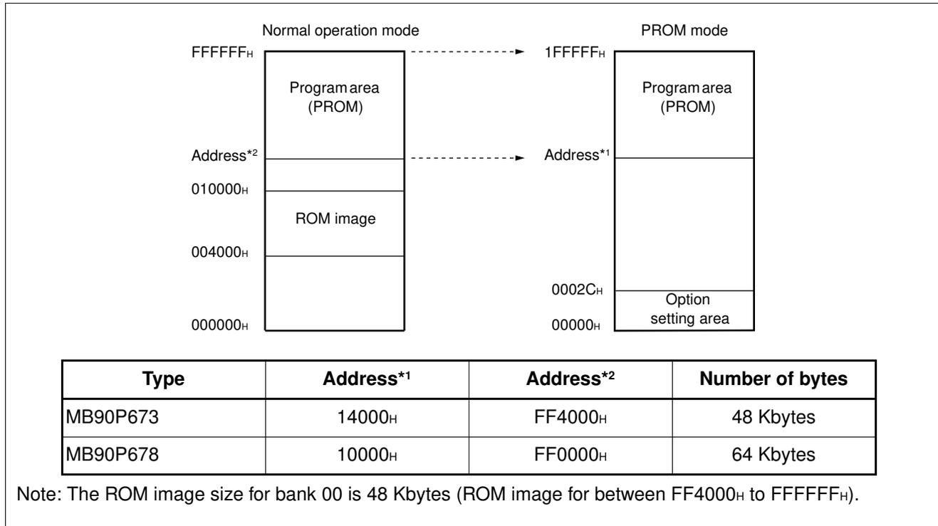
Write data to the one-time PROM microcontrollers according to the following sequence.
