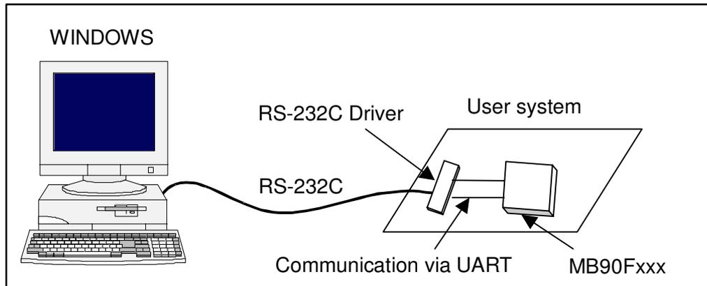
Using RS-232C cable connected to the personal computer (Windows PC), flash memory data in the microcontroller mounted in the user system can be reprogrammed. Note that the user system must have an RS-232C driver for communication with the microcontroller UART.
