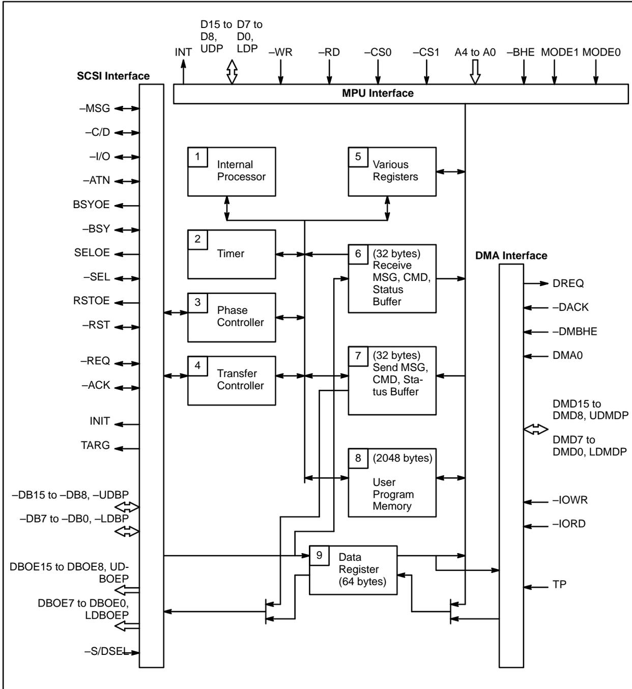
3.2. BLOCK DIAGRAM – PCI Bus Interface Mode
