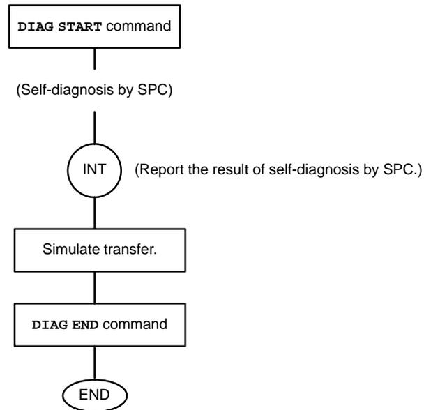
Note: Prior to execution of the **DIAG START** command, set the Bits 6 and 7 of Response Operation Mode Setting Register "disable". Do not execute the **DIAG START** and **DIAG END** command with the bits 6 and 7 enabled or with nexus with the other device established.
