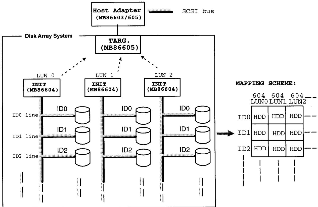
1. IN RAID 5 a block of data is written into one HDD:
