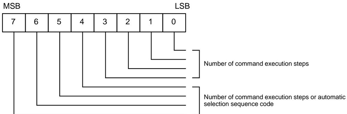
This register indicates the numbers of command execution steps and program steps in the user program. This is an 8-byte FIFO register that holds the command steps corresponding to the interrupt status register.
