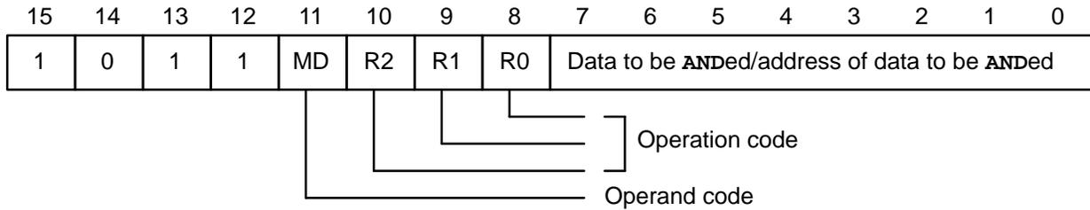
Load the value specified by the operation code to the accumulator and carry out the logical AND between the values indicated by the accumulator and operand. The results are stored in the SPC and can be used for the conditional branch command. The value in the accumulator is unchanged.
