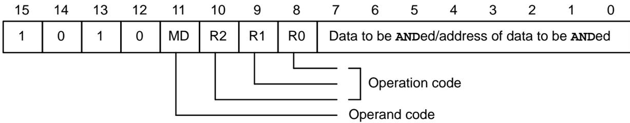
Load the value specified by the operation code to the accumulator and carry out the logical AND between the values indicated by the accumulator and the operand. The results are stored in the accumulator.
