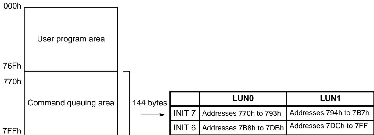
In order to store the received CDBs, set the **RECEIVE CMD** command as the user program command to addresses assigned for each queue.
