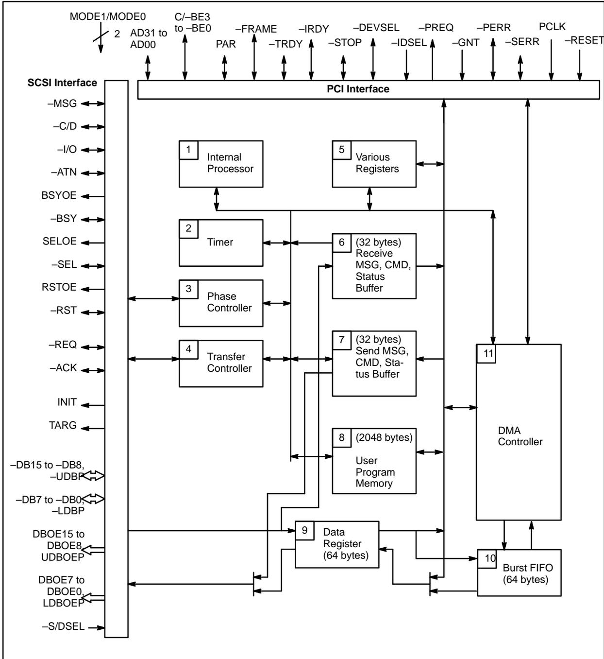
Note : A short bar “-” added to the pin name in the above diagram indicates the active-low signal pin.
