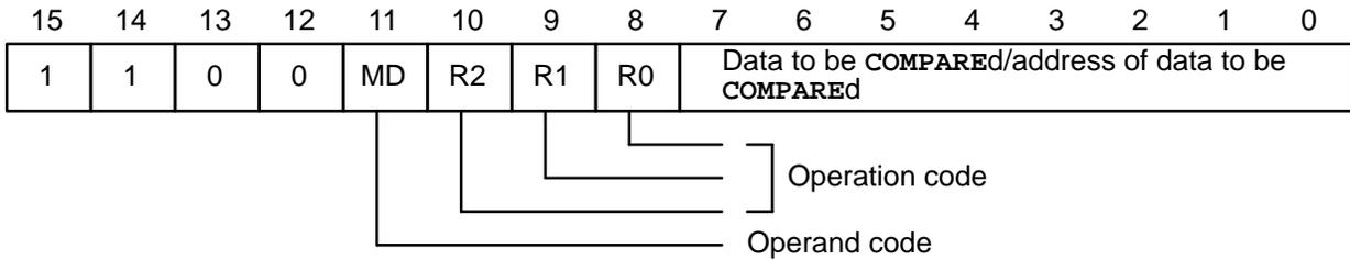
Load the value specified by the operation code to the accumulator and carry out the comparison operation between the values indicated by the accumulator and operand. The results are stored in the SPC and can be used for the conditional branch command. The value in the accumulator is unchanged.
