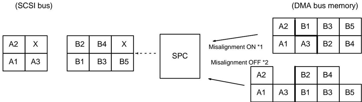
\* 1 : A1 to A3 are transferred by the misalignment OFF and B1 to B5 are by the misalignment ON.
