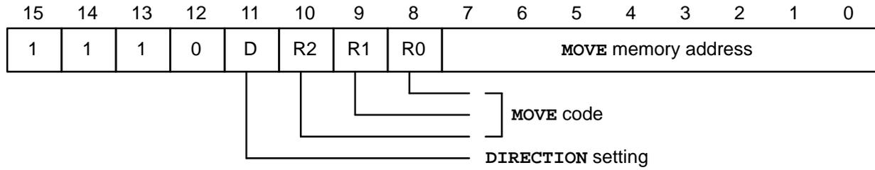
This command copies the value specified by the **MOVE** code to the memory address specified at the operand or the value of the memory address specified at the operand to the accumulator.
