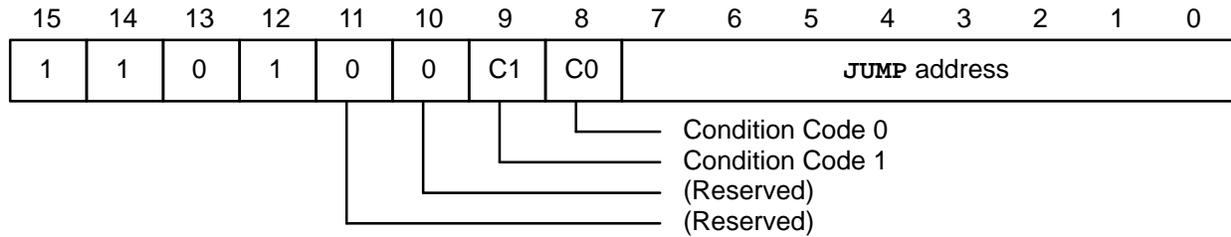
This command is used for conditional or unconditional branches, using the operation results obtained by executing the **COMPARE** and **TEST AND** commands. Even if the SPC is in Level-2 Interrupt Not Report Mode (Bit 1 of Auto Response Mode Setting Register = '1'), the result of the command execution can be found by this conditional branch since the result of command execution is held in the SPC.
