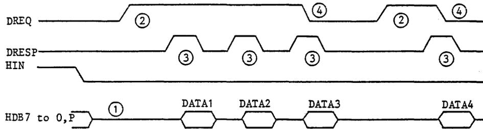
Fig. 5.2.2 Transfer to external data buffer (output operation)
