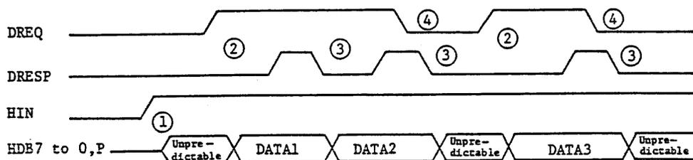
Fig. 5.2.1 Transfer with external data buffer (input operation)
