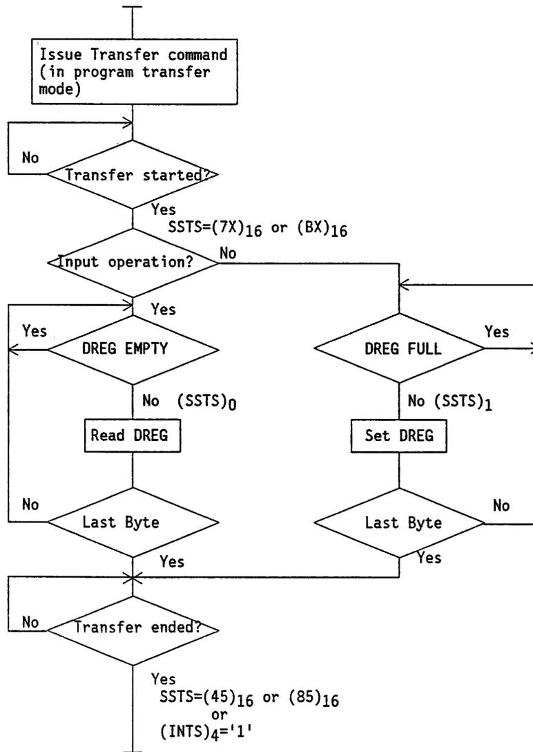
Fig. 4.6.1 DREG access procedure in program transfer mode
