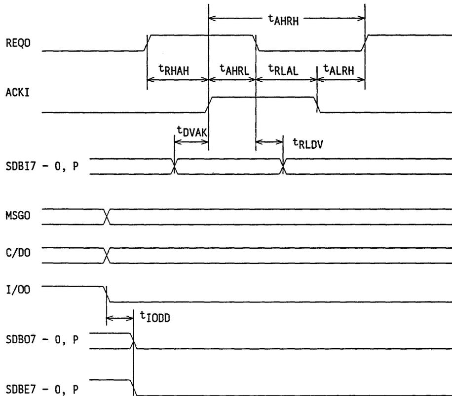
(3) Asynchronous transfer output (INITIATOR)
