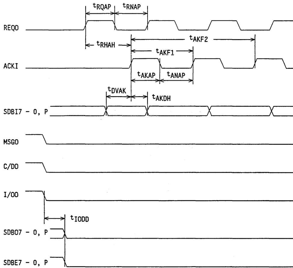
(7) Synchronous transfer Output (INITIATOR)
