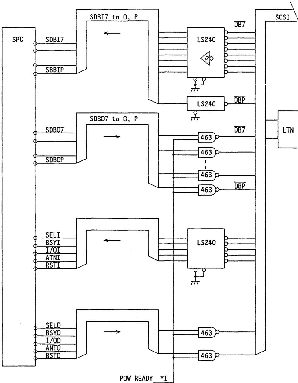
Fig. 5.1.2 Example of single ended type SCSI driver/receiver circuit
