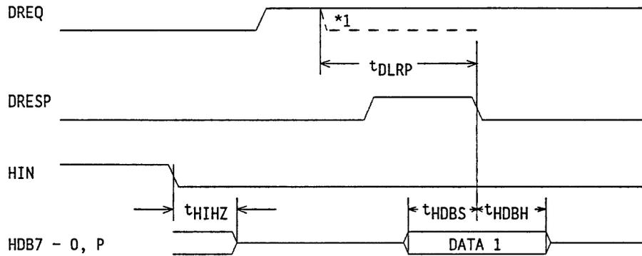
\*1 In the following cases, the DREQ signal becomes inactive asynchronously with the DRESP signal to stop refetching data during an output operation:
