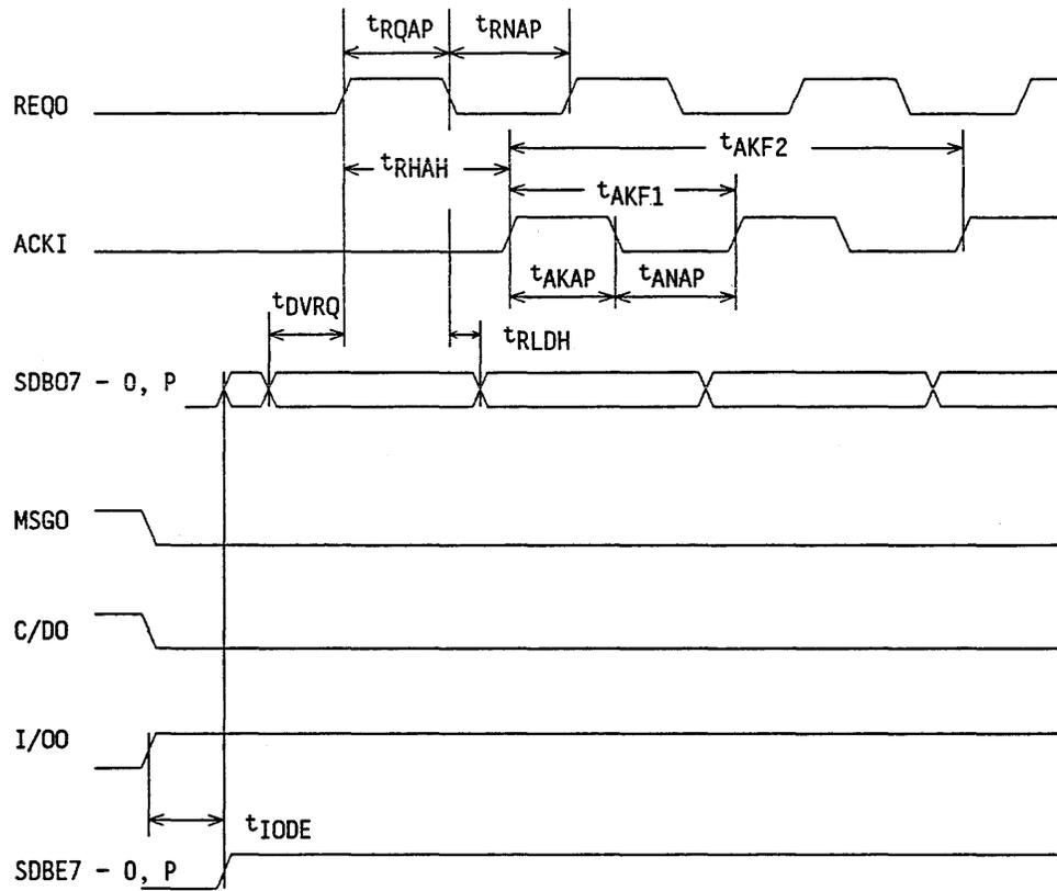
(6) Synchronous transfer input (TARGET)
