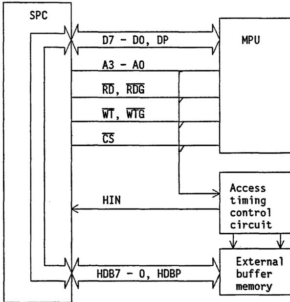
Fig. 4.14.1 Access from MPU to external buffer memory
