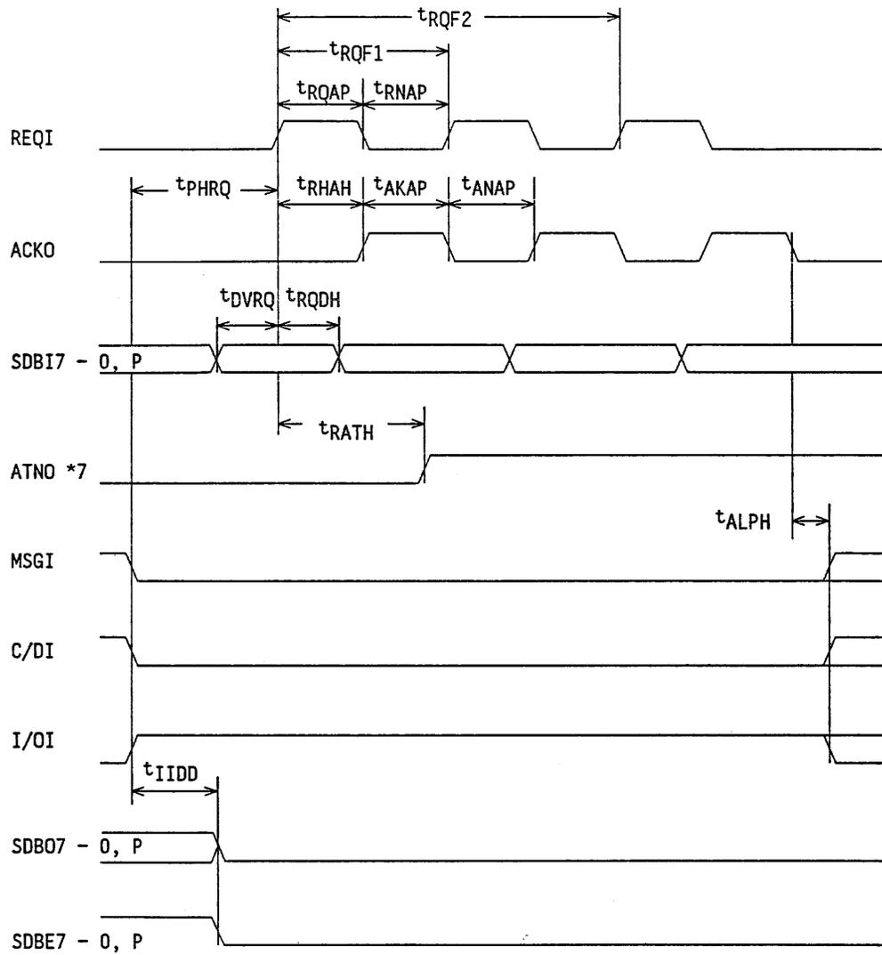
(8) Synchronous transfer input (INITIATOR)
