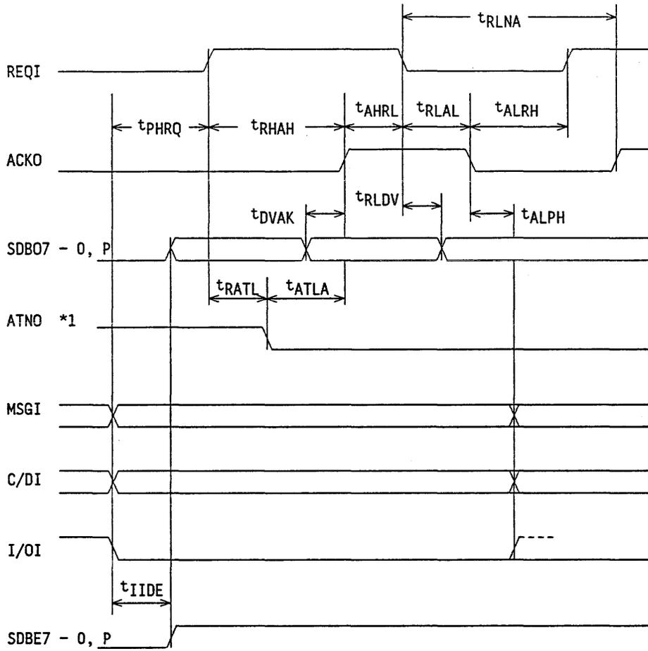
(4) Asynchronous transfer input (INITIATOR)
