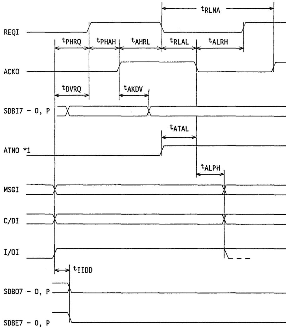
(5) Synchronous transfer output (TARGET)
