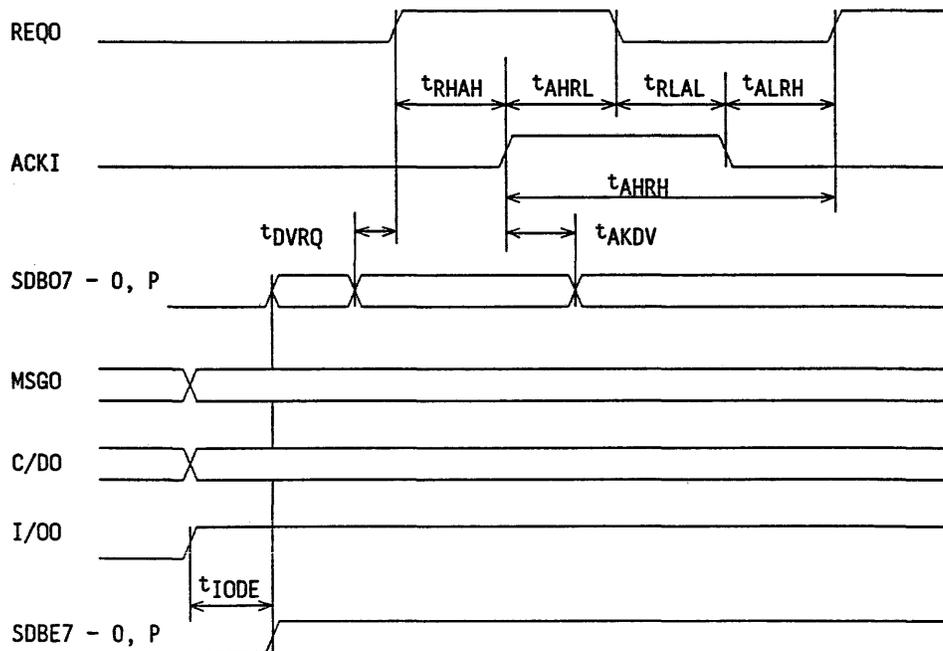
(2) Asynchronous transfer input (TARGET)
