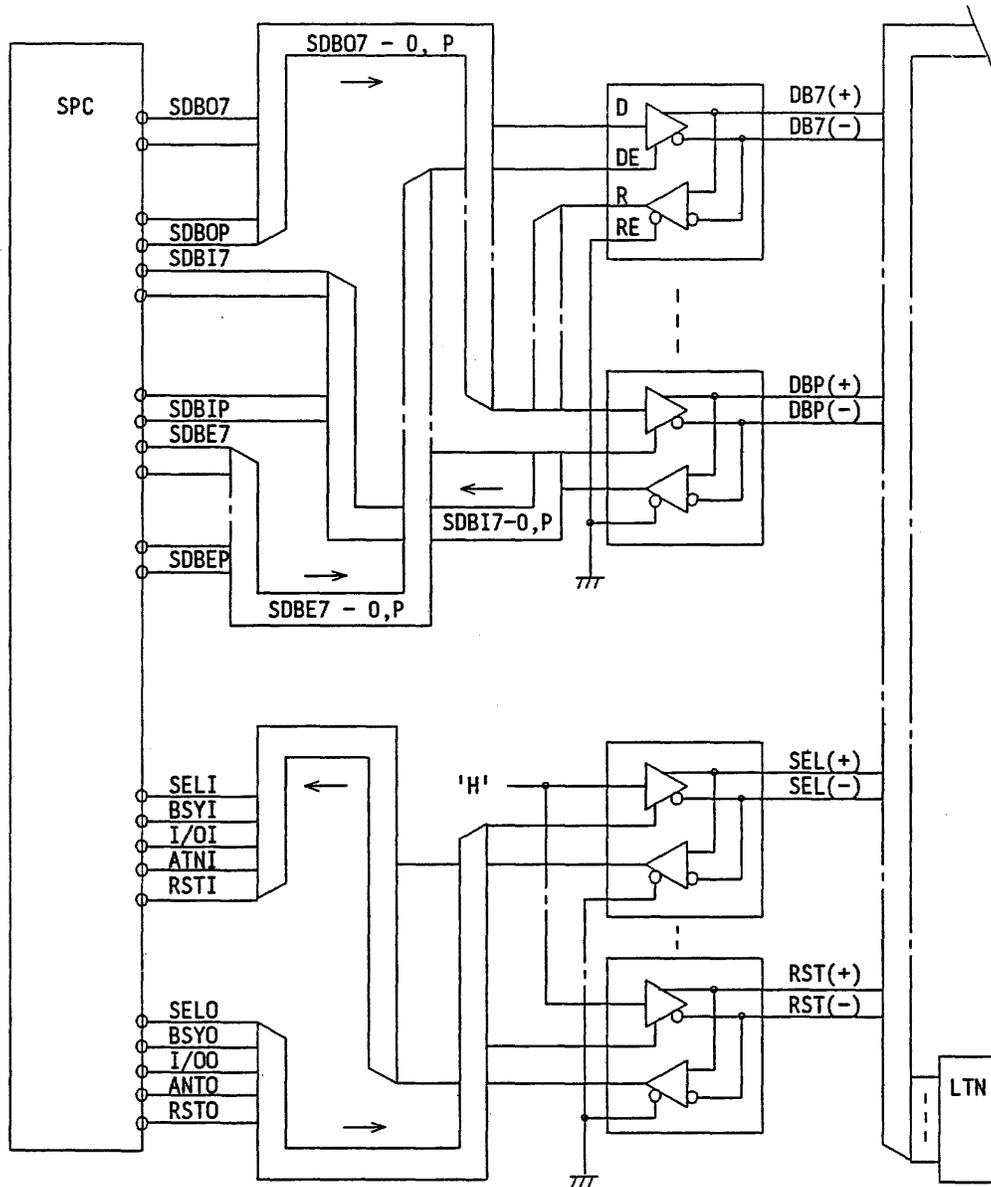
Fig. 5.1.3 Example of differential type SCSI driver/receiver circuit
