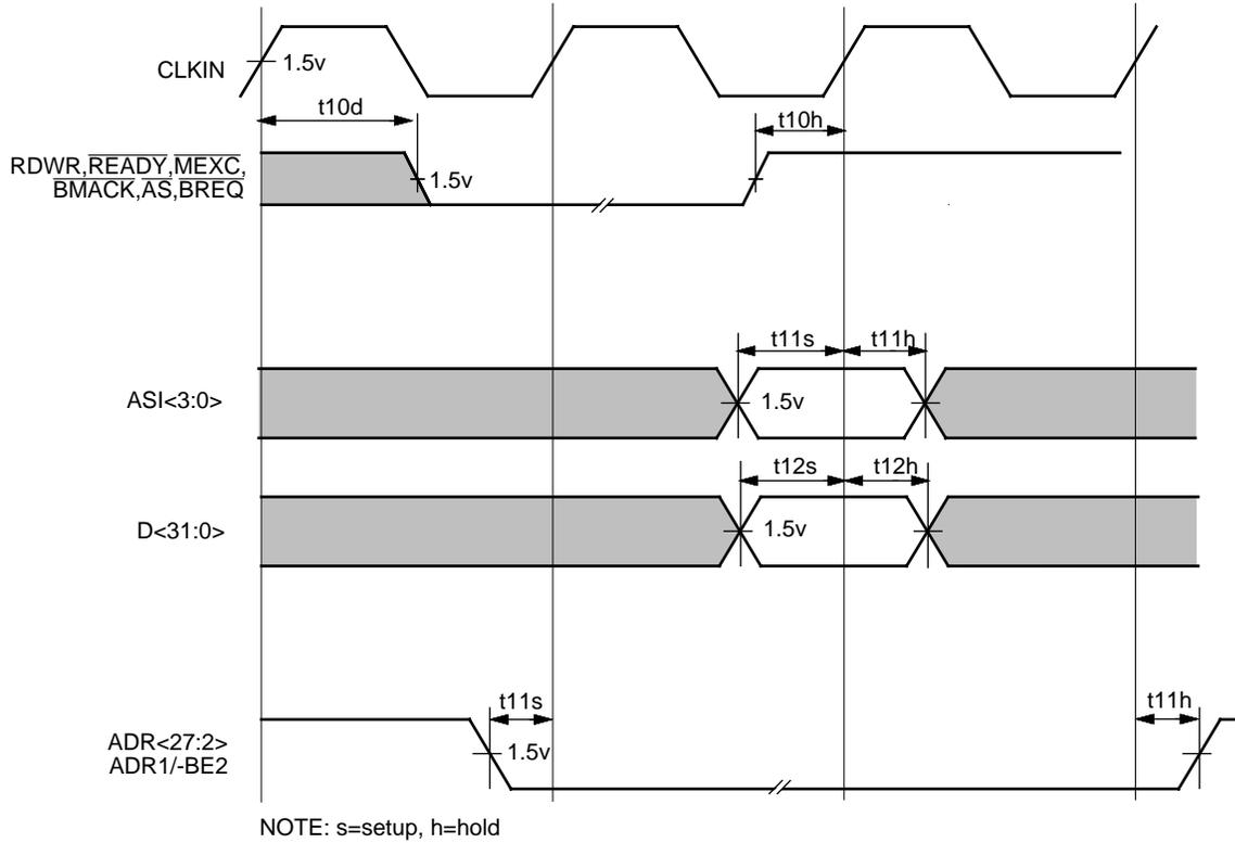
Figure 32. I/O Input Timing
