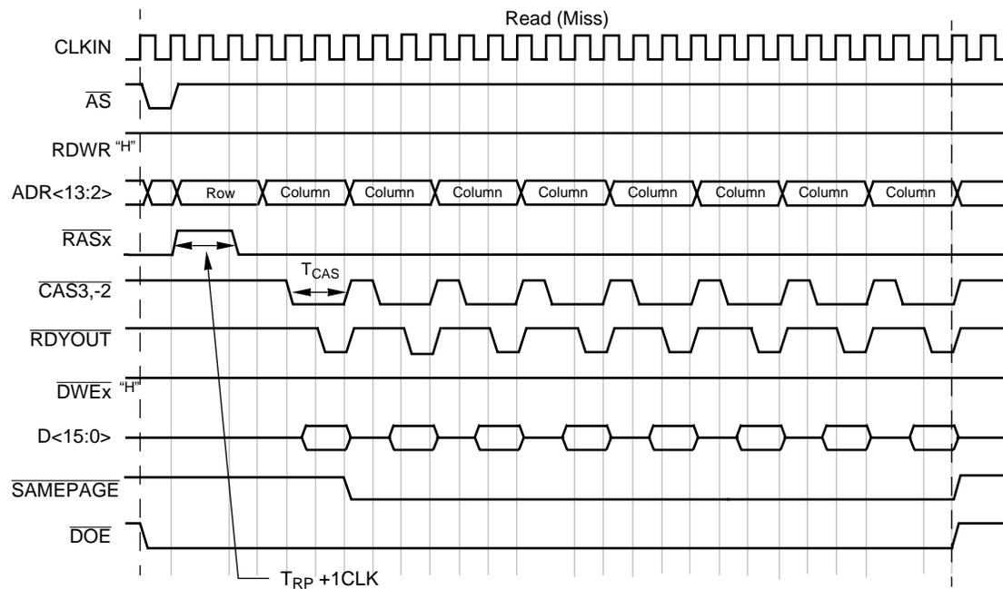
Figure 24. DRAM Controller Enabled, DRAM Burst Enabled, 16-Bit Page Mode Read Timing 1
