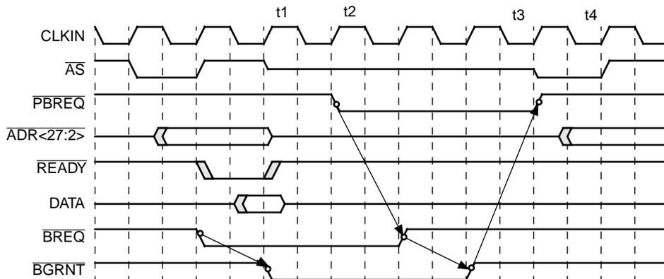
Figure 28. Example of  $\overline{\text{PBREQ}}$  Timing
