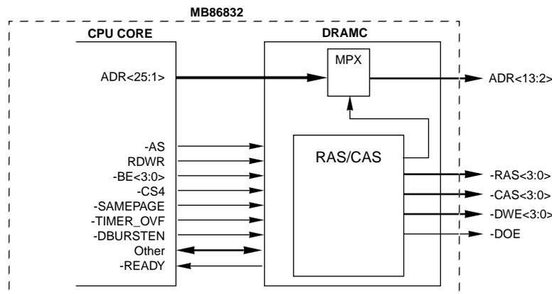
Figure 6. DRAM Controller Configuration
