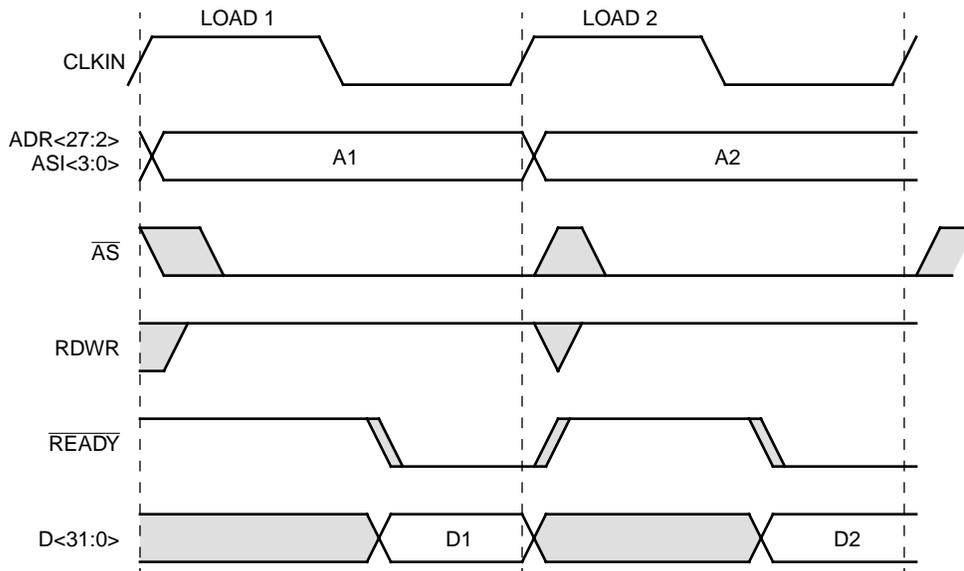
**Figure 7. Typical Back-to-Back Loads (Same as Load Double)**
