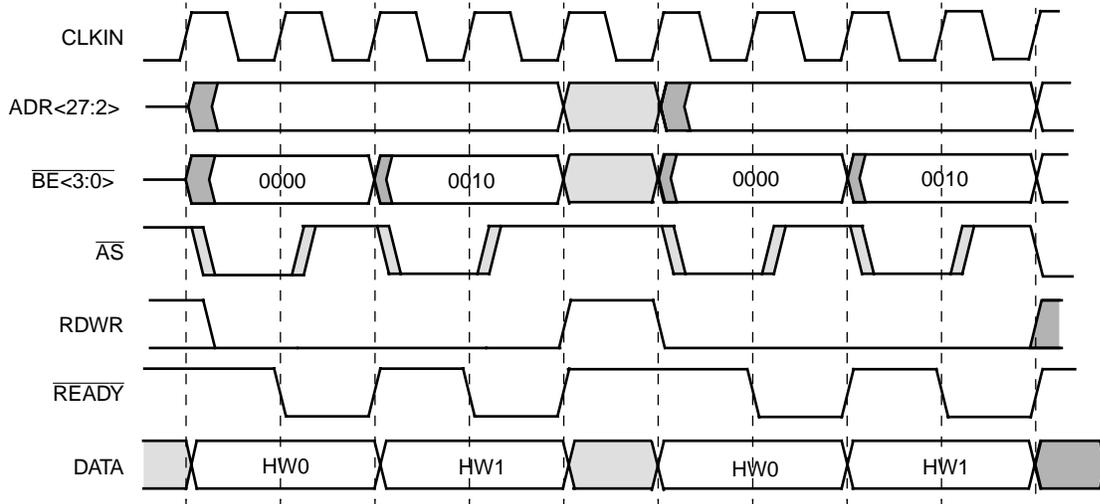
Figure 18. 16-Bit Bus Mode (1 Wait State) for Word Write
