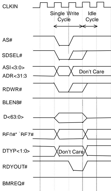
Figure 7-13<sup>2</sup> Single Writes in SDRAM Transparent Access
