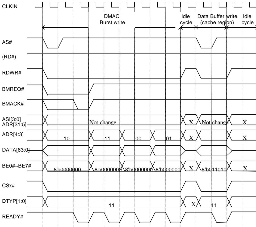
Figure 7-10 SPARClite Bus Burst WRITE Operation
