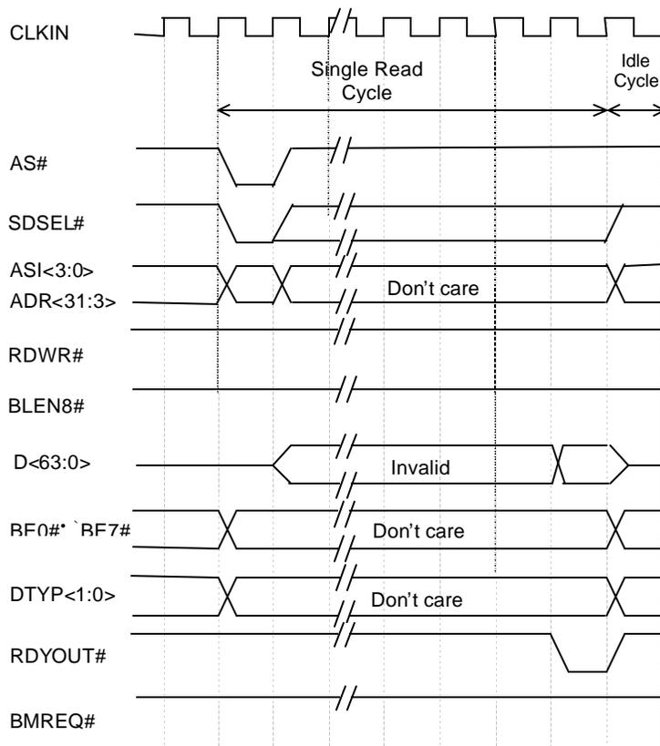
Figure 7-12 Single Reads in SDRAM Transparent Access
