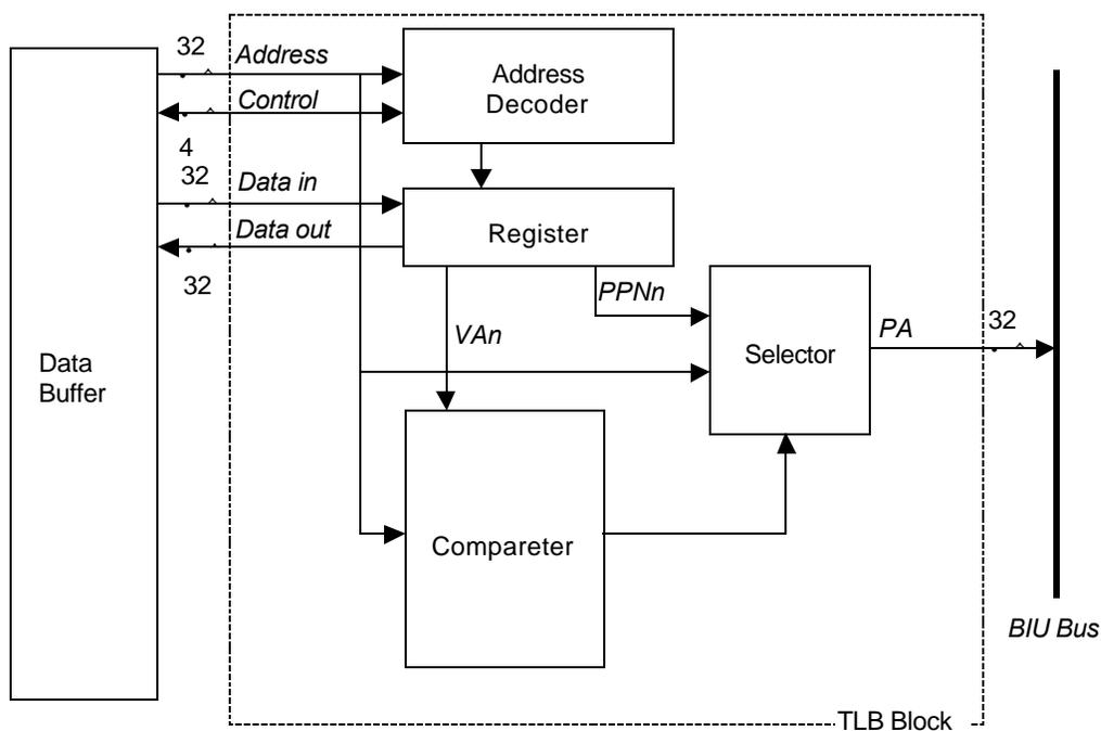
Figure 5-1 TLB Block Diagram
