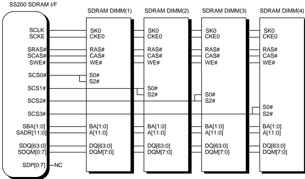
**Figure 8-5 Connect to MB8686 SDRAM I/F**
