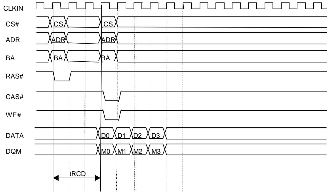
On the Registered SDRAM DIMM, Control Signals, which are CS,BA,ADR,RAS,CAS,WE and DQM, are delayed with 1 cycle and Data Input to SDRAM DIMM also needs to be delayed with 1 cycle.
