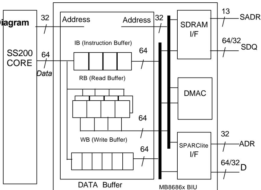
**Figure 1.1 MB8686x Processor Block Diagram**
