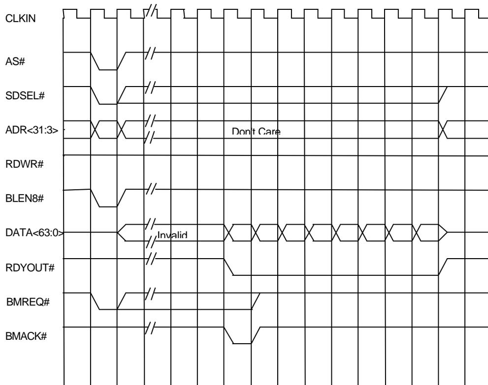
**Figure 7-14 Burst Reads in SDRAM Transparent Access (Burst Length 8)**
