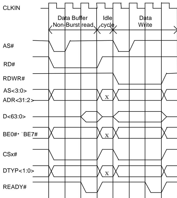
Figure 7-8 SPARClite Single Read/Write Operation
