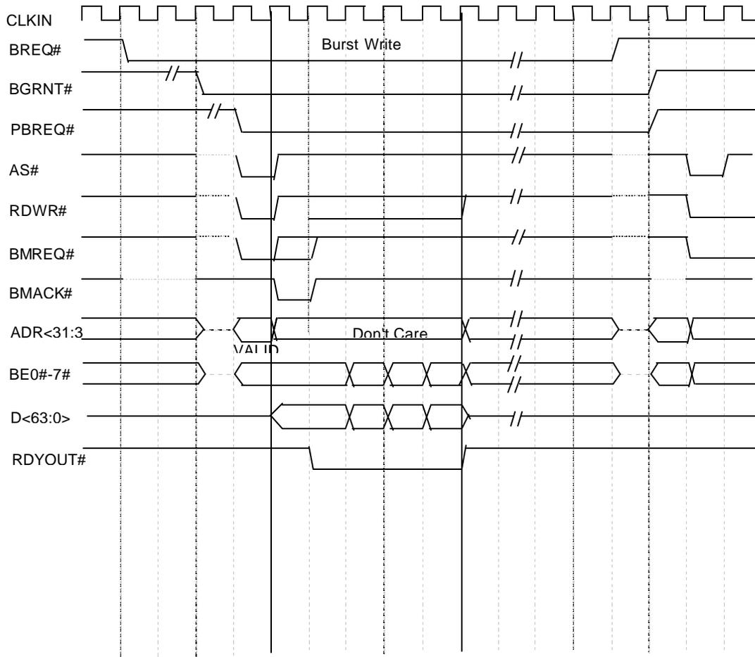
Figure 7-11 SPARClite Bus Open and Reopen
