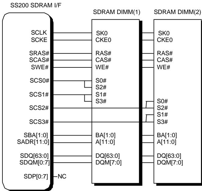
**Figure 8-6 Connect to MB8686x SDRAM**
