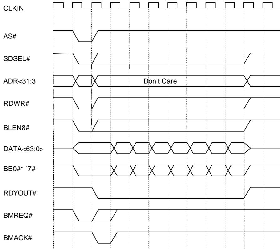
**Figure 7-15 Burst Writes in SDRAM Transparent Access (Burst Length 8)**
