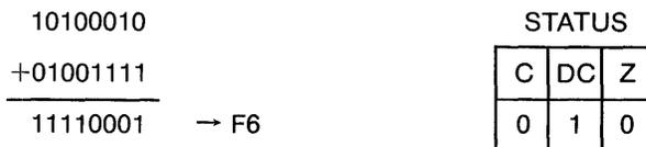
The Carry bit is reset, indicating no overflow (sum of 8-bit values in W register and file register  $\leq 255$ ). The Digit Carry bit is set indicating a digit overflow (sum of 4 LSB's in W register and file register  $> 15$ ). The Zero bit is reset, indicating that the result of the addition has not provided an 8-bit value of zero.
