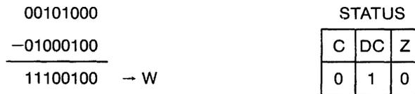
The Carry bit is reset, indicating an overflow (absolute value in the W register is greater than absolute value in F17). The Digit Carry bit is set, indicating no digit overflow.
