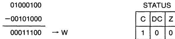
The Carry bit is set, indicating no overflow (absolute value in W register not greater than absolute value in F17). The Digit Carry bit is reset, indicating a digit-overflow (absolute value of 4 LSB's of F17 greater than absolute value of 4 LSB's of W Register).
