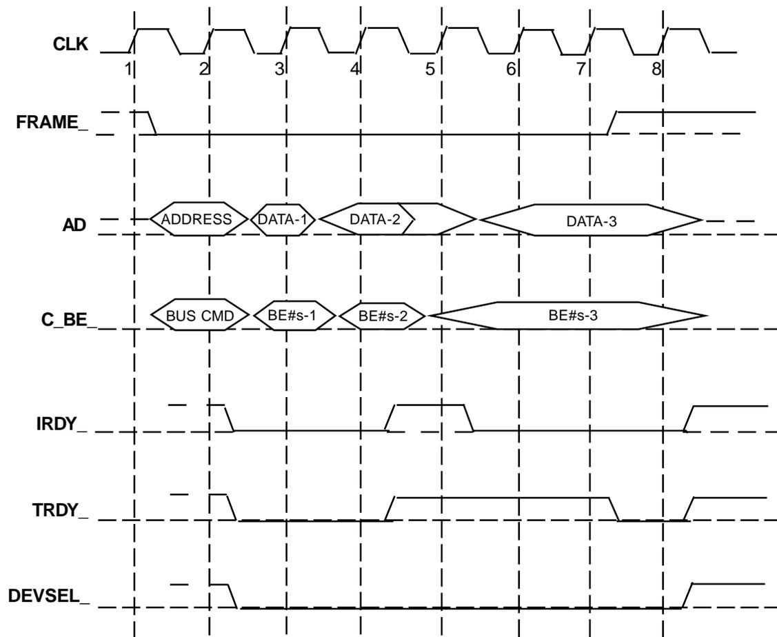
**\*Notes:** The transaction starts when **FRAME\_** is asserted for the first time which occurs on clock 2. A write transaction is similar to a read transaction except no turnaround cycle is required following the address phase because the master provides both address and data. Data phases work the same for both read and write transactions.
