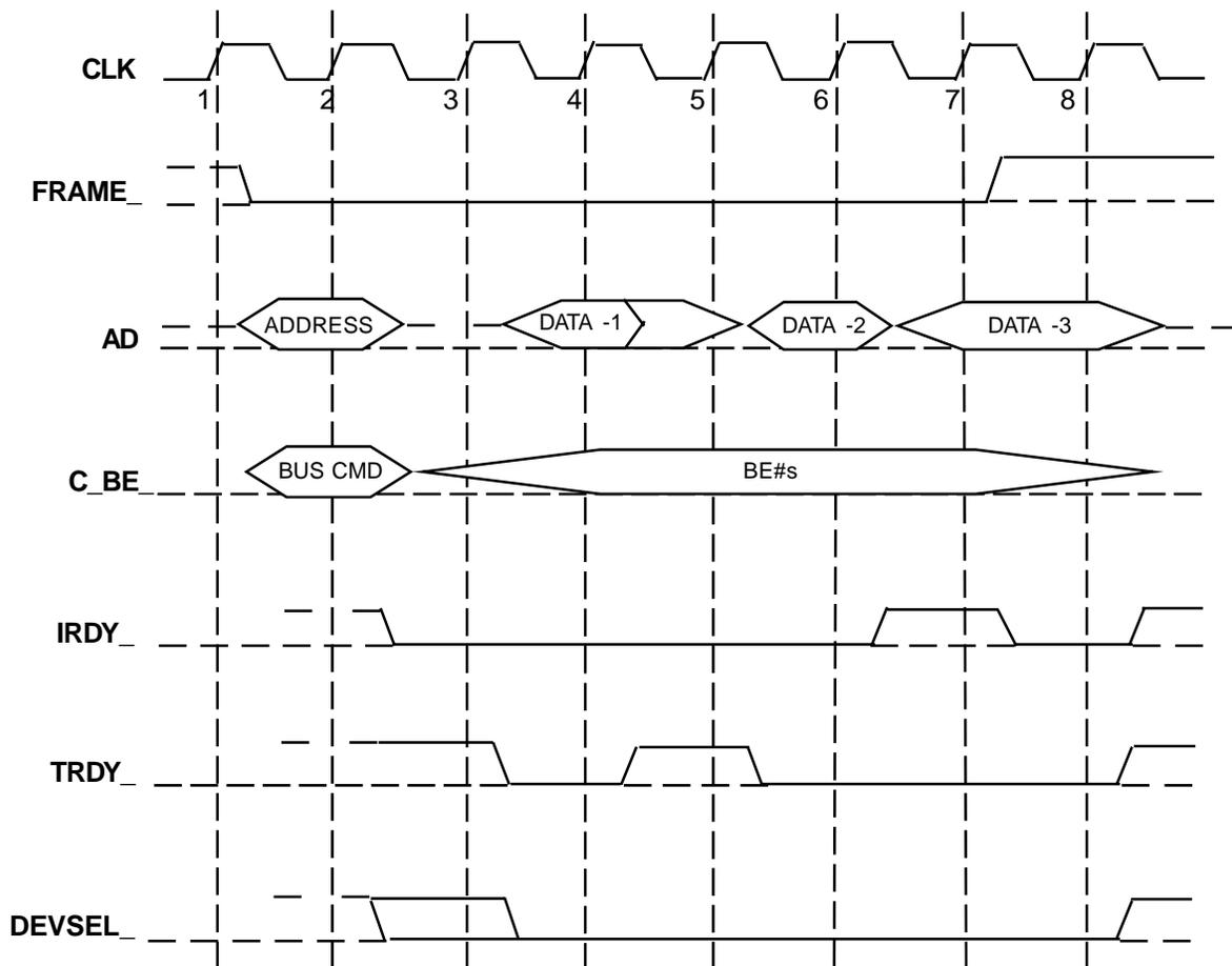
**\*Notes:** The transaction starts with an address phase which occurs when **FRAME\_** is asserted for the first time and occurs on clock2. During the address phase, **AD[31:0]** contain a valid address and **C\_BE\_[3:0]** contain a valid bus command.
