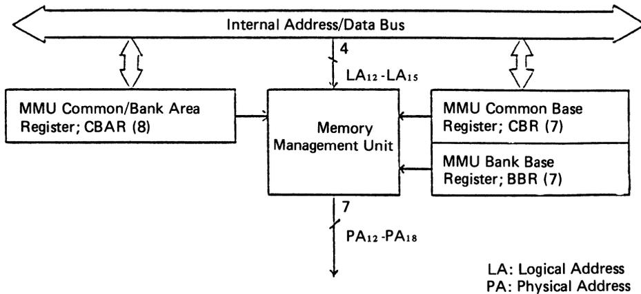
**Figure 2.6.3 MMU Block Diagram**
