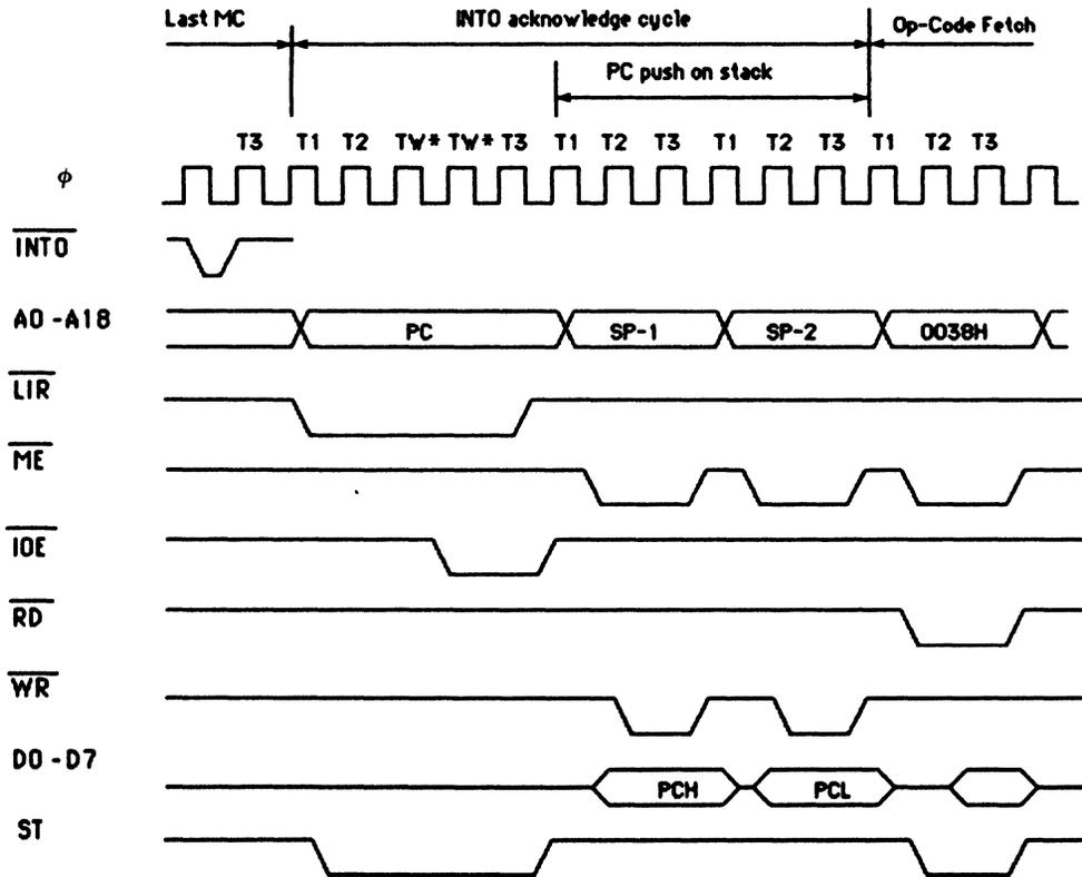
**Figure 2.7.7 INTO Mode 1 Timing**
