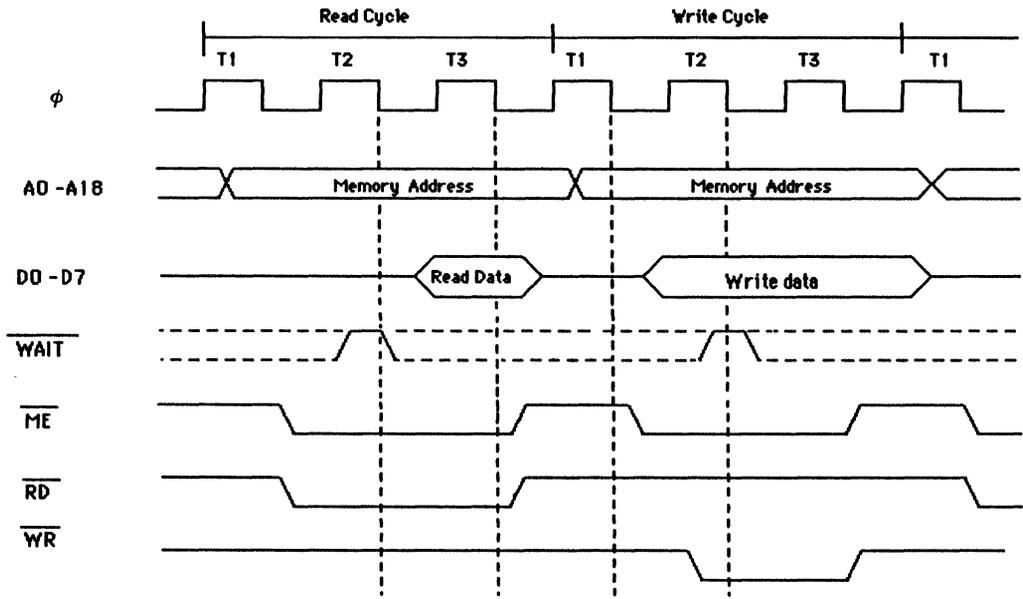
**Figure 2.2.3 Memory Read/Write Timing (without wait state)**
