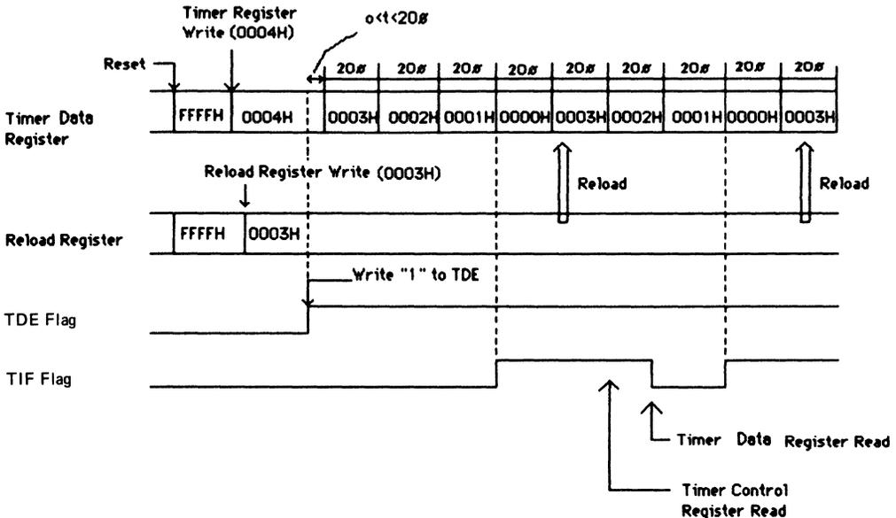
**Figure 2.12.2 Timer Operation Timing**
