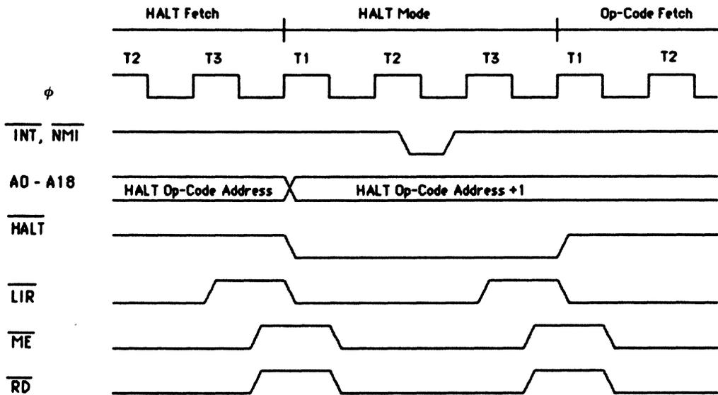
**Figure 2.4.1 HALT Timing**
