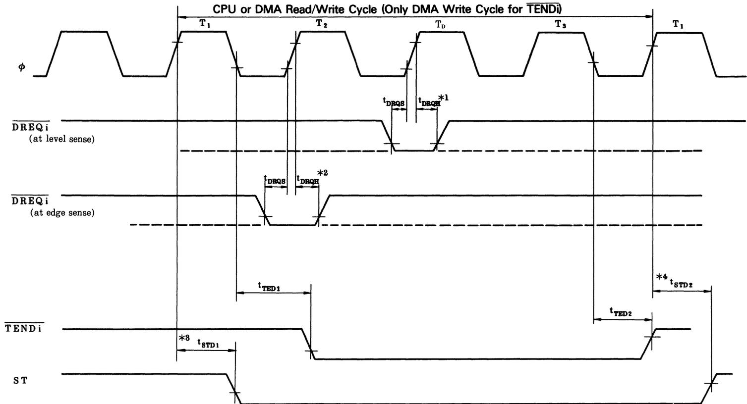
\*1  $t_{DRQS}$  and  $t_{DRQH}$  are specified for rising edge of clock followed by  $T_3$ .
