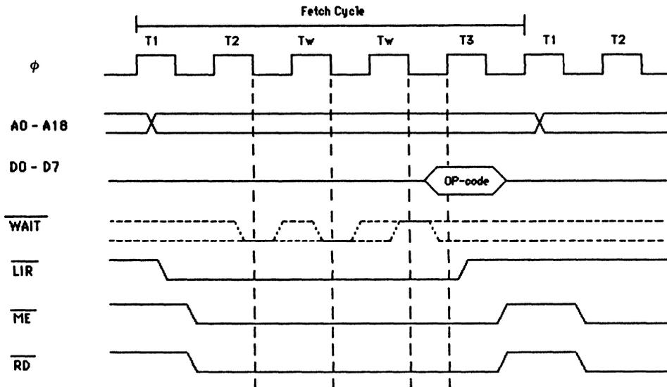
**Figure 2.2.2 Op-Code Fetch Timing (with wait state)**
