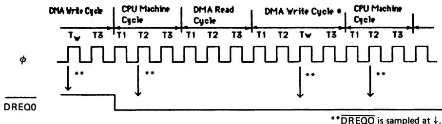
**Figure 2.9.4 CPU Operation and DMA Operation**
