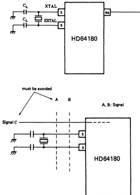
**Figure 2.14.3 Note for Board Design of the Oscillation Circuit**
