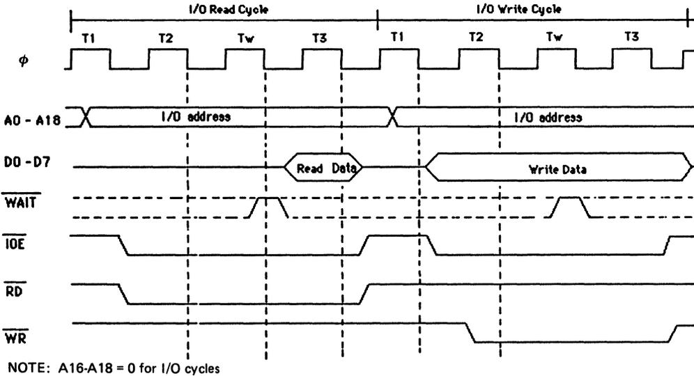
Figure 2.2.5 I/O Read/Write Timing
