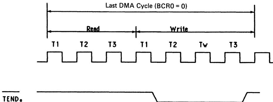
**Figure 2.9.5  $\overline{TEND0}$  Output Timing**
