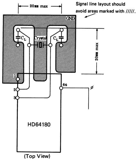
**Figure 2.14.4 Example of Board Design**
