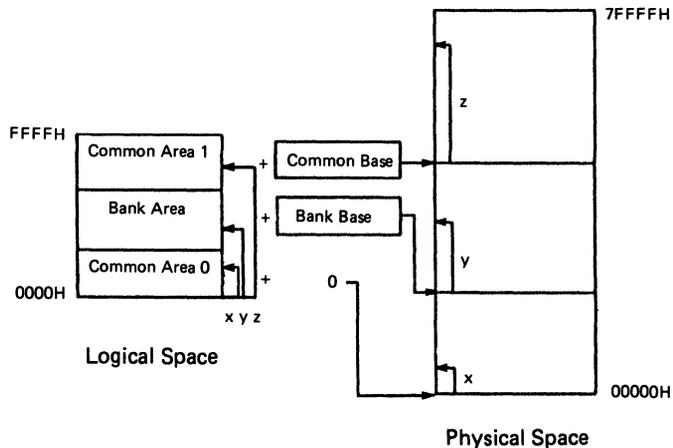
**Figure 2.6.2 Logical → Physical Memory Mapping Example**
