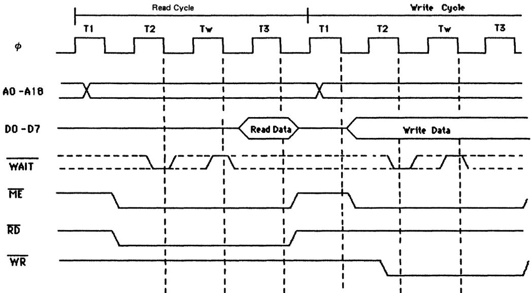
**Figure 2.2.4 Memory Read/Write Timing (with wait state)**
