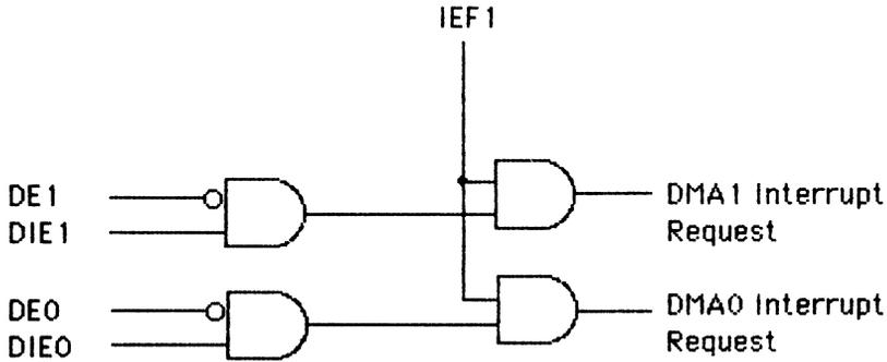
**Figure 2.9.6 DMAC Interrupt Request Circuit Diagram**
