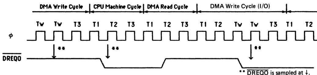
**Figure 2.9.3 CPU Operation and DMA Operation**
