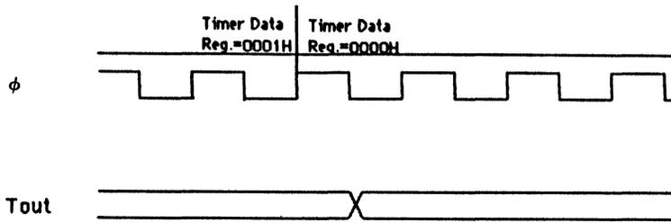
**Figure 2.12.3 Timer Output Timing**
