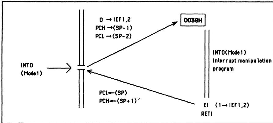
**Figure 2.7.6 INTO Mode 1 Interrupt Sequence**
