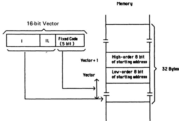
Figure 2.7.10 INT1, INT2 and Internal Interrupts Vector Acquisition
