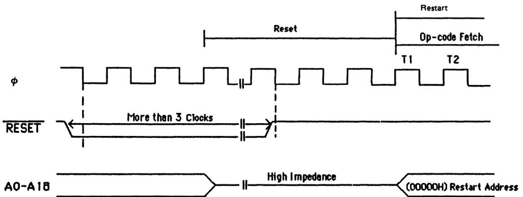
**Figure 2.2.7 RESET Timing**
