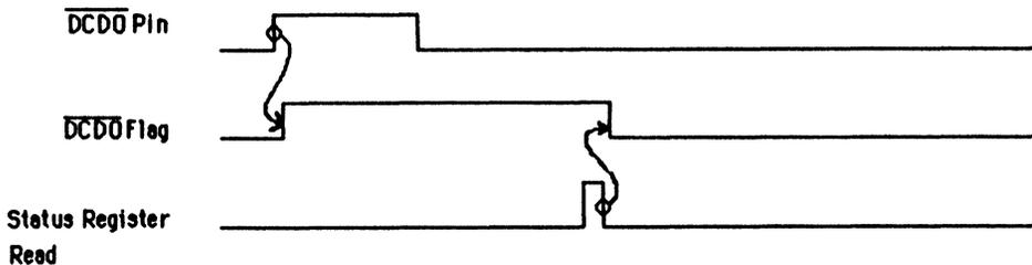
Figure 2.10.2 (a)  $\overline{\text{DCD0}}$  Timing
