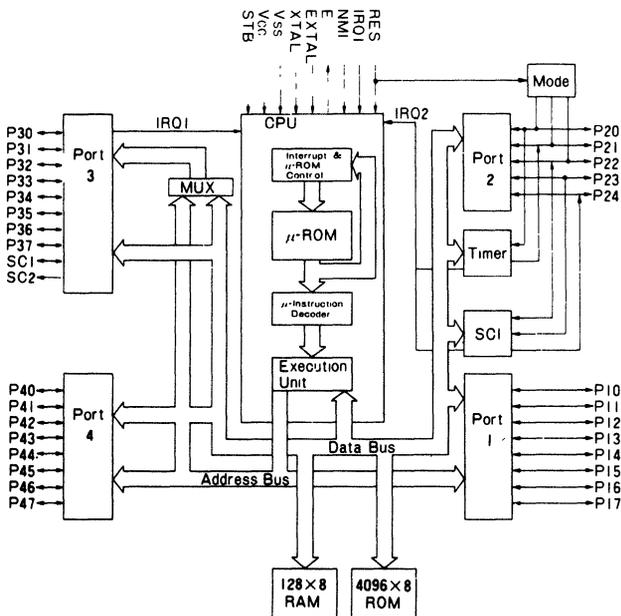
Fig. 6. Block diagram of HD6301.
