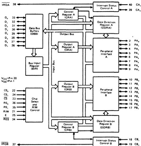
The functional configuration of the PIA is programmed by the MPU during system initialization. Each of the peripheral data lines can be programmed to act as an input or output, and each of the four control/interrupt lines may be programmed for one of several control modes. This allows a high degree of flexibility in the over-all operation of the interface.
