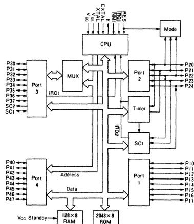
Fig. 3. Block diagram of HD6801S0.
