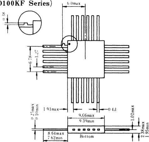
● 24 Pin Ceramic Dual-in-line Package
