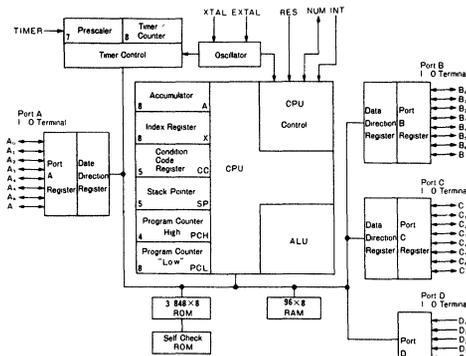
Fig. 1. Block diagram of HD6805V0.
