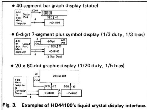
Fig. 3. Examples of HD44100's liquid crystal display interface.
