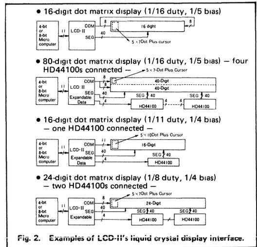
Fig. 2. Examples of LCD-II's liquid crystal display interface.
