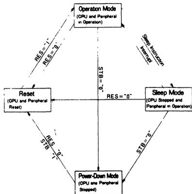
Fig. 7. Mode transition diagram of HD6301V.
