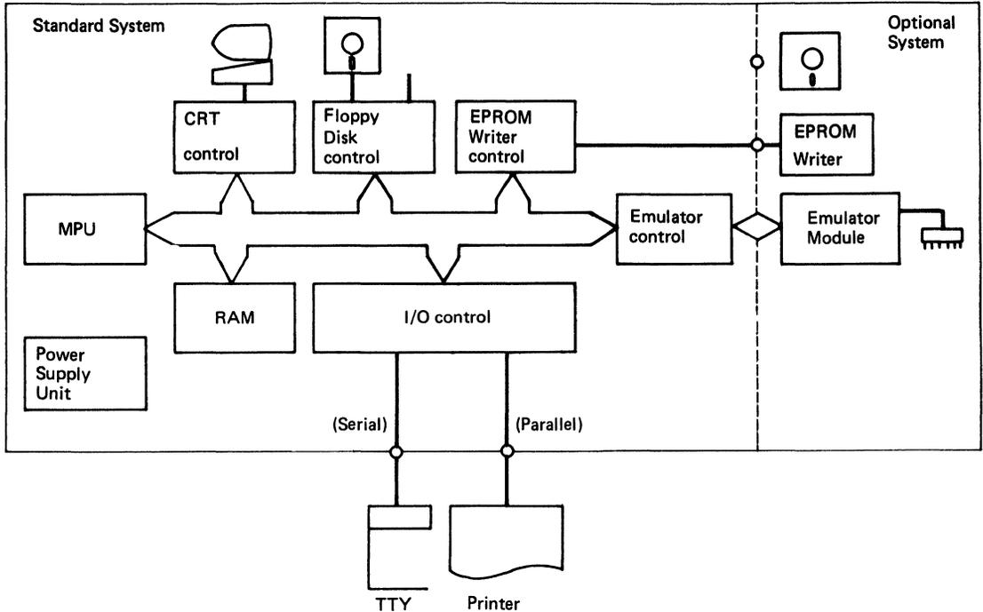
As shown in the above figure, the standard system of the H68SD5 consists of a power supply unit, 7 function blocks, a console display and one Floppy disk driver. User's system can be developed easily with this Floppy disk based system.
