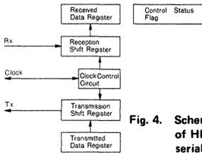
**Fig. 4. Schematic block diagram of HD6801S0 serial communication control section.**
