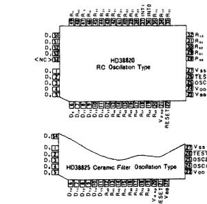
Fig. 2. Difference in pin arrangement between the RC oscillation type and ceramic filter oscillation.
