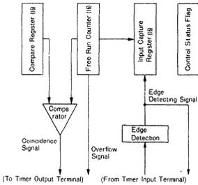
**Fig. 5. Schematic block diagram of HD6801S0 timer.**
