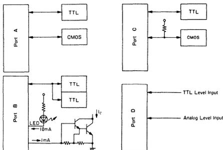
Fig. 2. An example of HD6805 family I/O ports in use.
