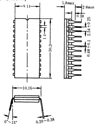
**Fig.2 Package (Dimensions in mm)**
