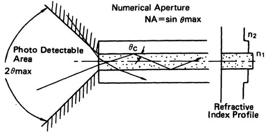
Figure 81 Structure of Step Index Fiber
