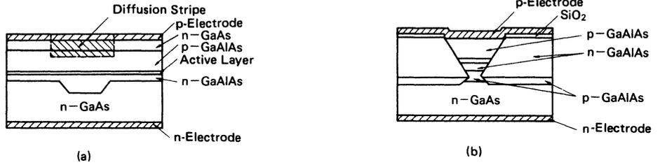
Figure 23 Various Stripe Laser Built-in Waveguide
