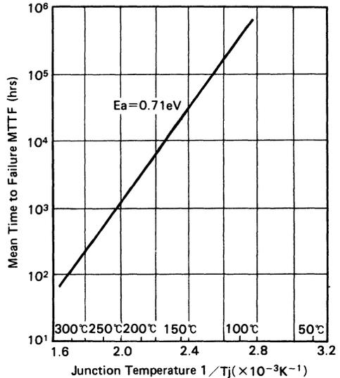
Figure 9 IRED Junction Temperature Dependency of Mean Time to Failure
