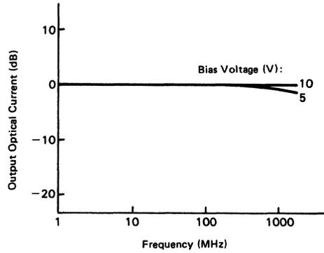
Figure 32 Frequency Response for InGaAsP/InP PIN Photodiode
