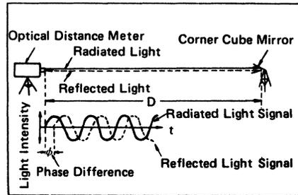
Figure 70 Light Wave Distance Meter
