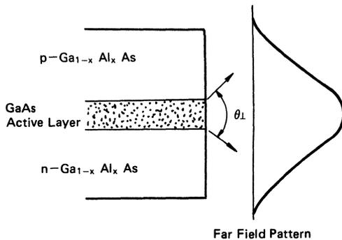
Figure 20 Perpendicular Transverse Mode
