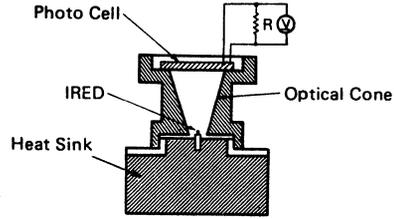
Figure 39 Measurement of Optical Output Power ( $P_O$ ) under CW Operation
