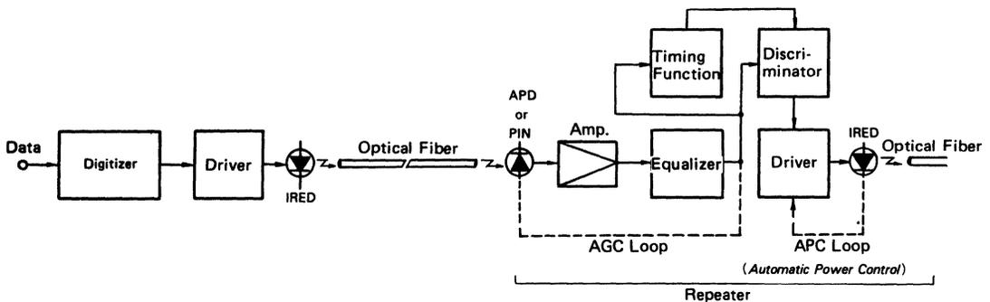
Figure 73 Digital Transmission System
