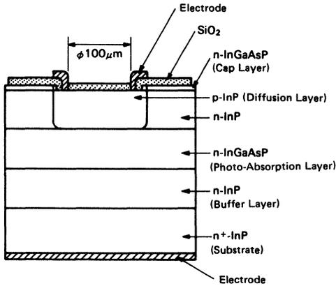
Figure 31 InGaAsP/InP PIN Photodiode Structure
