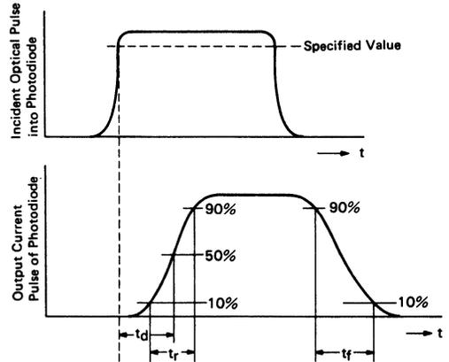
Figure 51 Definition of Photo-Detection Response time
