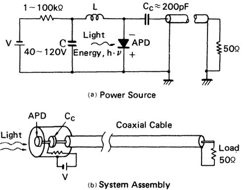
Figure 80 Receiving Unit Used with APD
