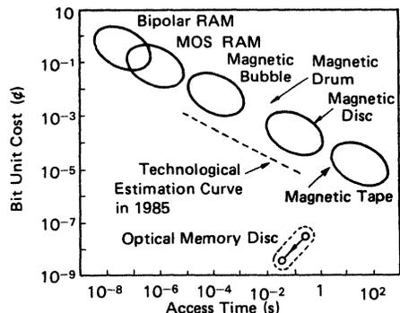
Figure 68 Access Time vs. Bit Unit Cost in Various Memory
