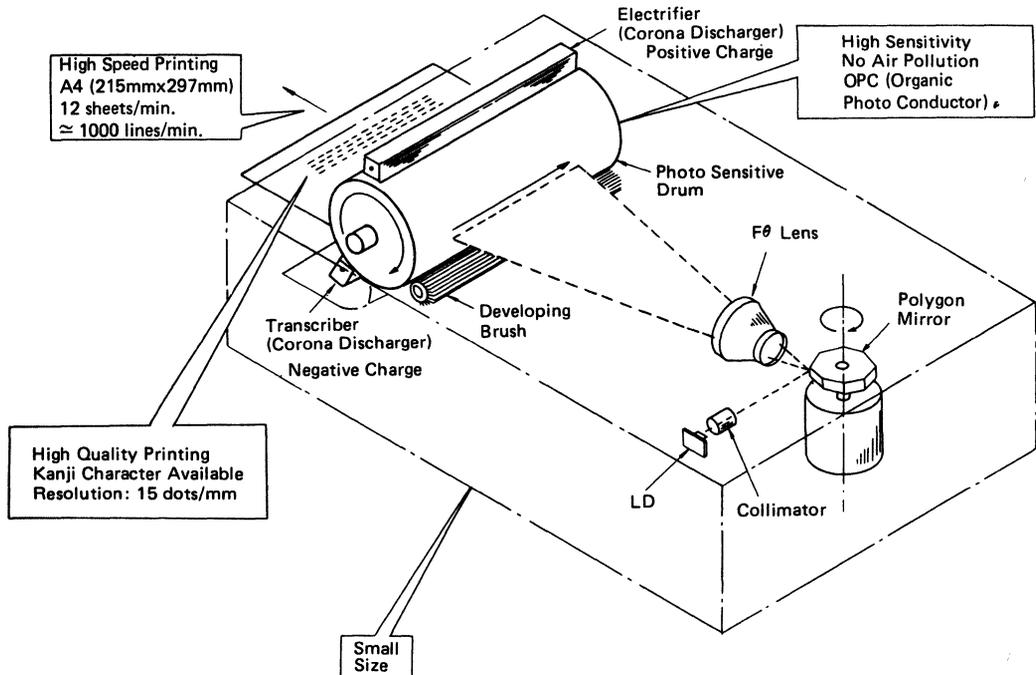
Figure 65 Structure of Laser Printer System
