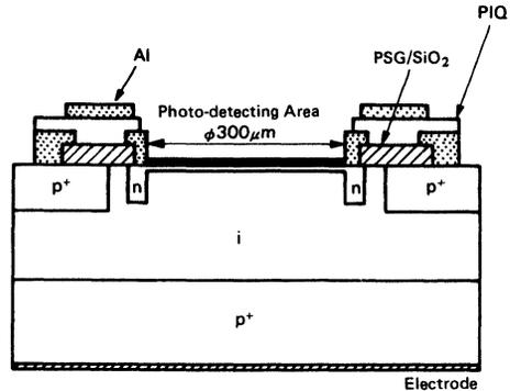
Figure 29 Si PIN Photodiode Structure
