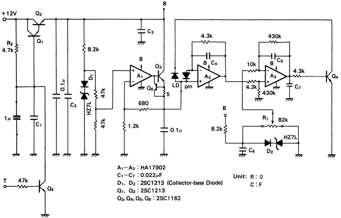
Figure 11 LD Experimental APC Circuit
