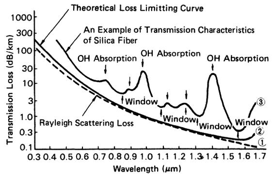
Figure 63 Transmission Loss of Typical Fiber
