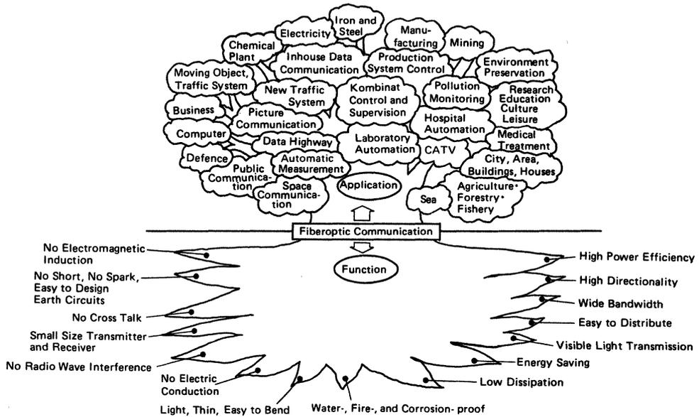
Figure 84 Optical Fiber Functions and Applications
