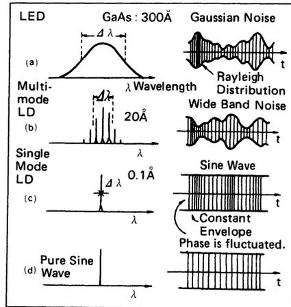
Figure 76 Spectrum of Light Carrier Wave and Modeling of Instant Waveform
