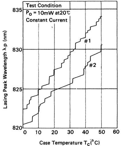
Figure 55 Temperature Dependence of Lasing Spectrum (HLP1400)
