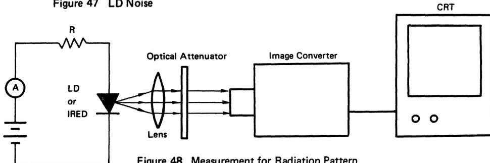
Figure 48 Measurement for Radiation Pattern
