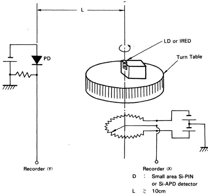
Figure 41 Measurement Setup for Far Field Pattern (FFP)
