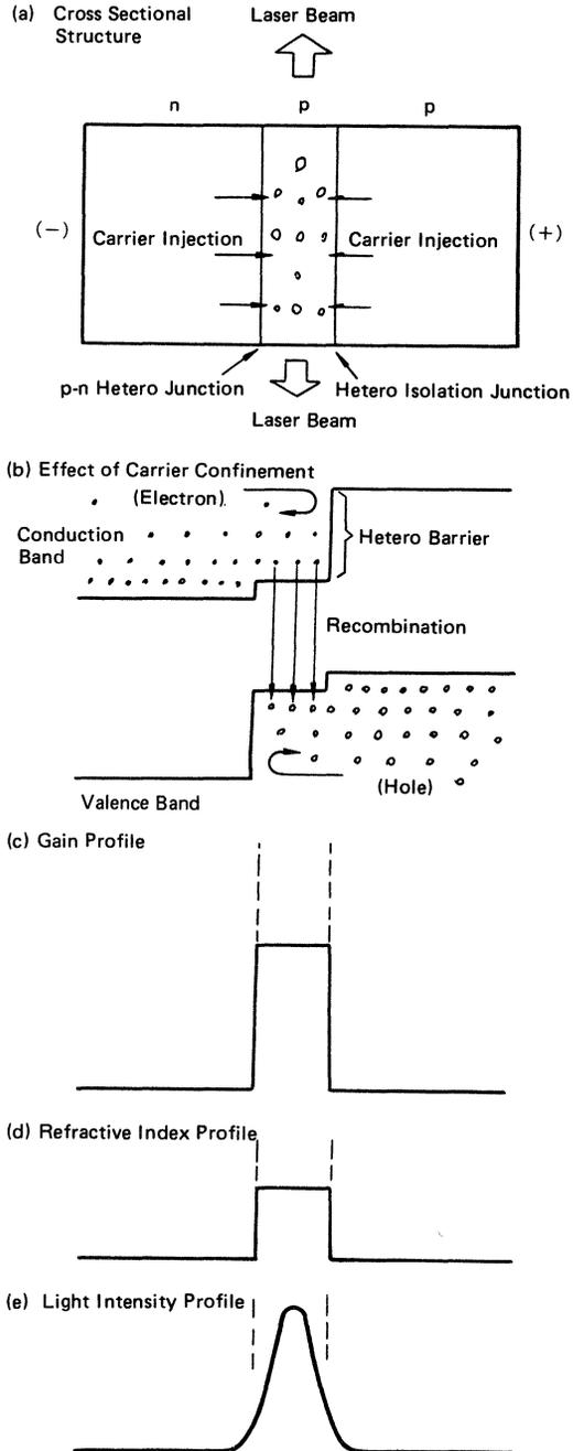
Figure 16 Operation Principle of Double Hetero Junction LD
