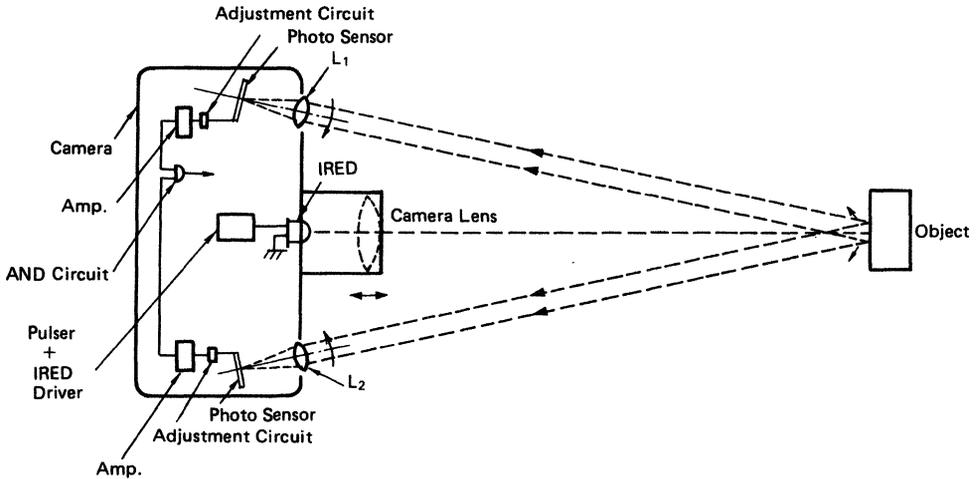
Figure 75 Operation Principle of Auto Focus Camera
