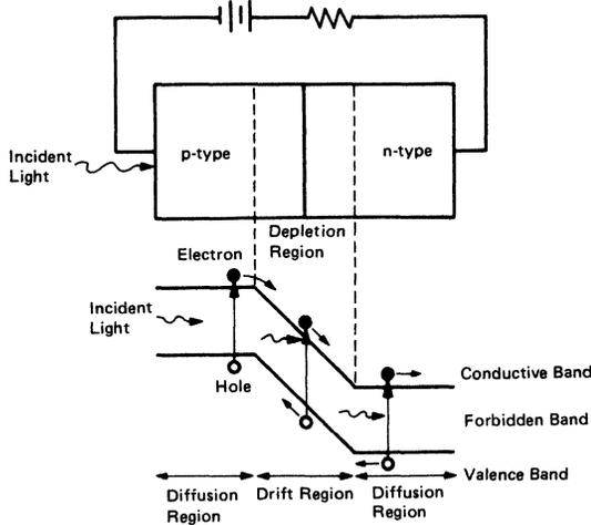
Figure 28 Photo-Detection Principle
