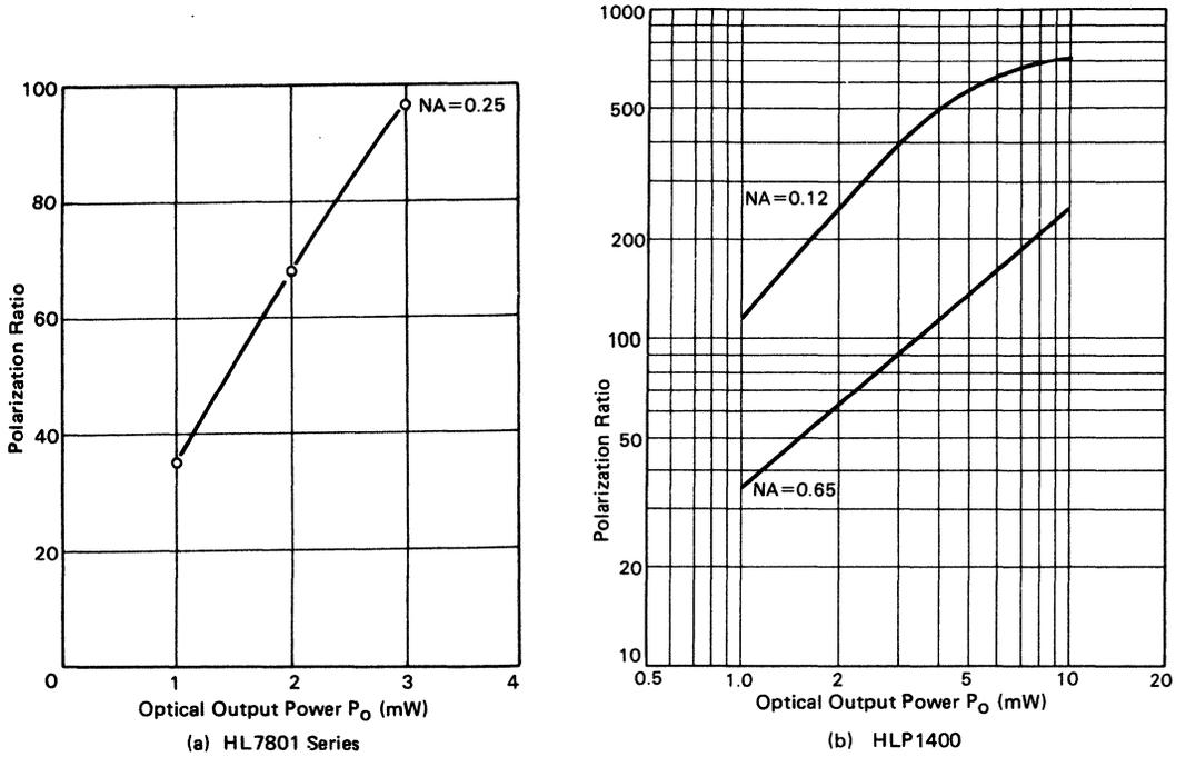
Figure 46 Output Power Dependence of Polarization Ratio
