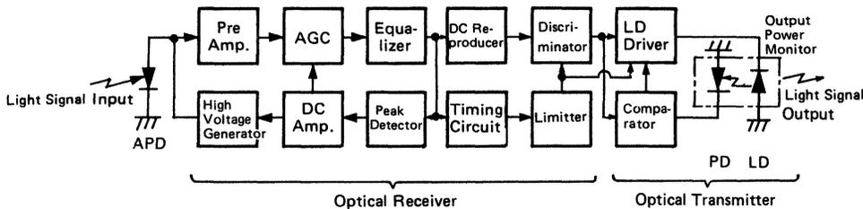
Figure 64 Block Diagram of Repeater for Digital System
