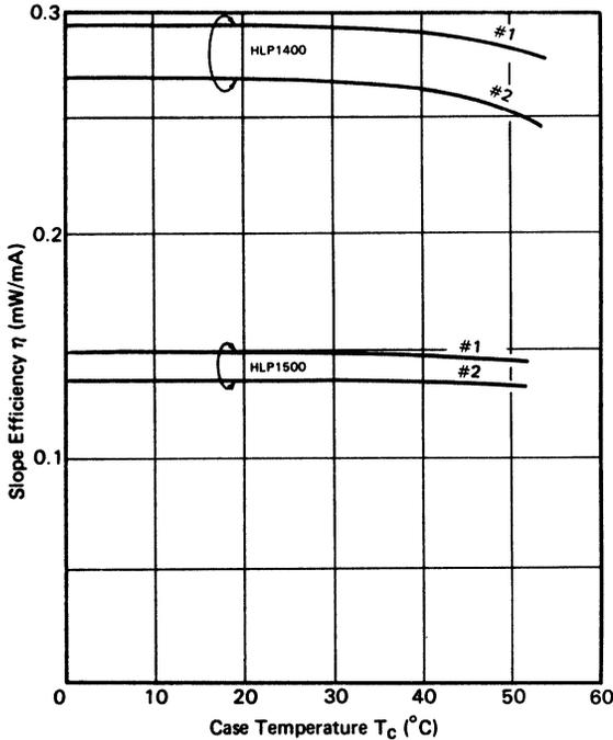
Figure 38 Temperature Dependence of Slope Efficiency
