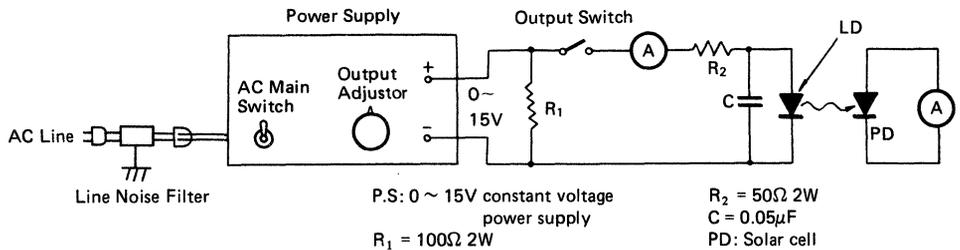
Figure 10 Simple Drive Circuit
