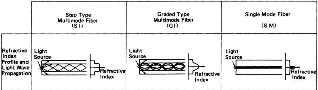
Figure 82 Classified Optical Fiber into Refractive Index Structure
