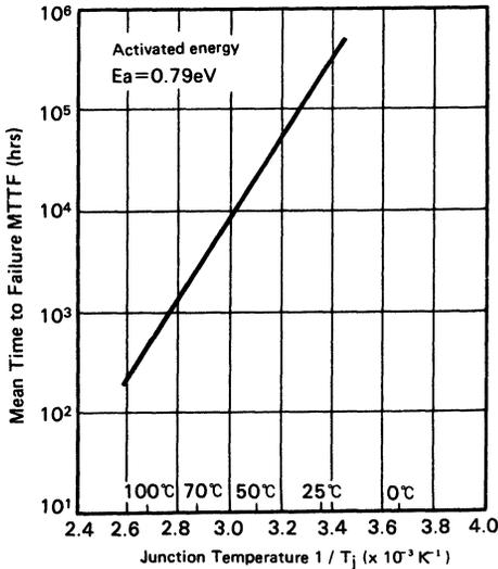
Figure 8 Example of LD Junction Temperature Dependency of Mean Time to Failure
