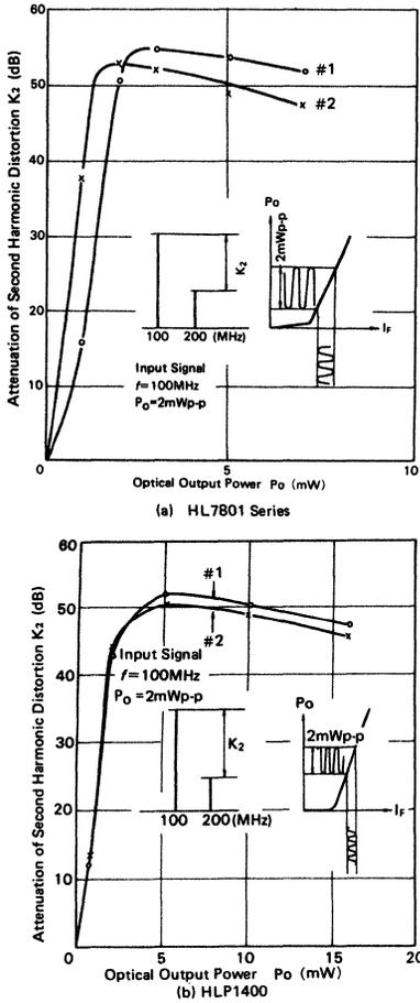
Figure 54 Second Harmonic Distortion of LD
