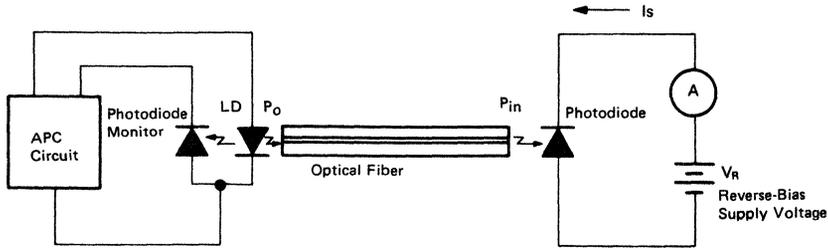
Figure 49 System for Measuring Photo-Detecting Sensitivity
