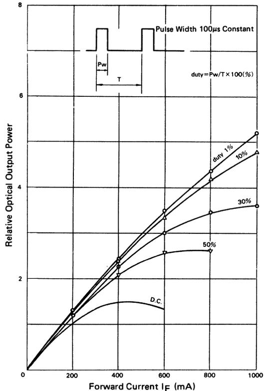
Figure 40 Light-Current Characteristics under Pulsed Operation
