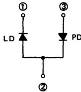
The photodetector built in for power monitoring simplifies and automatic power control circuit.
