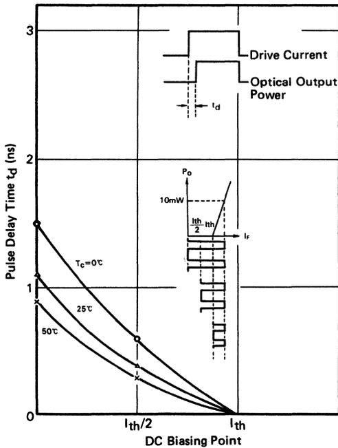
Figure 36 Bias Dependence of Pulse Delay Time (HLP1400)
