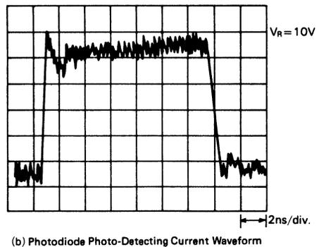
Figure 53 Photo-Detecting Response Wave for InGaAsP/InP PIN Photodiode (HR1101)
