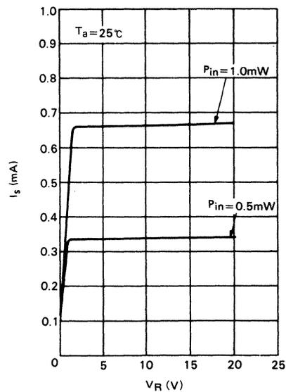
(b) InGaAsP/InP PIN Photodiode (HR1101)
