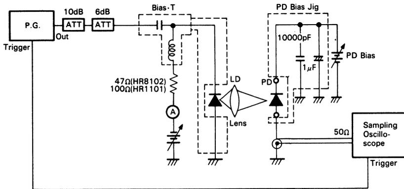
Figure 52 Setup for measuring Photo-Detection Response
