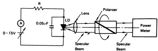
Figure 44 Measurement Setup for Polarization Ratio
