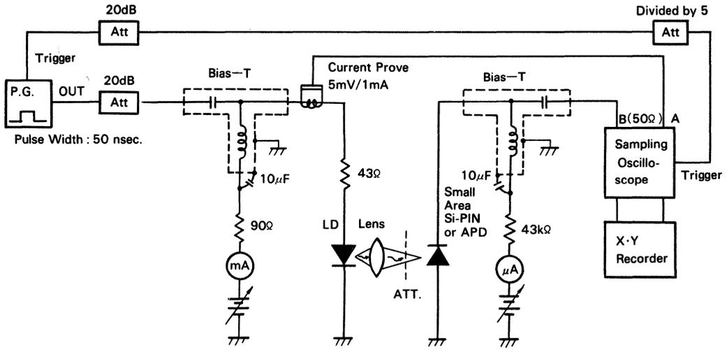
Figure 35 Measurement Setup for Fast Pulse Response
