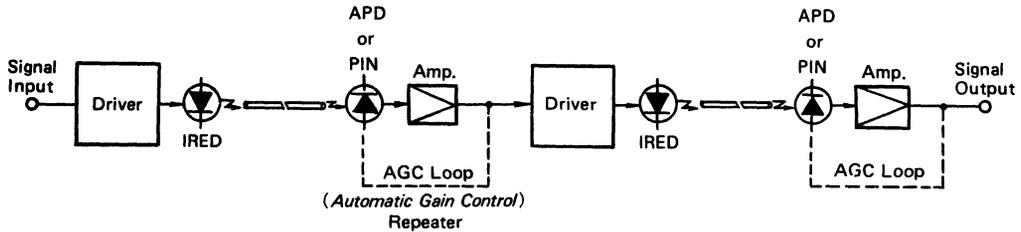
Figure 72 Direct Modulation Method Analog Transmission System
