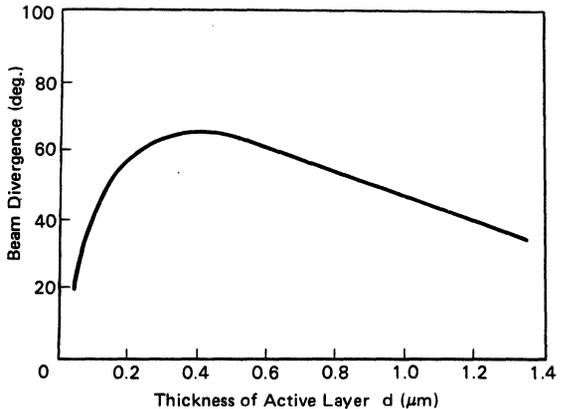
Figure 21 Thickness of Active Layer – Beam Divergence
