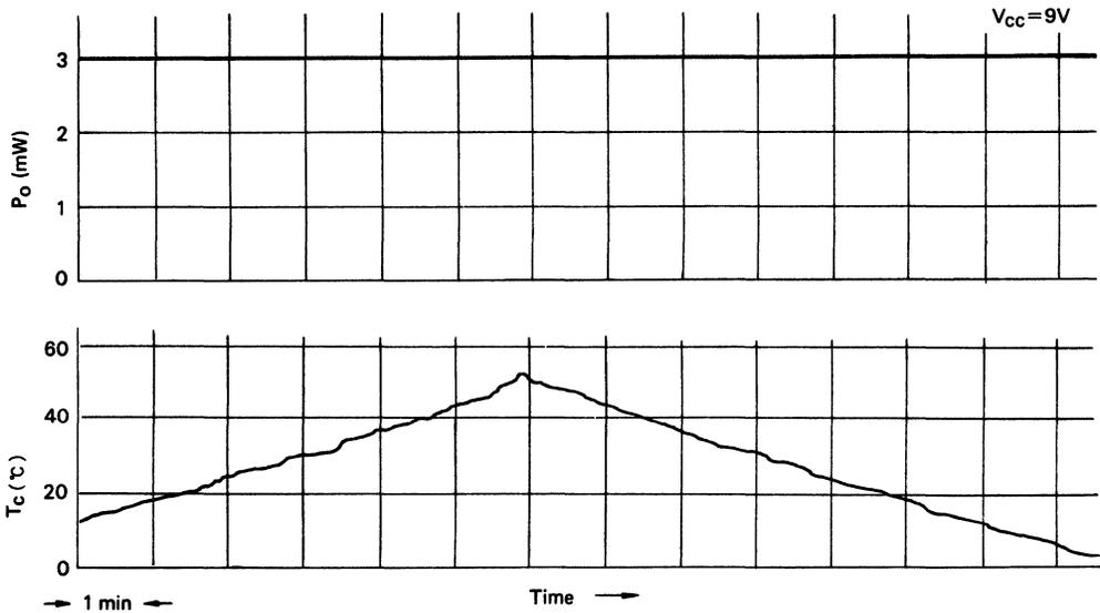
Figure 12 Temperature Characteristics of LD with APC Circuit (HL7801E)
