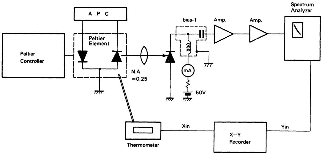
(a) Measurement Setup for Noise
