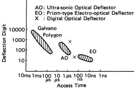
Figure 79 Diagram of Deflection Digit vs. Access Time
