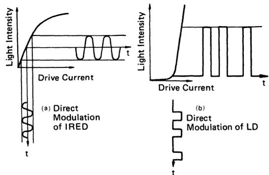
Figure 78 Principle of Direct Modulation
