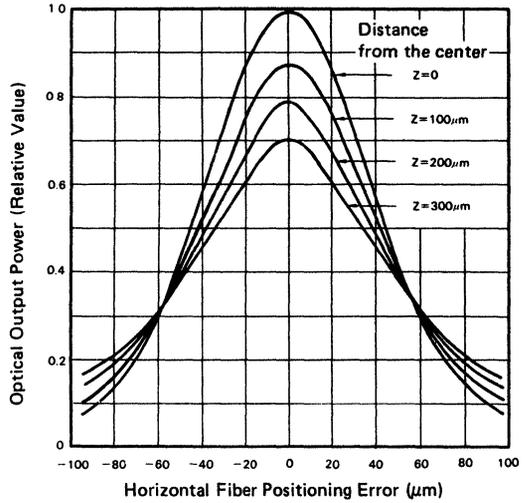
Figure 57 Relative Intensity vs. Horizontal Fiber Positioning
