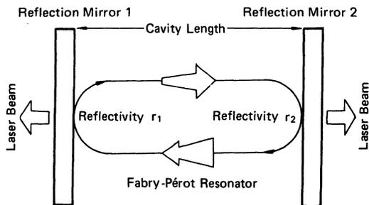
Figure 15 Fundamental Structure of Fabry-Pérot Resonator
