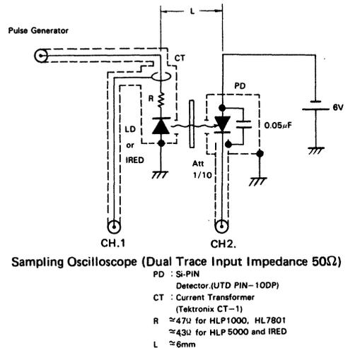
Figure 34 Measurement Setup for Light-Current Characteristics under Low Frequency Pulsed Operation
