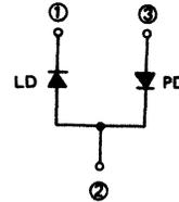
The photodetector built in for power monitoring simplifies an automatic power control circuit.
