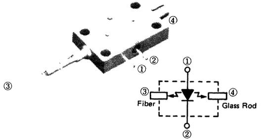
A monitor output guide is provided for external monitoring.
