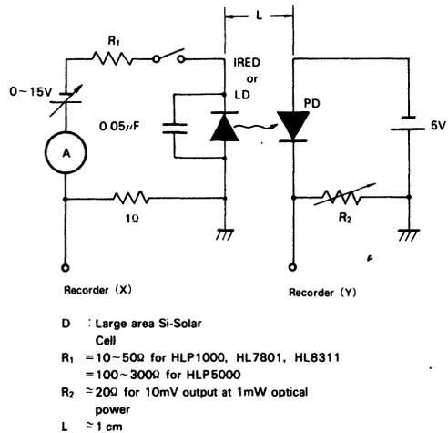
Figure 33 Measurement Setup for Light-Current Characteristics under CW Operation
