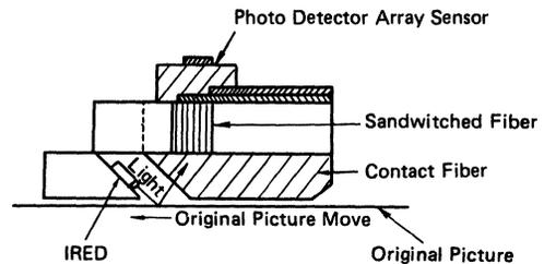
Figure 74 Principle of Contact Type Facsimile Pick-up Head
