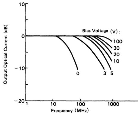
Figure 30 Frequency Response for Si PIN Photodiode
