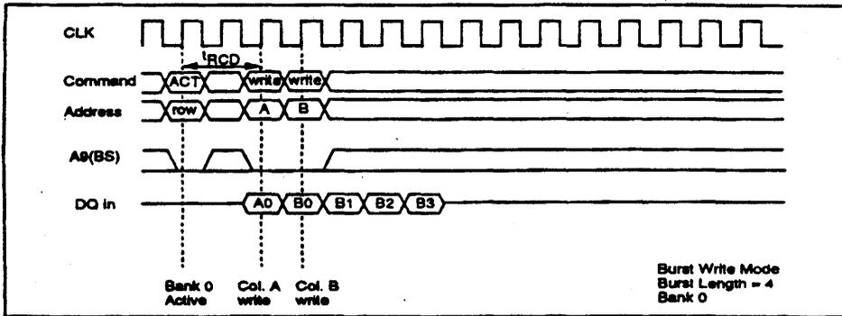
(2) Operation for the column in other ROW of the same bank: To write data on other row of the same bank, it is necessary to execute a precharge command and bank active command before executing next write command.
