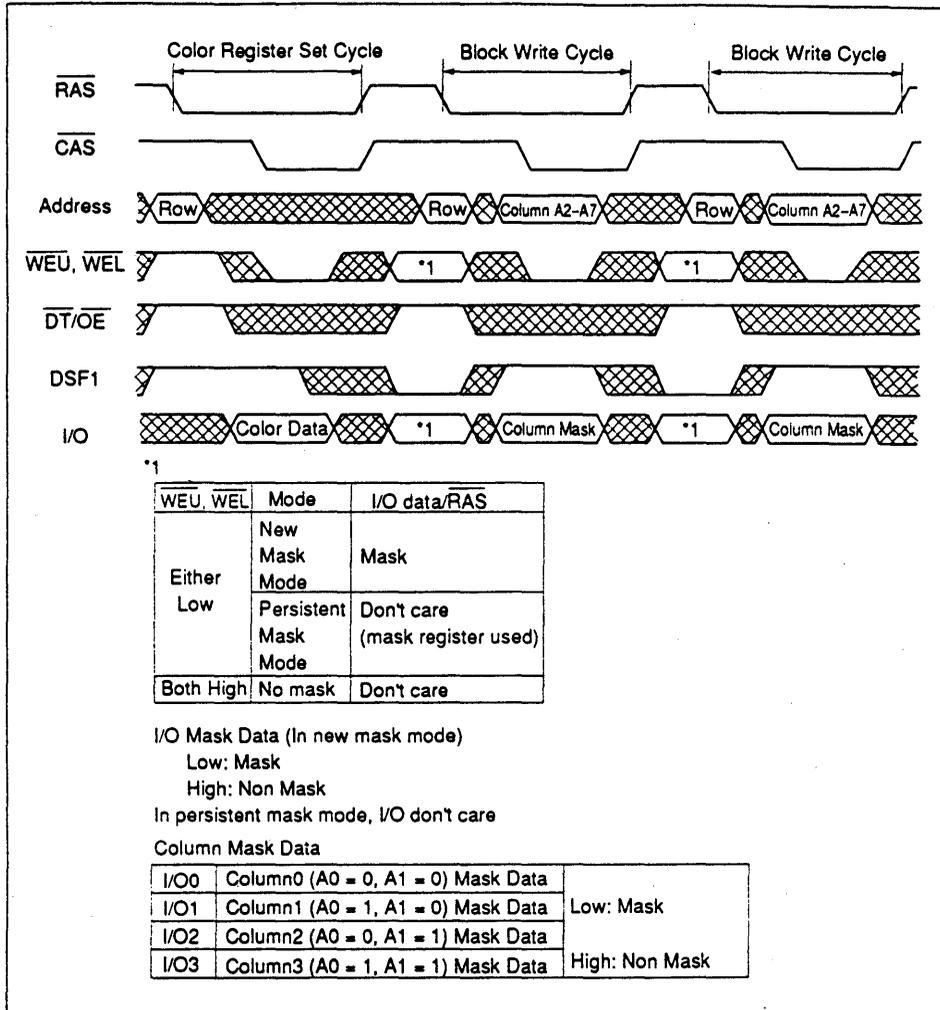
Figure 2 Use of Block Write
