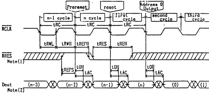
Notes: 1. The read address counter is reset at the first falling edge of RCLK after RRES falls, meeting the specifications of tREPS and tREPH, and it is not reset at the next falling edge of RCLK even if RRES is kept low.
