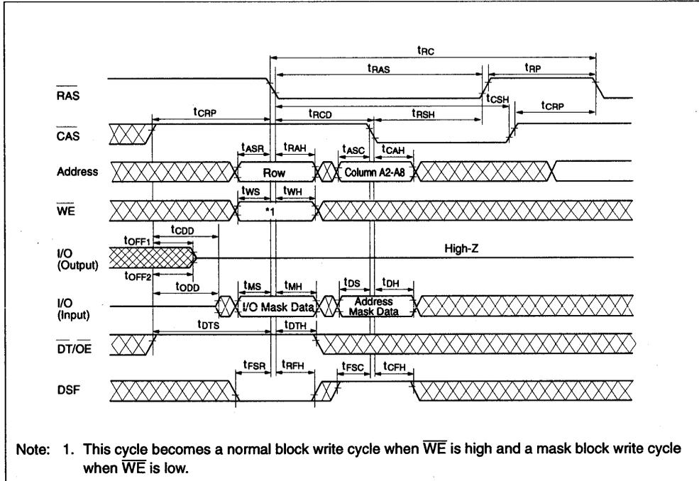
Note: 1. This cycle becomes a normal block write cycle when  $\overline{WE}$  is high and a mask block write cycle when  $\overline{WE}$  is low.
