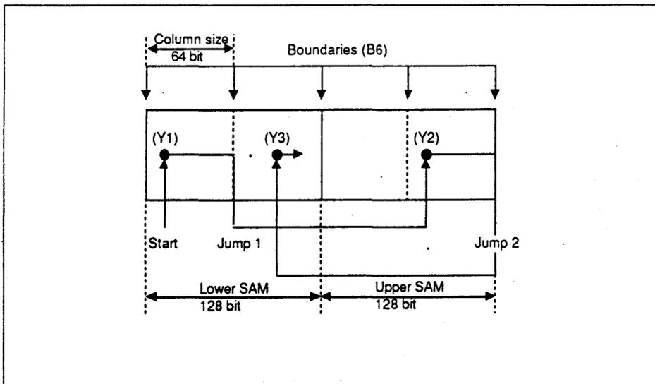
Figure 6 Example of Boundary Split Register
