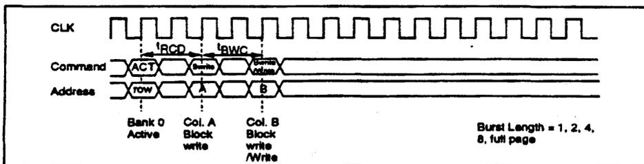
(2) Operation for the column in other ROW of the same bank: To execute write command or another block write command for other row of the same bank, It is necessary to execute a precharge command and bank active command before write or block write operation.
