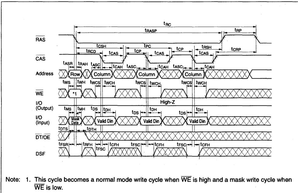
Note: 1. This cycle becomes a normal mode write cycle when  $\overline{WE}$  is high and a mask write cycle when  $\overline{WE}$  is low.
