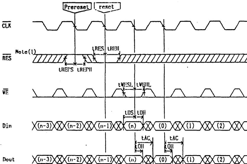
**Note:** The read address counter is reset at the first falling edge of CLK after RES falls, meeting the specifications of  $t_{REPS}$  and  $t_{REPH}$ , and it is not reset at the next falling edge of CLK even if RES is kept low.
