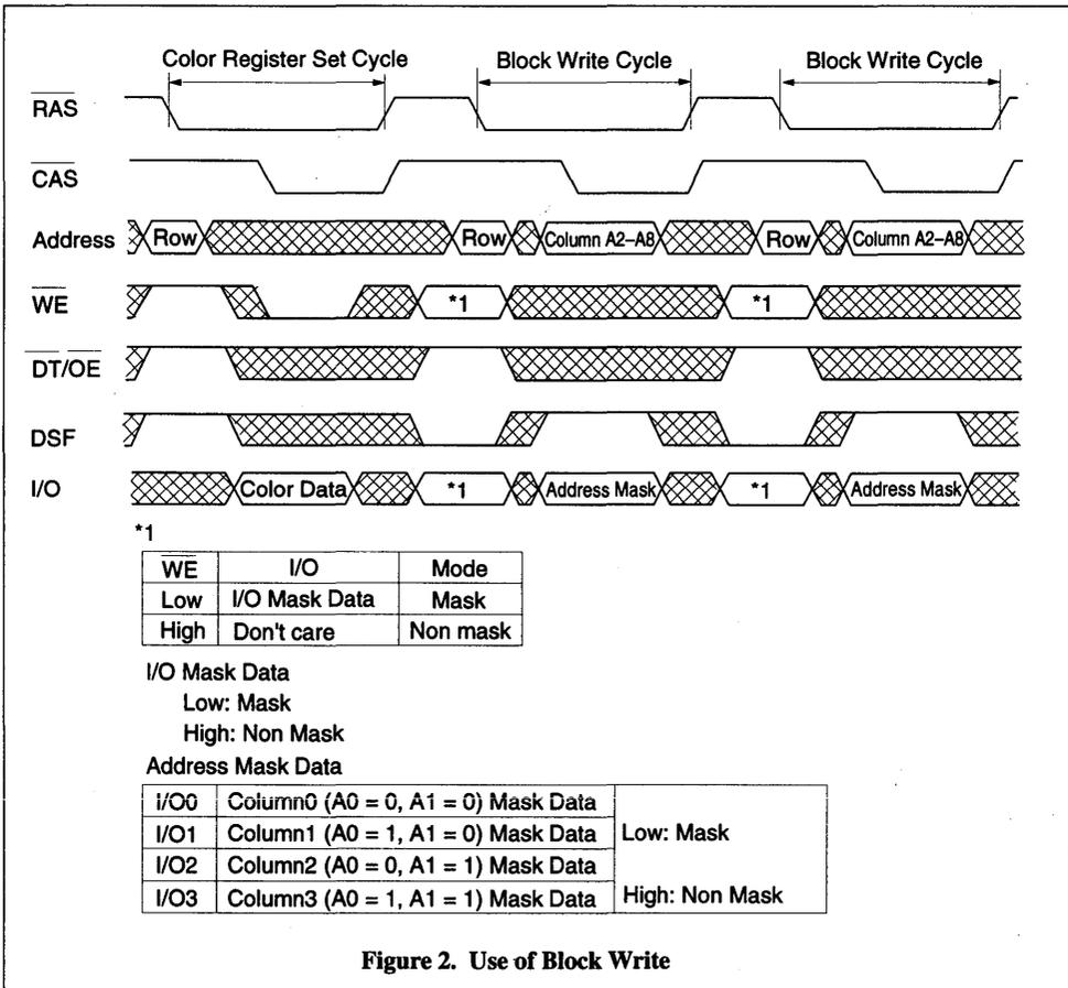
Figure 2. Use of Block Write
