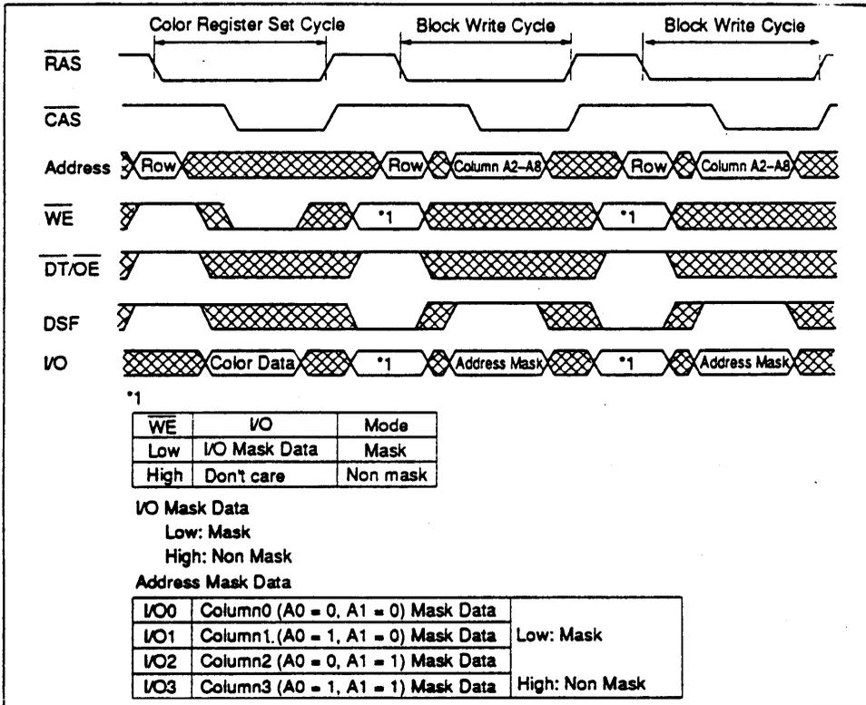
Figure 2 Use of Block Write
