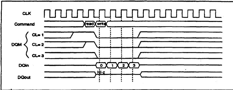
(2) Operation for the column in other ROW of the same bank: To execute write or block write for other row of the same bank, it is necessary to execute a precharge command and bank active command before executing these commands.
