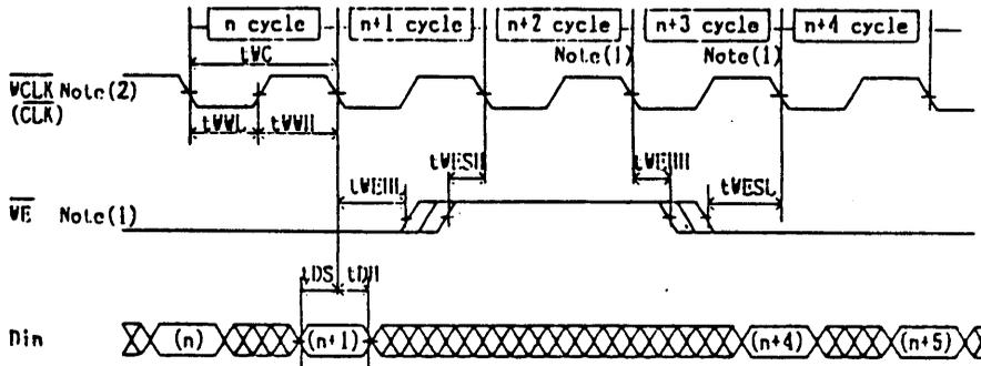
Notes: 1. When  $t_{WEHL}$ ,  $t_{WESH}$ ,  $t_{WEHH}$ , and  $t_{WESL}$  cannot meet this specifications, the write enable operation is not guaranteed.
