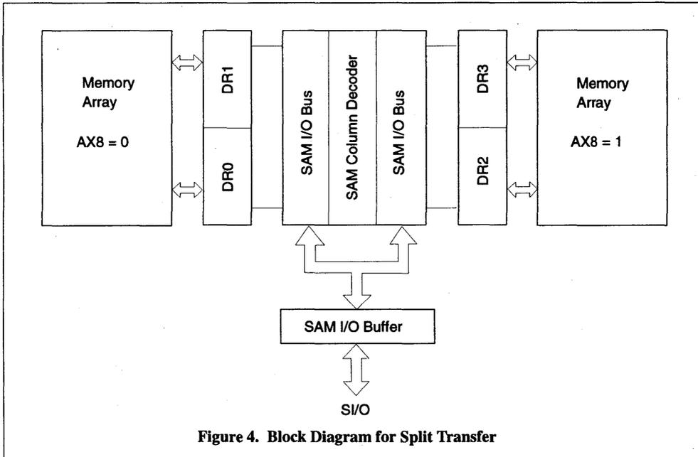
**Figure 4. Block Diagram for Split Transfer**
