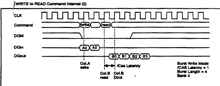
(2) Operation for the column in other ROW of the same bank: To execute read command for other row of the same bank, it is necessary to execute a precharge command and bank active command.
