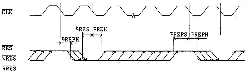
\* Hitachi recommends that  $t_m$  (time between mode set and the first cycle (Pre-reset)) should be kept for 2 cycle time (56 ns/68 ns /90 ns) or more while the power supply is on.
