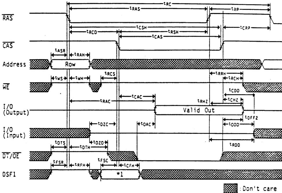
Note: 1. State of DSF1 at falling edge of  $\overline{\text{CAS}}$
