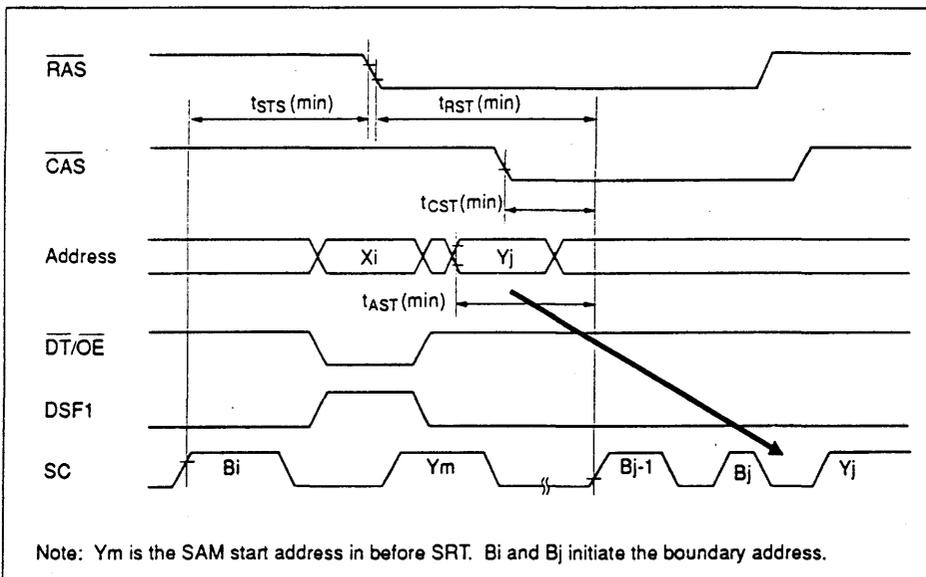
Note:  $Y_m$  is the SAM start address in before SRT.  $B_i$  and  $B_j$  initiate the boundary address.
