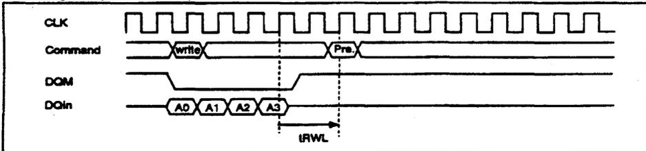
**Command intervals(cont.)****.Block write command to precharge command interval:**
