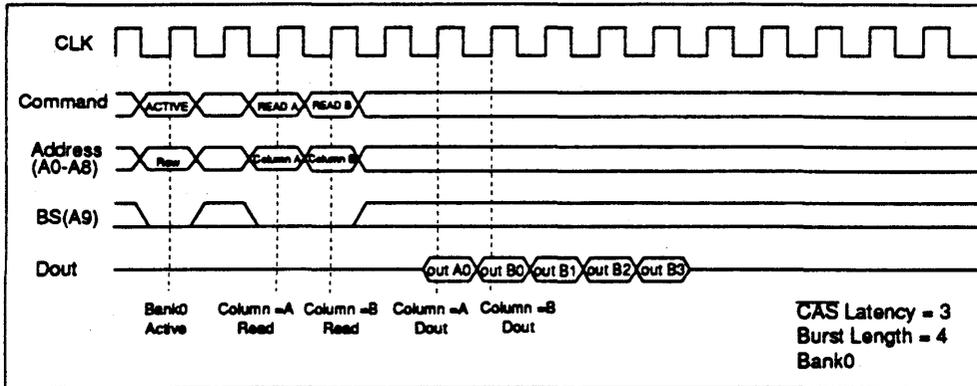
(2) **Same bank, different ROW address:** When the ROW address changes on same bank, consecutive read commands cannot be executed; it is necessary to separate the two read commands with a precharge command and a bank-active command.
