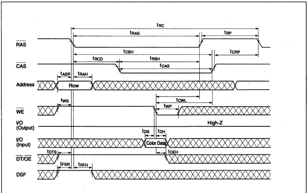
Color Register Set Cycle (Delayed Write)
