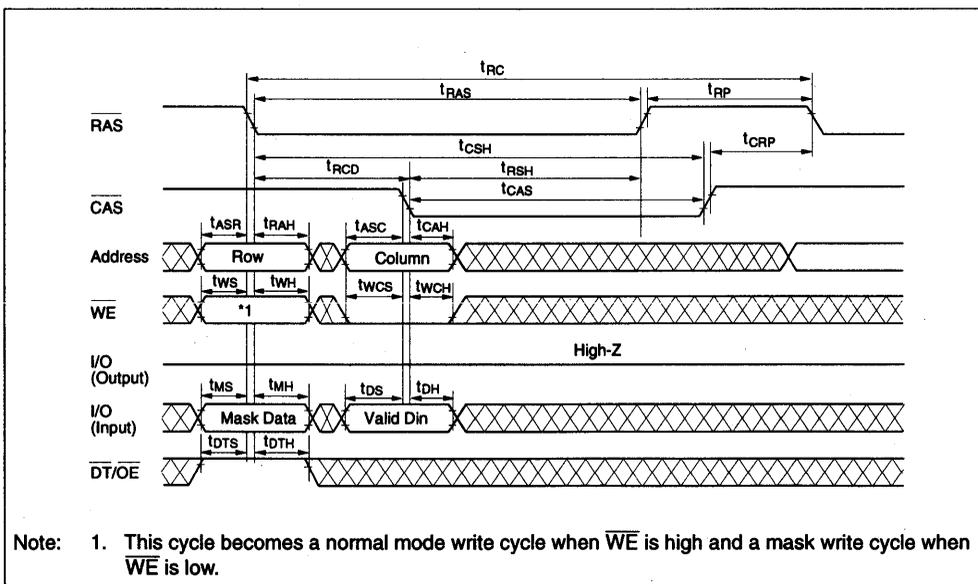
Note: 1. This cycle becomes a normal mode write cycle when  $\overline{WE}$  is high and a mask write cycle when  $\overline{WE}$  is low.
