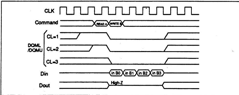
**(2) Same bank, different ROW address:** When the ROW address changes, consecutive write commands cannot be executed; it is necessary to separate the two write commands with a precharge command or a bank-active command.
