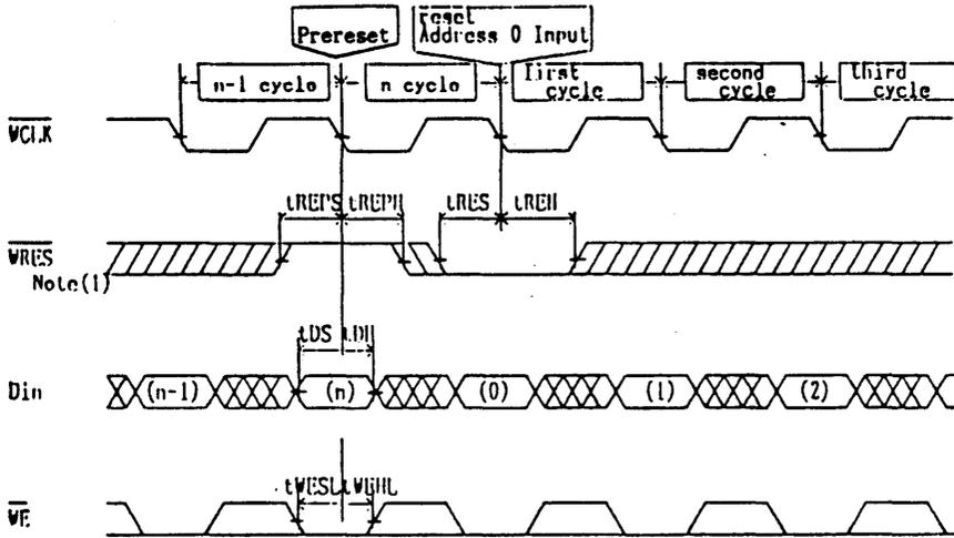
**Note:** The write address counter is reset at the first falling edge of WCLK after WRES falls, meeting the specifications of  $t_{REPS}$  and  $t_{REPH}$ , and it is not reset at the next falling edge of WCLK even if WRES is kept low.
