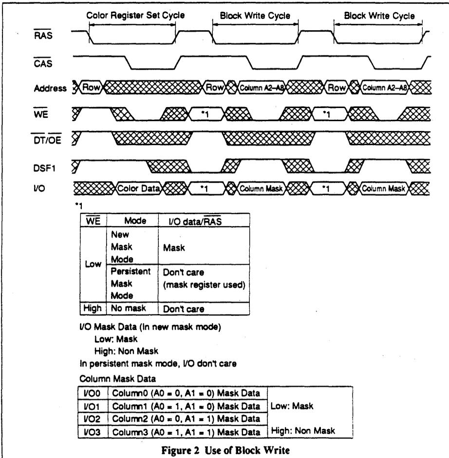
Figure 2 Use of Block Write
