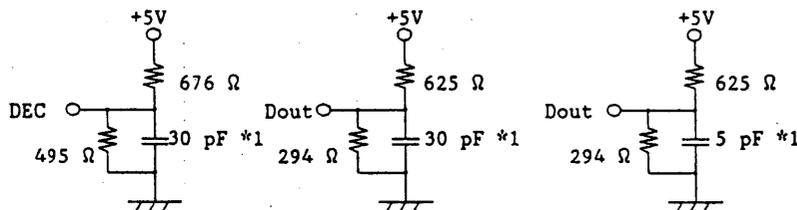
DEC output load    Dout output load (A)    Dout output load (B)
