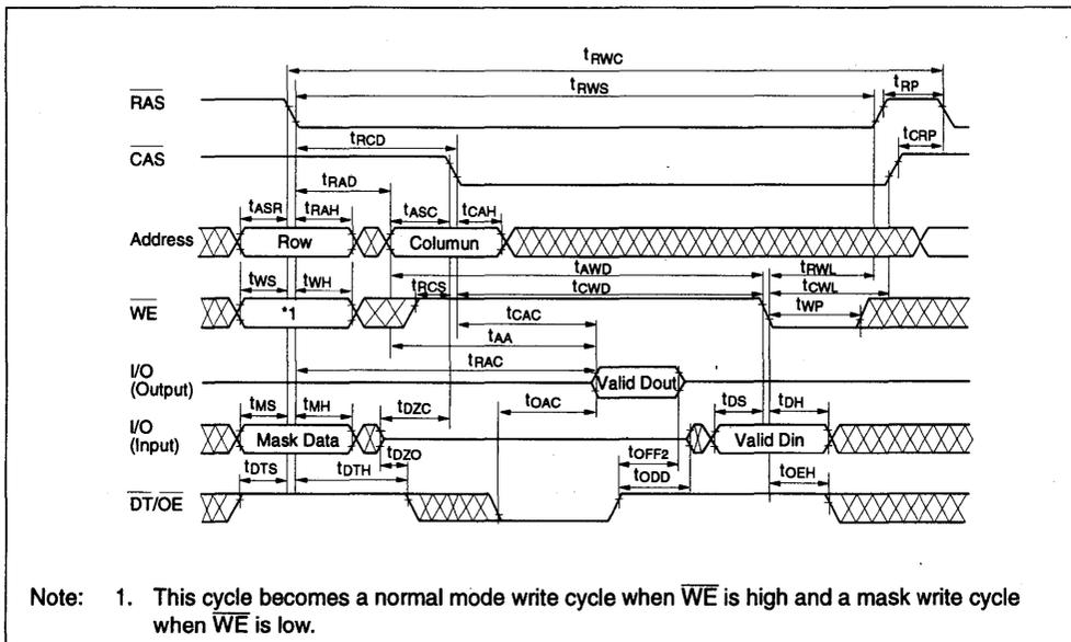
Page Mode Write Cycle (Delayed Write)
