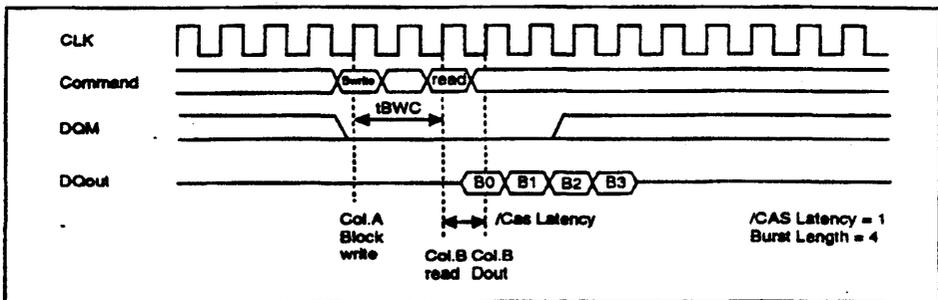
(2) Operation for the column in other ROW of the same bank: To execute read command for other row of the same bank, it is necessary to execute a precharge command and bank active command before write or block write operation.
