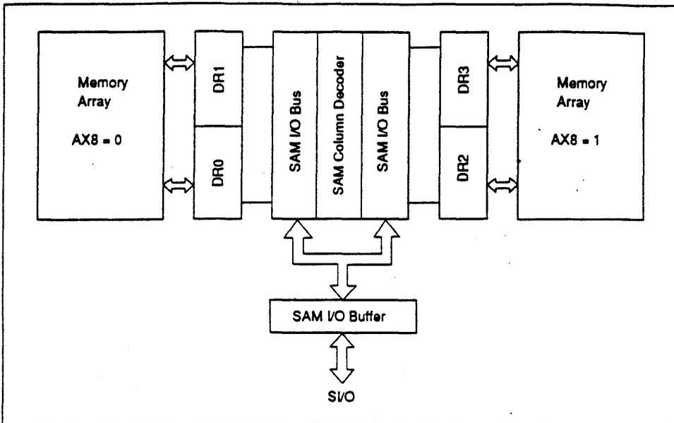
Figure 4 Block Diagram for Split Transfer
