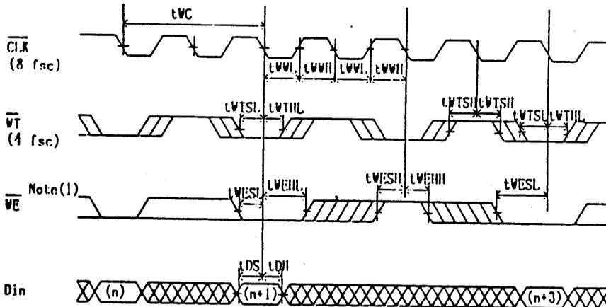
Note: When  $t_{WTSL}$ ,  $t_{WTHL}$ ,  $t_{WEHL}$ , and  $t_{WEHH}$  cannot meet the specifications, the write enable operation is not guaranteed.
