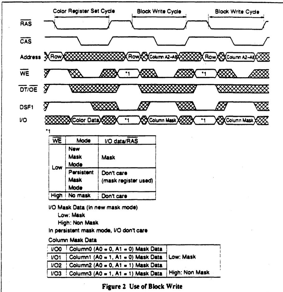
Figure 2 Use of Block Write
