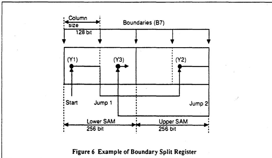
Figure 6 Example of Boundary Split Register
