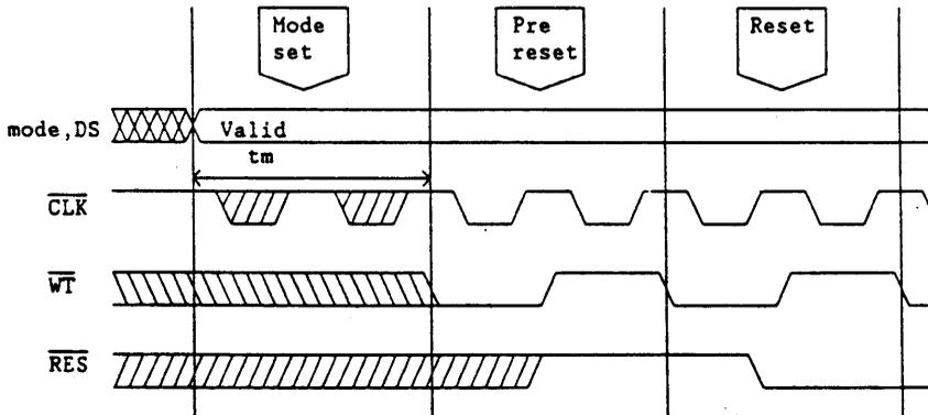
Note: When mode pins are fixed with  $V_{CC}$ ,  $V_{SS}$  in mode set while the power supply is on,  $t_m$  spec is not needed.
