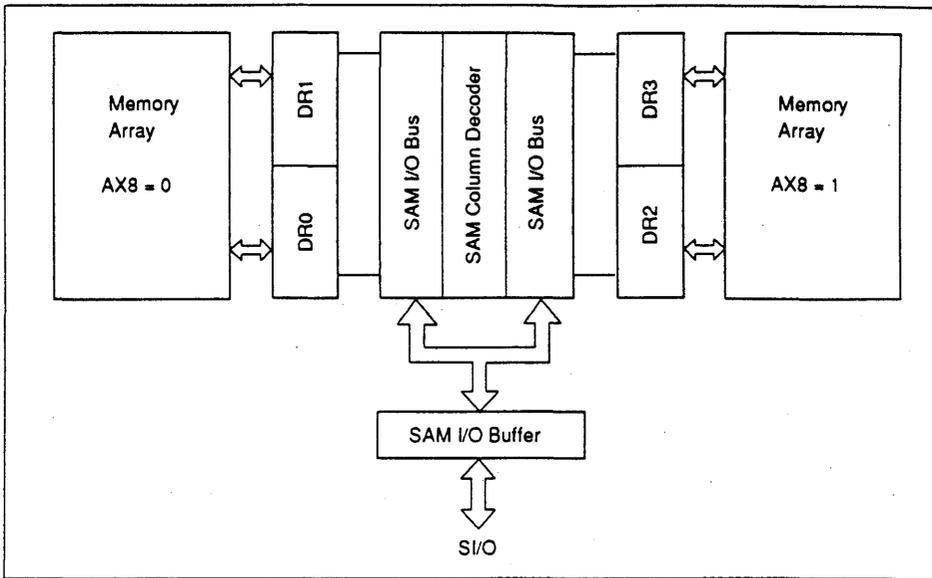
Figure 4 Block Diagram for Split Transfer
