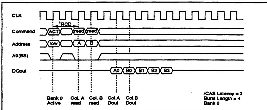
(2) Operation for the column in other ROW of the same bank: To read the data of other ROW of the same bank, it is necessary to execute a precharge command and a bank-active command before executing next read command.
