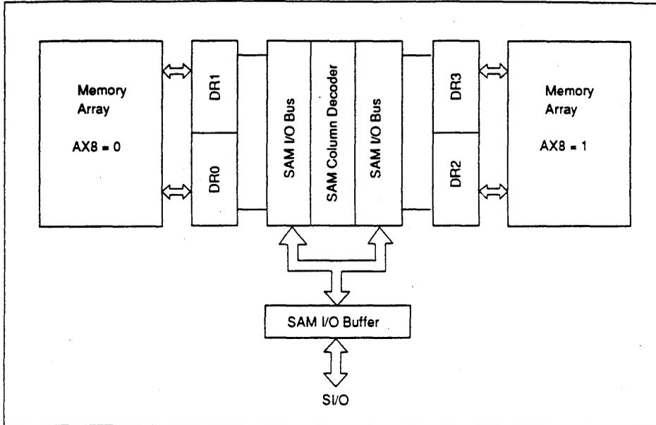
Figure 4 Block Diagram for Split Transfer
