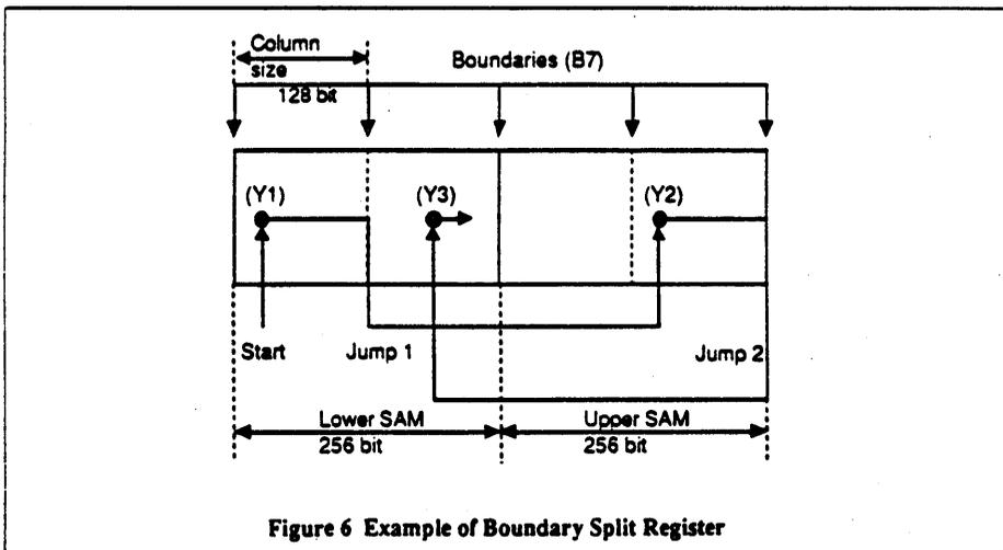
Figure 6 Example of Boundary Split Register
