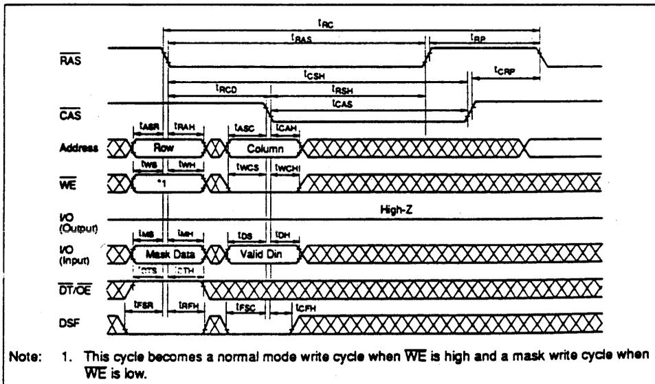
Note: 1. This cycle becomes a normal mode write cycle when WE is high and a mask write cycle when WE is low.
