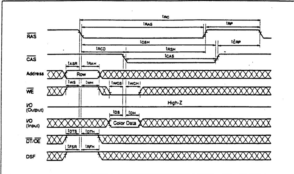
Color Register Set Cycle (Delayed Write)
