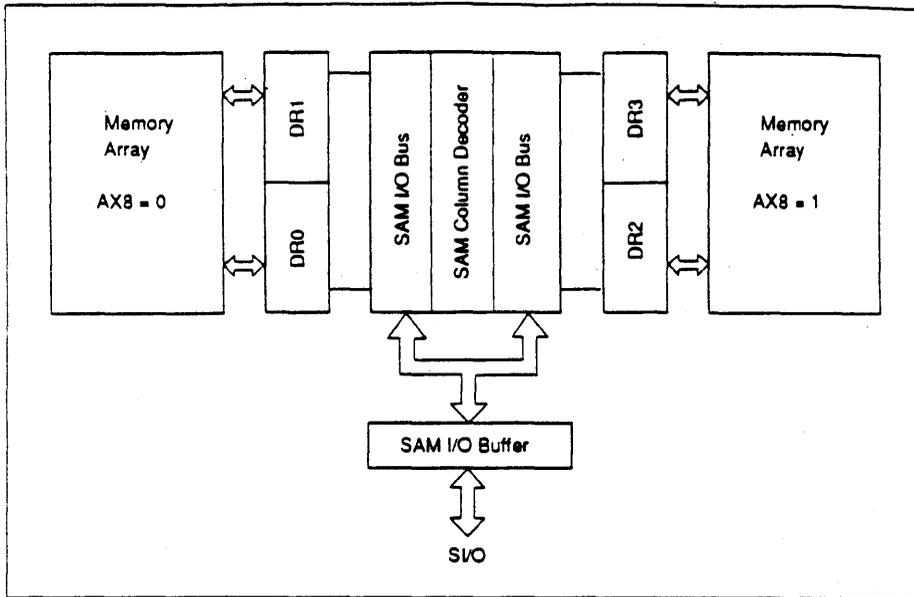
Figure 4 Block Diagram for Split Transfer
