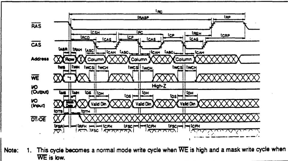
Note: 1. This cycle becomes a normal mode write cycle when WE is high and a mask write cycle when WE is low.
