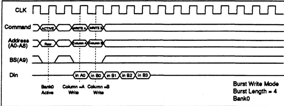
(2) Same bank, different ROW address: When the ROW address changes, consecutive write commands cannot be executed; it is necessary to separate the two write commands with a precharge command and a bank-active command.
